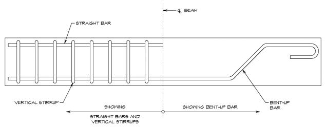
Figure 1. Illustration. Vertical Stirrups and Bent-up Longitudinal Bars.
