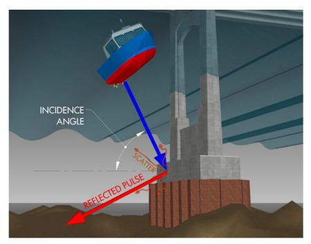
Figure 4. Graphic. Incidence angle.
