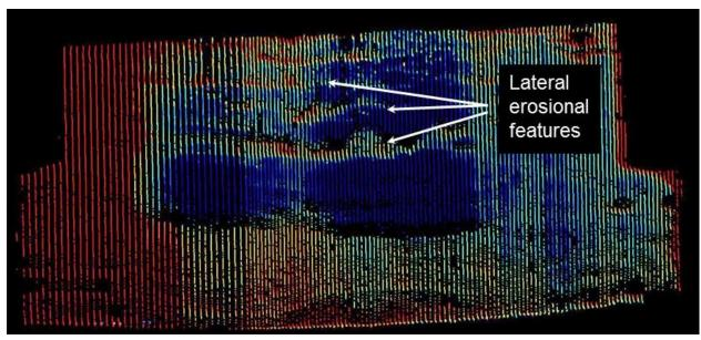
Figure 88. Image. 2D multibeam point cloud data of the east face of the W2 pier.
