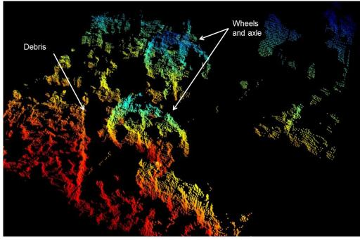
Figure 81. Image. Detail at bed near pier W2.
