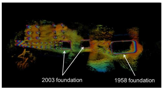
Figure 64. Image. Tower 3 plan view.
