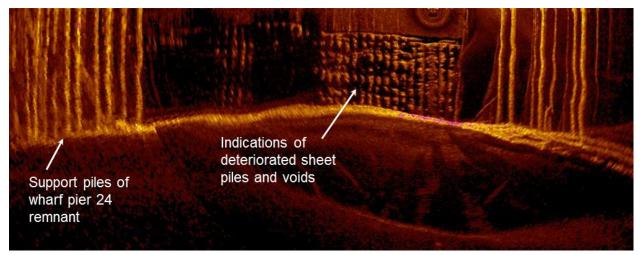
Figure 82. Image. Southeast corner of pier W2.
