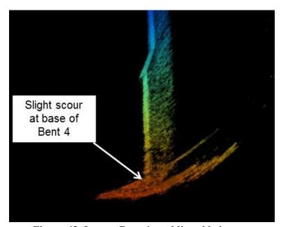
Figure 42. Image. Bent 4 mud line side image.
