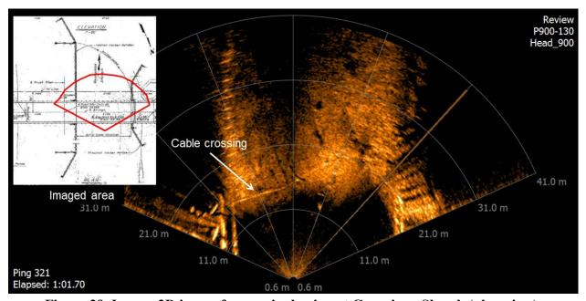
Figure 29. Image. 2D image from a single ping at Georgiana Slough (plan view).
