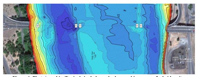
Figure 6. Photo/graphic. Typical single-beam hydrographic survey of a bridge site.
