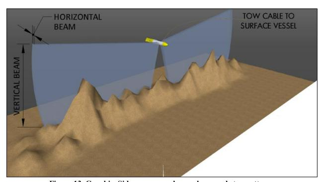
Figure 13. Graphic. Side-scan sonar beam shape and step pattern.
