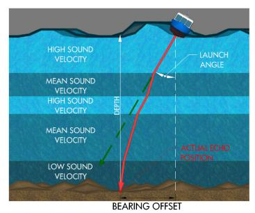
Figure 3. Graphic. Direction of sound waves through varying water layers.
