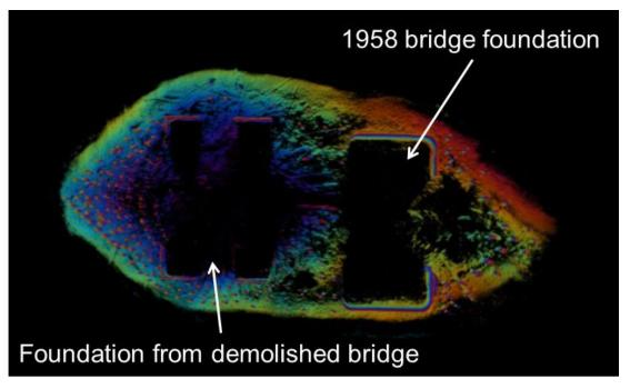
Figure 54. Image. Pier 3 plan view.
