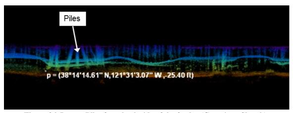
Figure 26. Image. Piles from back side of the fender (Georgiana Slough).
