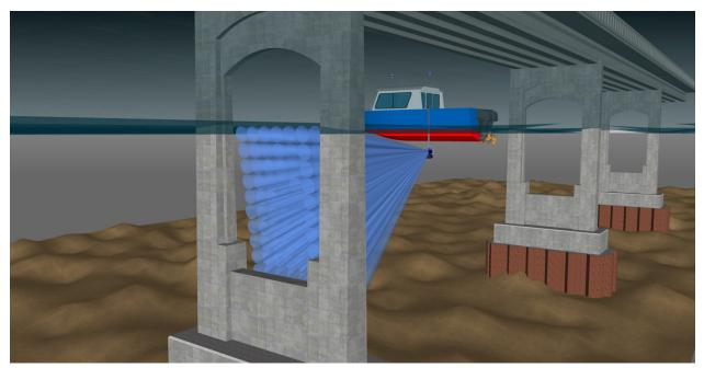
Figure 9. Graphic. Real-time multibeam sonar pattern.
