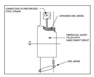
Figure 9-7 Zinc Mesh Pile Jacket
