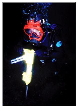
Figure 6-10 Hydraulic Powered Hammer Drill
