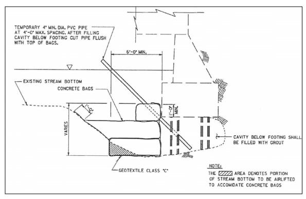
Figure 7-9 Grout Bag Repair at Abutment
