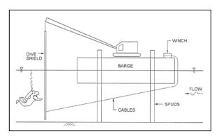
Figure 5-1 Dive Shield Deployed from a Barge
