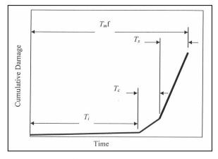
Figure 2-4 Concrete Deterioration Due to Corrosion
