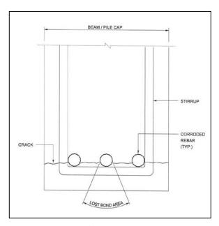
Figure 3-9 Bond Loss from Corrosion
