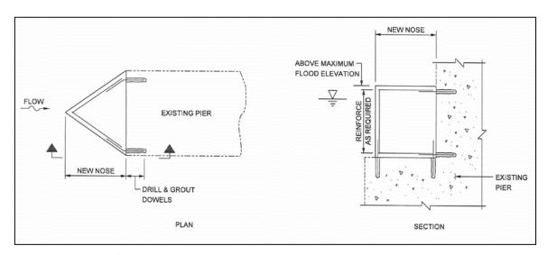
Figure 7-17 Modification to Pier Nose
