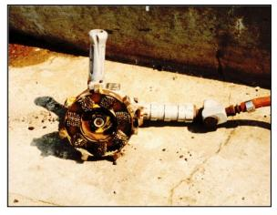
Figure 6-13 Rotary Mechanical Scrubber
