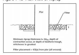
Figure 7-14 Riprap Section
