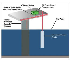
Figure 9-4 Impressed Current System
