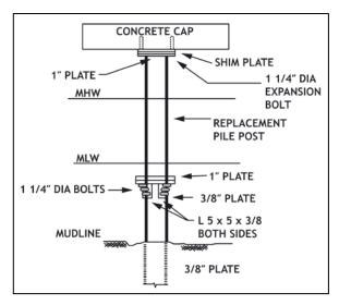
Figure 8-5 Partial Steel Pile Replacement
