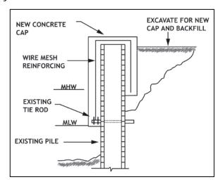
Figure 8-31 Facing Repair Concept
