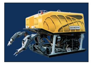
Figure 6-2 Work Class ROV
