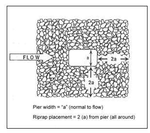
Figure 7-13 Plan View of Riprap
