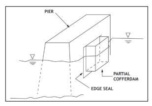
Figure 5-10 Limpet Cofferdam Schematic
