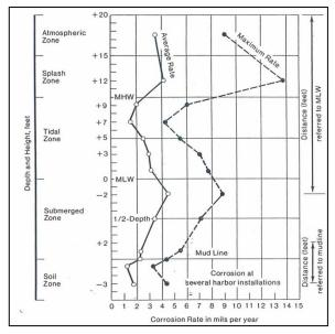
Figure 2-5 Corrosion Rate in mils per year
