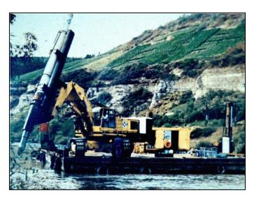
Figure 6-15 Specialized Underwater Hydraulic Hammer
