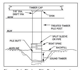
Figure 8-6 Timber Pile Replacement
