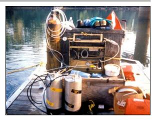
Figure 7-5 Epoxy Injection Equipment on Float
