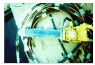
Figure 6-11 Hydraulic Chain Saw
