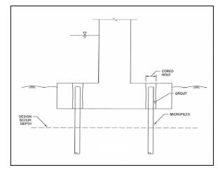
Figure 7-16 Footing Modification Using Micropiles
