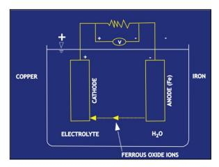
Figure 9-1 Electrochemical Corrosion Cell
