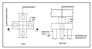
Figure 8-3 Supplemental Pile Bent
