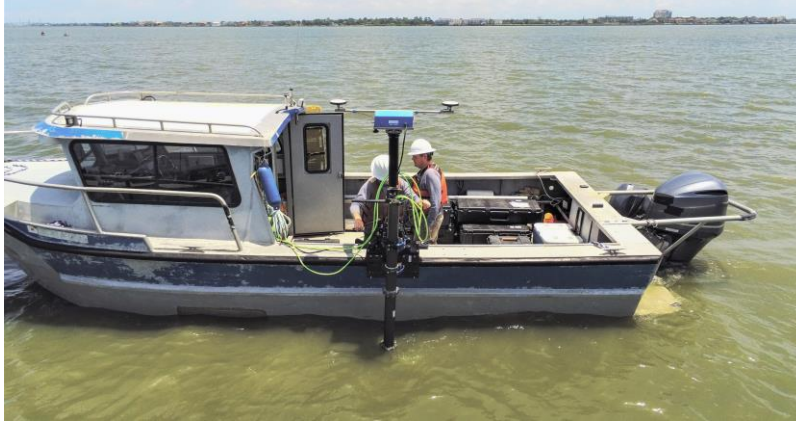
Figure 104. Photo. Inspection vessel outfitted with a 3D scan system. (Source FHWA).
