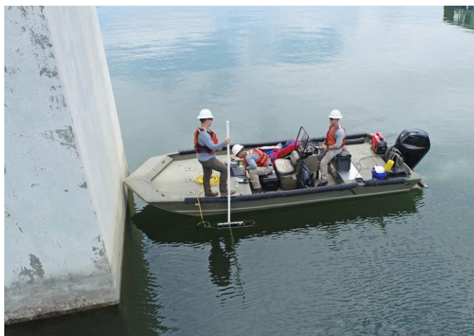
Figure 101. Photo. Inspection team collecting 2D acoustic imaging of a bridge pier as part of underwater bridge inspection. (Source FHWA).
