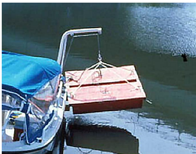
Figure 98. Photo. GPR antenna being lowered to the water surface. (Source FHWA).
