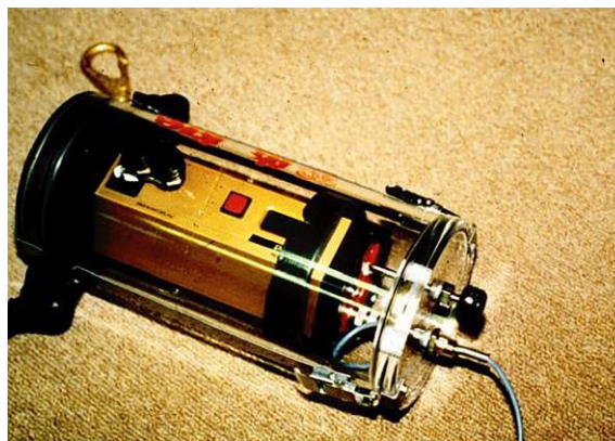
Figure 75. Photo. R-meter installed in an underwater housing. (Source FHWA).
