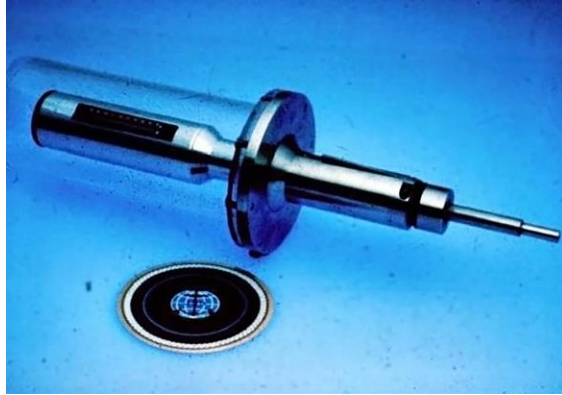
Figure 74. Photo. Rebound hammer in an underwater housing. (Source FHWA).
