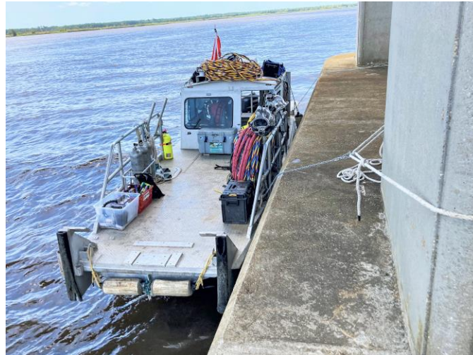
Figure 60. Photo. Dive vessel tied to bridge pier for underwater bridge inspection. (Source FHWA).
