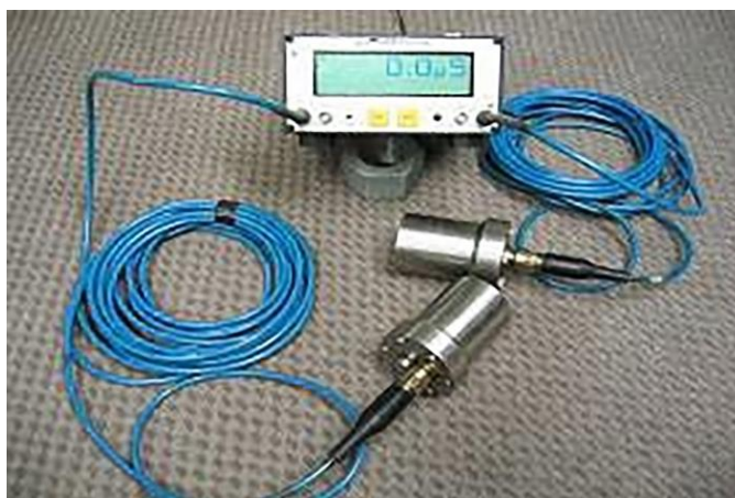
Figure 71. Photo. Ultrasonic pulse velocity meter with waterproof cables and transducers. (Source FHWA).
