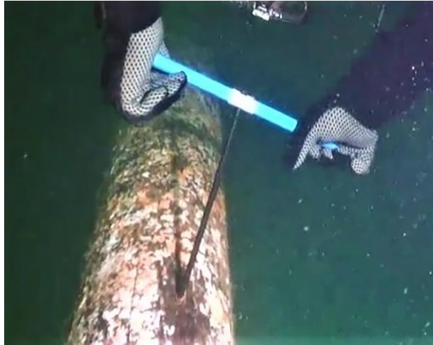
Figure 79. Photo. Diver extracting a core sample from a timber pile. (Source FHWA).
