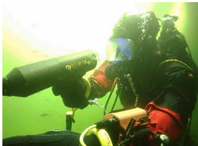
Figure 70. Photo. Diver using an underwater CP gun to measure electrical current on steel pile. (Source FHWA).
