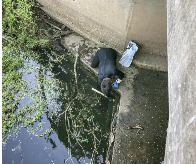
Figure 95. Photo. Diver probing undermined culvert to collect penetration depths. (Source FHWA).
