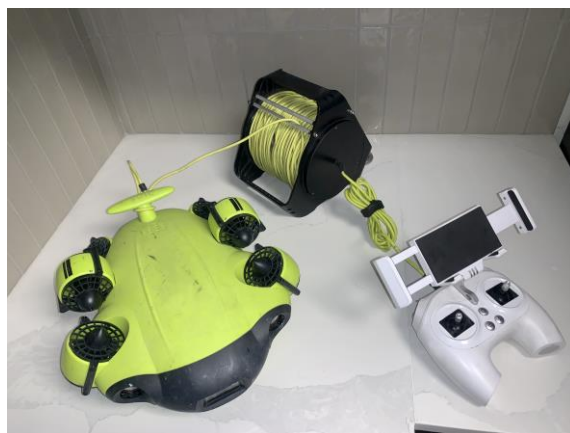
Figure 4. Photo. Example of ROV system used for underwater bridge inspection. (Source FHWA).
