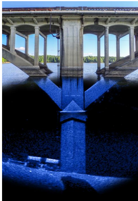
Figure 2. Graphic. Combined acoustic 2D image of a bridge pier. (Source FHWA).
