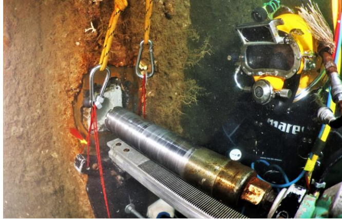
Figure 76. Photo. Diver extracting a concrete core from a bulkhead. (Source FHWA).
