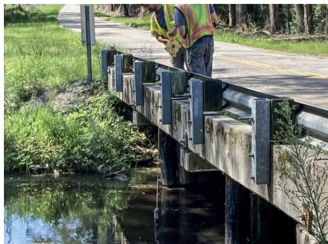
Figure 96. Photo. Inspector collecting soundings with an engineer tape from the bridge deck. (Source FHWA).
