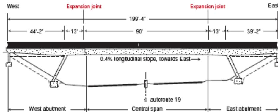
**Figure 3-4** Sketch showing the elevation of de la Concorde overpass; the simple central span of the bridge consisted of adjacent box girders, which rested on a beam seat that was built into the thickened slab that cantilevered from the abutments at each end (taken from [52]).
