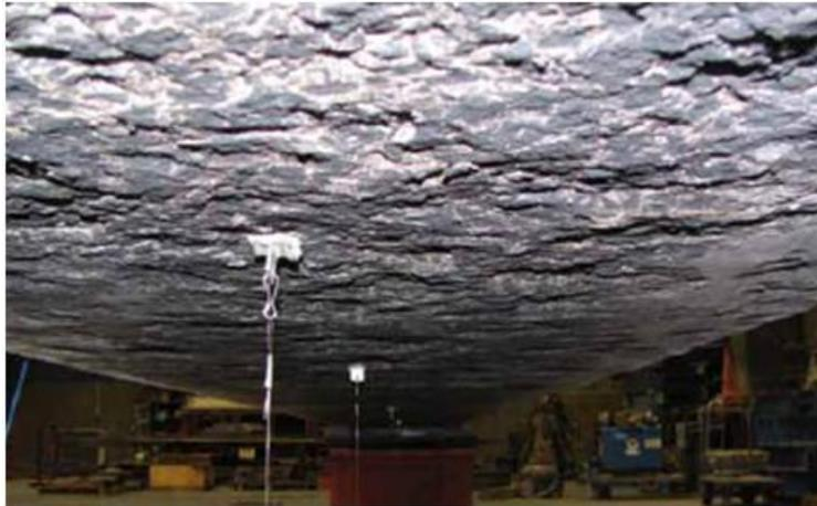
**Figure 3-5** *Photo of the bottom face of a tested beam subjected to fire while in service showing that the concrete has deteriorated such that sufficient pathways through the concrete to the bottom layer of prestressing strands have developed (taken from [56]).*
