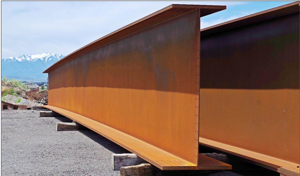
**Figure 49: Photo. Fabricated steel plate girders for the I-80 bridges.**
