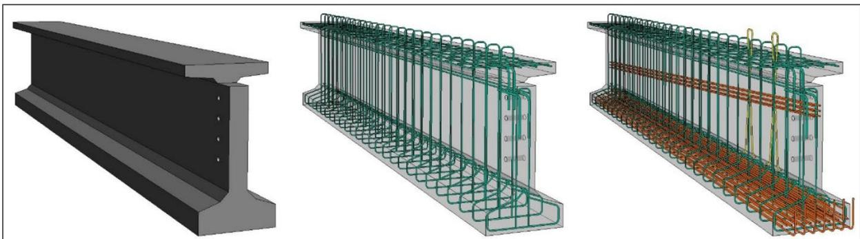
**Figure 23: Illustration. Three levels of development for a prestressed beam.**
