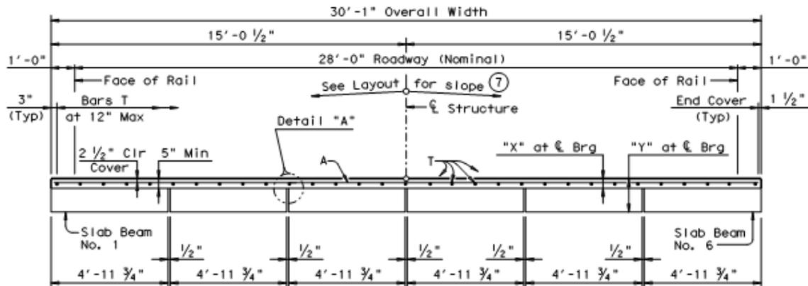
Figure 5.4.2-1 Precast Solid Slab Beam (Plank) Bridge
