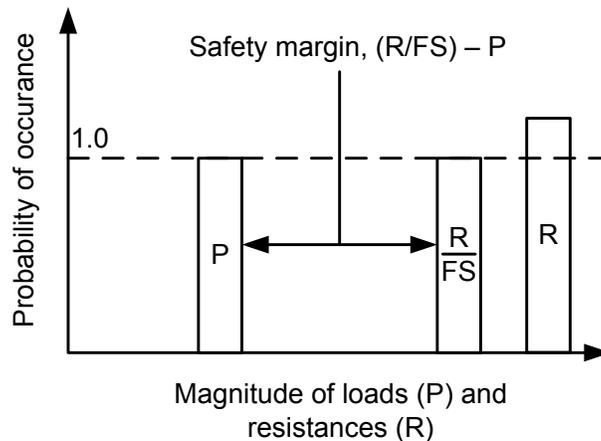
**Figure 1.2.2.2-1 Graphical Representation of Allowable Stress Design**
