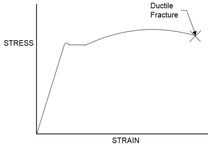
**Figure 6.5.5.3.1-1 Typical Stress-Strain Curve for Mild Steel**
