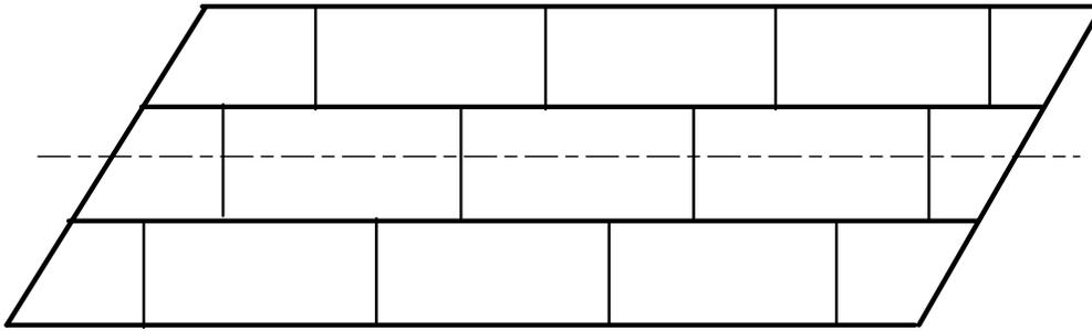
**Figure 6.3.2.9.4.3.2-2 Discontinuous (Staggered) Cross-Frame/Diaphragm Lines Along the Entire Span Normal to Girder Tangents (for Skew > 20°)**
