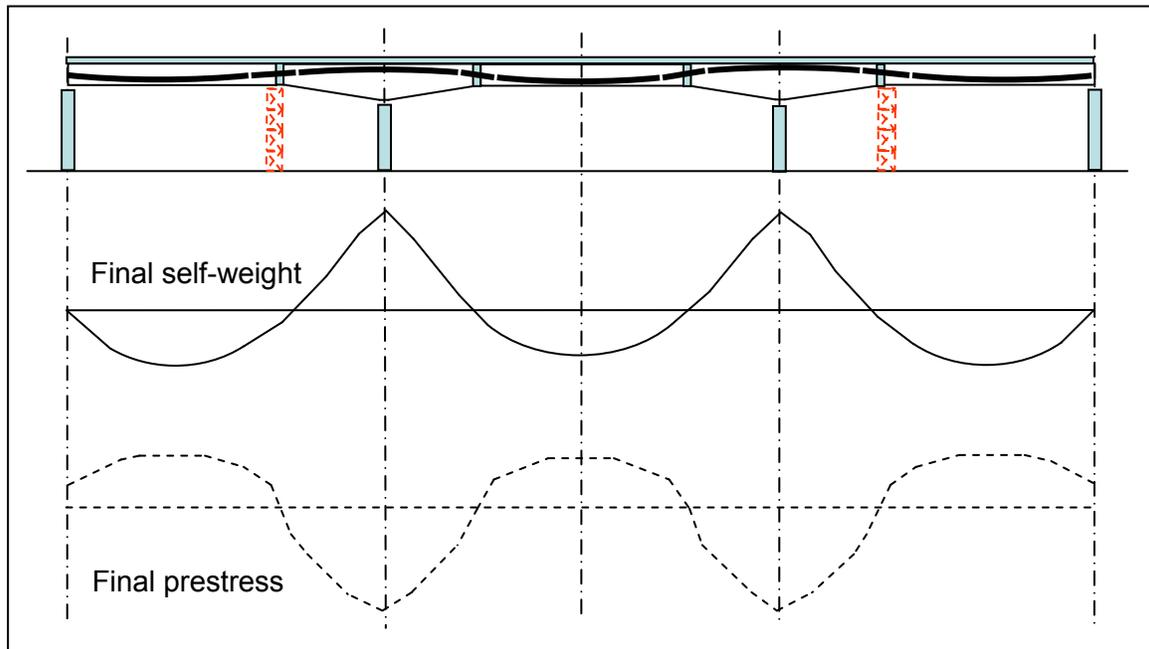
**Figure 5.10.4.2-6 Spliced Girder Construction - Final Moments**
