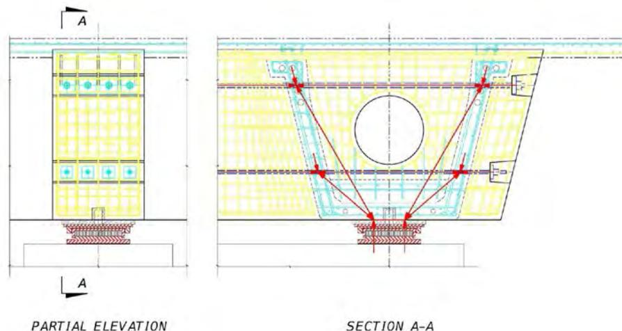
**Figure 5.6.1.3-1 Pier Segment Diaphragm in a Post-Tensioned Segmental Box Girder Bridge**
