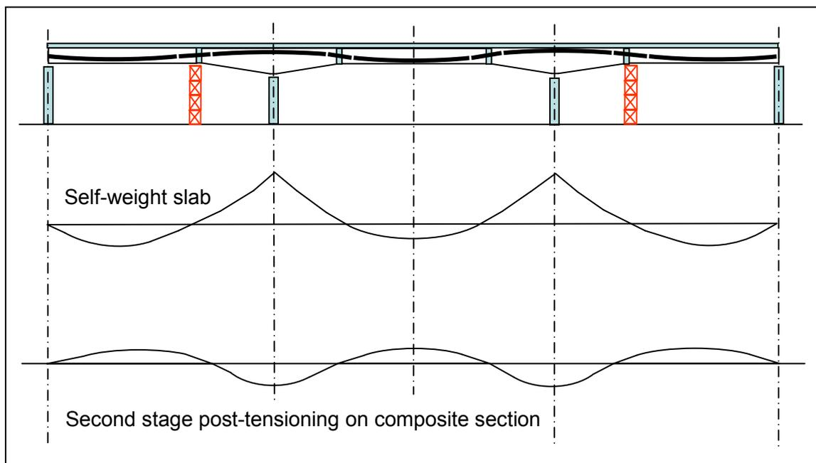
**Figure 5.10.4.2-5 Spliced Girder Construction - Slab and Stage 2 PT Moments**
