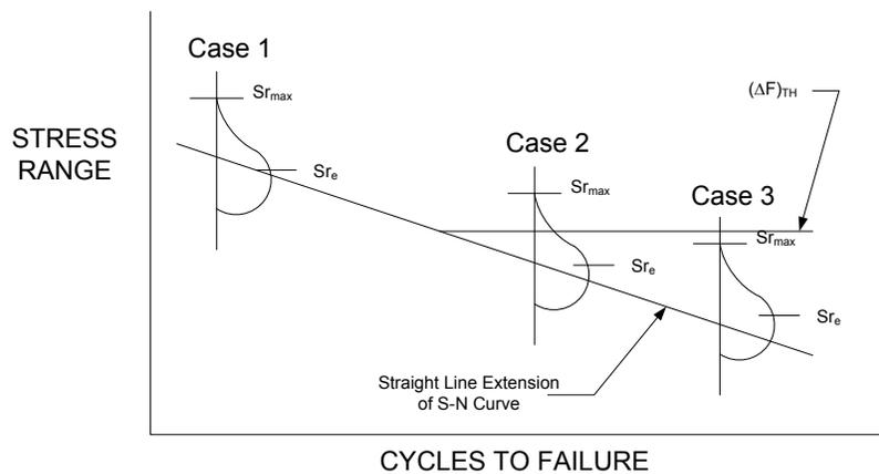
**Figure 6.5.5.2.2.1.4-1 Three Possible Cases of Variable-Amplitude Loading**
