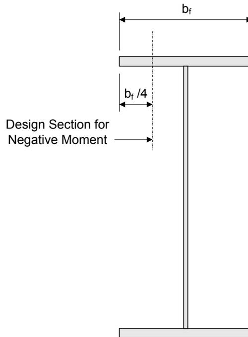
**Figure 7.3.2.4-3 Design Section for Negative Moment**
