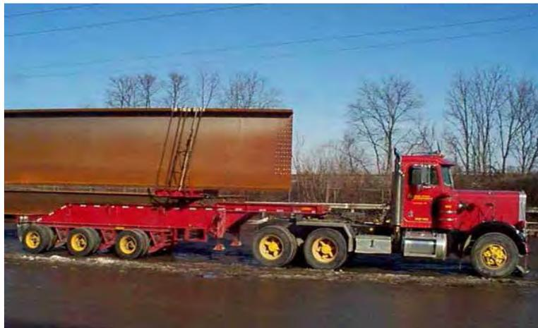
**Figure 6.3.2.4.1-1 Girder Field Section in Route to the Construction Site**
