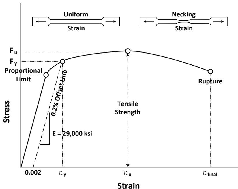
**Figure 6.2.7.1-1 Engineering Tensile Stress vs. Strain Curve for Structural Steels Without a Defined Yield Plateau (Wright, 2012)**
