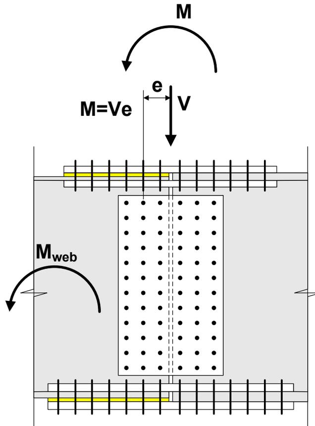
**Figure 6.6.5.2.3.1-1 Design Actions for Bolted Web Splices for Flexural Members**
