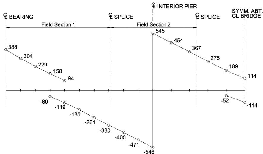
Figure 6.5.7.4.2.2-1 Example Problem Shears due to the Factored Loads – Strength I
