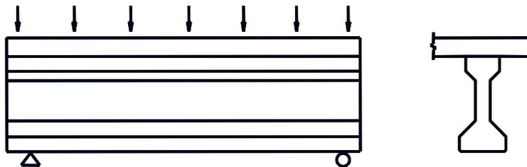
**Figure 5.6.4.2-2 Deck Placed on Noncomposite Beam**
