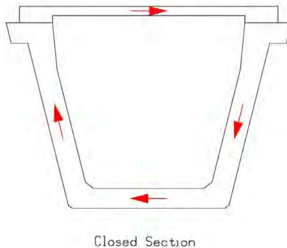
**Figure 5.6.3-2 Closed Section Torsion Flow**
