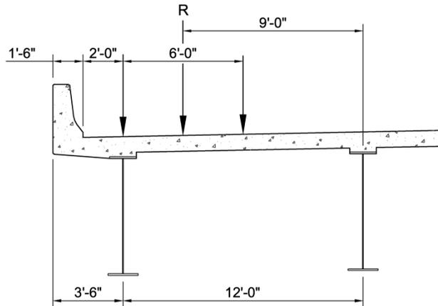
**Figure 4.4.2.2.2-2 Exterior Girder LLDF – Lever Rule**
