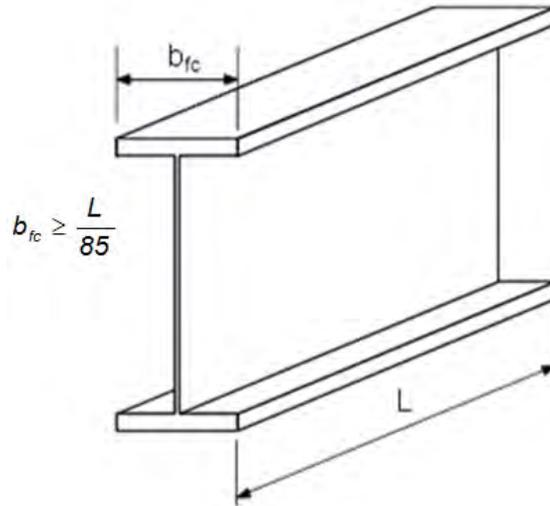
**Figure 6.3.4.4.2-1 Field Section L/b Ratio**
