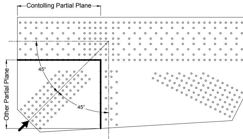
**Figure 6.6.7.2-1 Example of a Controlling Partial Shear Plane that Parallels the Chamfered End of the Compression Member Since that Member Frames in at an Angle of 45 Degrees to Both the Chord and the Vertical**
