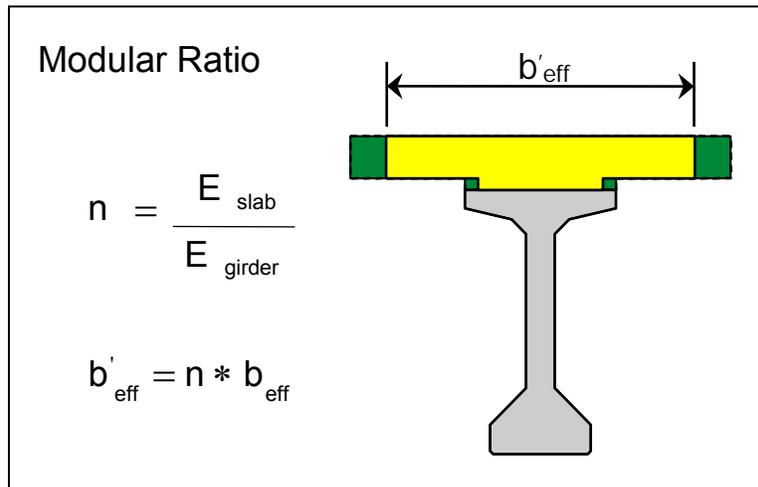
Figure 5.5.3.2.2-3 Modular Ratio (n) of Slab to Girder Concrete
