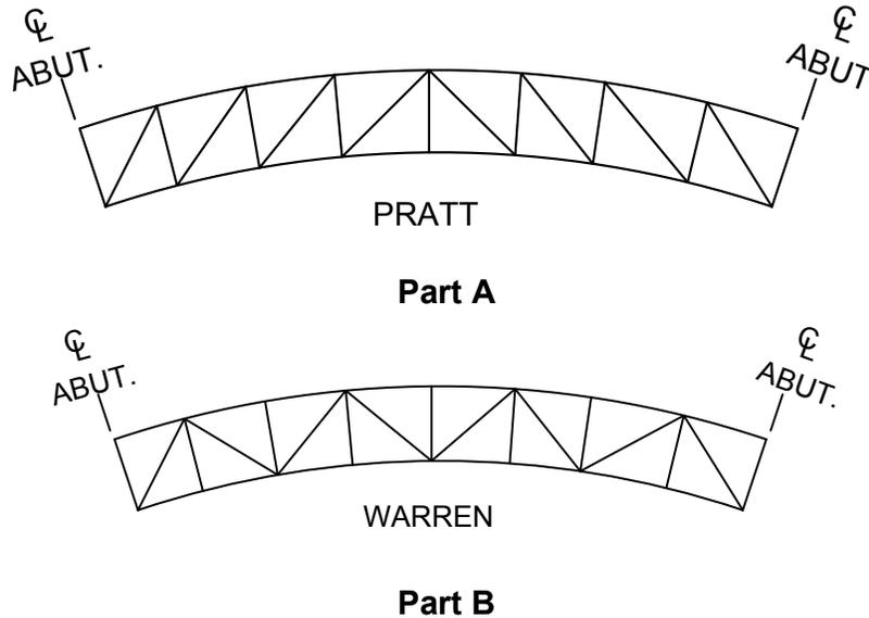
**Figure 6.3.2.10.3-1 Full-Length Single-Diagonal Lateral Bracing Patterns**
