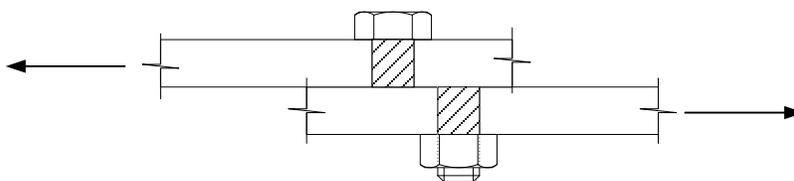
**Figure 6.6.4.2.5.2-1 Shear Failure of a Bolt**
