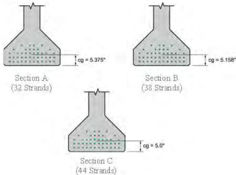
**Figure 5.10.3.3.2.1-5 Prestressing Layout and Debonding**
