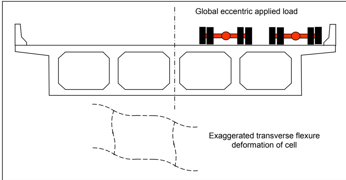
**Figure 5.10.6.1.2-2 Transverse Deformation of Cells from Eccentric Load**
