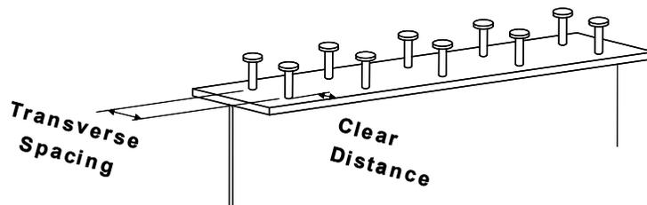
Figure 6.6.2.2.3.1-1 Transverse Spacing and Clear Distance
