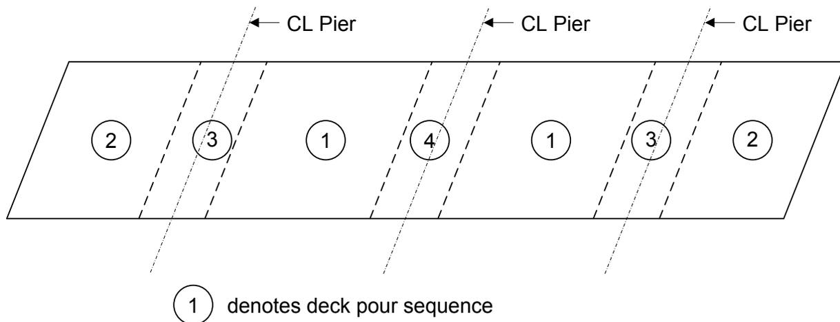
**Figure 7.3.7.2-1 Sample Deck Placement Sequence Plan**
