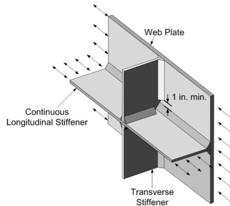
**Figure 6.5.5.2.2.1.3-1 Weld Detail at a Continuous Attachment Parallel to the Applied Stress with a Discontinuous Transverse Attachment**
