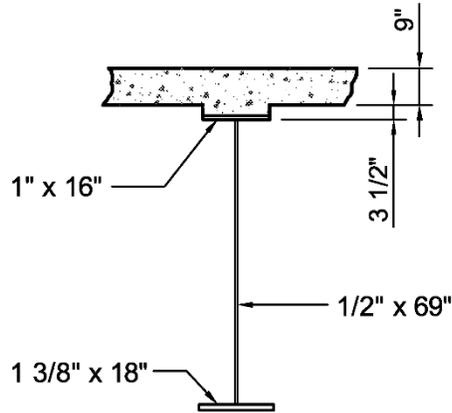
**Figure 6.4.2.3.2.3-1 Example Composite Cross-Section – Exterior Girder – Positive Flexure Region**
