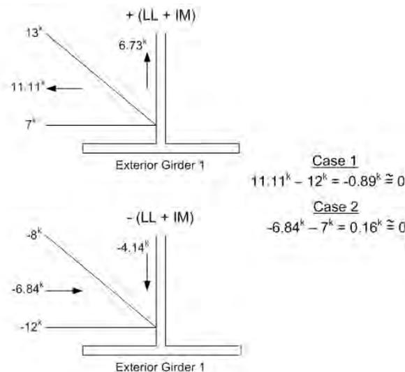
**Figure 6.6.4.4-3 Equilibrium Check for ( $+LL+IM$ ) and ( $-LL+IM$ ) Cross-Frame Horizontal Forces at the Bottom of an Exterior Girder**
