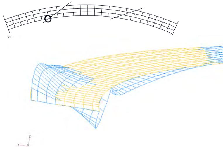
**Figure 4.4.3.2.1-2 Influence Surface for Vertical Bending Moment at Pier 1 of G1 in the Example I-Girder Bridge**
