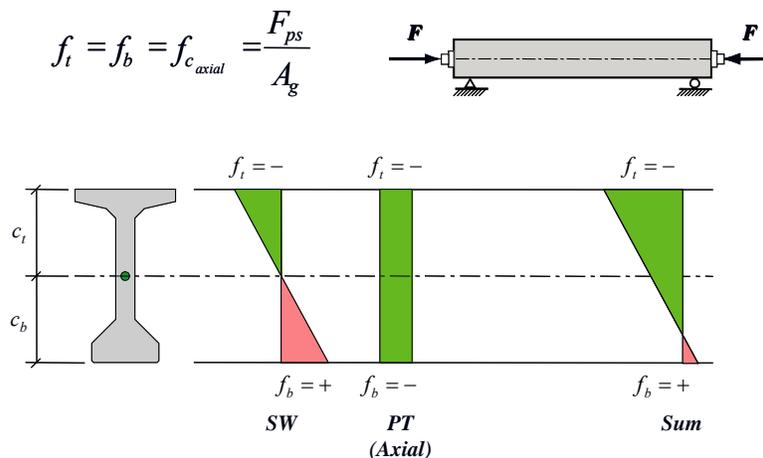
**Figure 5.3.3-2 Self Weight Plus Axial Compression**
