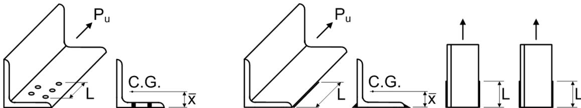
**Figure 6.6.3.3.2.4-1 Determination of  $\bar{x}$  and  $L$  in the Calculation of the Shear Lag Reduction Factor,  $U$ , from Equation 6.6.3.3.2.4-1**
