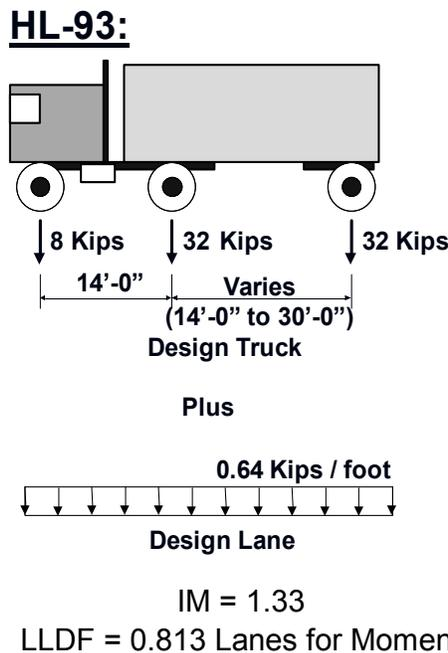
**Figure 4.4.3.1-5 HL-93 Live Load plus IM and Multi-Lane Moment LLDF for the Example Two-Span Bridge**
