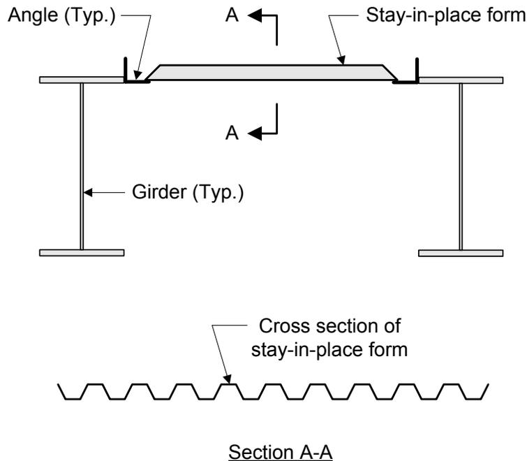
**Figure 7.3.5.2.1-1 Steel Stay-in-place Formwork**
