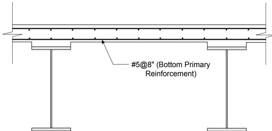
**Figure 7.3.2.4-5 Primary Reinforcement in Bottom of Deck**
