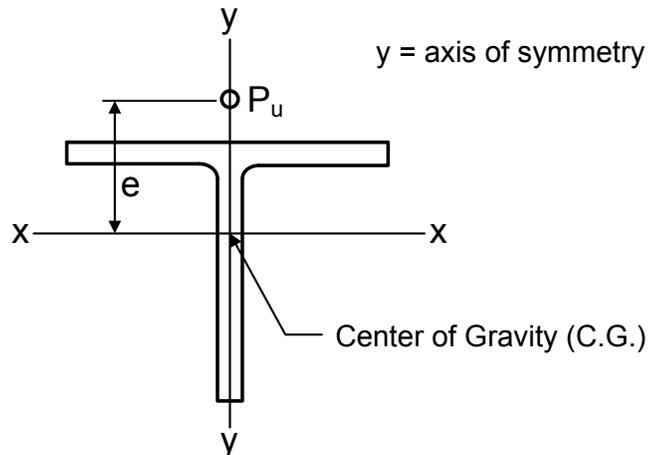
**Figure 6.6.3.5.3-2 Tee Member Geometry and Eccentricity of Applied Load,  $P_u$**
