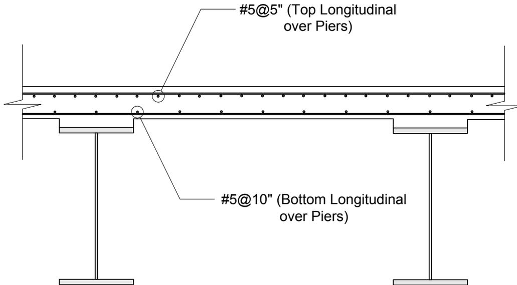
**Figure 7.3.2.6-1 Longitudinal Reinforcement over Piers**
