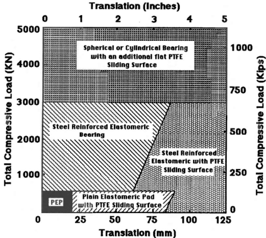
Figure 8.2.3.6-3 Preliminary Bearing Selection Diagram for Large Design Rotation (Rotation > 0.015 Radians)
