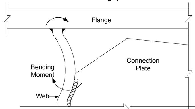
**Figure 6.5.5.2.3-1 Web Gap Distortion**
