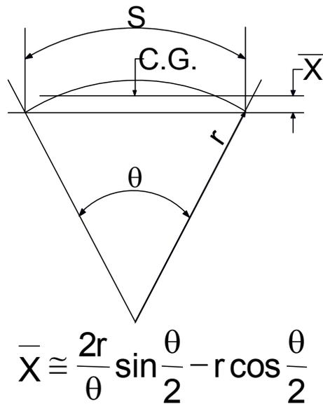
**Figure 6.3.2.4.3.2-1 Locating Pick Points on a Curved I-Girder**
