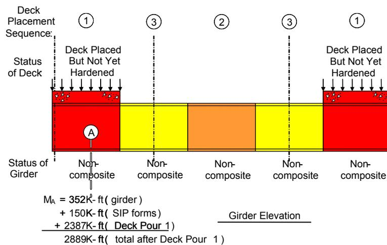
**Figure 6.5.3.3.4-4 Sample Deck Placement Analysis (Cast 1)**
