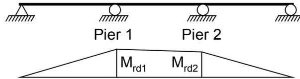
**Figure 6.5.6.6.3.2-1 Typical Redistribution Moment Diagram for a Three-Span Continuous Bridge**
