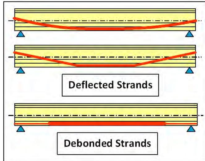
Figure 5.7.4.1.2-1 Typical Prestressing Steel Layouts
