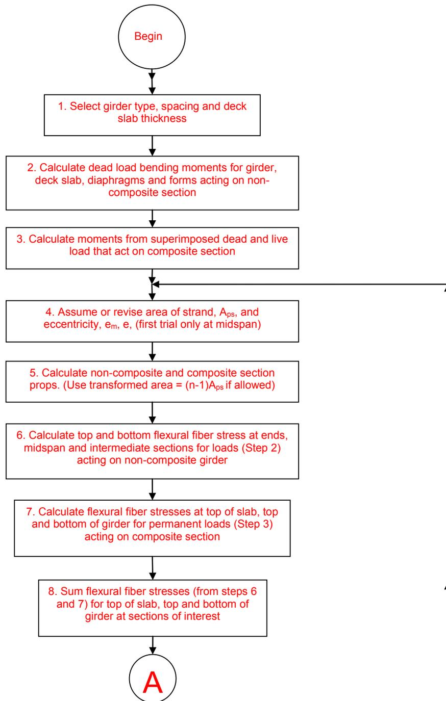
**Figure 5.5.3.4.3-3 Flowchart for Determination of Prestress Force and Strand Pattern, Part (a)**
