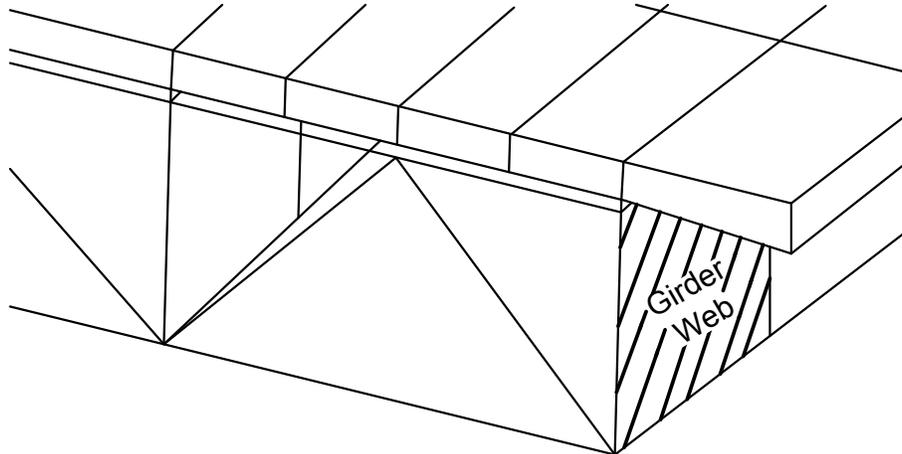
**Figure 4.5.3.3.2.3.2-2 Shell Element Used to Model a Girder Web**
