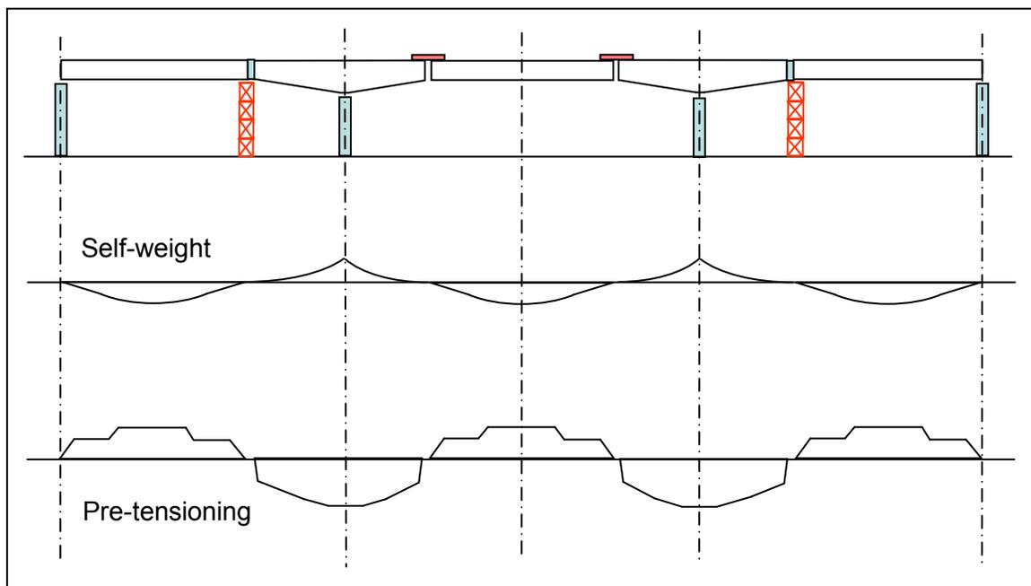
**Figure 5.10.4.2-3 pliced Girder Construction - Self Weight and Pretensioning Moments**
