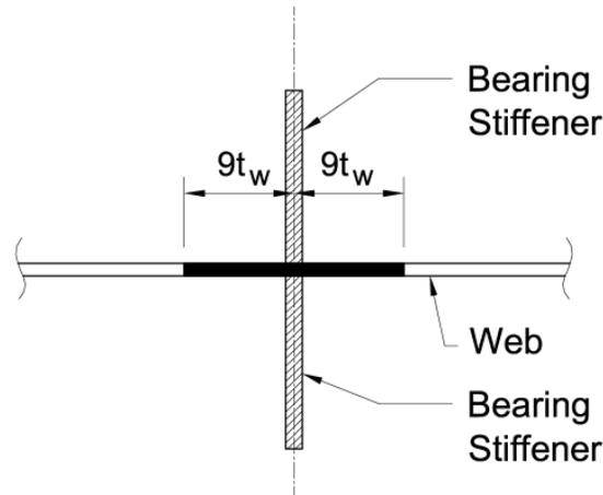
**Figure 6.6.6.3.4.2-1 Effective Column Section for Welded Bearing Stiffener Design (One Pair of Stiffeners Welded to a Web)**
