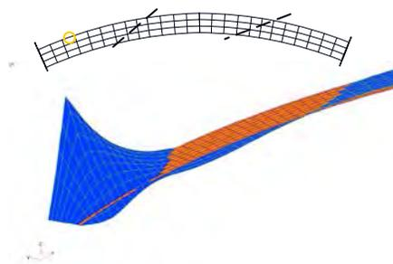
**Figure 4.4.3.2.2-4 Influence Surface for Vertical Bending Moment at Node 24 in Span 1 of G4 of the Example I-Girder Bridge**
