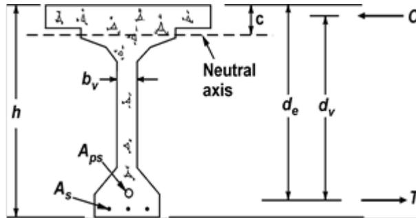
**Figure 5.6.1-1 Terms Used in Sectional Analysis**
