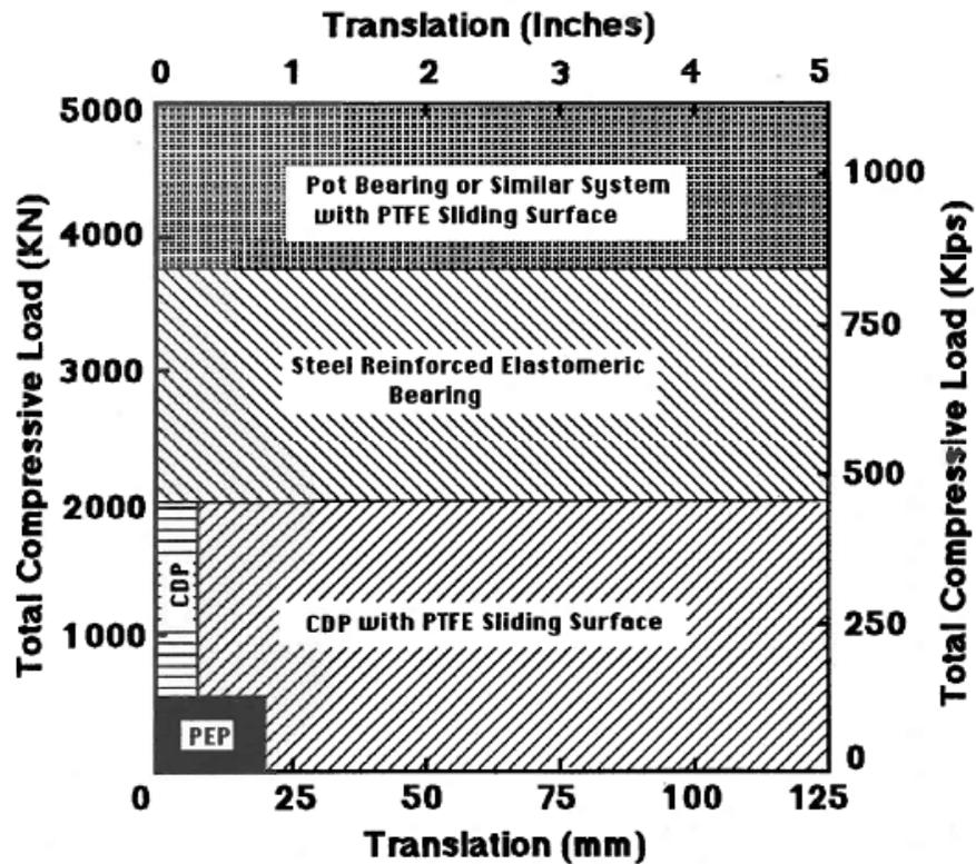
Figure 8.2.3.6-1 Preliminary Bearing Selection Diagram for Minimal Design Rotation (Rotation  $\leq 0.005$  Radians)
