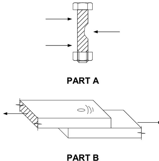
**Figure 6.6.4.2.5.3-1 Bearing Failure of Bolt (Part A) and Connected Material (Part B)**
