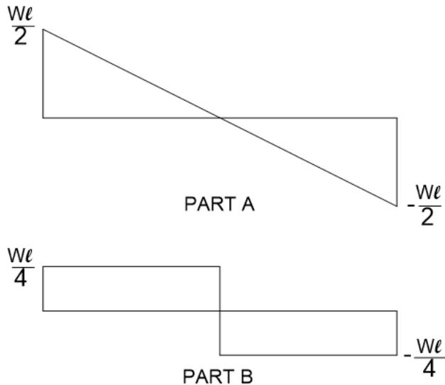
**Figure 4.3.2-2 Shear Diagram for Deck Weight**
