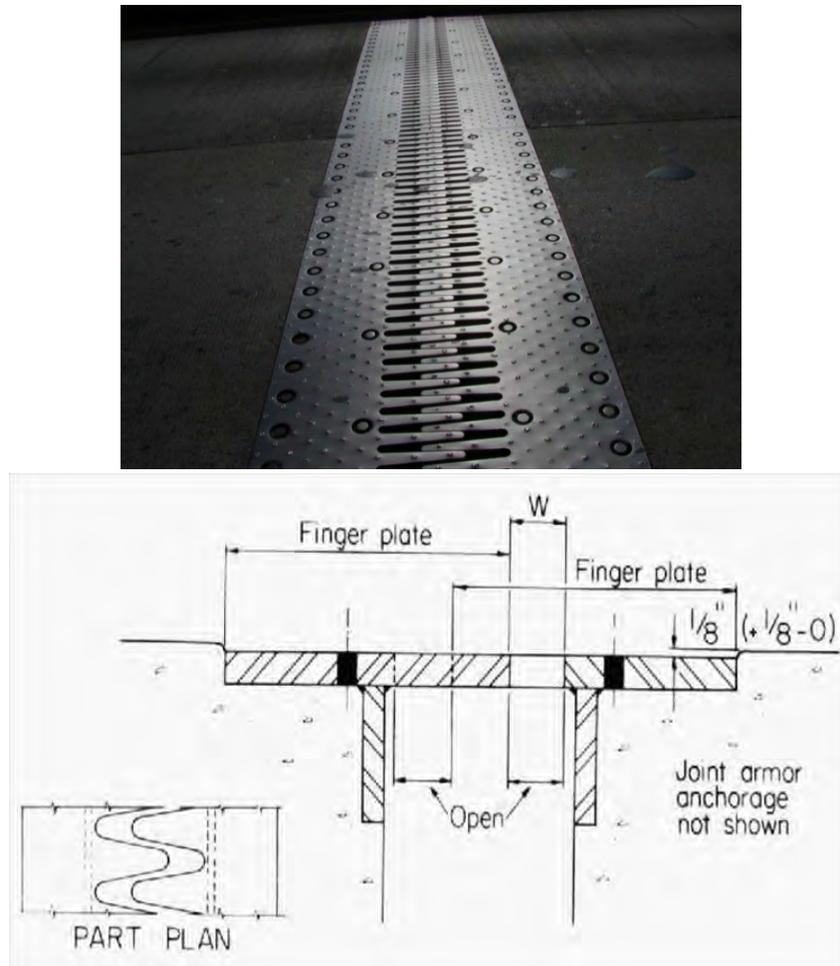
**Figure 8.3.2.4-1 Finger Plate Joint**
