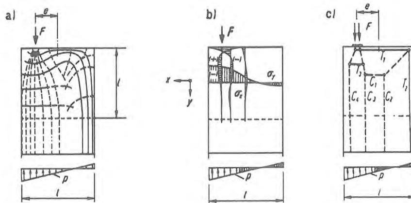
**Figure 5.7.4.3.1-1 Development of Strut-and-Tie Model for Pretensioning**
