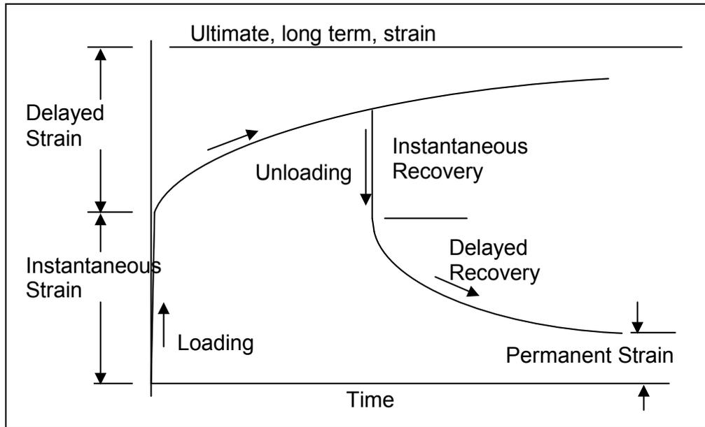
**Figure 5.2.1.2.3.2-1 Creep and Concrete's Response to Sustained Stress**
