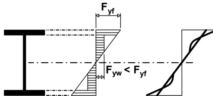
**Figure 6.4.5.7-1 Load Shedding from the Web to the Flanges Due to Early Web Yielding in a Hybrid Section**
