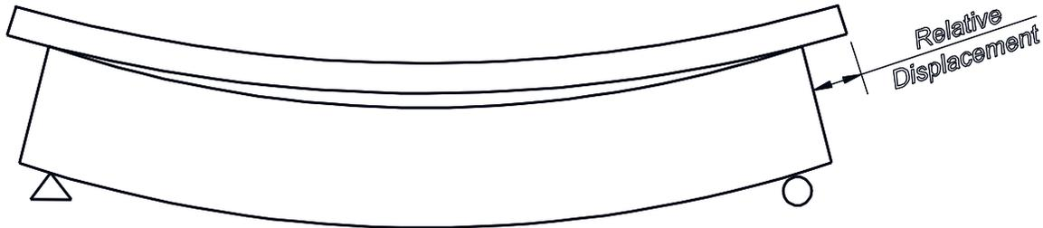
**Figure 5.6.4.2-3 Independent (Noncomposite) Behavior between Precast Girder and Deck**
