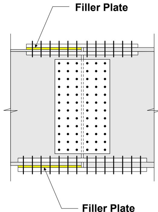
Figure 6.6.5.5.1-1 Filler Plates in Bolted Flange Splices
