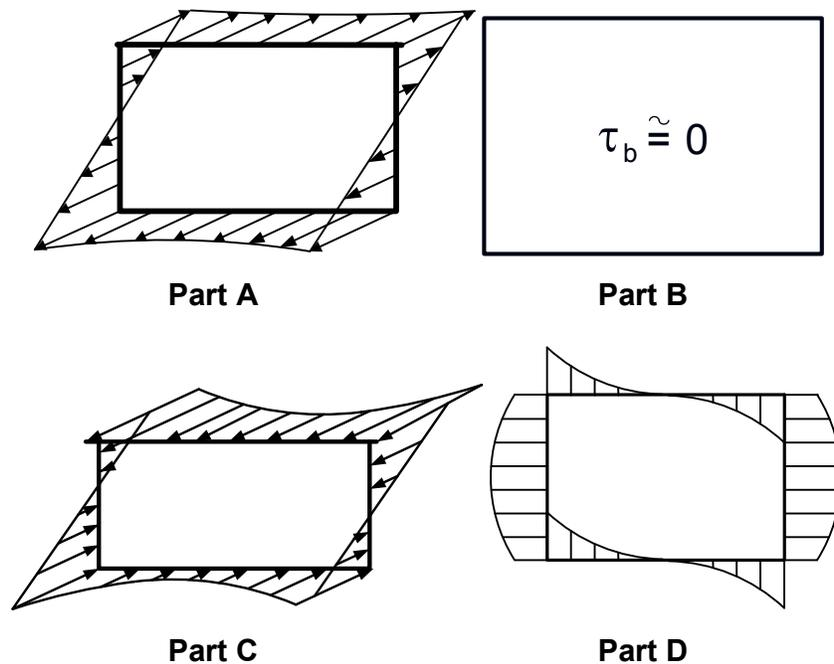
**Figure 6.4.8.3.1-3 Normal and Shear Stress Distributions – Box Section**
