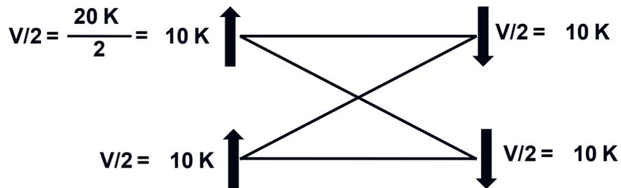
**Figure 4.5.3.2.2.5.3-10 Assumed Distribution of Shears in the Example Cross-Frame**
