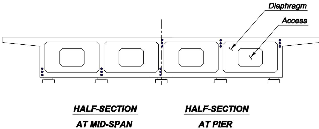
Figure 5.4.2-6 Four-Cell CIP Box Girder Bridge
