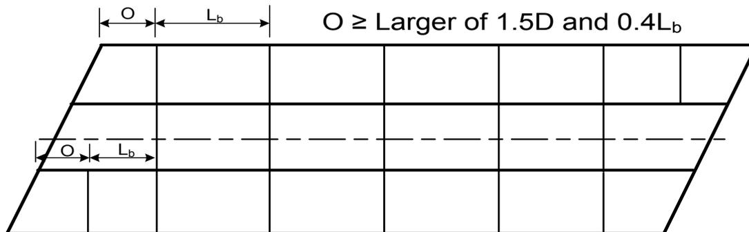
**Figure 6.3.2.9.4.3.2-1 Contiguous Cross-Frame/Diaphragm Lines (Within the Span) Normal to the Girder Tangents (for Skew > 20°)**
