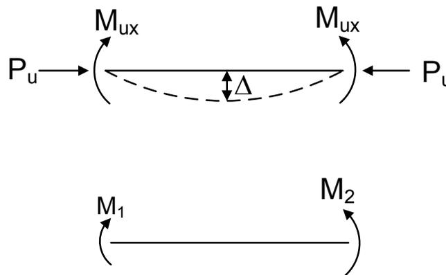
**Figure 6.6.3.4.3.2-1 Magnification of  $M_{ux}$ , and End Moments  $M_1$  and  $M_2$**
