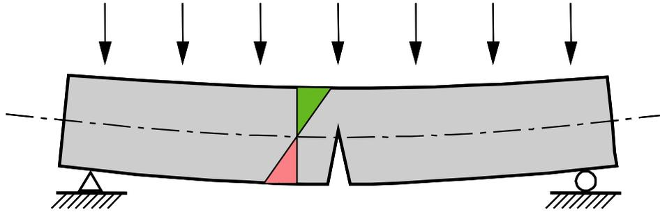
**Figure 5.3.1-1 Plain, Unreinforced Concrete Beam in Flexure**
