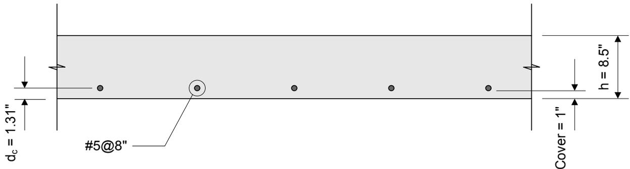
**Figure 7.3.2.4-4 Crack Control by Distribution of Reinforcement**
