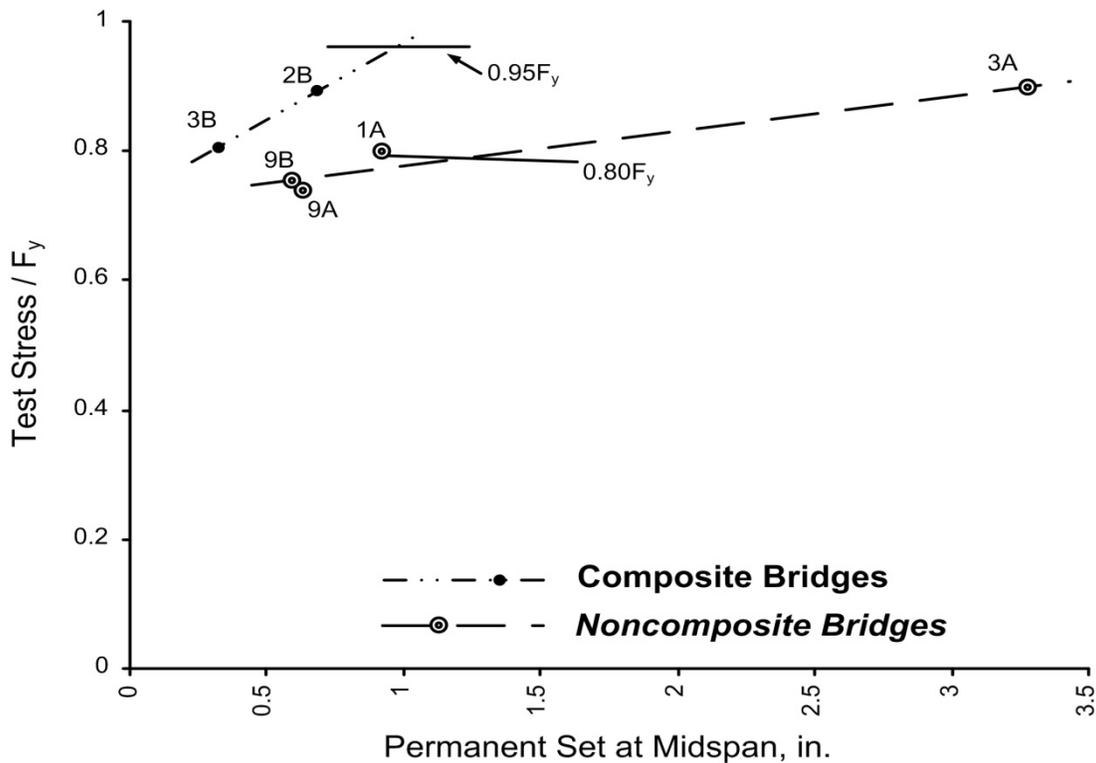
**Figure 6.5.4.3.2.1-1 Measured Permanent Set of AASHTO Road Test Bridges**
