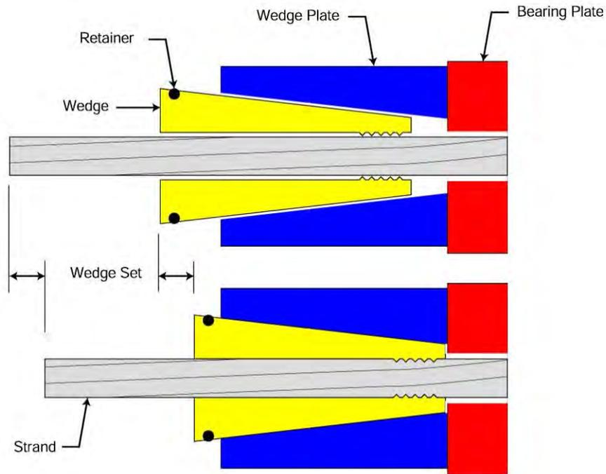
**Figure 5.7.3.3.1.3-2 Gripping of Strands by Wedges**
