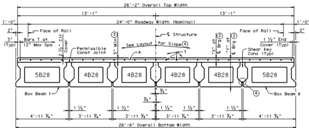
Figure 5.4.2-2 Adjacent Precast Box Beam Bridge
