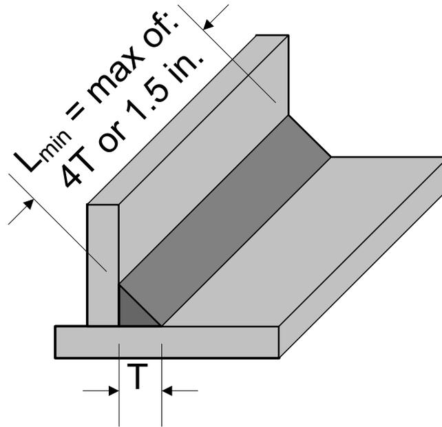
**Figure 6.6.4.3.3.2-2 Minimum Effective Length of Fillet Welds**
