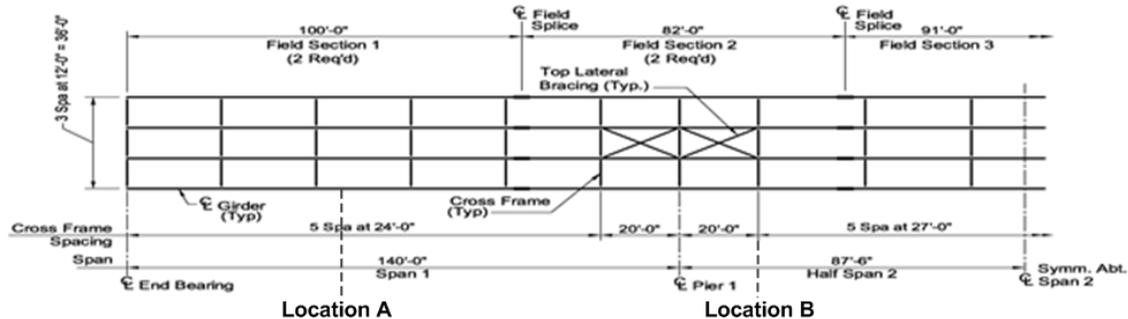
**Figure 6.5.3.6-1 Fully Erected Non-Composite Framing Plan for Wind Load Example**
