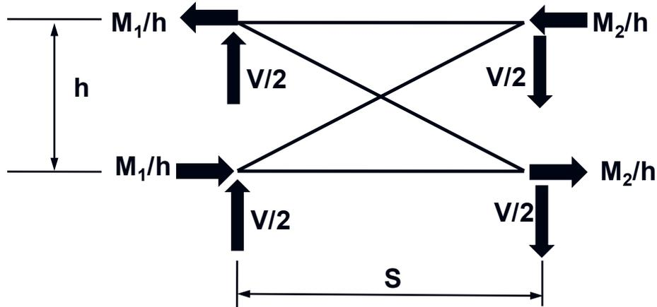
**Figure 4.5.3.2.2.5.3-8 Resolution of the End Moments into Force Couples (X-Type Cross-Frame)**
