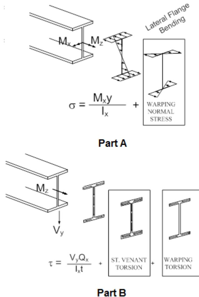
**Figure 6.4.8.2.3-3 I-Section Bending Stresses and Shears for Design**
