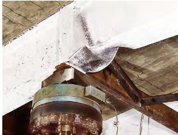
**Figure 6.5.6.2.2.2.1-1 Local Buckling of Compression Flange of a Laboratory Specimen**
