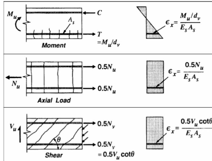
**Figure 5.6.1.1.8-1 Longitudinal Strain Caused by Applied Loads and Prestressing**
