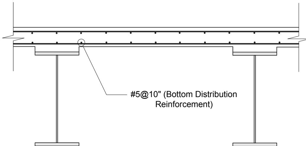
**Figure 7.3.2.5-1 Distribution Reinforcement in Bottom of Deck**
