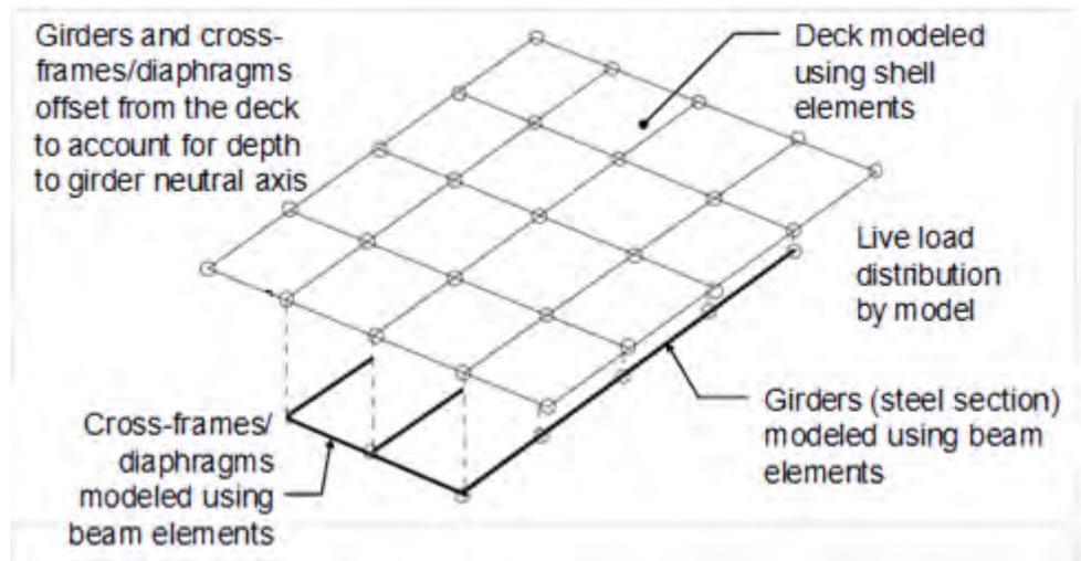
**Figure 4.5.3.2.2.3-1 Plate and Eccentric Beam Model**
