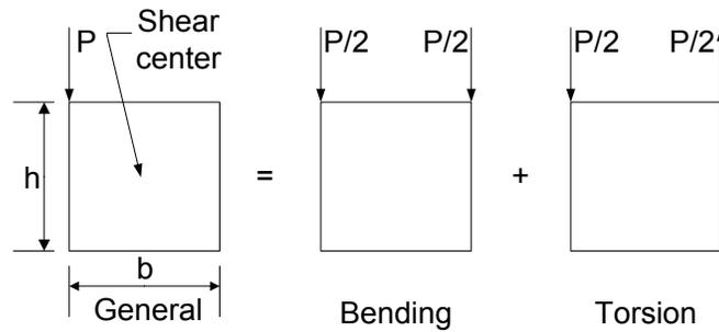
**Figure 6.4.8.3.1-2 Vertical Bending and Torsion Components – Box Section**
