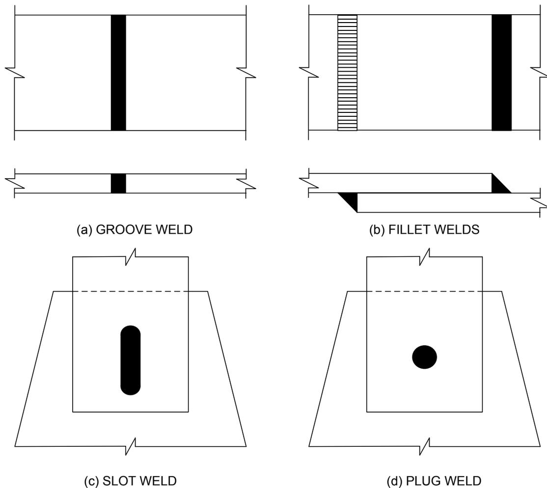
**Figure 6.6.4.3.3.1-1 Types of Welds**
