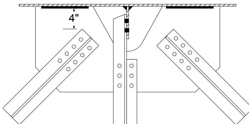
**Figure 6.3.2.10.4-4 Alternative Recommended Lateral Connection Plate Detail for Plate Attached to the Girder Web – Plate on Same Side of Web as Transverse Stiffener**
