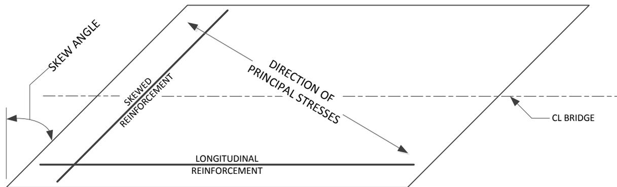
Figure 7.3.1.3-1 Reinforcement Layout for a Highly Skewed Deck
