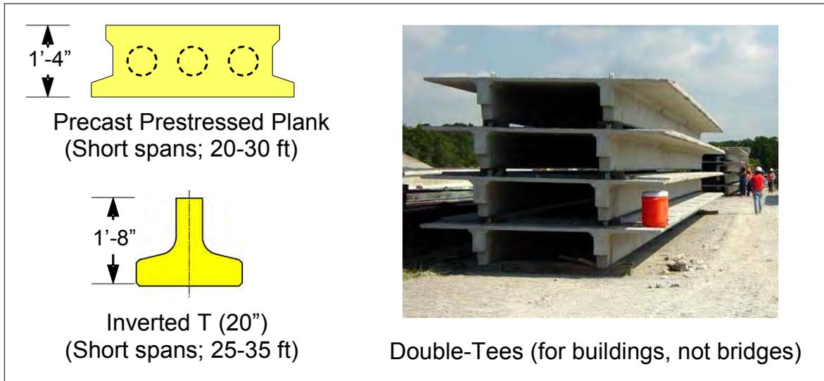
**Figure 5.10.2-1 Other Miscellaneous Precast Concrete Sections**
