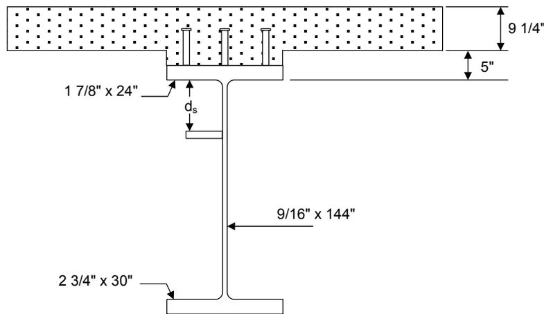
**Figure 6.4.5.5.2.2-2 Longitudinally Stiffened Girder Section – Positive Flexure Region**
