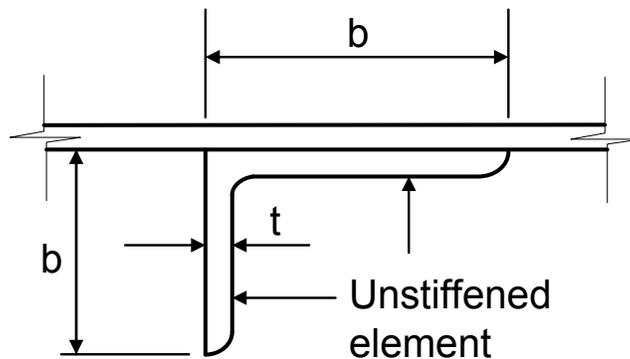
**Figure 6.6.3.4.2.4.3-1 Unstiffened Elements for a Single-Angle Member**
