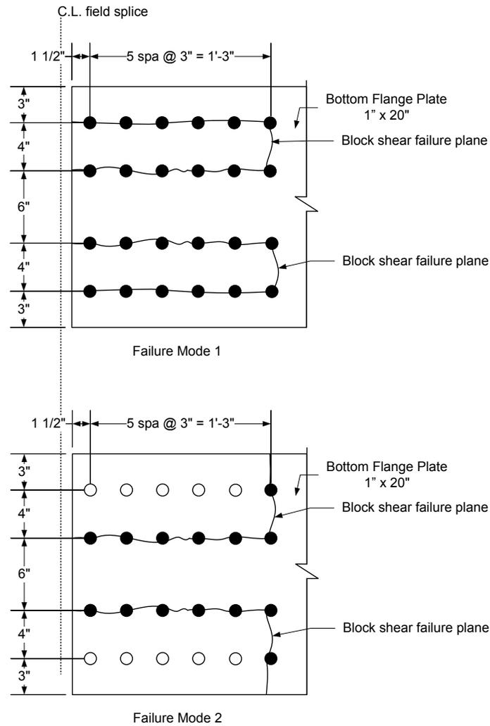
**Figure 6.6.5.2.3.4-4 Bottom Flange Splice – Assumed Block Shear Failure Planes in the Flange on the Right-Hand Side of the Splice**
