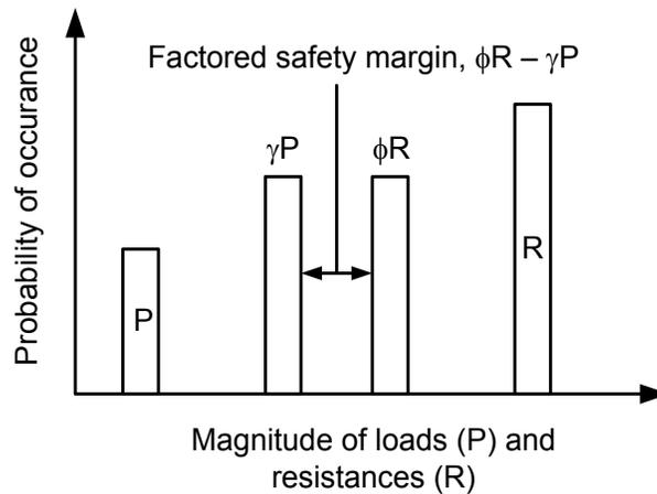
**Figure 1.2.2.4-1 Graphical Representation of Load and Resistance Factor Design**
