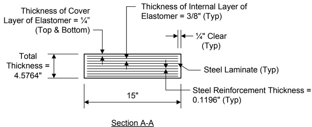
**Figure 8.2.4.1.2.9-1 Final Configuration of Elastomeric Bearing Design Example**
