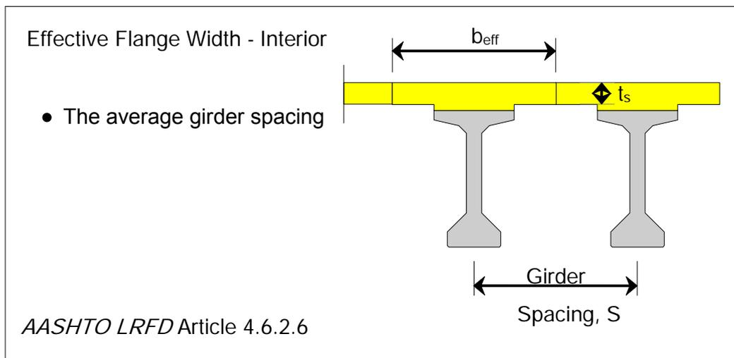
**Figure 5.5.3.2.2-1 Effective Flange Width of Interior Girder**
