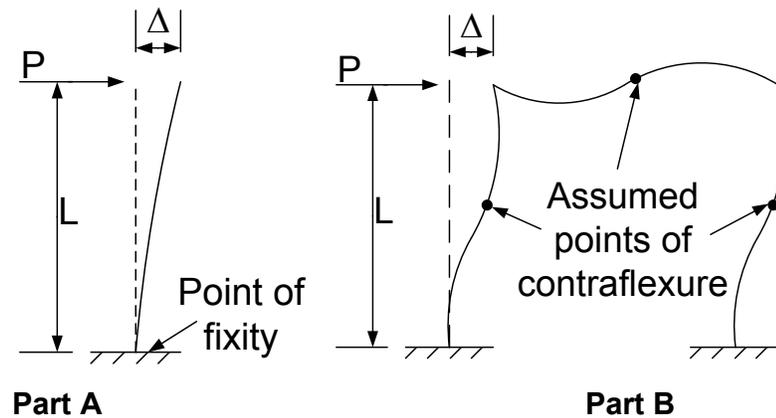
**Figure 6.3.3.3.7-1 Schematic Representations of a Typical Pier in the Longitudinal and Transverse Directions**
