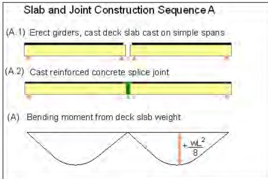
**Figure 5.10.3.2.3.3-1 Construction Sequence Effects – Case (A)**
