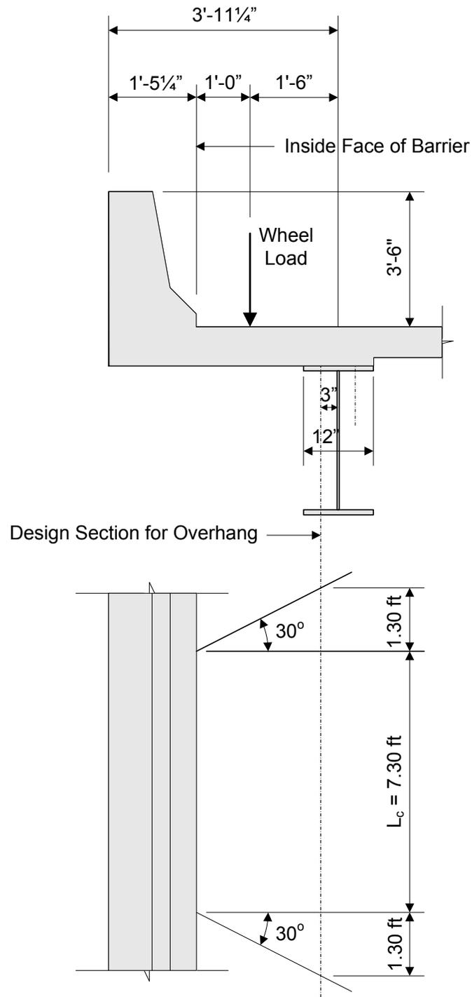
**Figure 7.3.4.2.1-4 Assumed Distribution of Collision Moment Load in the Overhang**
