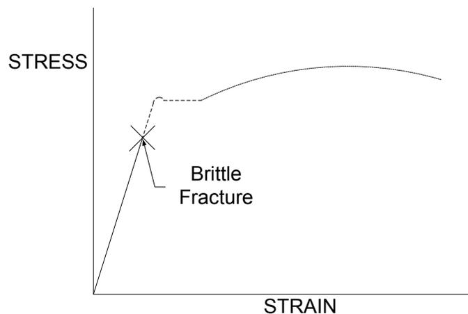
**Figure 6.5.5.3.1-2 Stress-Strain Curve Indicative of a Brittle Fracture**
