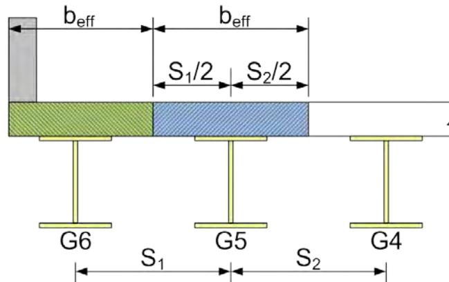
**Figure 4.2.2.1-2 Effective Deck Width Based on Tributary Width of Deck over Each Girder**
