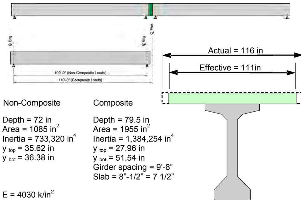
**Figure 5.10.3.3.2.1-1 Two-Span Structure of Type VI Girders**
