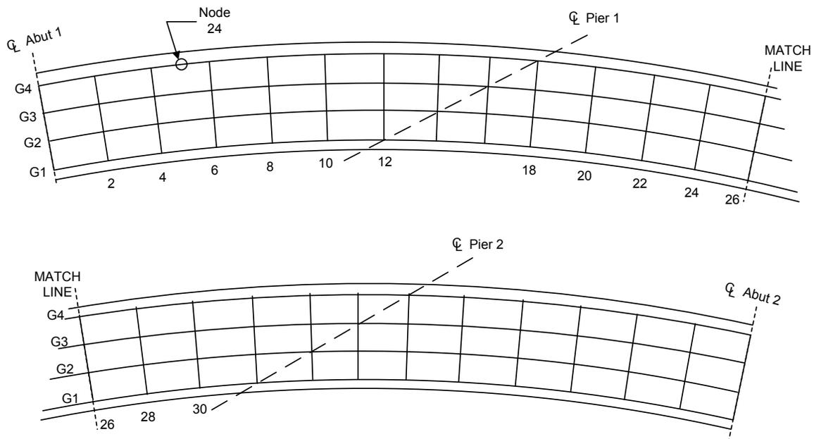
**Figure 4.4.3.2.2-3 Plan View of the Example I-Girder Bridge with a Contiguous Cross-Frame Arrangement**
