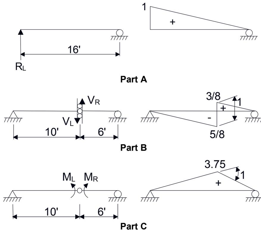
**Figure 4.4.3.1-1 Application of the Müller-Breslau Principle**
