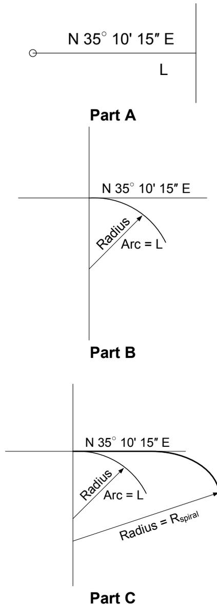
**Figure 4.5.3.2.2-1 Horizontal Node Layout for Different Alignments**
