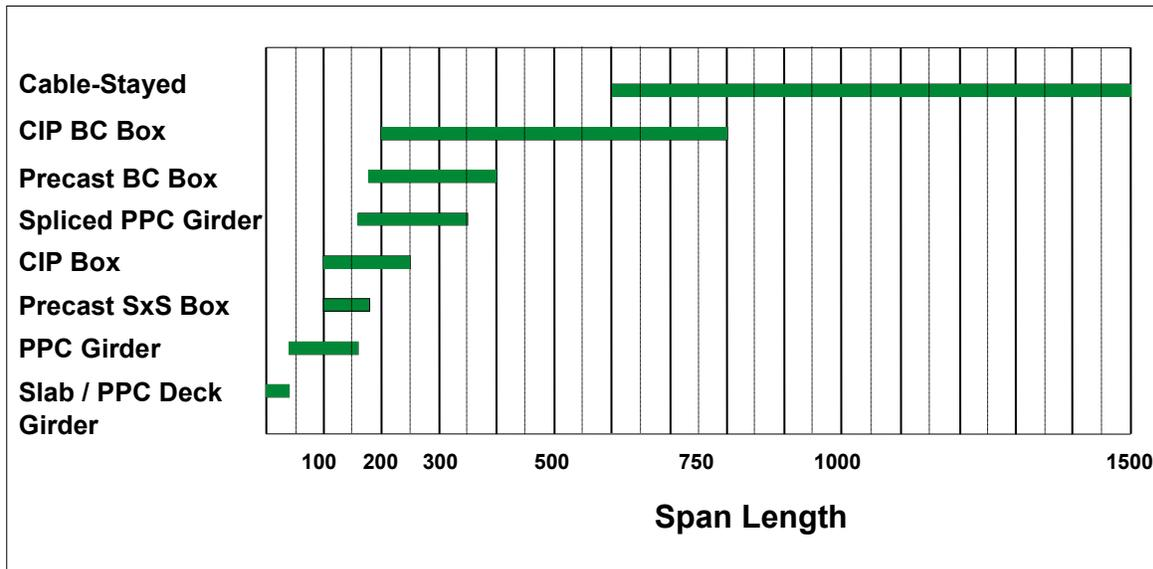
**Figure 5.4.2-8 Bridge Type vs. Applicable Span Range**
