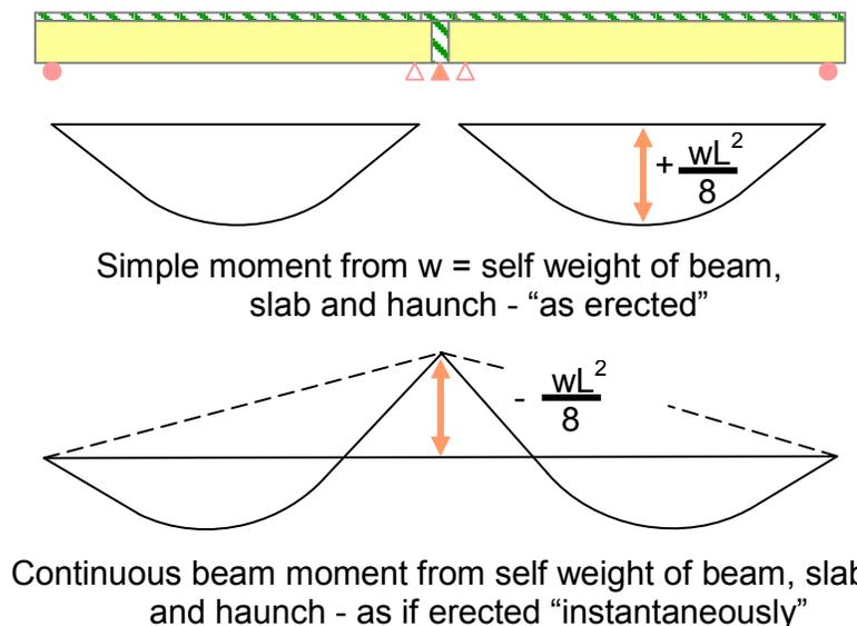
**Figure 5.10.3.3.2.1-4 Two-Span, Self-Weight Continuity Moment**
