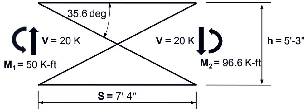
**Figure 4.5.3.2.2.5.3-9 Global Forces on Example Cross-Frame from 2D Analysis Model**
