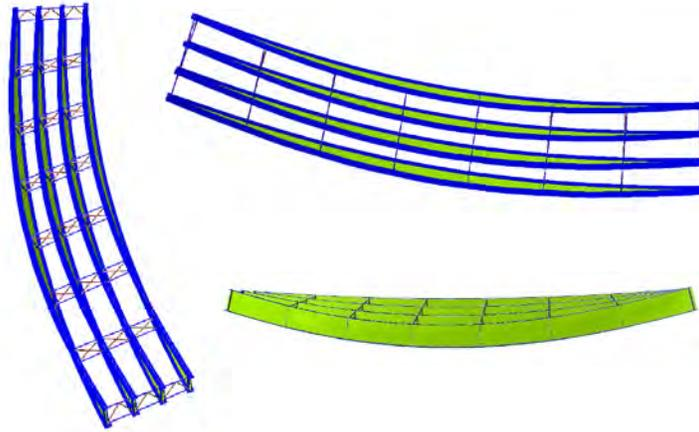
**Figure 6.4.9.5.1.2-1 Magnified Girder Vertical Deflections and Twist for Four Horizontally Curved Simple Span I-Girders on Non-Skewed Supports Subjected to Steel Dead Load**
