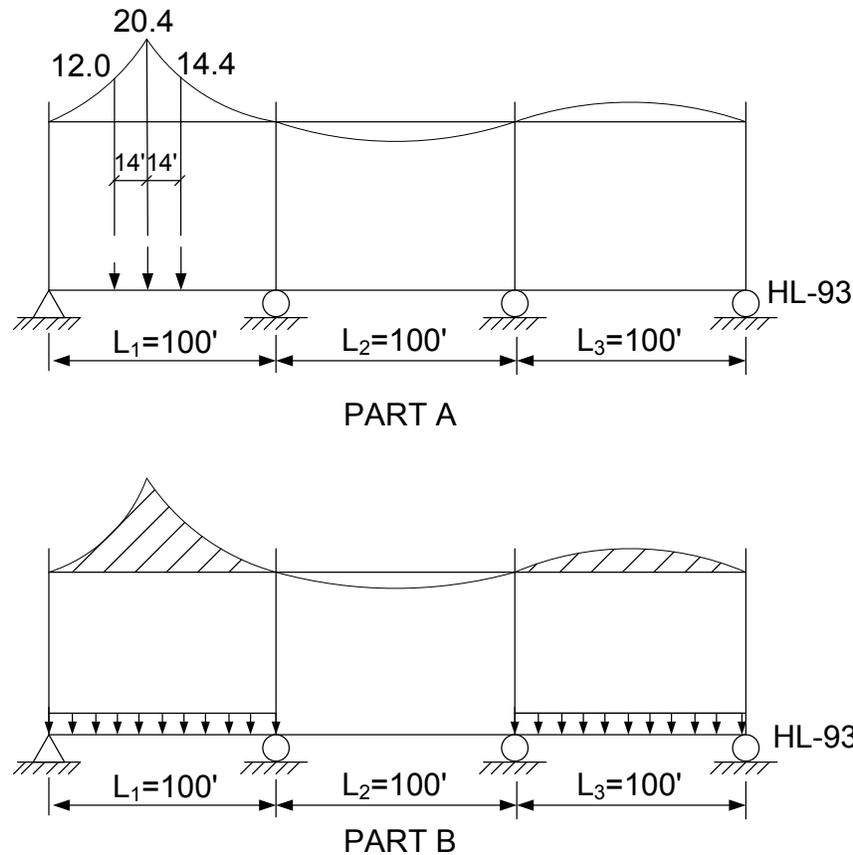
**Figure 4.4.3.1-3 Application of HL-93 Live Load to an Influence Line for a Three-Span Continuous Beam to Determine the Vertical Bending Moment at  $0.4L_1$**
