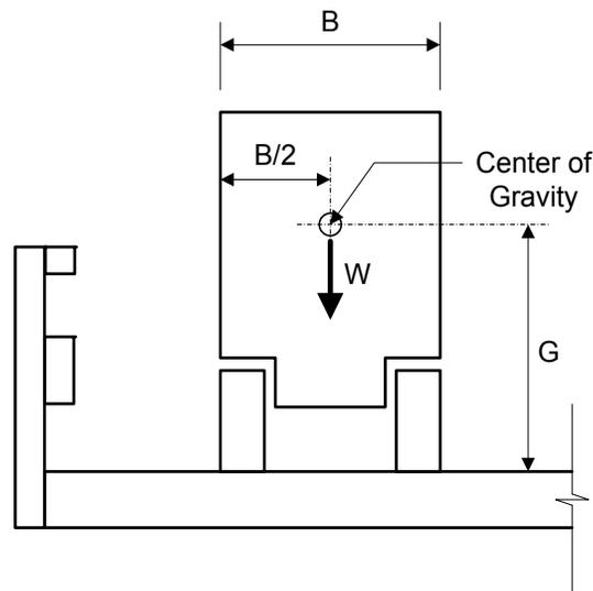
**Figure 3.4.11-1 Vehicular Collision Force**
