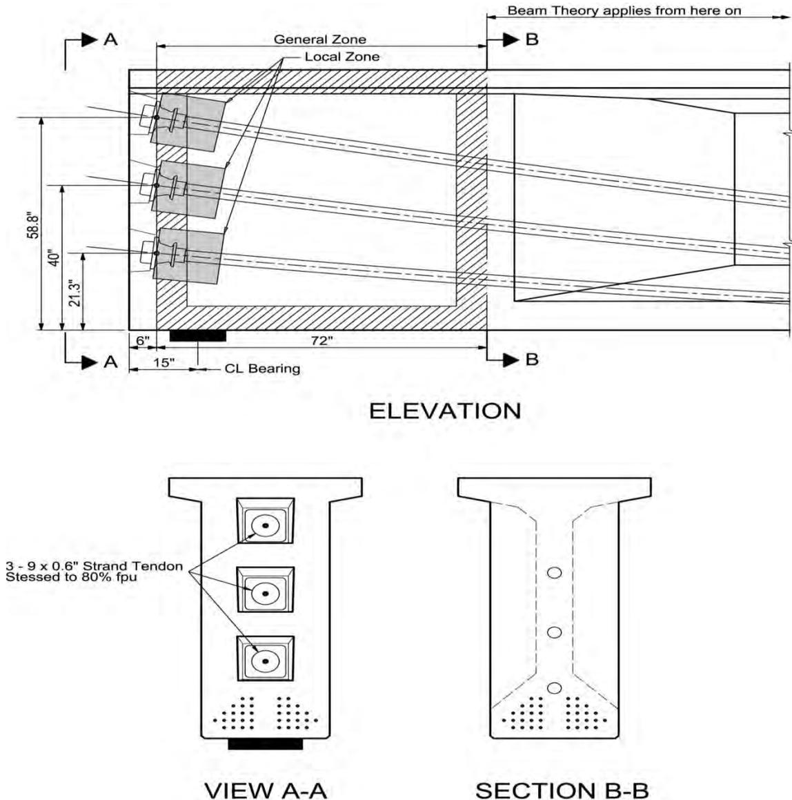
Figure 5.7.5.2.2-1 Anchor Zones for a Post-Tensioned Girder
