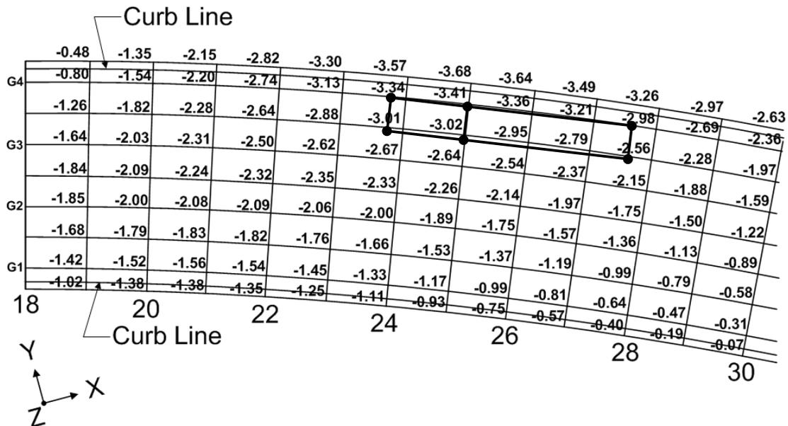
**Figure 4.4.3.2.2-12 Wheel-Load Model of the Fatigue Live Load Positioned on Influence Surface to Maximum the Negative Vertical Bending Moment at Node 24**
