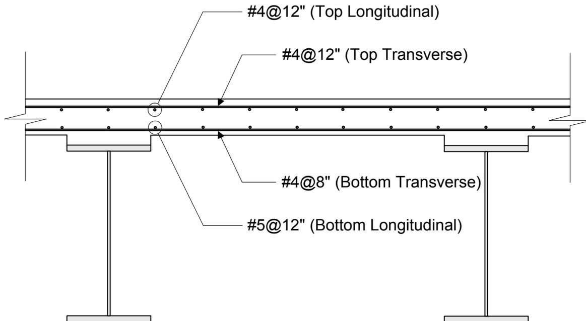
**Figure 7.3.3.4-1 Bridge Deck Based on Empirical Design Method**
