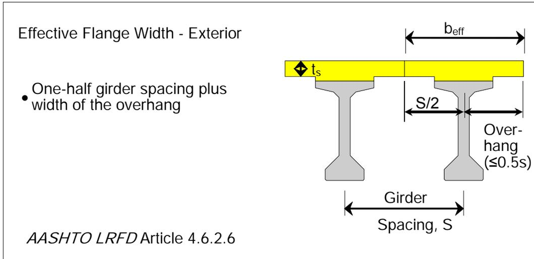
Figure 5.5.3.2.2-2 Effective Flange Width of Exterior Girder
