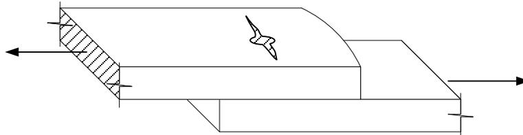
**Figure 6.6.4.2.5.6.1-1 Tensile Failure of a Connected Element by Net Section Fracture**
