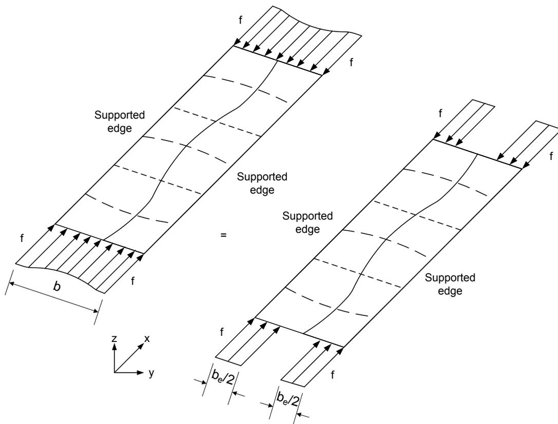
**Figure 6.6.3.4.2.4.3-3 Average vs. Idealized Stress Distribution Across the Width of a Post-Buckled Stiffened Plate Element**
