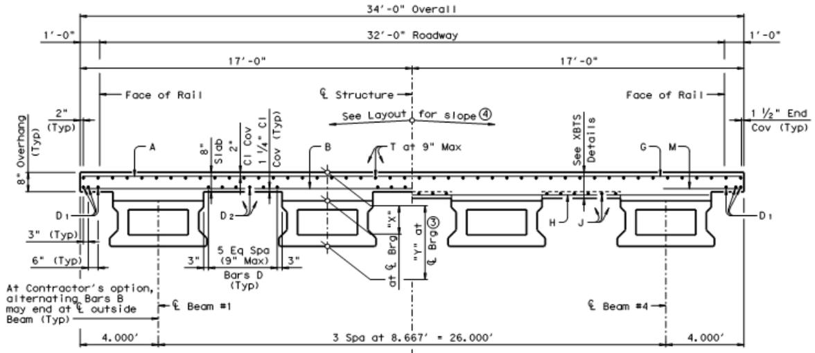
Figure 5.4.2-3 Spread Precast Box Beam Bridge
