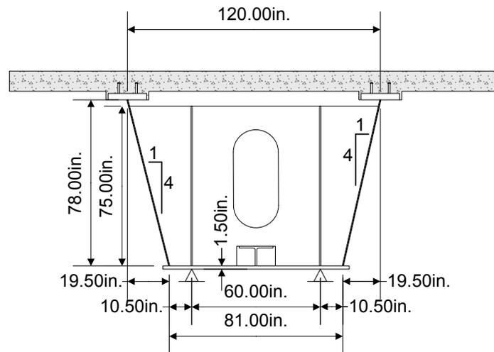
**Figure 6.6.3.6.2-1 Example Tub Girder Section at an Interior Pier**
