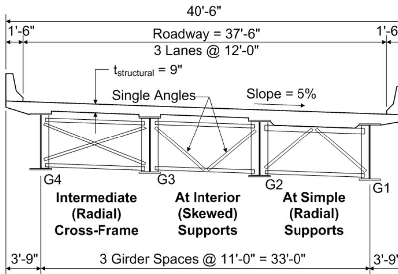
Figure 3.4.9.4-1 Example I-Girder Bridge Cross Section
