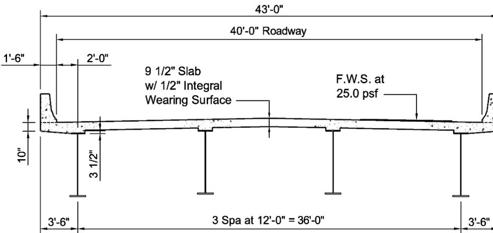
**Figure 6.5.4.2.2-1 Straight Steel I-Girder Bridge Example Cross-Section**
