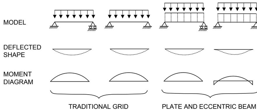
**Figure 4.5.3.2.2.4-1 Effects of Different Boundary Condition Assumptions on Traditional Grid and Plate and Eccentric Beam Models**
