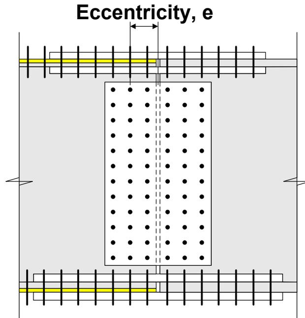
**Figure 6.6.5.2.3.2.2-1 Eccentricity of the Design Shear for a Web Splice**
