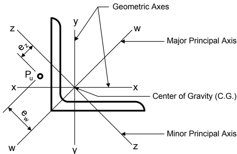
Figure 6.6.3.4.5.1-1 Single-Angle Member Geometry
