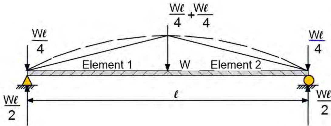
**Figure 4.3.2-1 Discretization of Model for Deck Weight Using Two Elements – Bending Moment**
