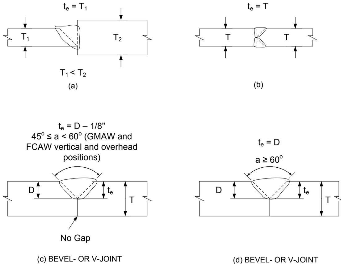
**Figure 6.6.4.3.3.2-1 Effective Throat Dimensions for Groove Welds (SMAW, SAW, GMAW & FCAW)**
