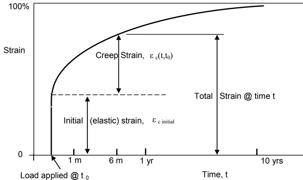
**Figure 5.10.3.3.7-1 Development of Creep Strain with Time**
