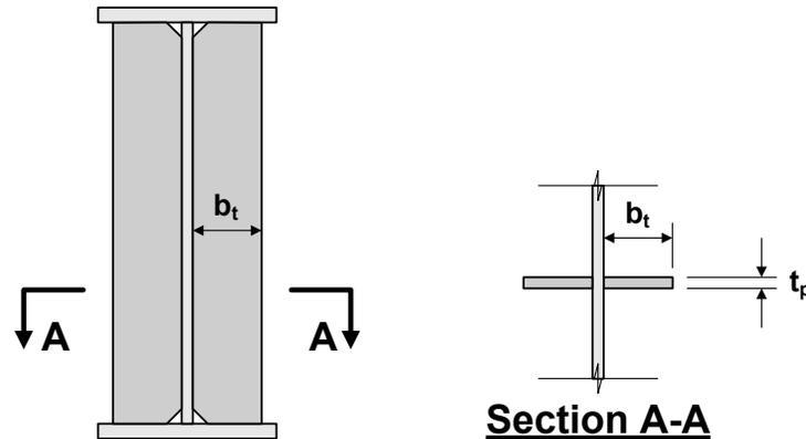
Figure 6.6.6.3.2-1 Projecting Width of Bearing Stiffener
