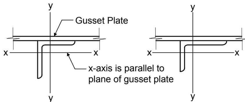
**Figure 6.6.3.4.5.2-1 Single-Angle Geometric Axes Utilized in the Effective Slenderness Ratio Expressions - for Equal-Leg Angle and Unequal-Leg Angle Connected Through the Longer Leg**
