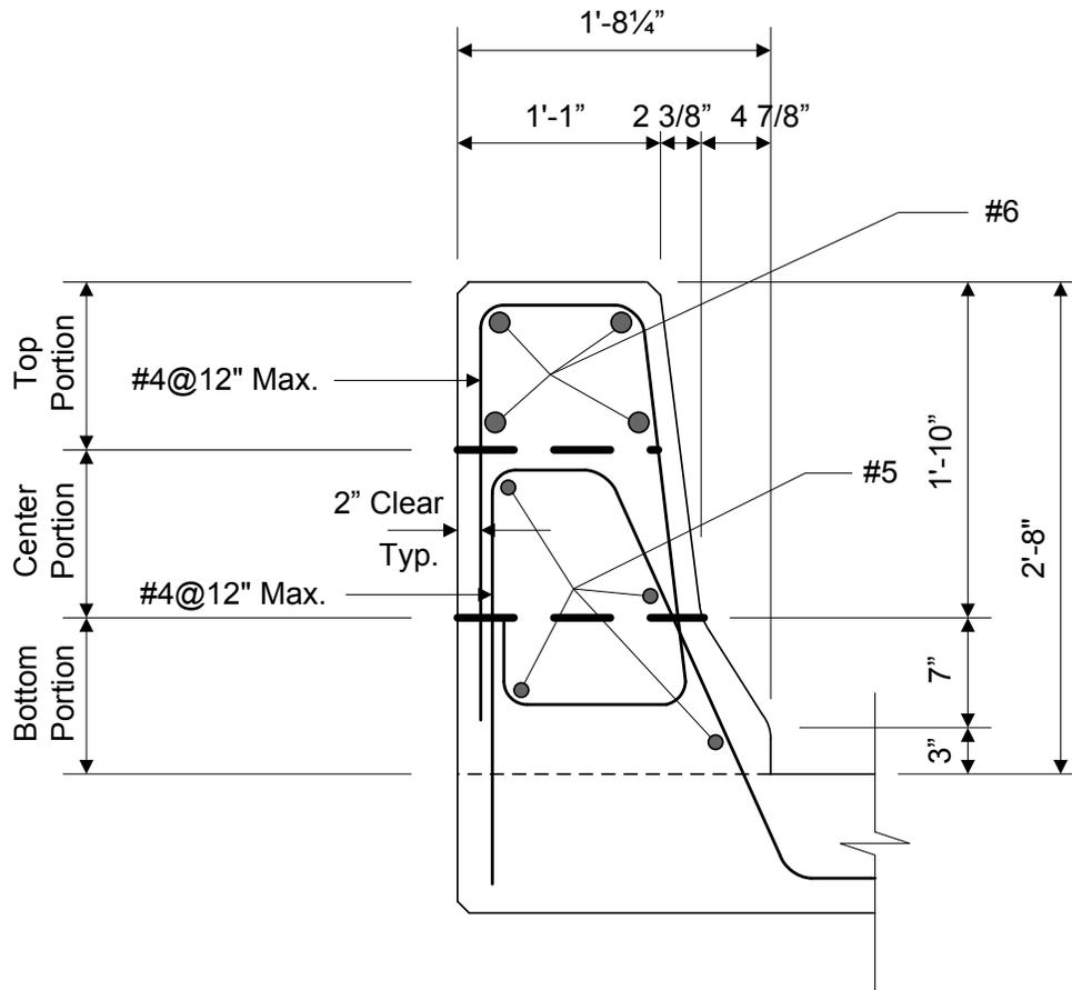
Figure 7.3.4.2.1-3 Three Portions of Barrier for Computation of  $M_w$
