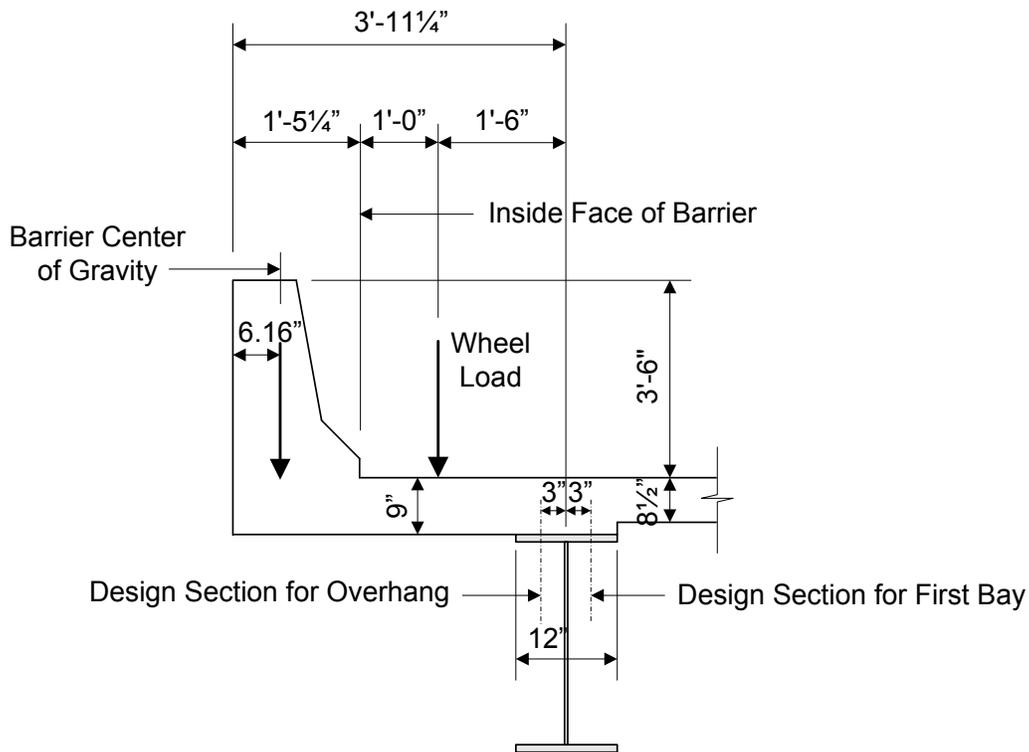
**Figure 7.3.4.1-1 Deck Overhang Dimensions and Live Load**
