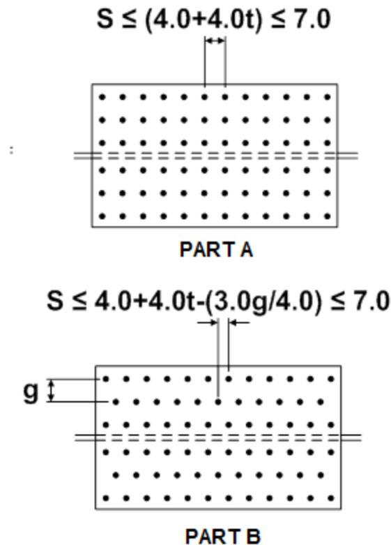
**Figure 6.6.4.2.2.2-1 Maximum Spacing Requirements for Sealing Bolts**
