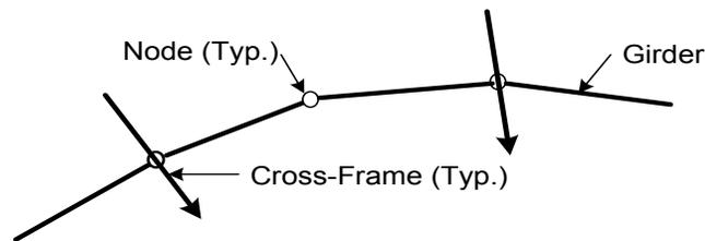
**Figure 4.5.3.2.2.5.2-1 Additional Node Placed in-between the Cross-Frames in a 2D Model of a Horizontally Curved Girder**
