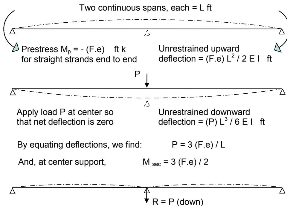
Figure 5.10.3.2.3.4-1 Secondary Reaction and Moment in Continuous Beam
