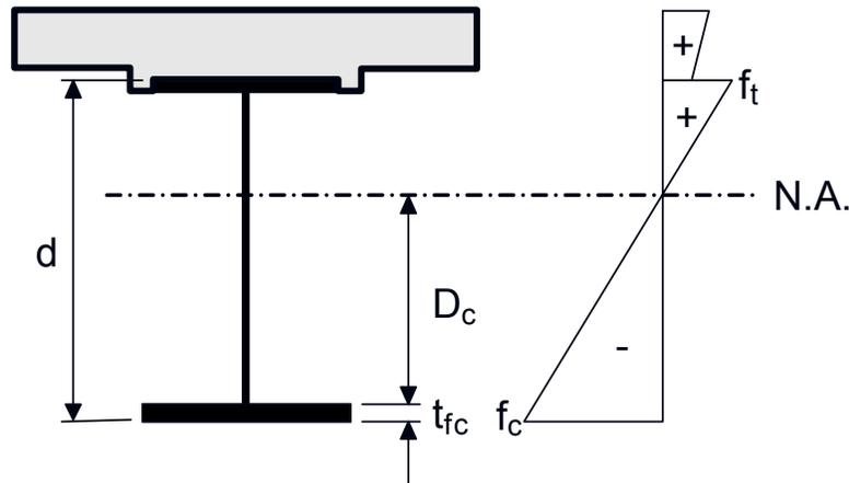
**Figure 6.4.5.4.1.3-1  $D_c$  for a Composite Section in Negative Flexure**
