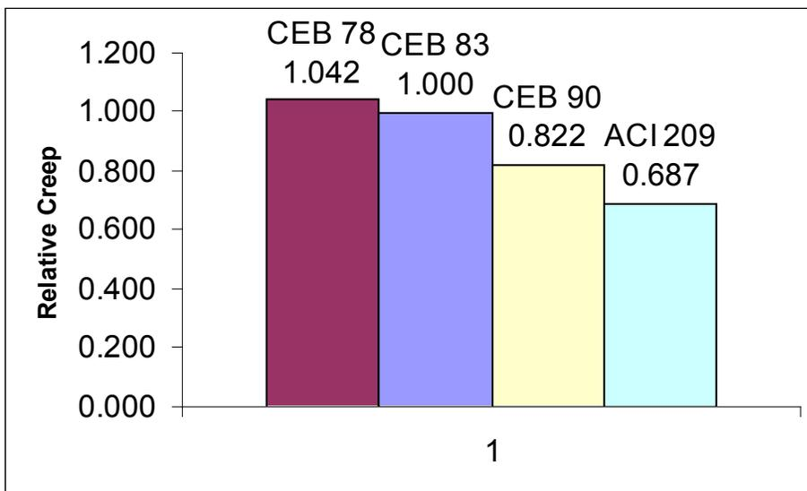
Figure 5.2.1.2.3.2-3 Relative Creep by Different Codes
