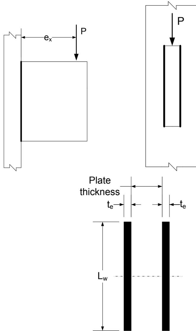
**Figure 6.6.4.3.7.2.3-3 Eccentrically Loaded Fillet Welded Connection Subject to Combined Shear & Bending**
