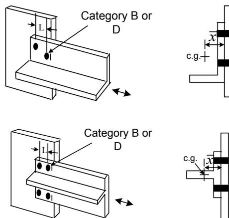
**Figure 6.6.3.3.5.3-1 Bolted Connection of a Single-Angle and a Tee Member to a Gusset Plate**
