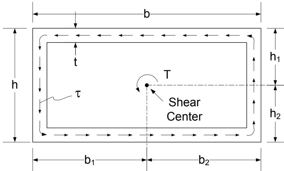
**Figure 6.4.8.3.2-3 Shear Flow for a Thin-Walled Rectangular Box Section**
