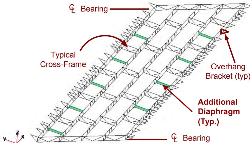
**Figure 4.5.3.3.2.5.1-1 Overhang Brackets in a 3D Model**
