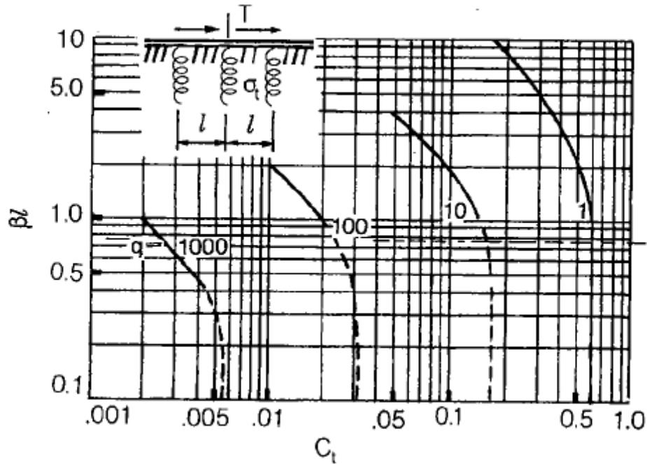
Figure 6.5.5.2.2.3.2-8 BEF Factor,  $C_t$ , for Distortional Transverse Bending Stress at Cross-Bracing due to a Concentrated Torque,  $T$ , at Cross-Bracing
