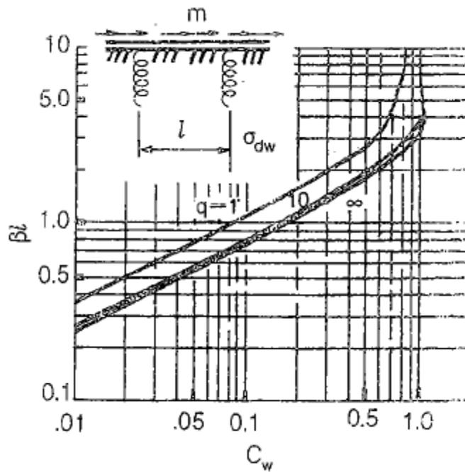
Figure 6.5.5.2.3.2-3 BEF Factor,  $C_w$ , for Distortional Longitudinal Warping Stress at Cross-Bracing due to a Uniform Torque,  $m$
