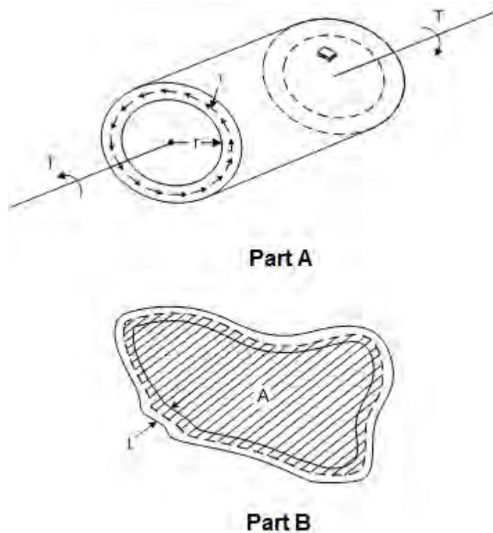
**Figure 6.4.8.3.2-2 Cylindrical Tube and Enclosed Area of a Hollow Shaft**
