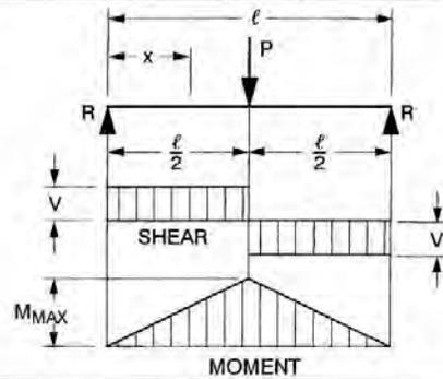
**(3) SIMPLE BEAM – CONCENTRATED LOAD AT ANY POINT**
