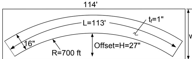
Allow 3 in. for cutting and plate camber
