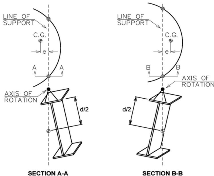
**Figure 6.3.2.4.3.2-3 Rigid Body Rotation of a Horizontally Curved Girder During Lifting**
