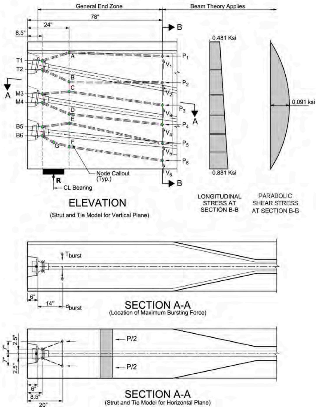
**Figure 5.7.5.2.4-1 Strut-and-Tie Models for a Post-Tensioned Girder**
