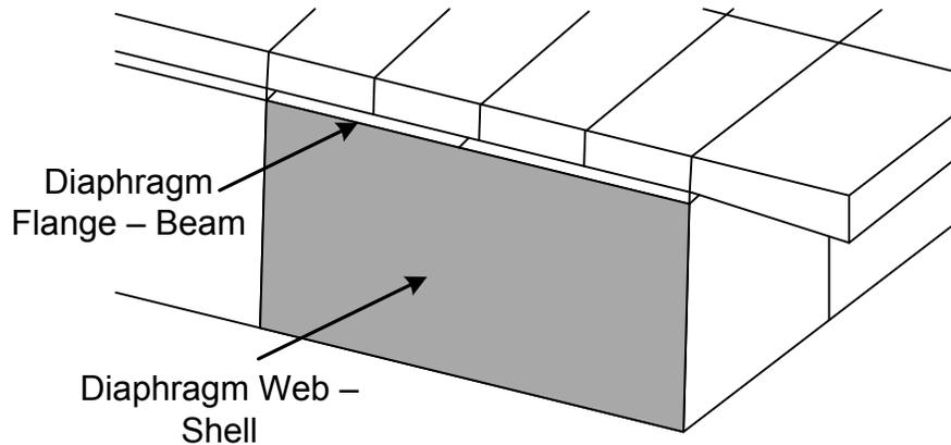
**Figure 4.5.3.3.2.3.6-2 Shell Elements Used to Model Diaphragm Webs and Beam Elements Used to Model Diaphragm Flanges**
