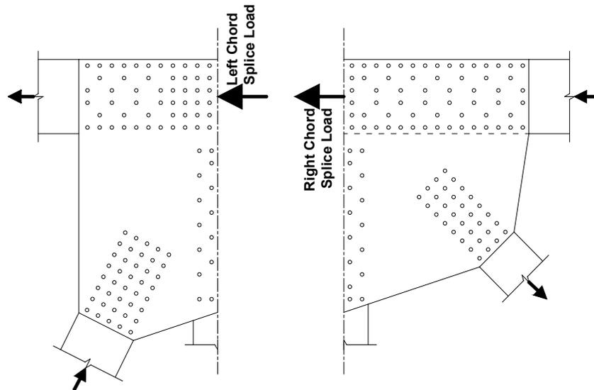
**Figure 6.6.7.5-1 Example Connection Showing the Resolution of the Member Forces into Forces Acting on Each Side of a Chord Splice**
