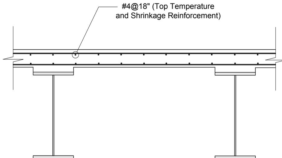
**Figure 7.3.2.5-2 Temperature and Shrinkage Reinforcement in Top of Deck**
