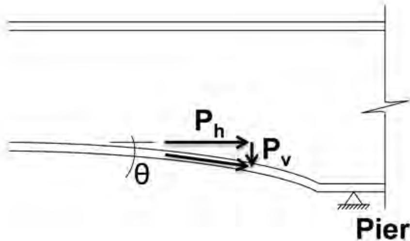
**Figure 6.3.3.2.2-3 Vertical and Horizontal Components of Force in the Inclined Bottom Flange of a Parabolic Haunch at an Interior Pier**
