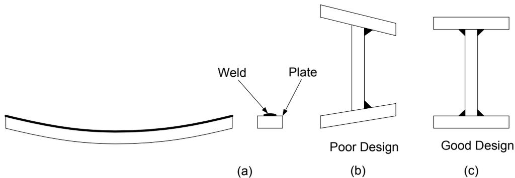
**Figure 6.6.4.3.5-1 Welding Distortion**
