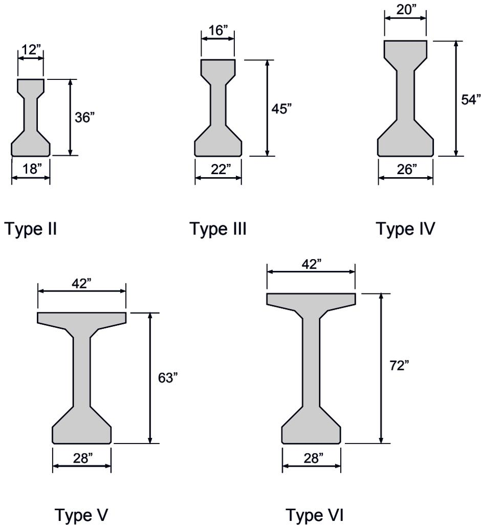
**Figure 5.10.3.1.1-1 Standard AASHTO I-Girder Sections for Prestressed Bridges**
