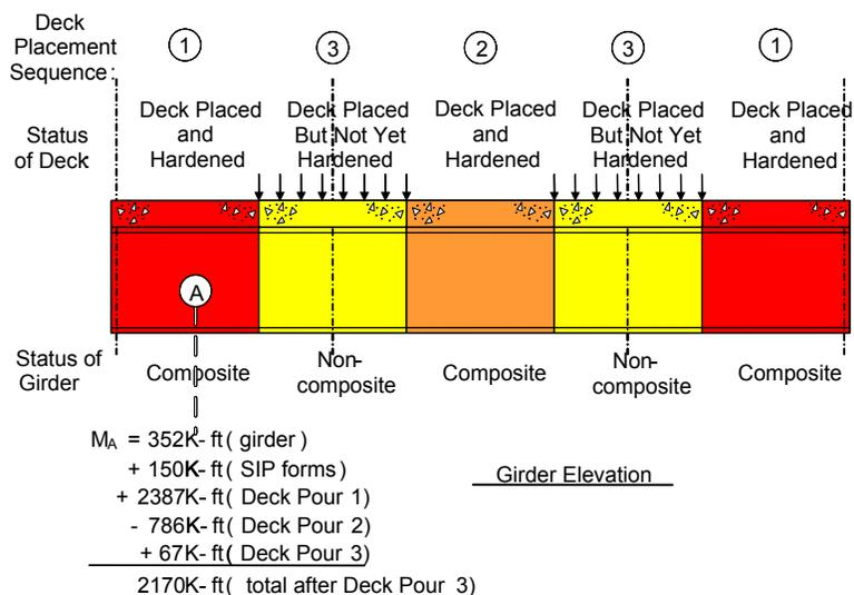
**Figure 6.5.3.3.4-6 Sample Deck Placement Analysis (Cast 3)**
