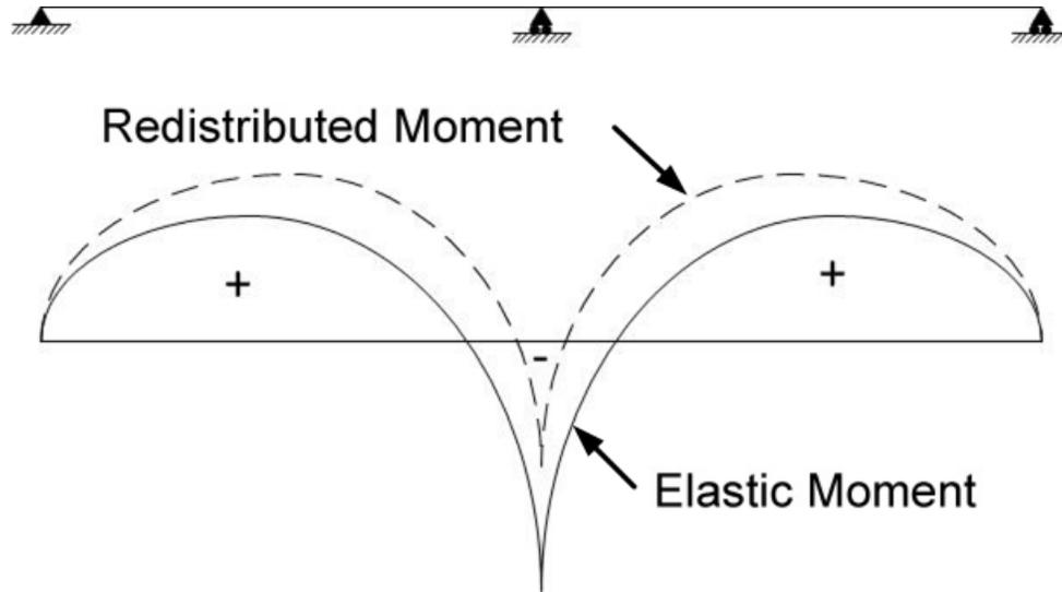
**Figure 4.2.6-1 Redistribution of Bending Moment in a Multi-Span Girder Superstructure**
