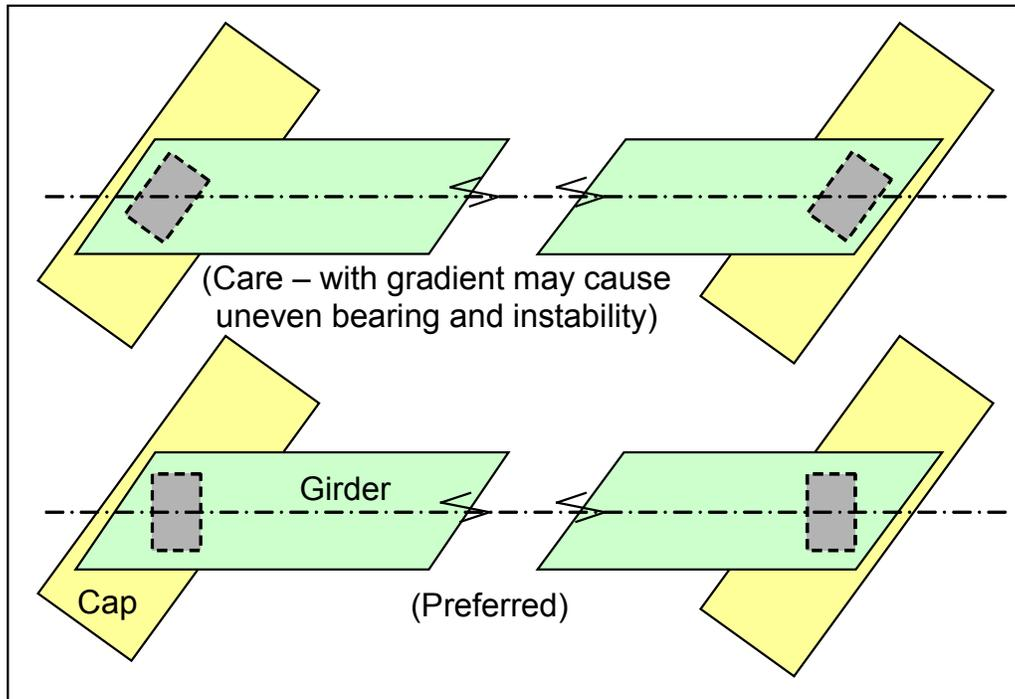
**Figure 2.3.3.2-2 Bearing Orientation for High Skew**
