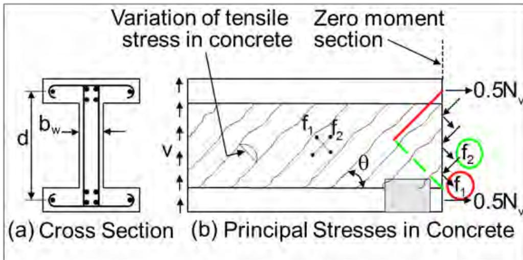
**Figure 5.6.1.1.4-1 Equilibrium Conditions by Modified Compression Field Theory in Diagonally Cracked Beam**
