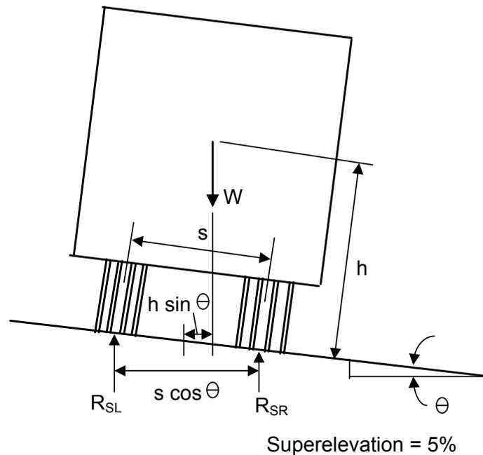
**Figure 3.4.9.1-2 Effects of Superelevation on Wheel-Load Reactions**
