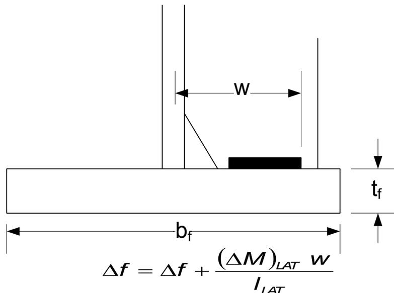
**Figure 6.5.5.2.2.1.5-1 Effect of Bottom Flange Lateral Bending on the Stress Range**
