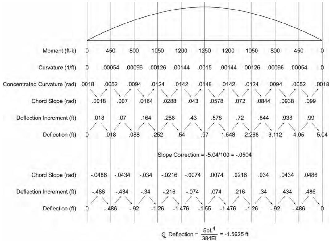
**Figure 5.5.8.2-6 Numerical Integration for Slopes and Deflections (Newmark)**
