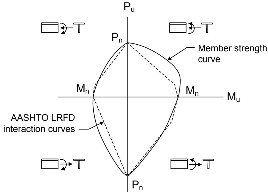
**Figure 6.6.3.4.3.3-1 Interaction Curves for Tees Subjected to Combined Axial Forces and Flexure**
