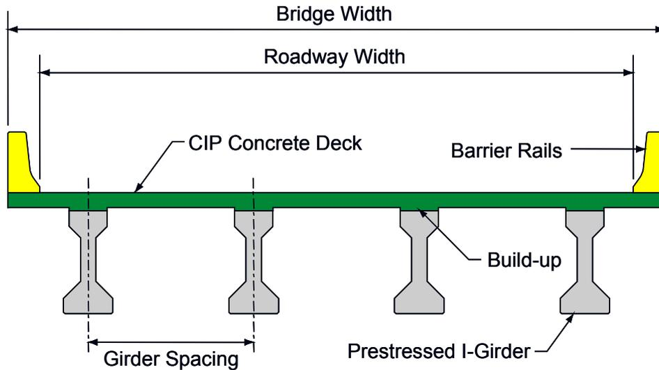
**Figure 5.10.3.1-1 Typical Prestressed Concrete Girder Bridge Deck**
