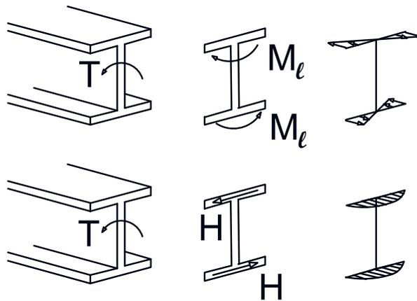
**Figure 6.4.8.2.3-2 I-Sections with Effects of Warping Torsion**
