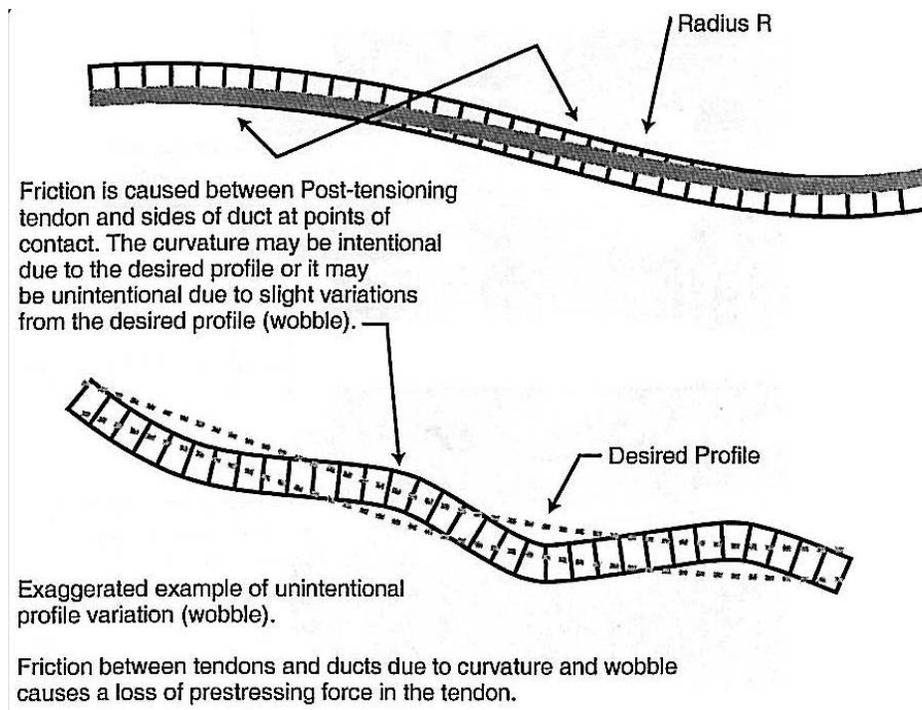
**Figure 5.7.3.3.1.2-1 Friction Caused by Wobble and Duct Curvature**
