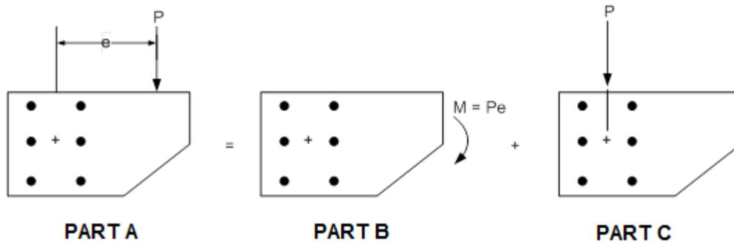
**Figure 6.6.4.2.6-1 Bolted Connection Subject to Eccentric Shear**
