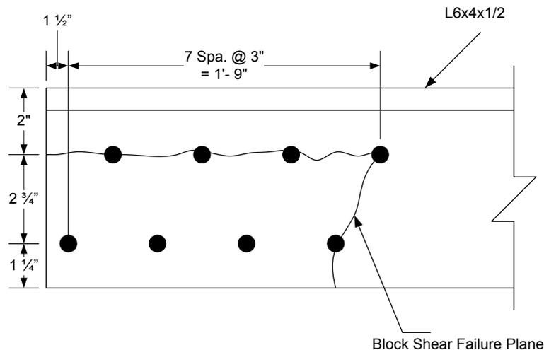
**Figure 6.6.3.3.2.5-4 Example – Assumed Block Shear Failure Planes in Single-Angle Bracing Member**
