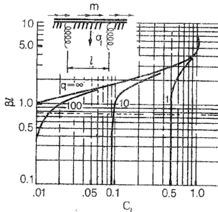
Figure 6.5.5.2.2.3.2-5 BEF Factor,  $C_t$ , for Distortional Transverse Bending Stress at Midpanel due to a Uniform Torque,  $m$
