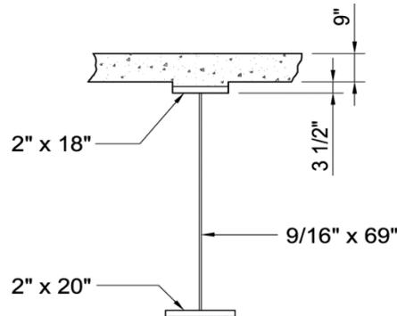
**Figure 6.4.2.3.3-1 Example Composite Cross-Section – Exterior Girder – Negative Flexure Region**
