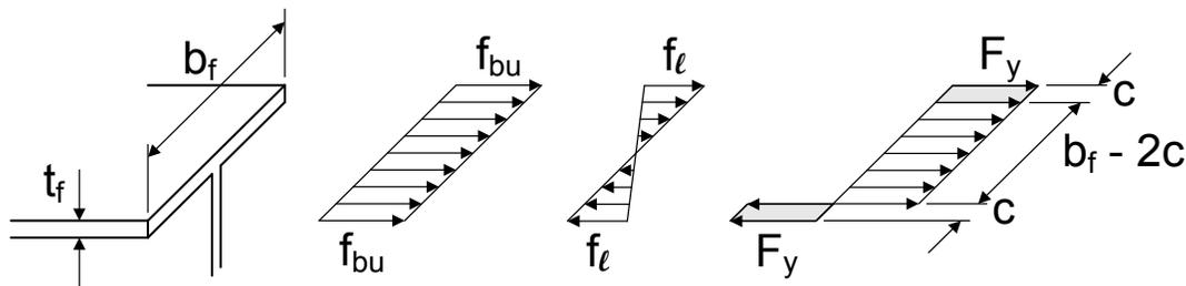
**Figure 6.5.2.1.2-1 Fully-Plastic Stress Distribution under Combined Vertical and Lateral Bending (Compact Flange)**
