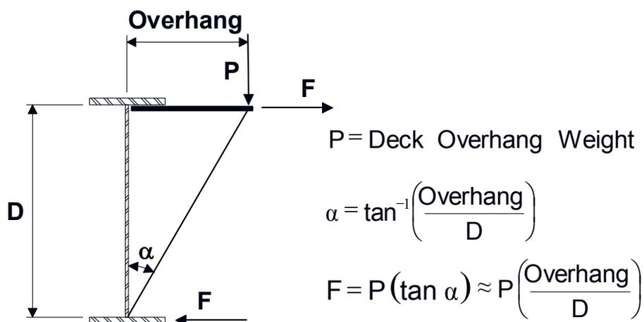
Figure 6.5.3.4.2-1 Lateral Flange Forces from Deck Overhang
