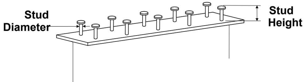
Figure 6.6.2.2.2-1 Minimum Height-to-Diameter Ratio
