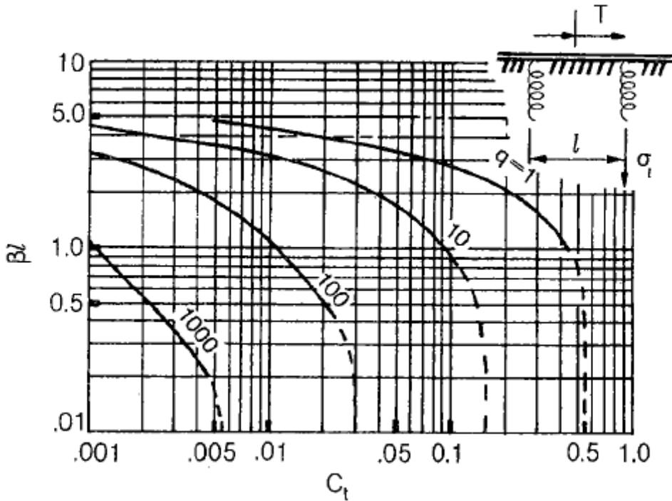
Figure 6.5.5.2.3.2-7 BEF Factor,  $C_t$ , for Distortional Transverse Bending Stress at Cross-Bracing due to a Concentrated Torque,  $T$ , at Midpanel
