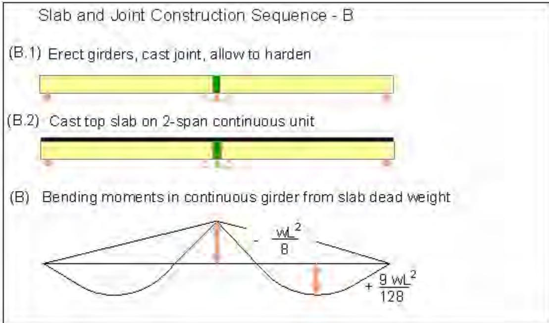
**Figure 5.10.3.2.3.3-2 Construction Sequence Effects – Case (B)**
