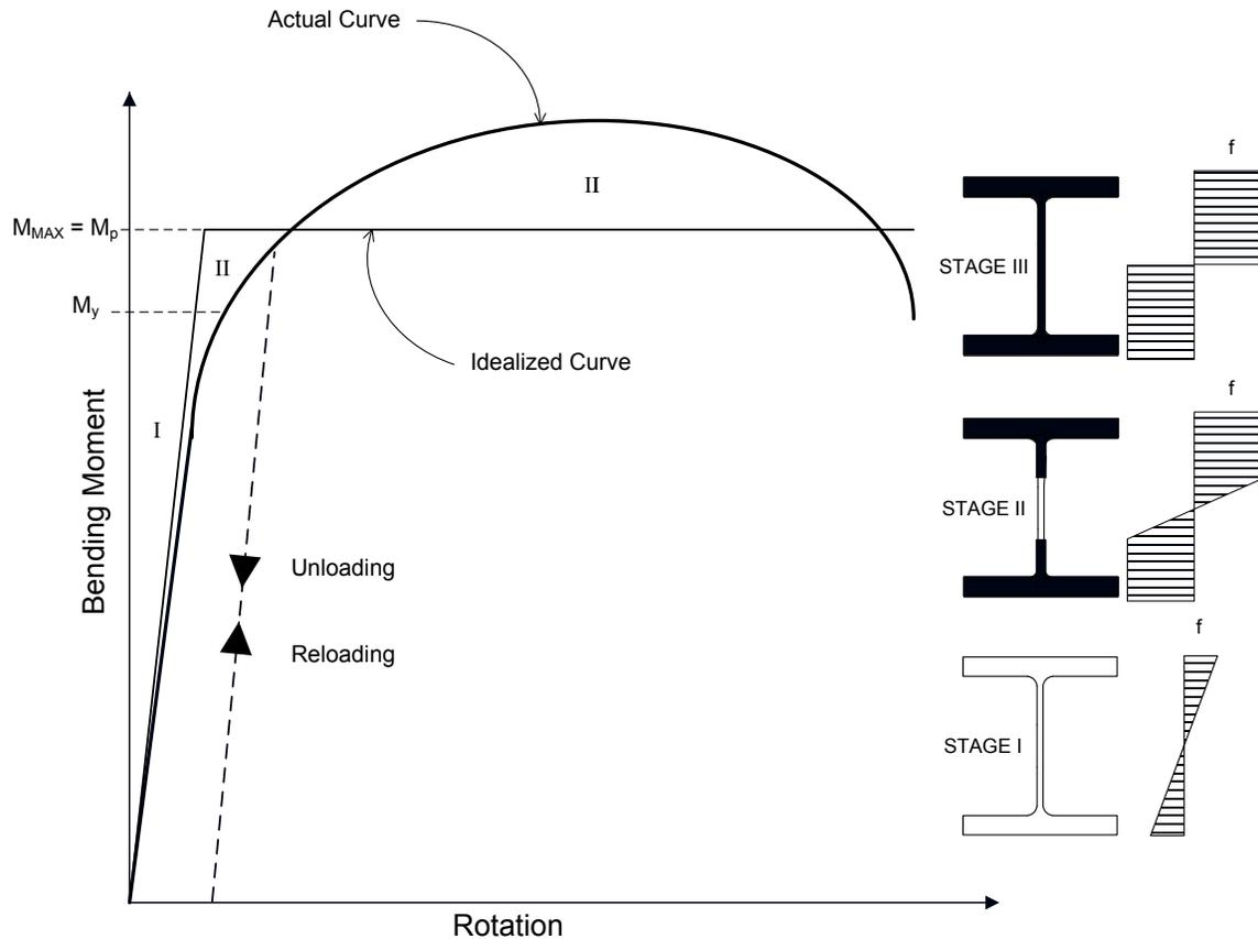
**Figure 6.5.6.2.1.2-1 Bending Moment versus Rotation for a Homogenous Compact Web Section**
