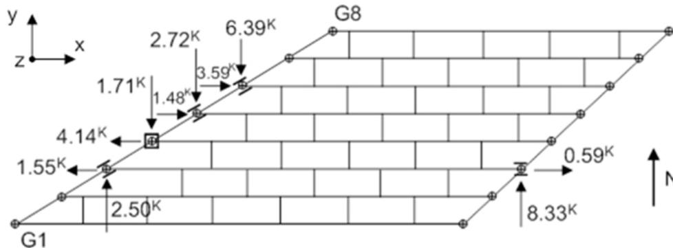
**Figure 6.3.3.3.7-9 Horizontal Bearing Reactions (X-Y Plane) due to Thermal Expansion – Guided Bearings All Guided Toward Fixed Bearing at West End of G4**
