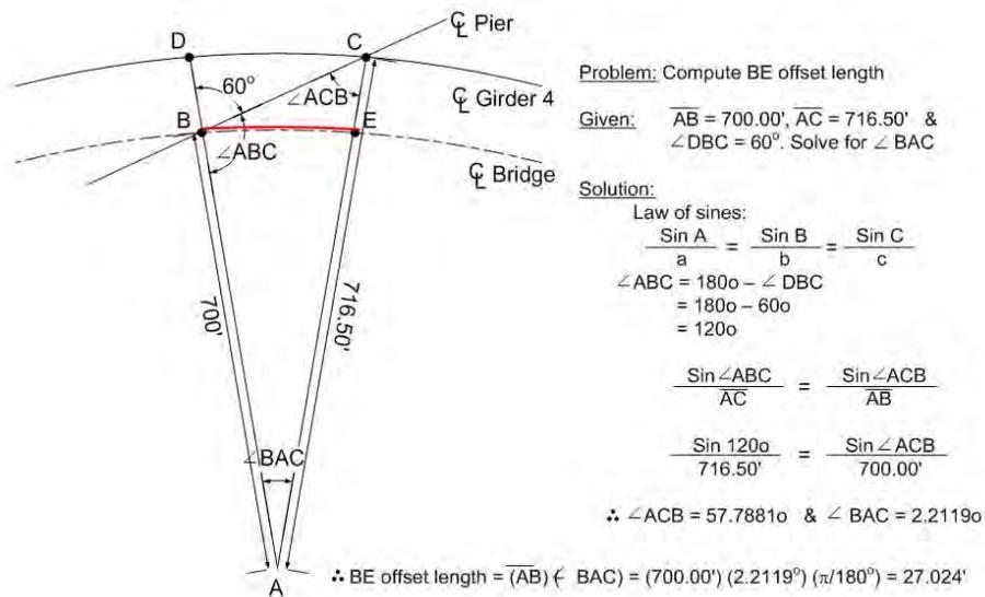
**Figure 4.5.3.3.2.2-2 Calculation of Offset Length for Skewed Support Nodes**
