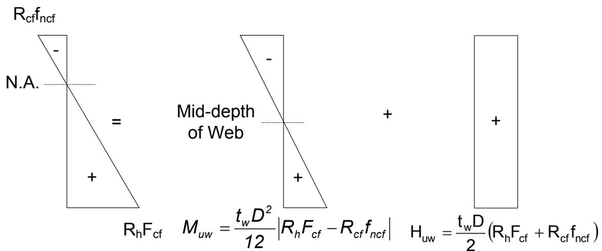
**Figure 6.6.5.2.3.2.3-1 Assumed Flexural Stress Distribution in the Web for the Design of a Bolted Web Splice in a Composite Section Subject to Positive Flexure**
