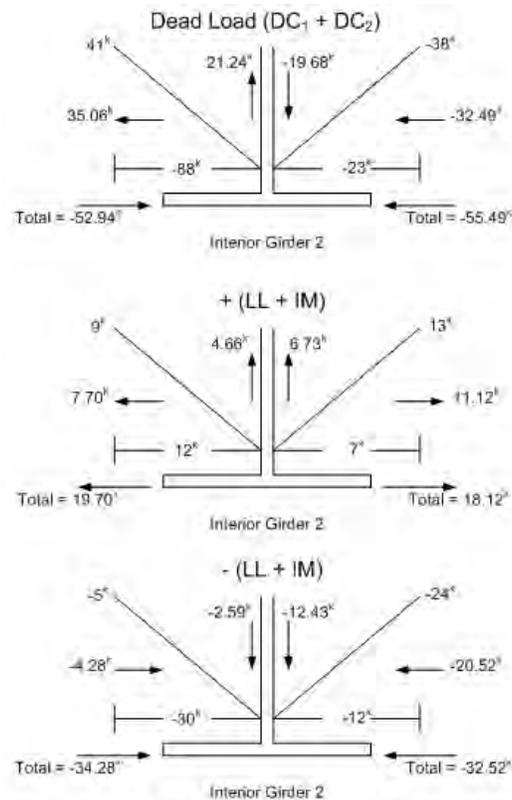
**Figure 6.6.4.4-4 Equilibrium Check for  $DC_1 + DC_2$ ,  $(+LL+IM)$  and  $(-LL+IM)$  Cross-Frame Horizontal Forces at the Bottom of an Interior Girder**
