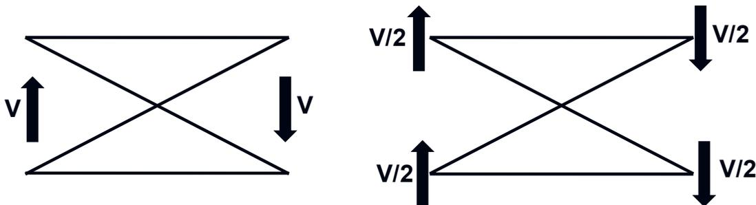
**Figure 4.5.3.2.2.5.3-7 Assumed Distribution of Shear Forces for an X-Type Cross-Frame**
