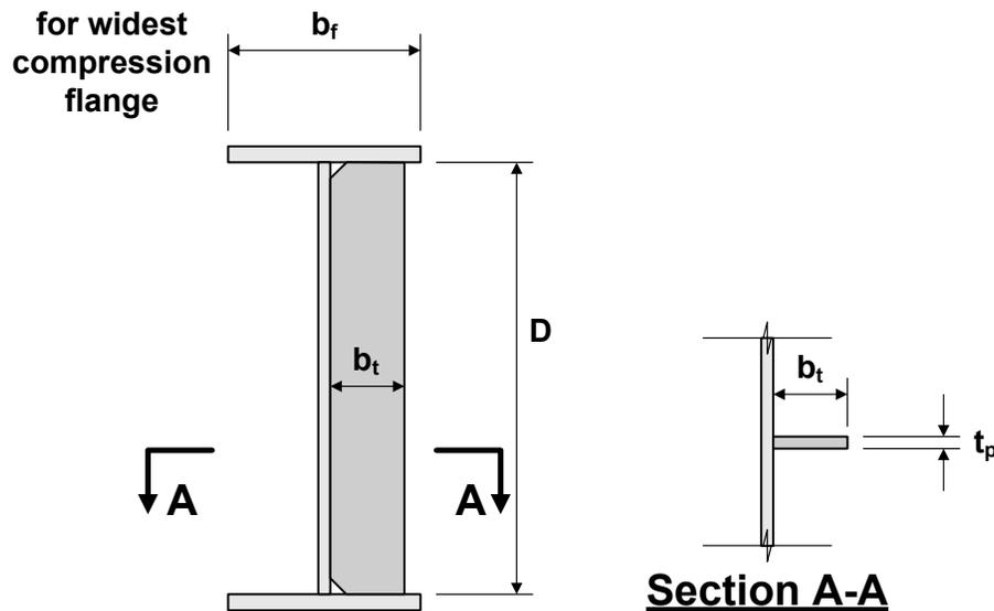
**Figure 6.6.6.2.2-1 Projecting Width of Transverse Stiffeners**
