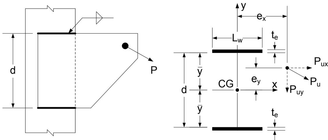
**Figure 6.6.4.3.7.2.3-1 Eccentrically Loaded Fillet Welded Connection Subject to Combined Shear & Torsion**
