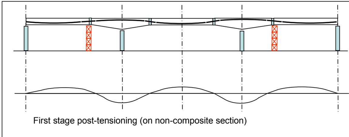
**Figure 5.10.4.2-4 Spliced Girder Construction - Stage 1 PT Moments**
