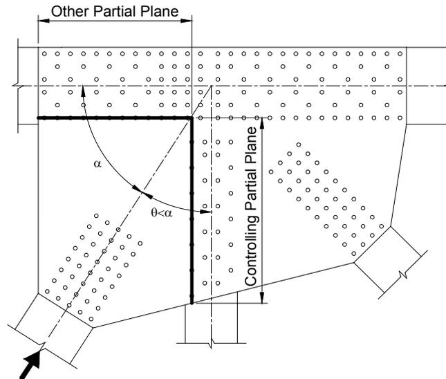
**Figure 6.6.7.2-2 Example of a Controlling Partial Shear Plane on the Side of a Compression Member Without a Chamfered End that has the Smaller Framing Angle between that Member and the Other Adjoining Members (i.e.  $\theta < \alpha$ )**
