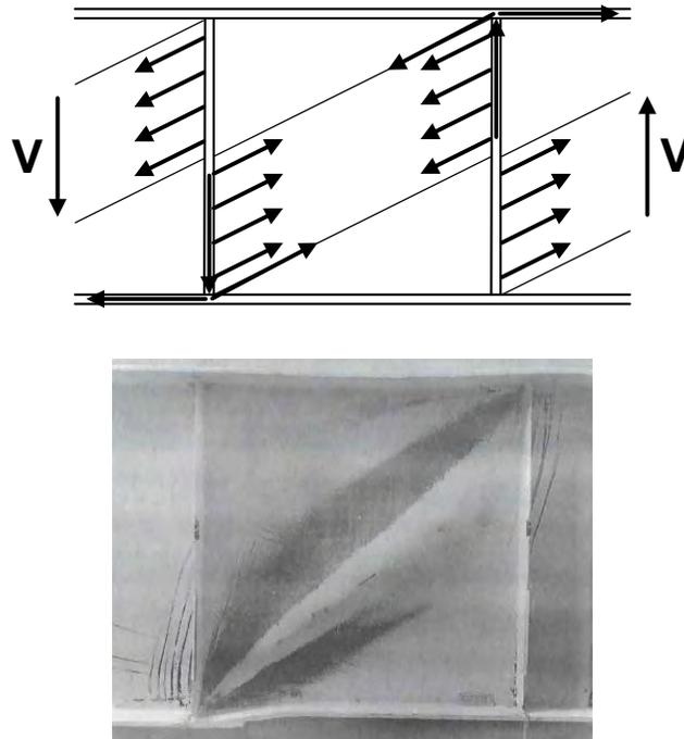
**Figure 6.5.7.3-1 Web Post-Buckling Shear Resistance – Tension-Field Action**
