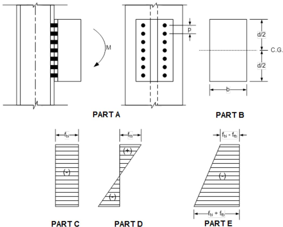
**Figure 6.6.4.2.5.5-2 Tension and Shear from Eccentric Loading – Stresses on Contact Area**
