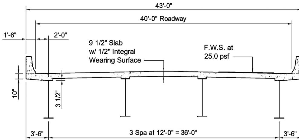
**Figure 6.5.3.4.4.1-2 Example Bridge Cross-Section**
