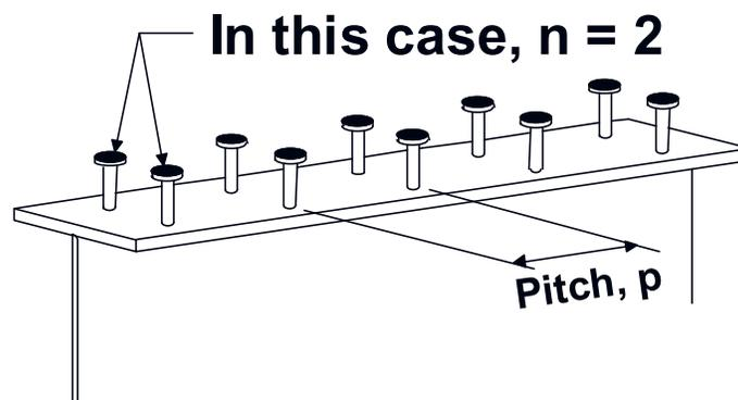
Figure 6.6.2.3.2.1-1 Number of Shear Connectors in a Cross-Section,  $n$
