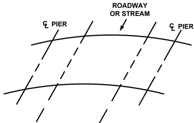
**Figure 6.4.9.3-1 Curved Bridge with Skewed Supports to Match Roadway/Stream**
