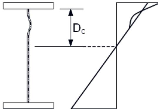
**Figure 6.4.5.6-1 Load Shedding from the Web to the Compression Flange**
