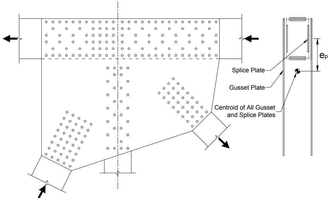
**Figure 6.6.7.5-3 Illustration of the Combined Spliced Section at a Chord Splice**
