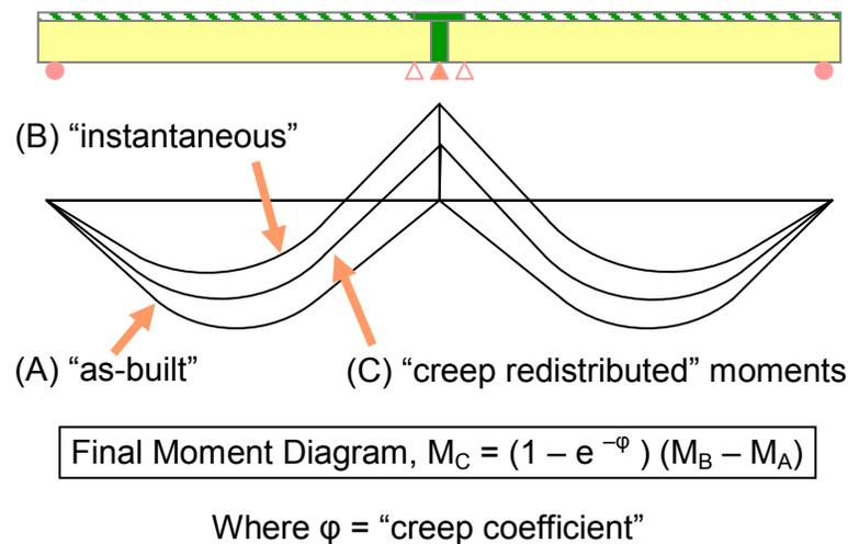
**Figure 5.10.3.3.1-1 Creep Redistribution of Slab Weight in Continuous Spans**
