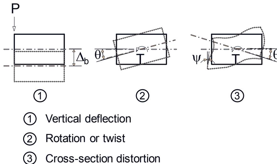
**Figure 6.4.8.3.1-1 Deformation of Box Sections**
