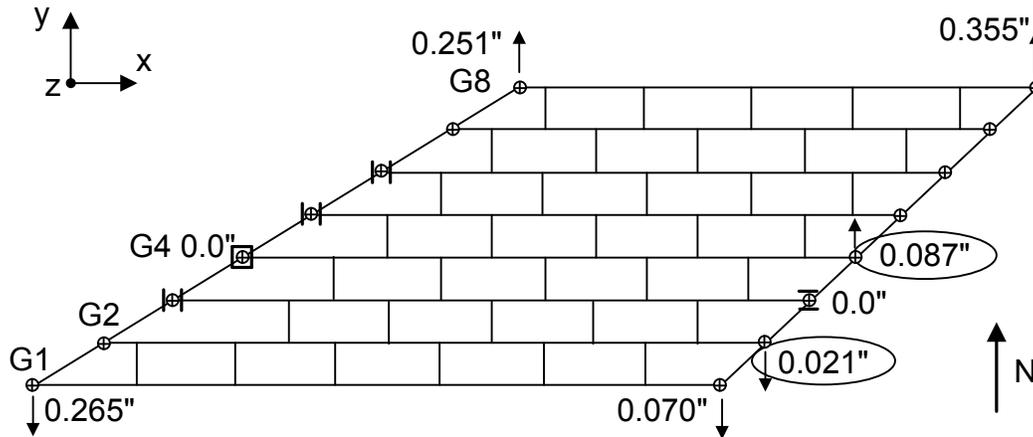
**Figure 6.3.3.3.7-6 Transverse (Lateral) Thermal Expansion with a Single Bearing Constrained Transversely at Each End**
