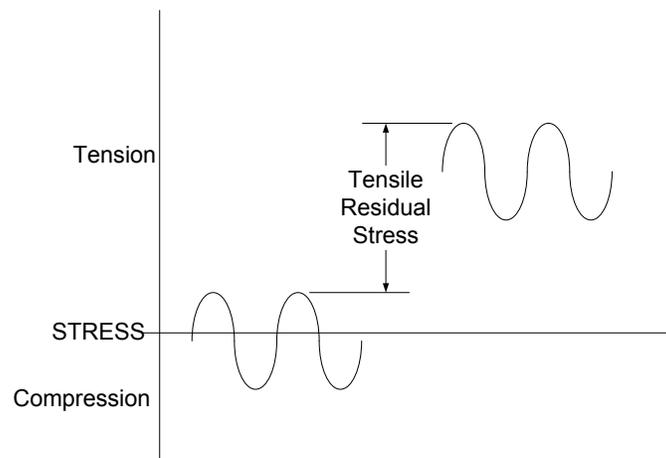
**Figure 6.5.5.2.2.1.1-2 Effect of Tensile Residual Stress on a Stress Cycle**
