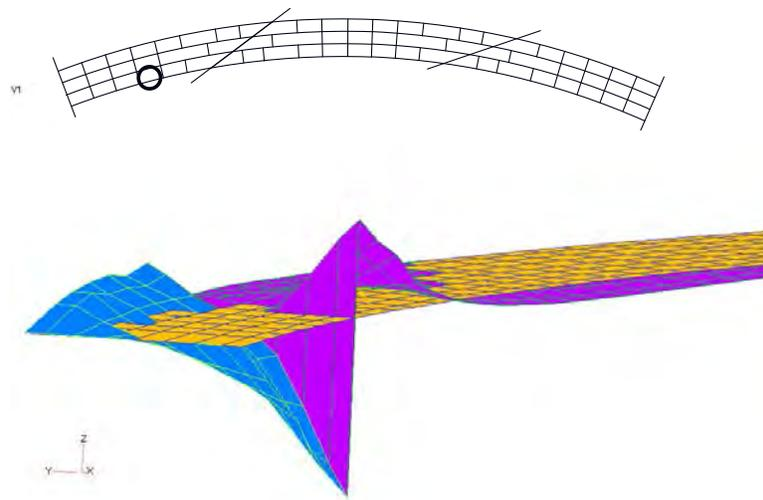
**Figure 4.4.3.2.1-3 Influence Surface for Vertical Shear in Span 1 of G1 of the Example I-Girder Bridge**
