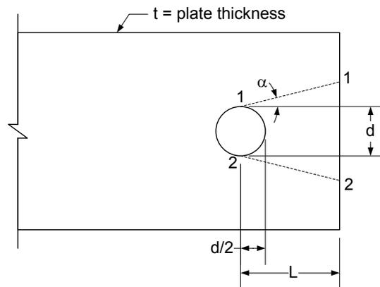
**Figure 6.6.4.2.5.3-2 Bearing Resistance Related to End Distance**
