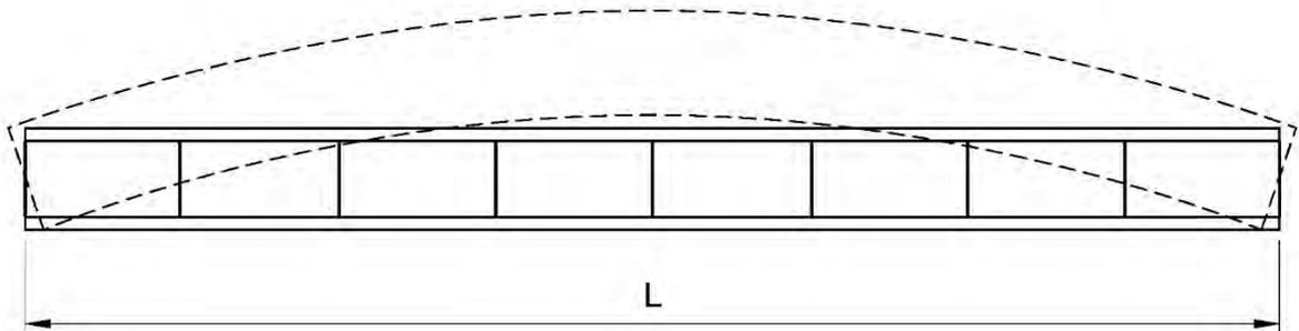
**Figure 6.5.3.3.5-1 Global Displacement Amplification in a Slender I-Girder Bridge Unit**
