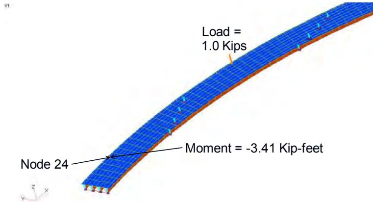
**Figure 4.4.3.2.2-11 Determination of the Influence Surface Ordinate for Vertical Bending Moment at Node 24 for a Load Applied Over G4 in Span 2**
