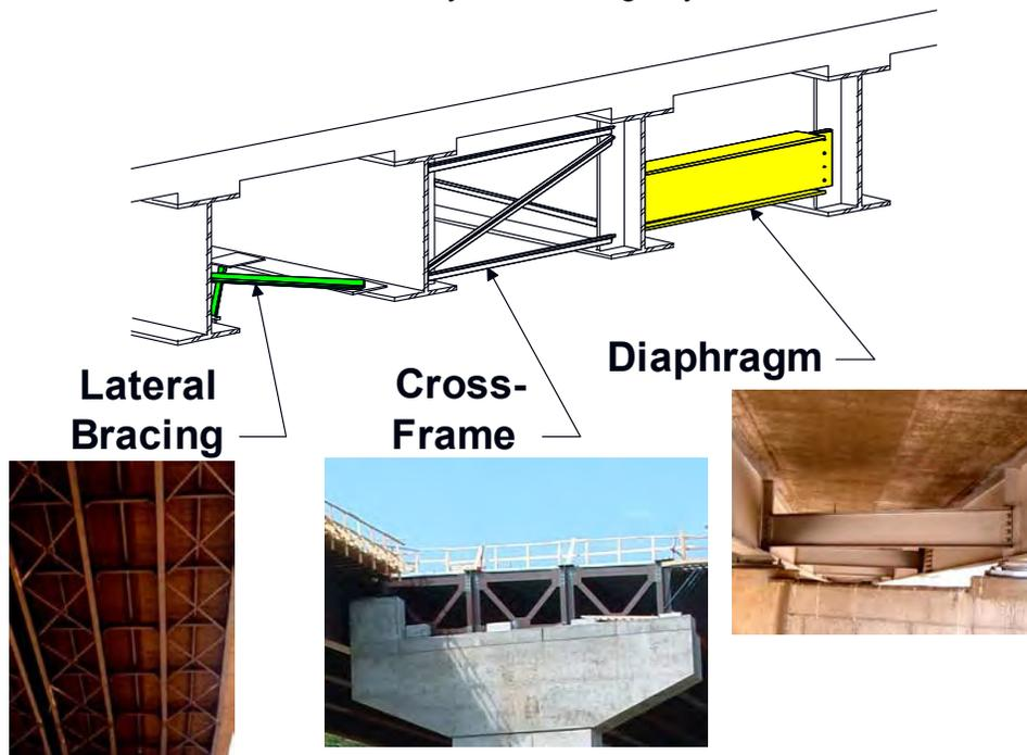
**Figure 6.3.2.9.1-1 Definitions of Cross-Frame, Diaphragm and Lateral Bracing**
