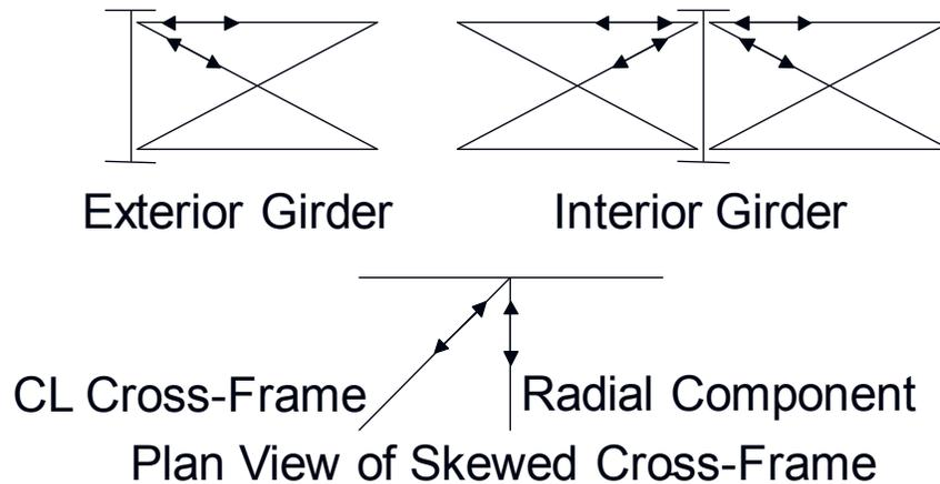
**Figure 6.6.2.3.2.3.2-1 Resolution of the Horizontal Cross-Frame Force Ranges due to the Factored Fatigue Load at the Level of the Top Chord to Determine  $F_{rc}$**
