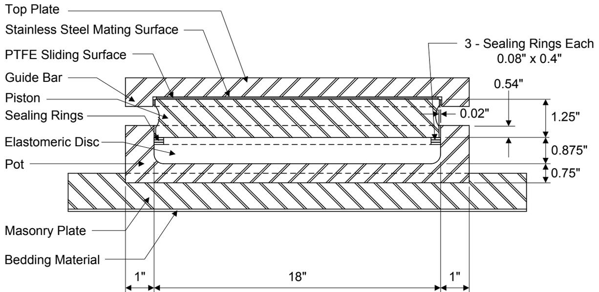
**Figure 8.2.4.2.1.8-1 Final Configuration of Pot Bearing Design Example**
