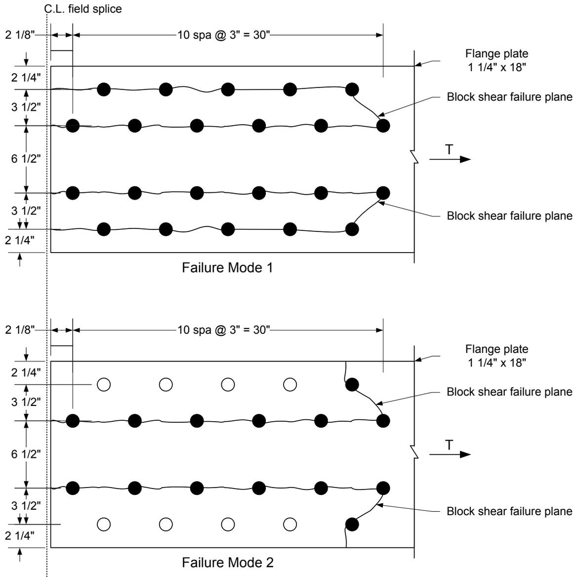
**Figure 6.6.4.2.5.6.1-4 Block Shear Rupture Resistance Example – Smaller Flange at a Bolted Splice**
