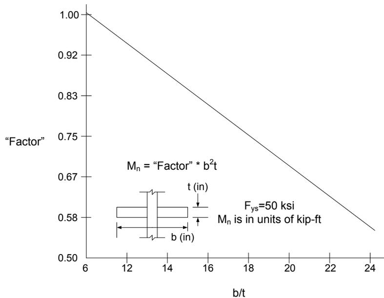
**Figure 6.3.2.9.6.3.1-1 “Factor” for Computing Nominal Local Buckling Resistance of Double-Sided Connection Plates from Equation 6.3.2.9.6.3.1-1 and Equation 6.3.2.9.6.3.1-2**
