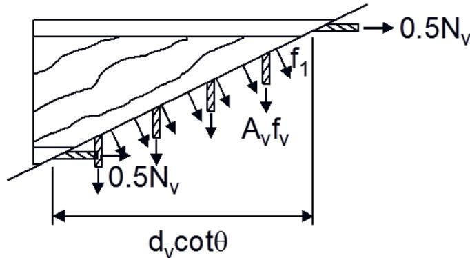
**Figure 5.6.1.1.5-2 Force Transfer in Uncracked Concrete Between Two Cracks (Calculated Average Stresses)**
