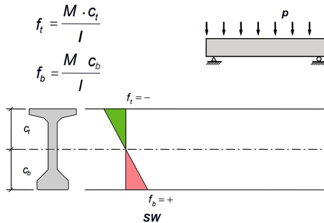
**Figure 5.3.3-1 Self Weight Flexure Stress in Simply-Supported Beam**
