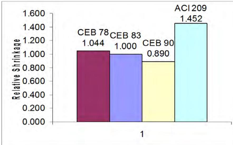
Figure 5.2.1.2.3.2-2 Relative Shrinkage by Different Codes
