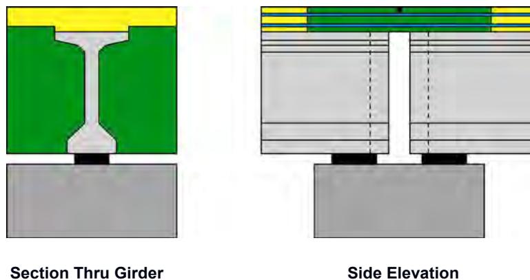
**Figure 5.10.3.2.1-1 Deck Slab (“Poor-Boy”) Continuity Only**
