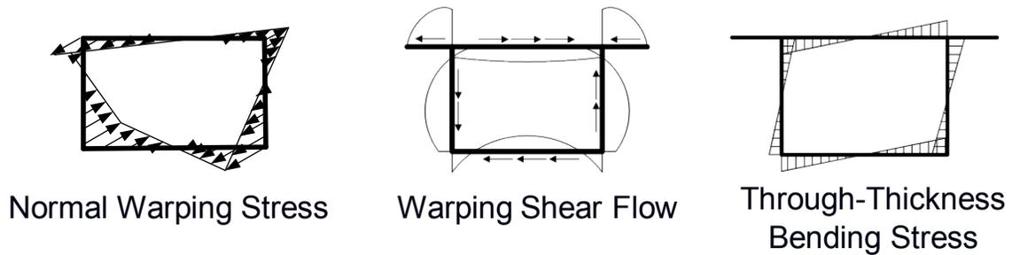
**Figure 6.4.8.3.4-1 Distortion Stresses – Box Section**
