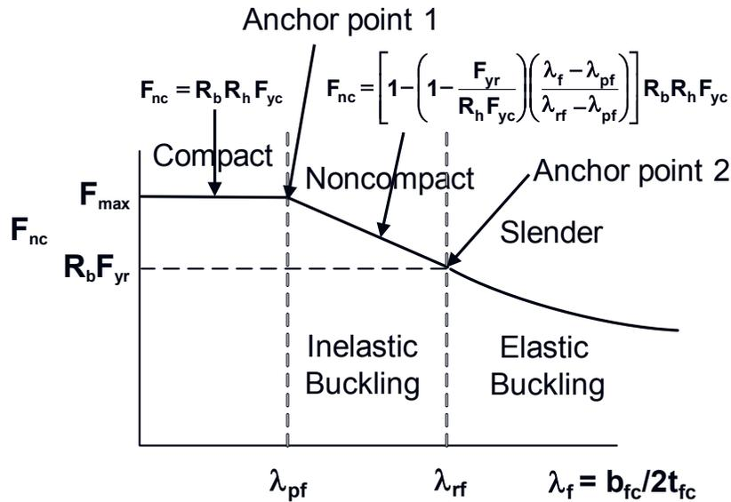
**Figure 6.5.6.2.2.1-2 Local Buckling Resistance,  $F_{nc}$**
