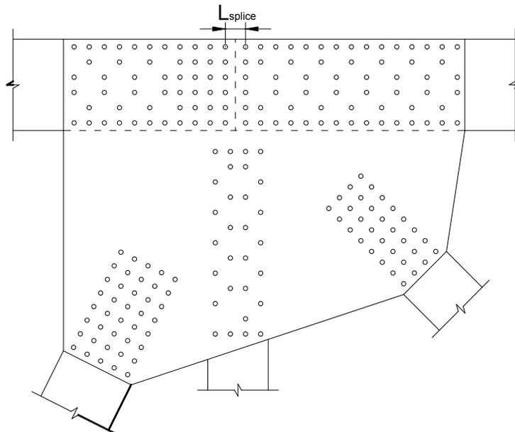
**Figure 6.6.7.5-2 Example Connection Showing Chord Splice Parameter,  $L_{splice}$**
