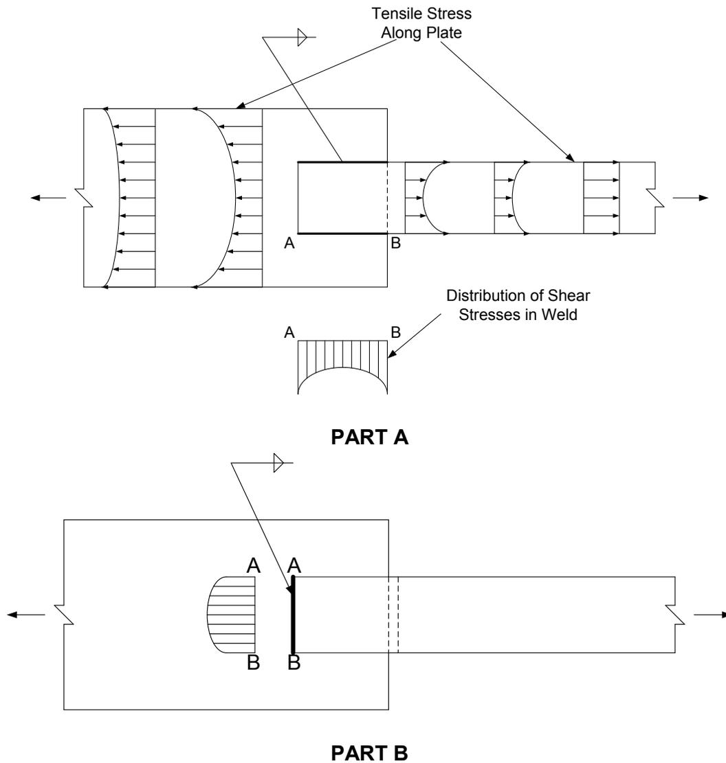
**Figure 6.6.4.3.7.2.1-1 Typical Fillet Weld Shear Stress Distributions in a Lap Joint**
