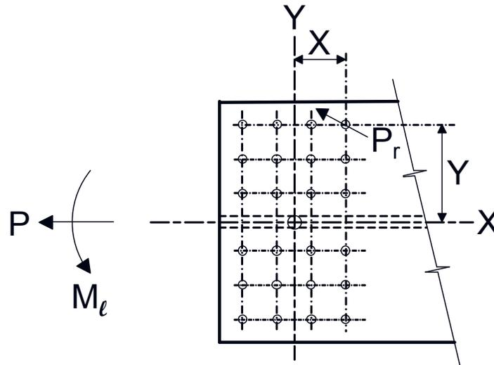
**Figure 6.6.5.2.2.4-4 Resultant Bolt Force,  $P_r$ , and Distances  $X$  and  $Y$**
