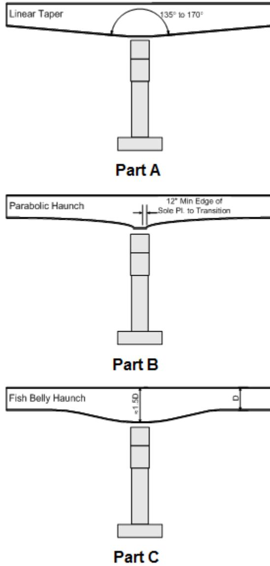
Figure 6.3.3.2.2-1 Variable Web-Depth Member Configurations
