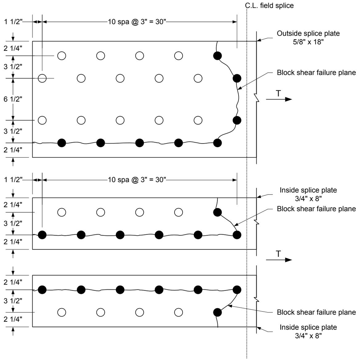
**Figure 6.6.4.2.5.6.1-3 Block Shear Rupture Resistance Example – Bolted Flange Splice Plates**
