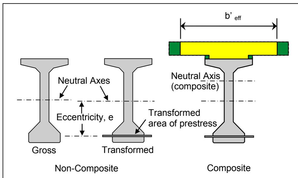
Figure 5.5.3.2.3-1 Transformed Area of Prestress
