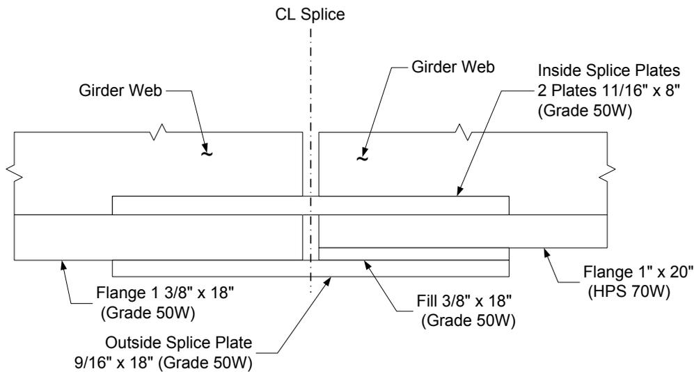
**Figure 6.6.5.2.3.4-1 Example Bottom Flange Splice**
