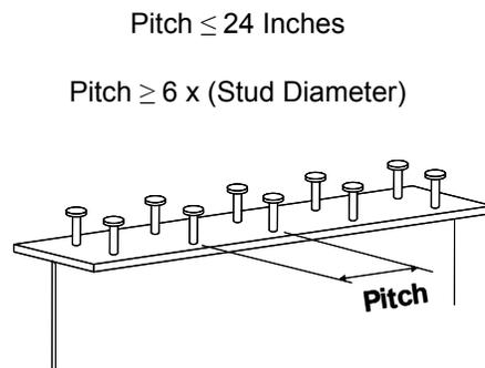
**Figure 6.6.2.2.5-1 Minimum and Maximum Pitch**
