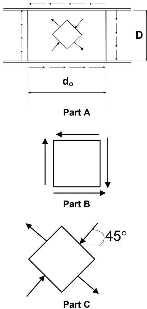
**Figure 6.5.7.2-1 A) Web Panel Subjected to Pure Shear; B) Web Element Subject to Pure Shear; C) Equivalent Principal Stresses**
