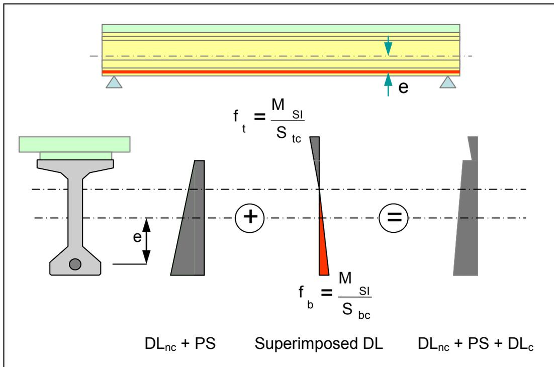
Figure 5.5.3.4.1-4 Application of Superimposed Dead Load on Composite Section
