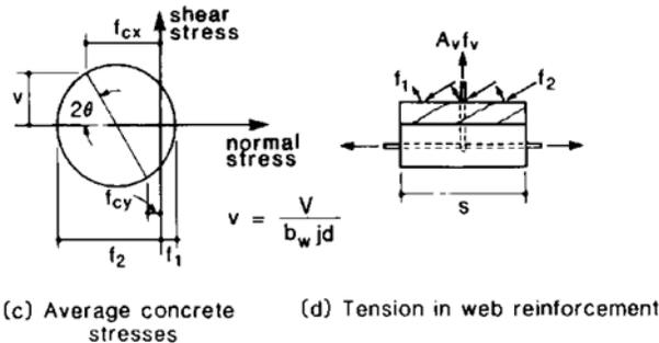
**Figure 5.6.1.1.4-2 Equilibrium Conditions by Modified Compression Field Theory in Diagonally Cracked Beam**
