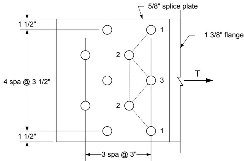
**Figure 6.6.4.2.5.6.1-2 Net Section Fracture Resistance Example – Bolted Flange Splice Plate**
