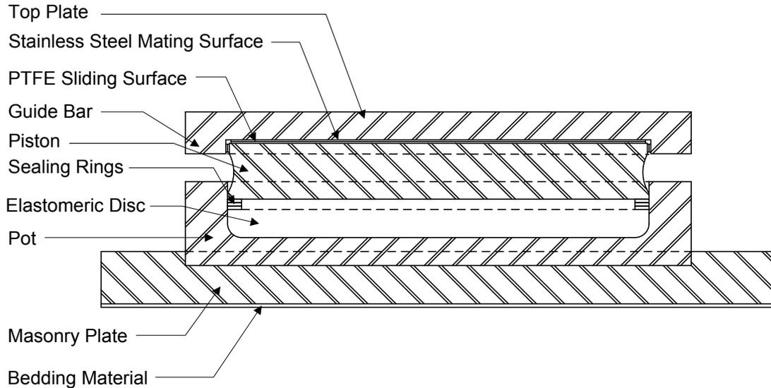
**Figure 8.2.3.3.2-1 Components of a Pot Bearing**
