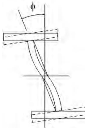
**Figure 6.4.8.2.3-1 Web Distortion in an I-Section**
