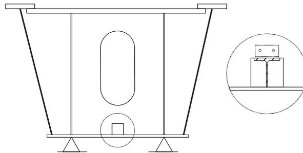
**Figure 6.5.6.2.4.2.1-2 Suggested Longitudinal Flange Stiffener Detail at an Internal Diaphragm**
