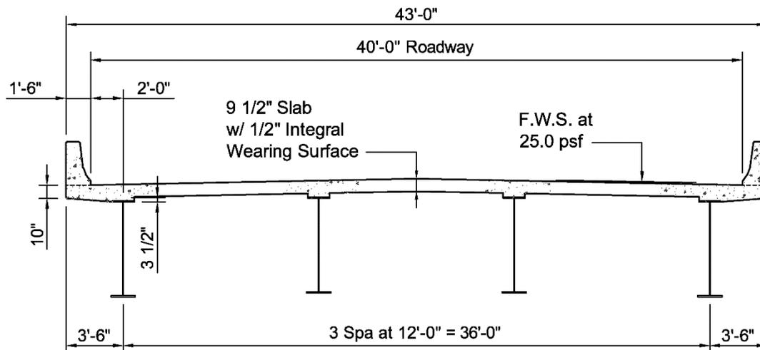
**Figure 4.4.2.2.2-1 Example Steel I-Girder Bridge Cross-Section**
