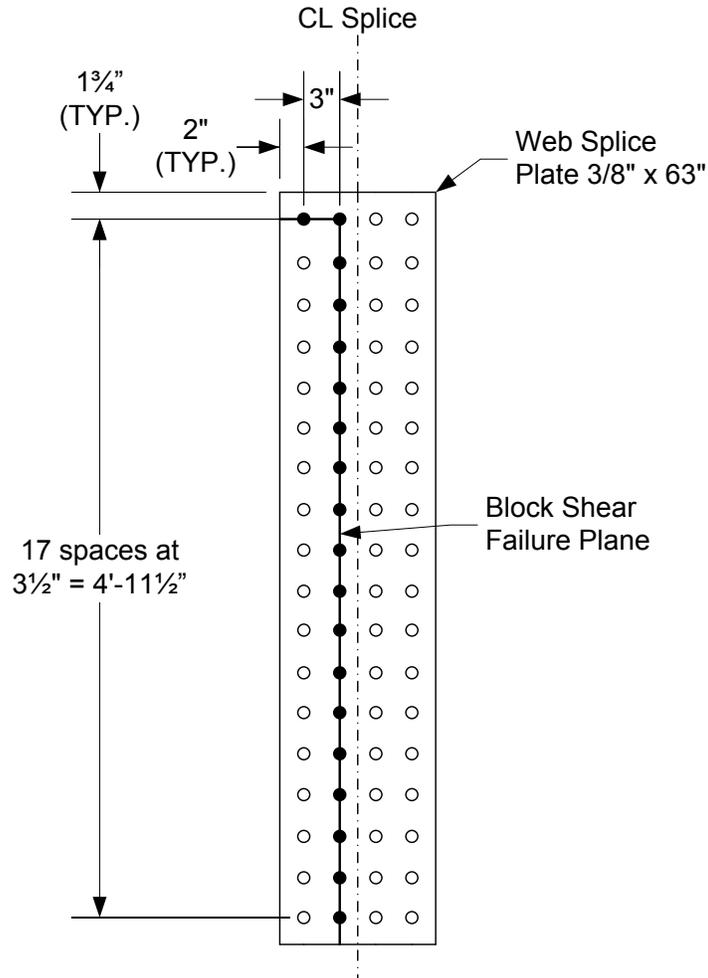
**Figure 6.6.5.2.3.4-8 Web Splice Plate – Assumed Block Shear Failure Plane in the Web Splice Plates**
