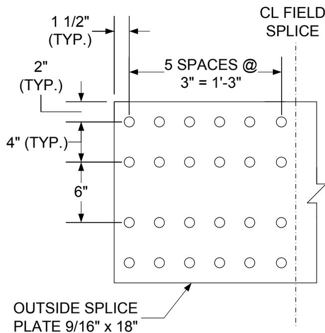
**Figure 6.6.5.2.3.4-2 Outside Bottom Flange Splice Plate – Plan View**
