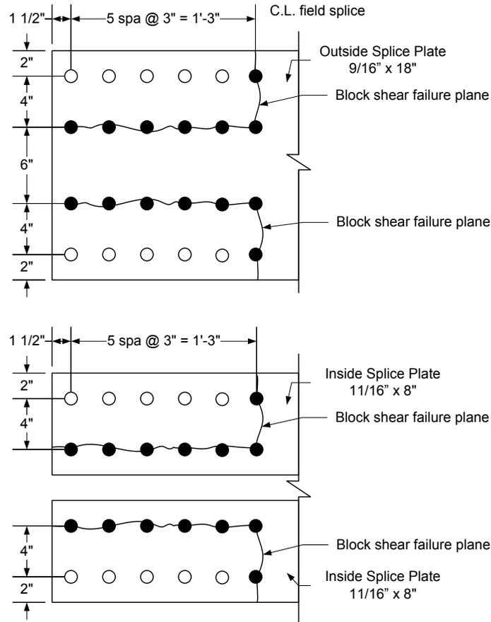
**Figure 6.6.5.2.3.4-3 Bottom Flange Splice – Assumed Block Shear Failure Planes in the Splice Plates**
