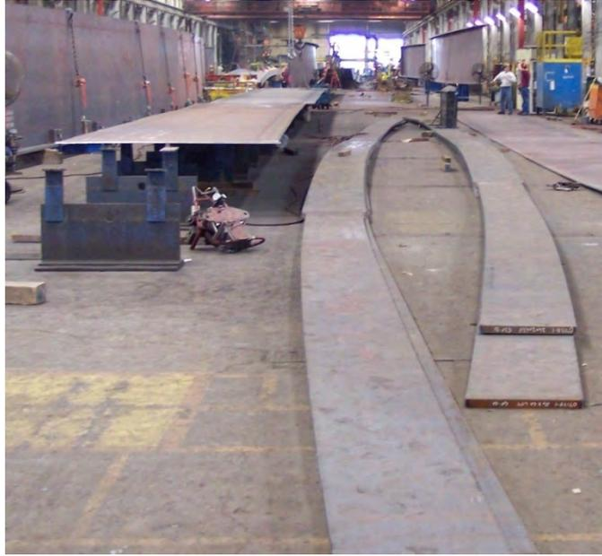
**Figure 6.4.9.4-3 Cut Curved I-Girder Flanges in the Fabrication Shop**
