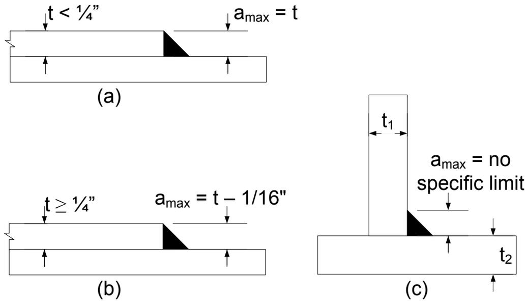
**Figure 6.6.4.3.3.3-1 Maximum Size Requirements for Fillet Welds**
