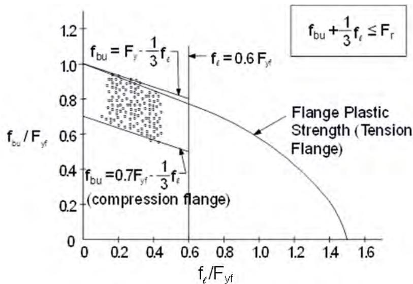
Figure 6.5.2.1.2-2 Normalized Plot of  $f_{bu}$  vs.  $f_\ell$
