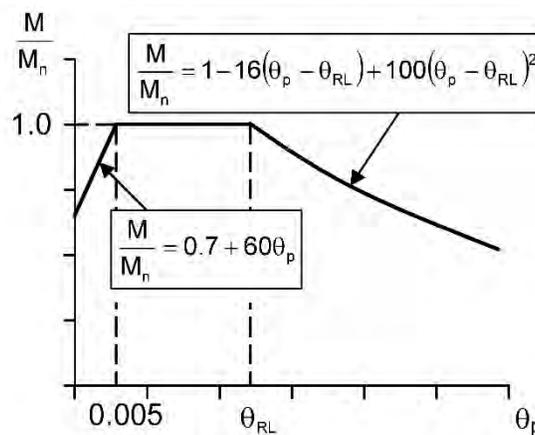
**Figure 6.5.6.6.4-1 Nominal Moment-Rotation Curve for Interior-Pier Sections Satisfying *AASHTO LRFD* Article B6.2**
