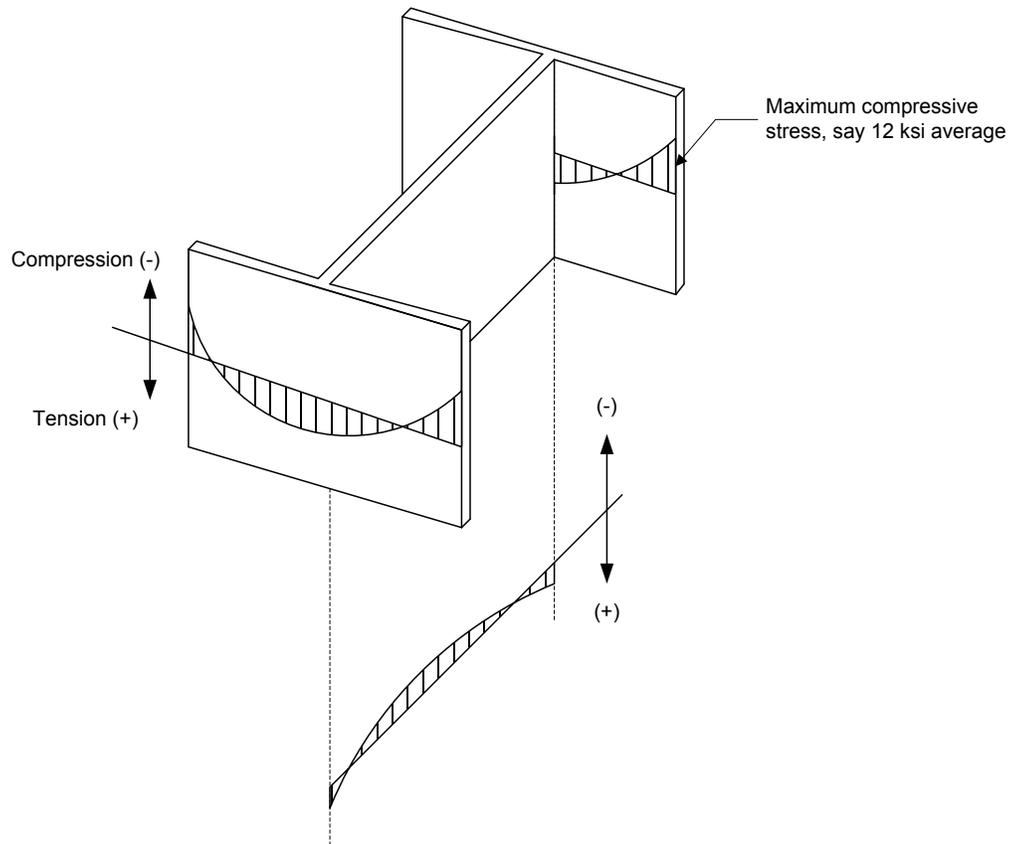
**Figure 6.6.3.4.2.3.2-1 Typical Residual Stress Distribution for Rolled Shapes**
