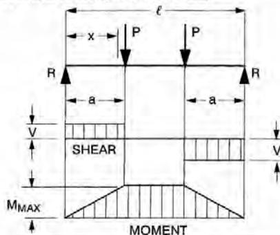
**Figure 5.5.8.2-3 Deflection of Simply-Supported Beam under External Load**
