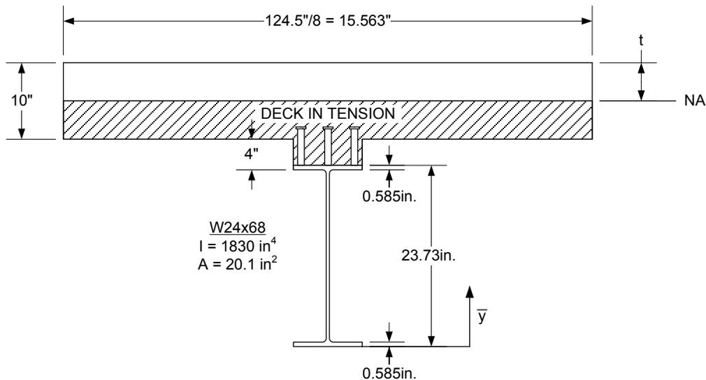
**Figure 6.4.2.3.2.1-1 Composite Rolled-Beam Substringer Subject to Positive Flexure**
