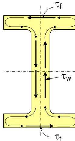
**Figure 6.4.8.2.1-2 Torsion and Torsional Shear Stress on an I-Girder**
