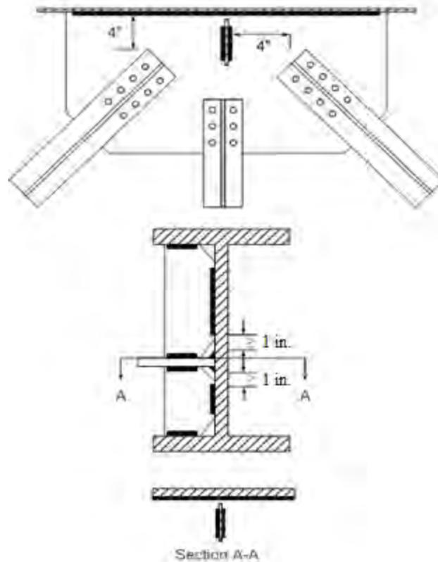
**Figure 6.3.2.10.4-3 Recommended Lateral Connection Plate Detail for Plate Attached to the Girder Web – Plate on Same Side of Web as Transverse Stiffener**
