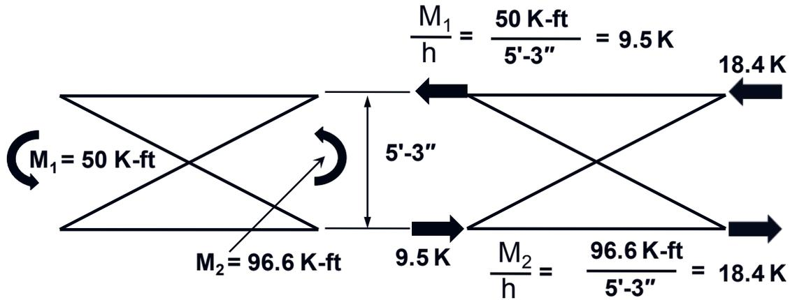
**Figure 4.5.3.2.2.5.3-11 Resolution of End Moments into Force Couples for the Example Cross-Frame**
