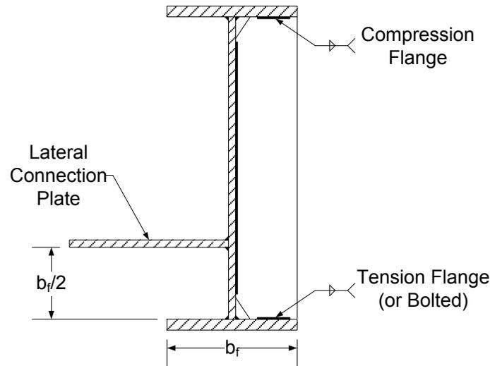
**Figure 6.3.2.10.4-2 Recommended Lateral Connection Plate Detail for Plate Attached to the Girder Web – Plate Opposite Transverse Stiffener**
