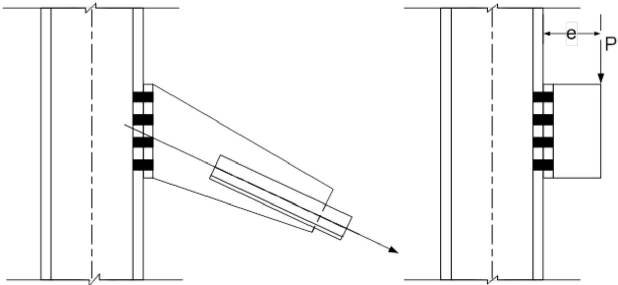
**Figure 6.6.4.2.5.5-1 Bolted Connections Subject to Combined Tension and Shear**
