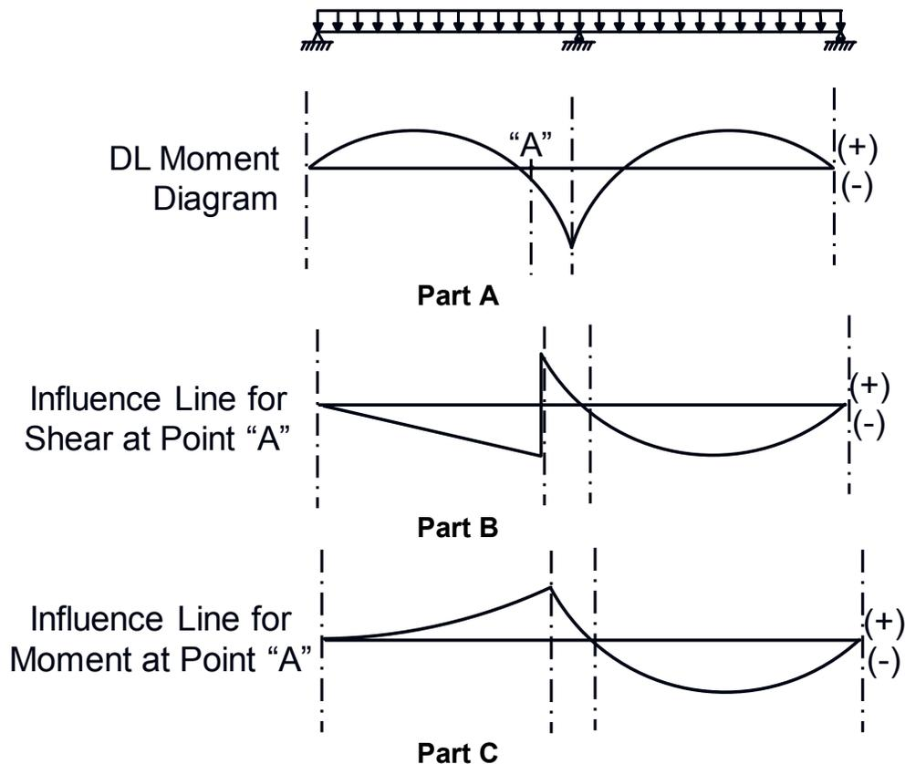
**Figure 6.4.2.1-2 Positive Live Load Moment Resulting from the Loading Causing the Maximum Shear Range in a Dead Load Negative Moment Region**
