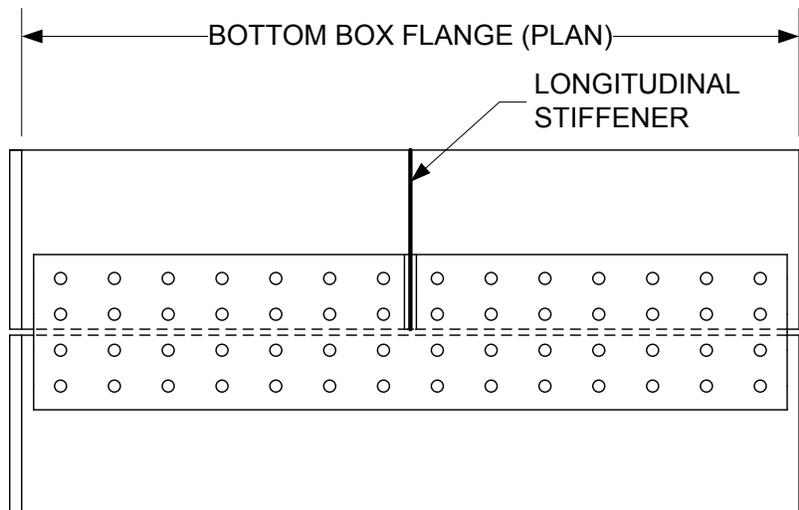
**Figure 6.5.6.2.4.2.1-3 Suggested Box-Flange Bolted Splice Detail at Flange Stiffener Termination**
