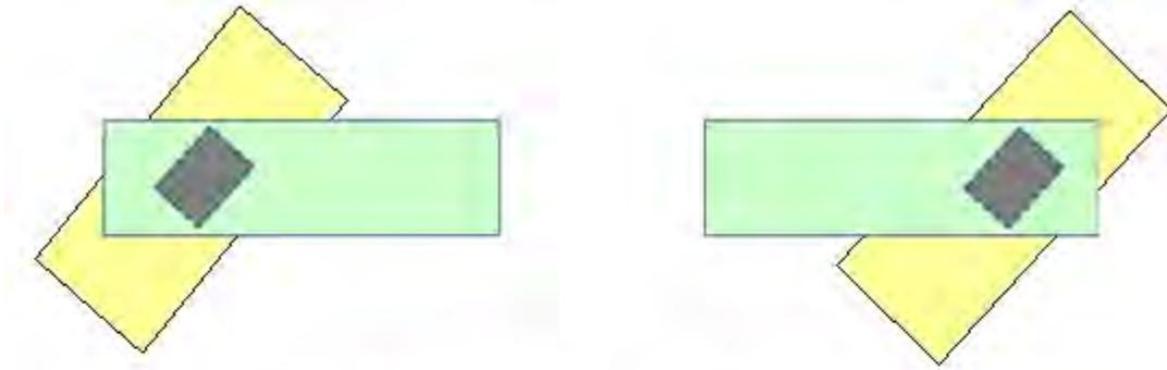
Figure 5.4.1-2(a) Bearings oriented parallel with pier caps.
