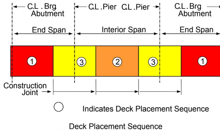
**Figure 6.5.3.3.4-2 Sample Deck Placement Sequence**
