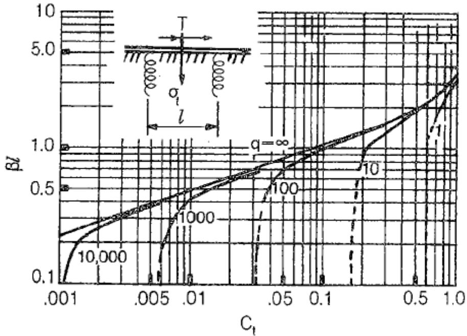
Figure 6.5.5.2.3.2-6 BEF Factor,  $C_t$ , for Distortional Transverse Bending Stress at Midpanel due to a Concentrated Torque,  $T$ , at Midpanel
