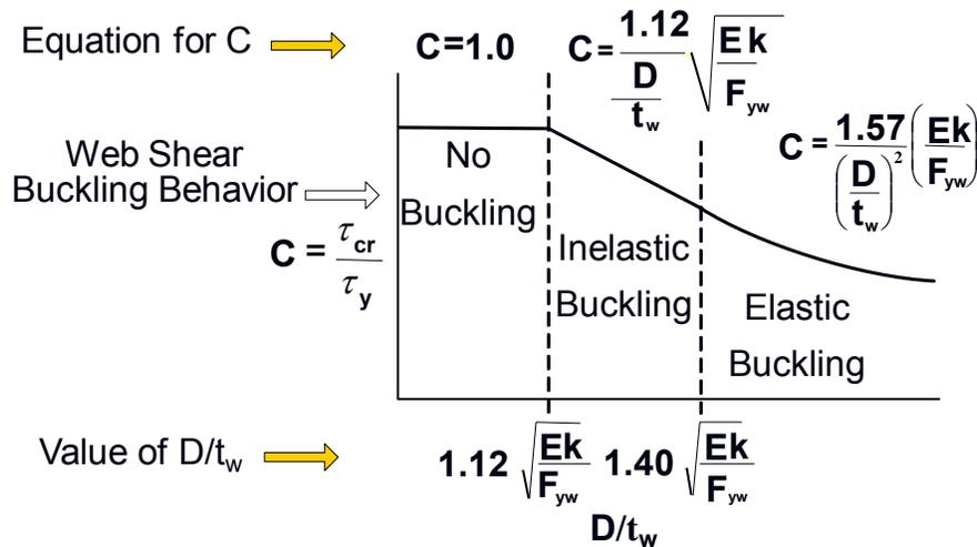
**Figure 6.5.7.2-2 Web Shear Buckling Resistance – the Constant C**
