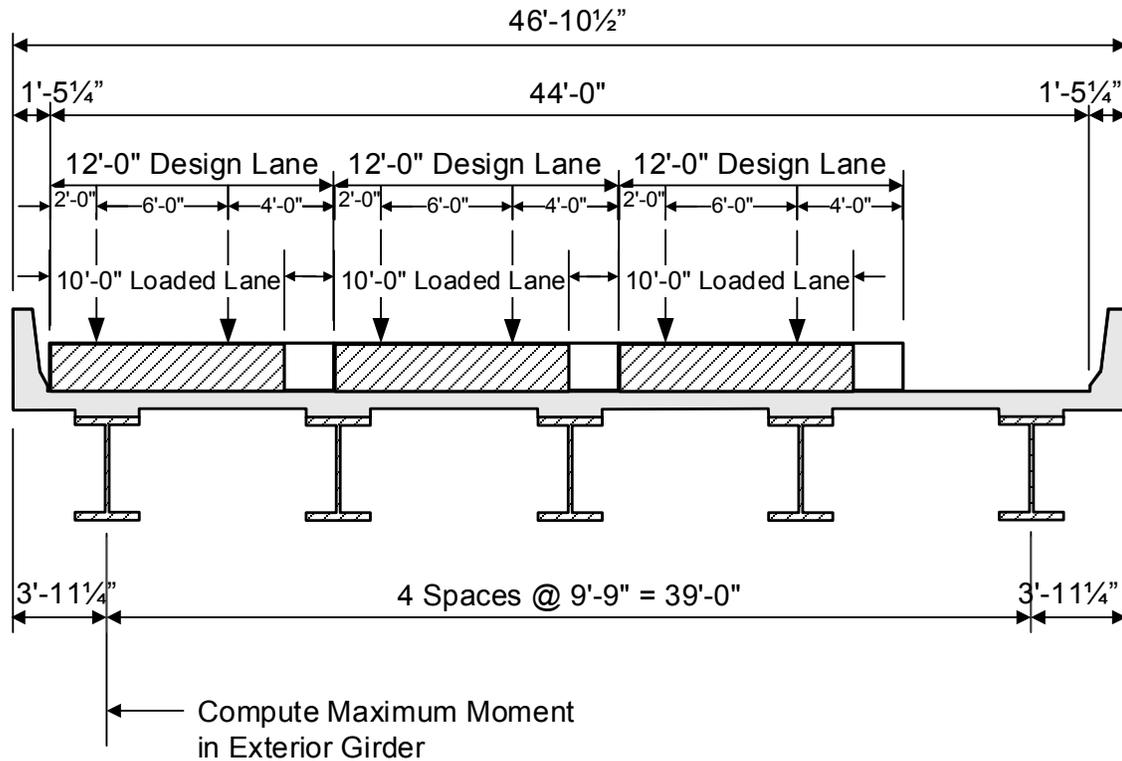
**Figure 3.4.1.1-2 Position of Loaded Width within Design Lanes**
