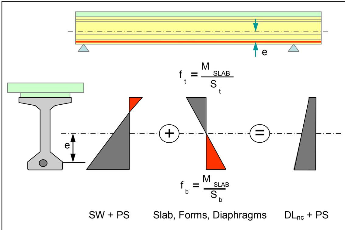
Figure 5.5.3.4.1-3 Loads of Slab, Forms and Diaphragms Applied to Non-Composite Section
