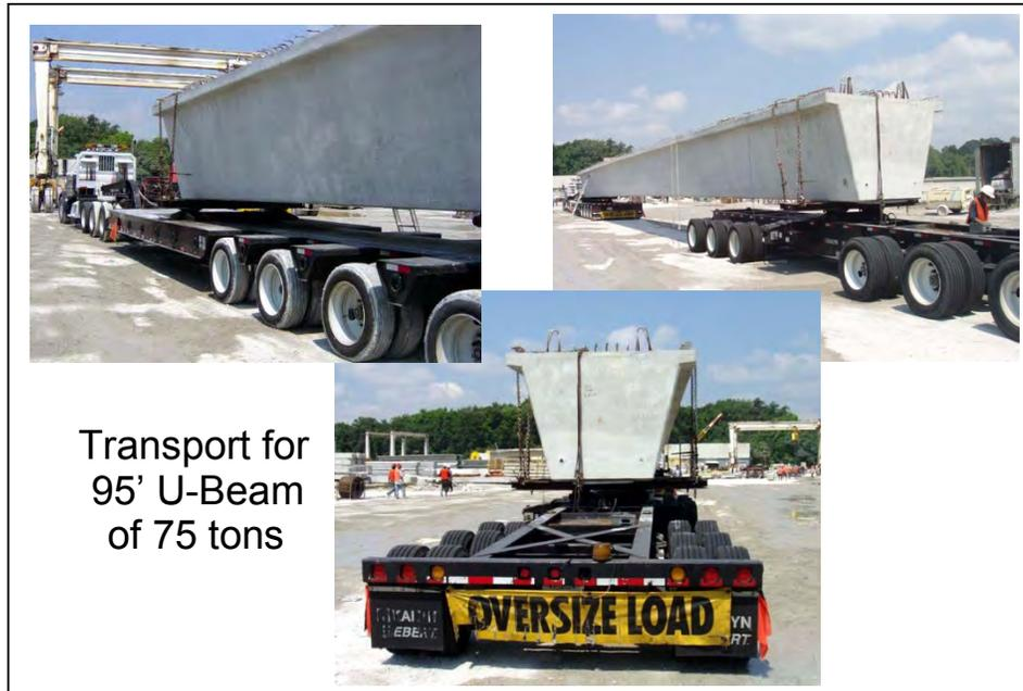
**Figure 5.4.1-3 Roadway Transport of Prestressed Concrete U-beams**
