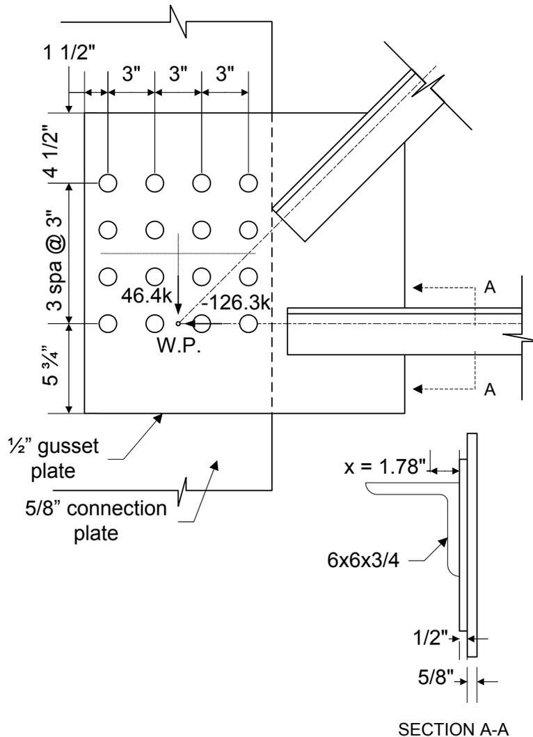
**Figure 6.6.4.2.6-4 Example Gusset-Plate Configuration for Bolted Bracing Member Connection – Option 1**
