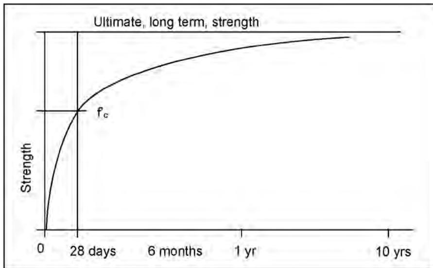
Figure 5.2.1.1.1-1 Gain of Concrete Strength with Time
