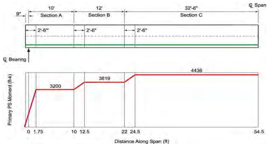
**Figure 5.10.3.3.2.1-6 Prestress Moment for Simply-Supported Girder**
