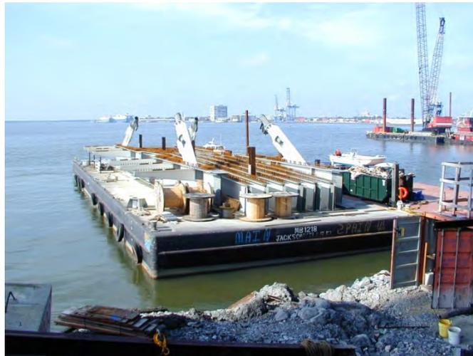
**Figure 6.3.2.4.2.3-1 Steel-Girder Sections Loaded on a Barge**
