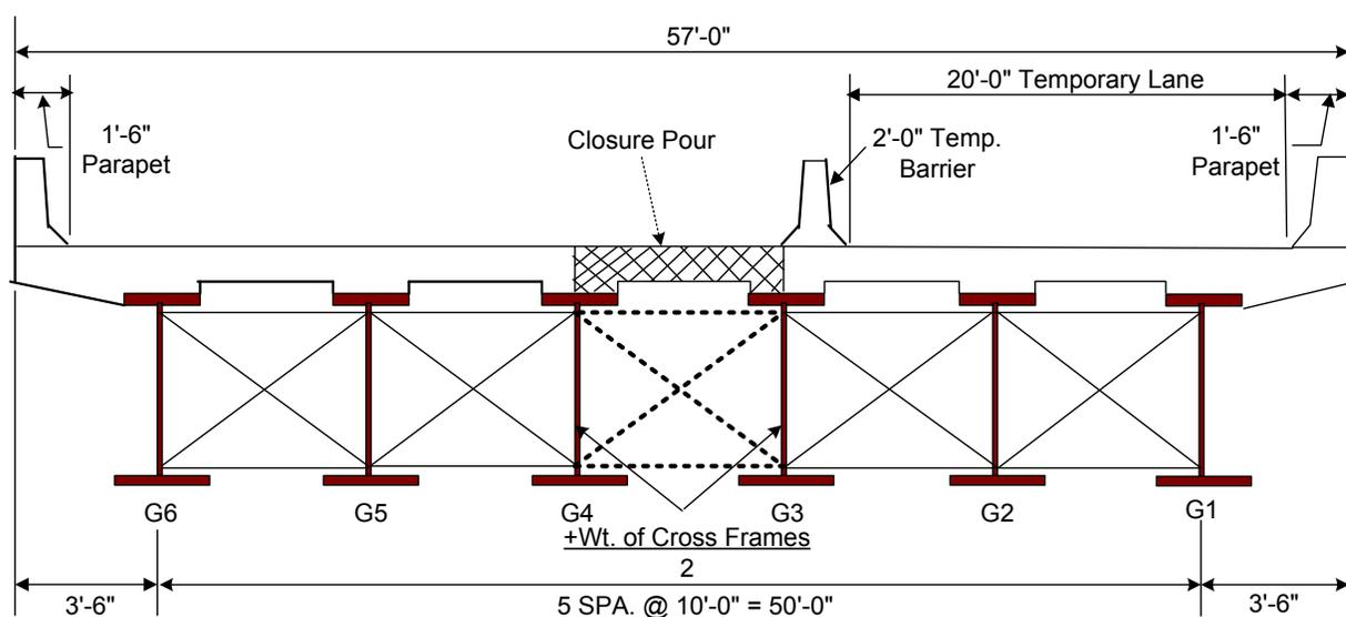
Figure 6.3.2.5.4.2-1 Phased Construction with a Closure Pour
