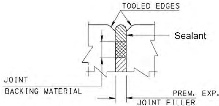
**Figure 8.3.2.2-1 Pourable Joint Sealer**
