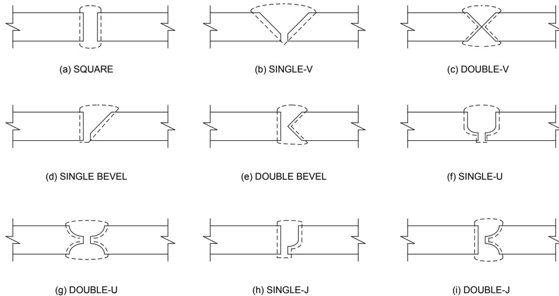
**Figure 6.6.4.3.3.2.2-1 Types of Groove Welds**
