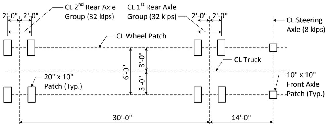
**Figure 3.4.4.4-1 Refined Design Truck Footprint for Fatigue Design of Orthotropic Decks**
