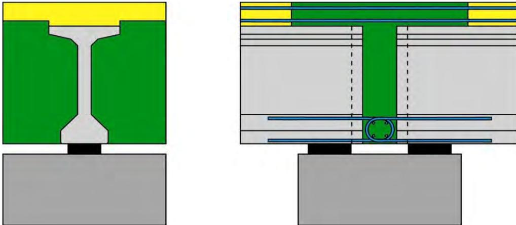
Figure 5.10.3.3.5-1 Bottom Reinforcement in Closure Joint at Pier
