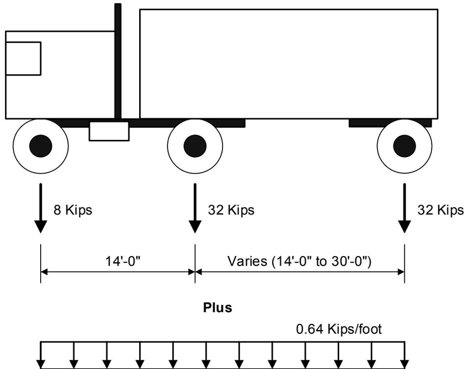
**Figure 3.4.3.1-2 Effect of Design Truck Plus Design Lane Load**
