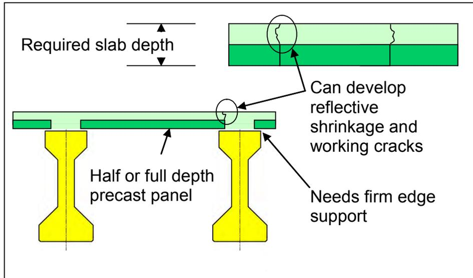
**Figure 2.3.3.4-3 Precast Concrete Deck Slab Panels**
