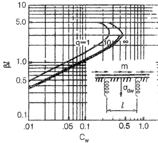
Figure 6.5.5.2.3.2-2 BEF Factor,  $C_w$ , for Distortional Longitudinal Warping Stress at Midpanel due to a Uniform Torque,  $m$
