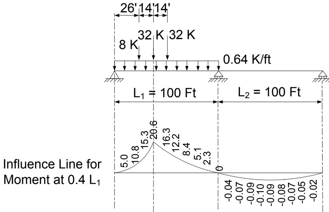
**Figure 4.4.3.1-6 HL-93 Live Load Applied to Influence Line for Vertical Bending Moment at  $0.4L_1$  in the Example Two-Span Bridge**
