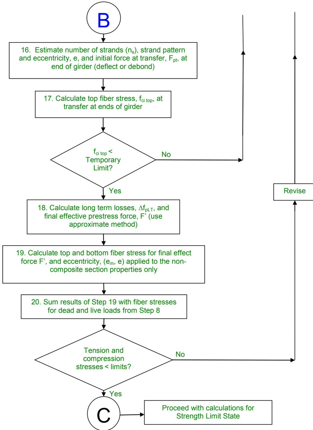
Figure 5.5.3.4.3-5 Flowchart for Determination of Prestress Force and Strand Pattern, Part (c)
