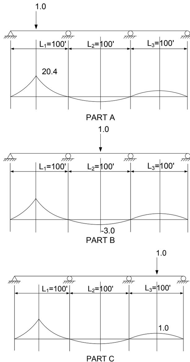
**Figure 4.4.3.1-2 Development of Influence Line Ordinates for Vertical Bending Moment at  $0.4L_1$  in a Three-Span Continuous Beam by Application of Unit Loads**
