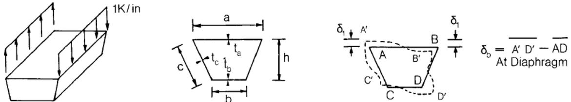
**Figure 6.5.5.2.2.3.2-1 Box Under Uniform Torsional Loading**
