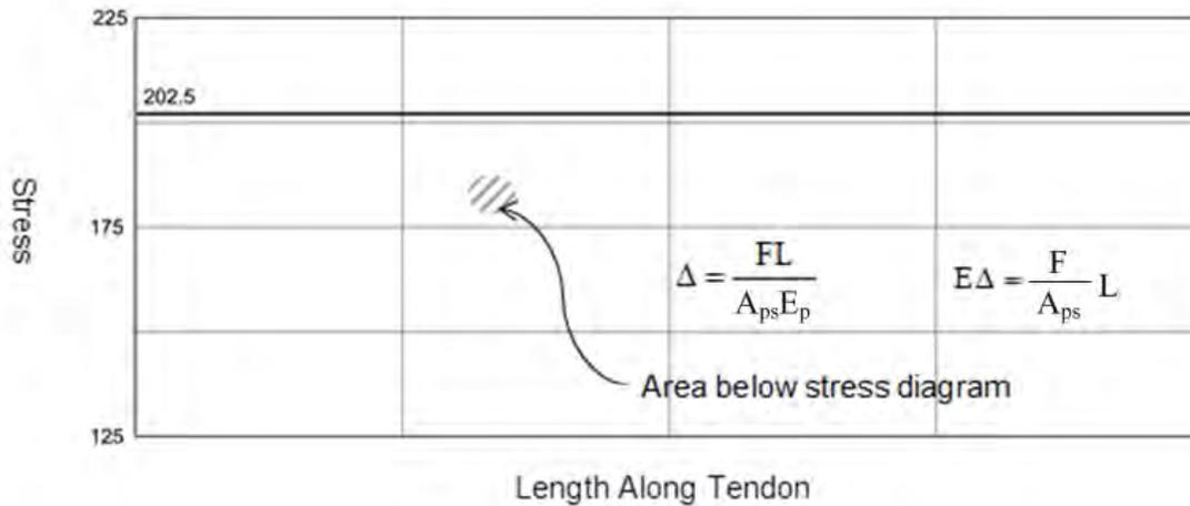
**Figure 5.7.3.3.1.4-1 Stress Diagram of Straight Tendon**
