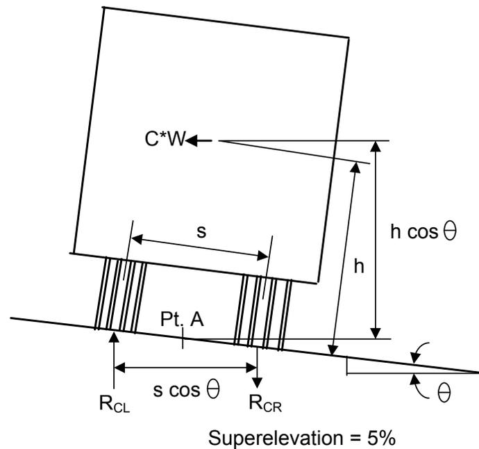
**Figure 3.4.9.1-1 Vehicular Centrifugal Force Wheel-Load Reactions**
