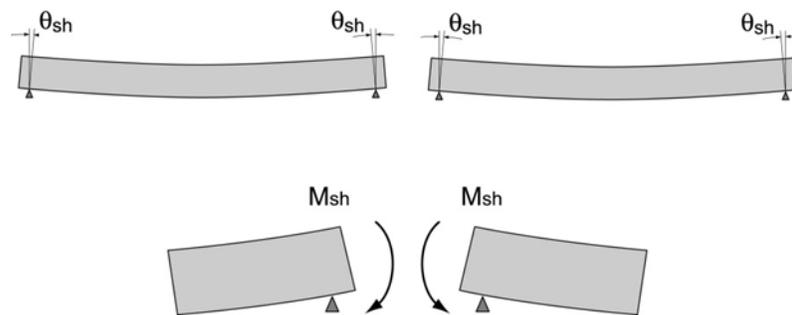
**Figure 5.10.3.2.3.5-1 Differential Shrinkage**
