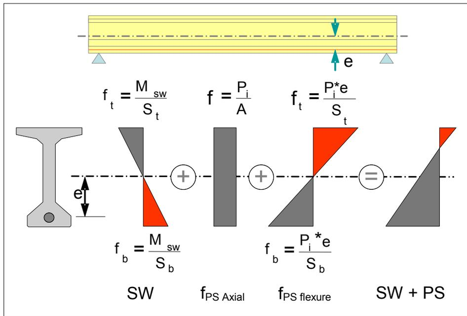
Figure 5.5.3.4.5-1 Girder Self-Weight and Prestress Only, at Transfer
