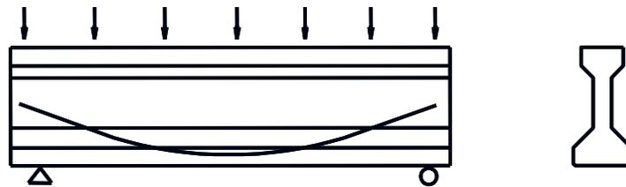
**Figure 5.6.4.2-1 Noncomposite Beam Subjected to Beam Self-Weight, Pretensioning Effects and Slab Dead Weight**
