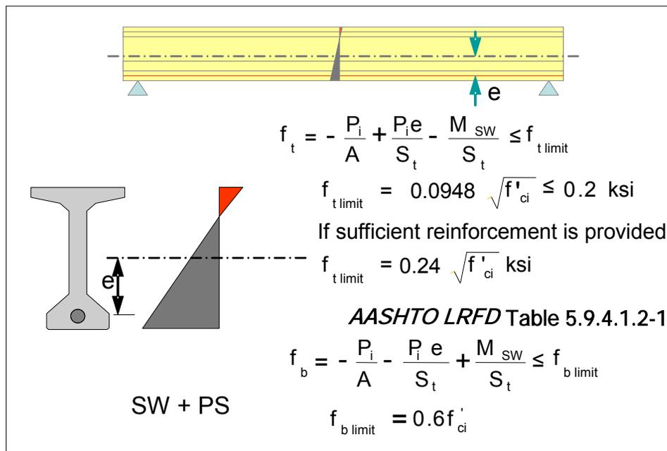
Figure 5.5.3.4.5-2 Stress Limits at Transfer
