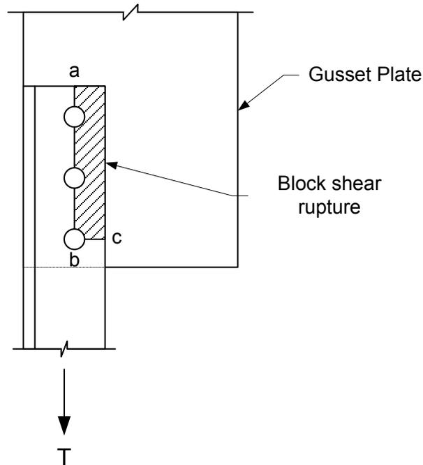
**Figure 6.6.3.3.2.5-1 Tension Failure of a Bolted Single Angle Member by Block Shear Rupture**
