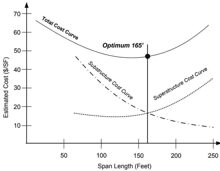
**Figure 6.3.2.3.3-1 Sample Cost Curves for Span Optimization**
