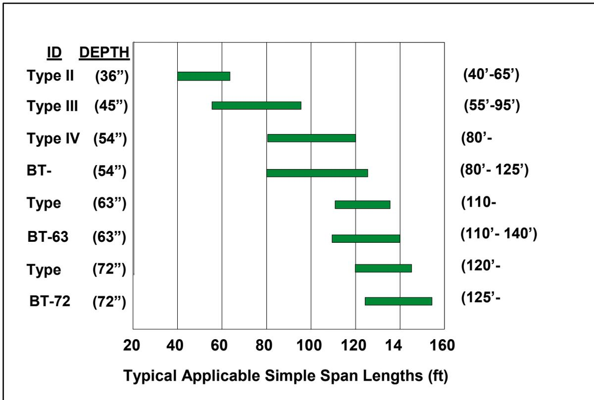
**Figure 5.4.3-1 Simple-Span Precast Girder Types and Typical Span Ranges (AASHTO I-Girders; PCI Bulb-Tees)**
