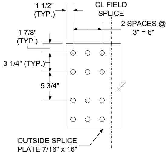
**Figure 6.6.5.2.3.4-6 Outside Top Flange Splice Plate – Plan View**
