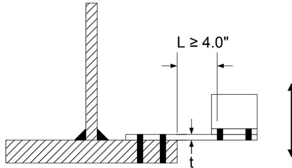
**Figure 6.3.2.10.4-1 Lateral Connection Plate Bolted to Flange – Minimum Recommended Gap to Reduce Vibration Stresses**
