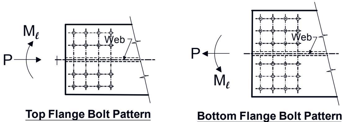
**Figure 6.6.5.2.4-1 Top and Bottom Flange Splices Subject to Flange Lateral Bending**
