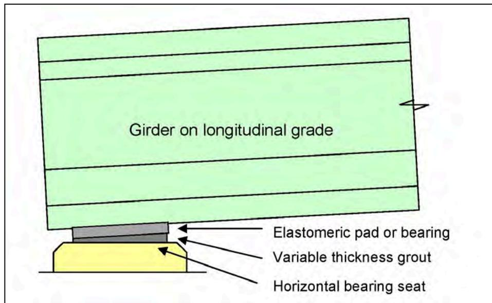
**Figure 2.3.3.2-1 Elastomeric Bearing Detail for Longitudinal Gradient**
