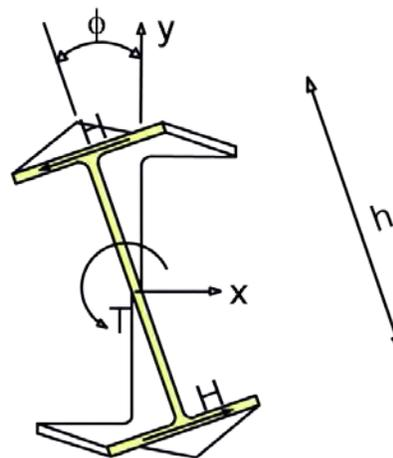
**Figure 6.4.9.4-1 I-Girder Subjected to Torsion**
