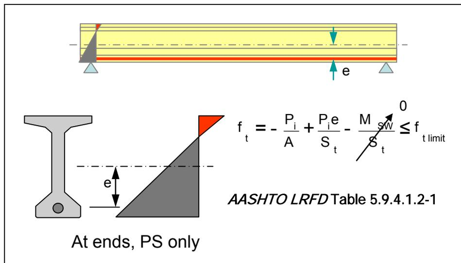
Figure 5.5.3.4.5-3 End Conditions at Transfer
