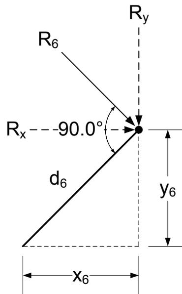
**Figure 6.6.4.2.6-3 Horizontal and Vertical Components of Shear Force,  $R$**
