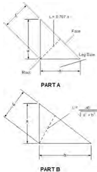
**Figure 6.6.4.3.3.2-1 Effective Throat Dimensions for Fillet Welds**
