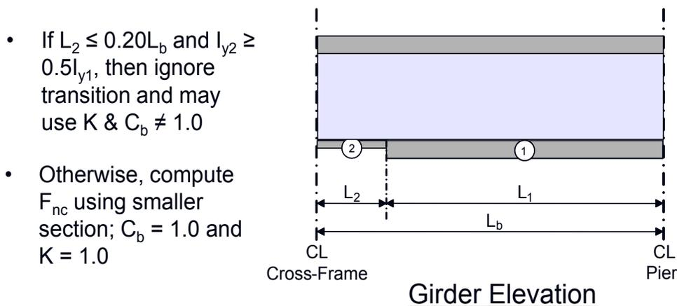
**Figure 6.5.6.2.2.2-5 Unbraced Length with a Single Section Transition**
