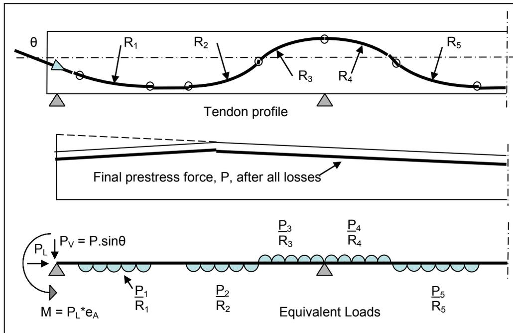
Figure 5.10.4.2.3-1 Equivalent Loads Represent Post-tensioning Effects
