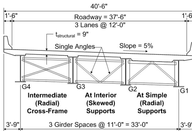
**Figure 4.4.3.2.2-2 Example I-Girder Bridge Cross-Section**
