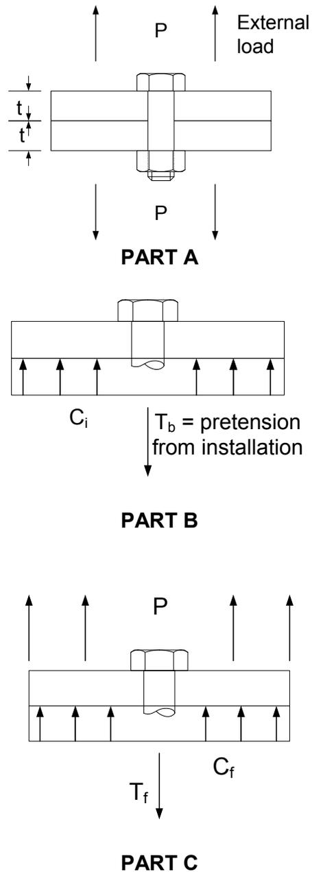
**Figure 6.6.4.2.5.4.1-2 Pretensioning Effect on a Bolted Joint**
