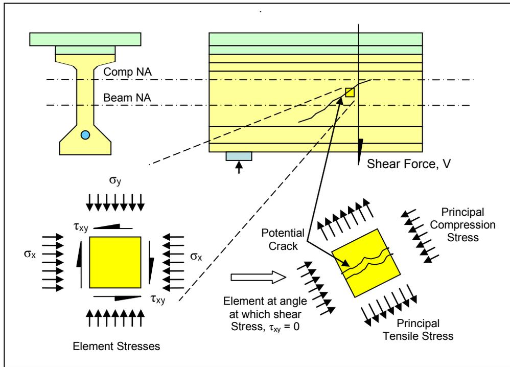
Figure 5.6.2-1 State of Stress in Web Element near the End of a Beam
