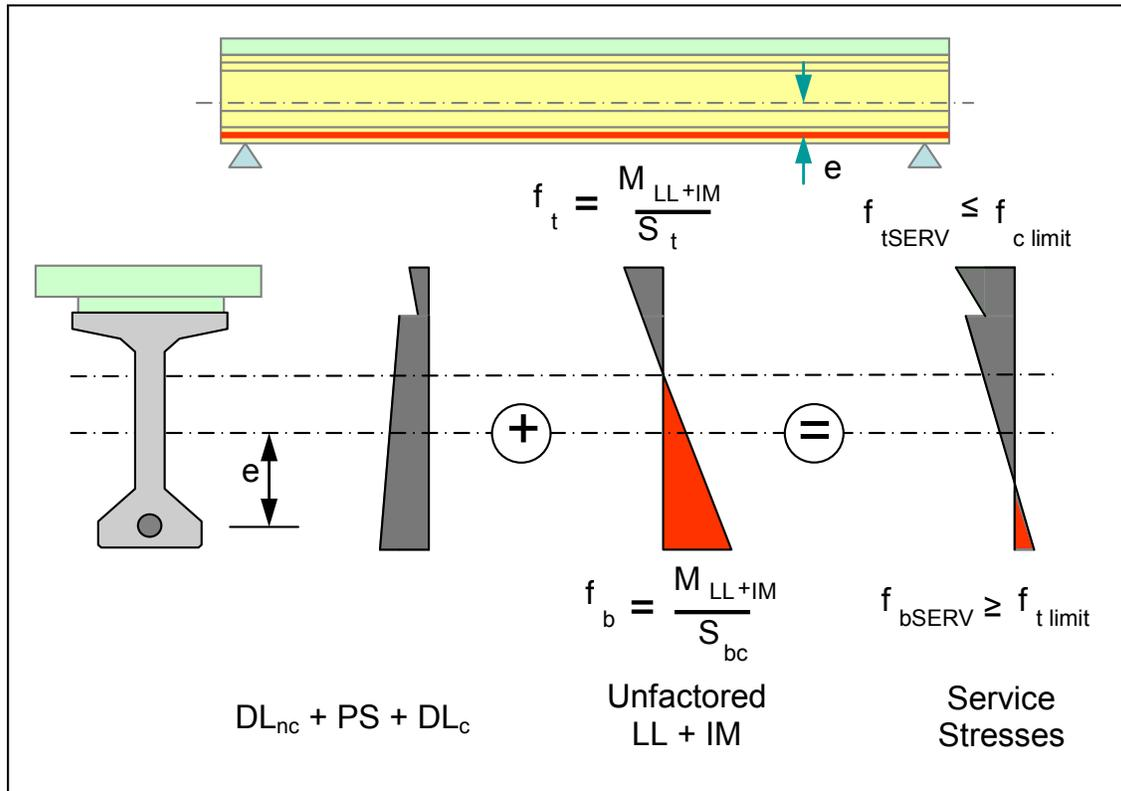
**Figure 5.5.3.4.1-5 Application of Live Load on Composite Section**
