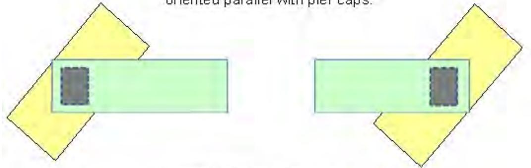
Figure 5.4.1-2(b) Bearings oriented normal to girders.
