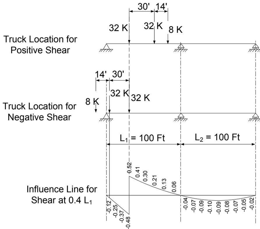
**Figure 4.4.3.1-8 Fatigue Live Load Applied to Influence Line for Shear at  $0.4L_1$  in the Example Two-Span Bridge**
