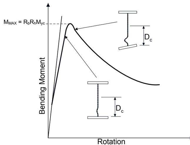
**Figure 6.5.6.2.2.1.4-1 Moment versus Curvature for a Homogeneous Slender Web Section**
