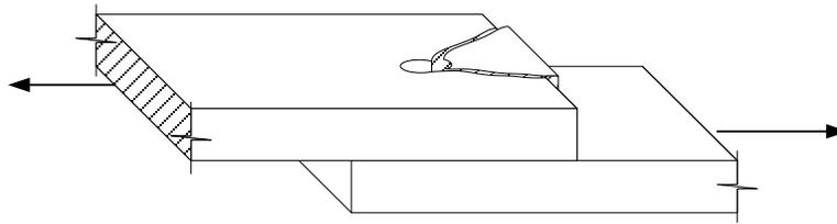
**Figure 6.6.4.2.5.6.2-1 Shear Rupture Failure of a Connected Element**
