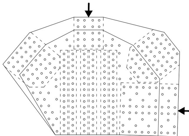
**Figure 6.6.7.2-3 Example Showing Truss Vertical and Chord Members in Compression that Do Not Require a Partial Shear Plane Check**
