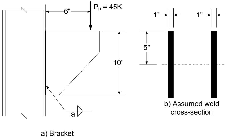
**Figure 6.6.4.3.7.2.3-5 Eccentrically Loaded Fillet-Welded Bracket Example 2**
