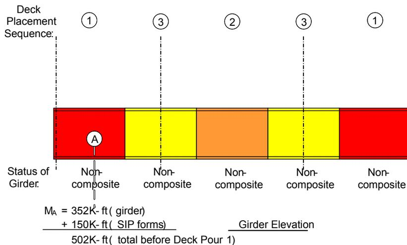
**Figure 6.5.3.3.4-3 Example Girder Elevation View**
