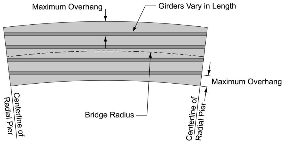
**Figure 5.4.1-1 Typical Span of a Curved Girder Bridge**
