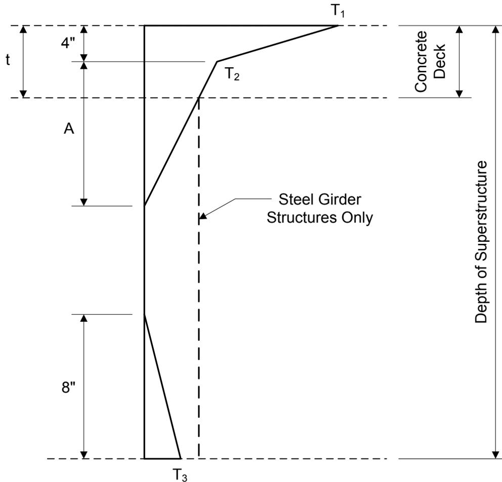
**Figure 3.7.3-2 Positive Vertical Temperature Gradient**
