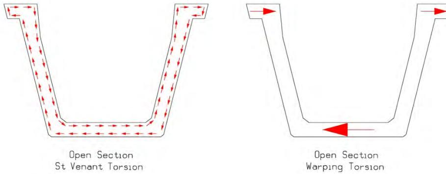
**Figure 5.6.3-1 Comparison of St. Venant Torsion and Warping Torsion in an Open Cross Section**
