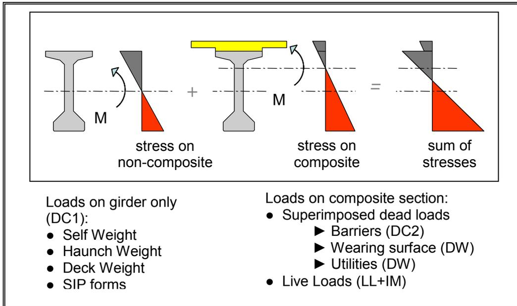
**Figure 5.5.3.1-1 Loads and Stresses in Composite Construction**
