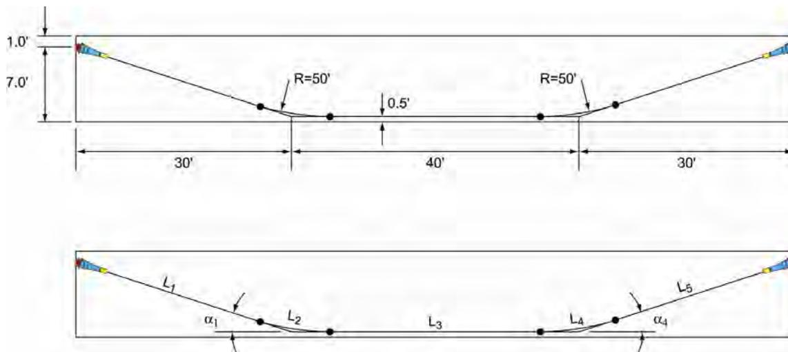
**Figure 5.7.3.3.1.4-2 Example of Deviating Post-Tensioning Tendon**
