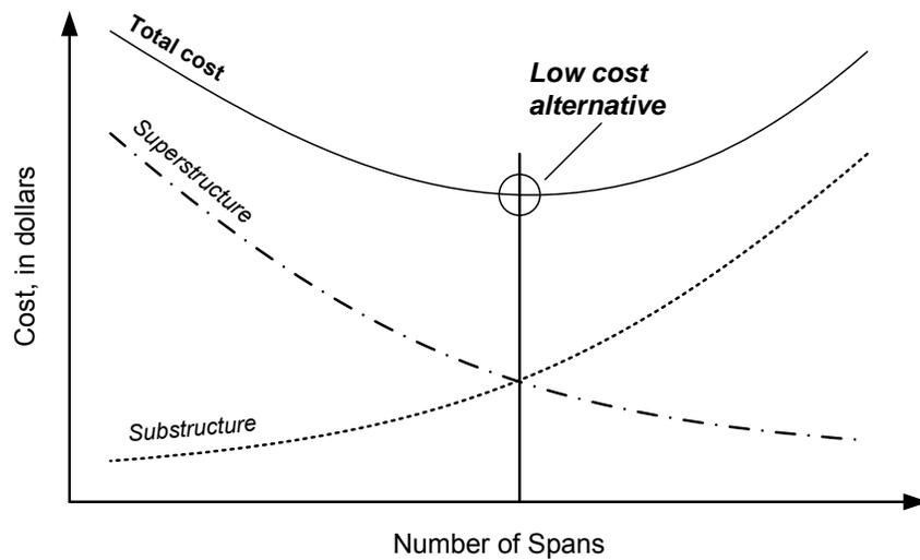
**Figure 2.3.4.2-1 Number of Spans versus Cost**
