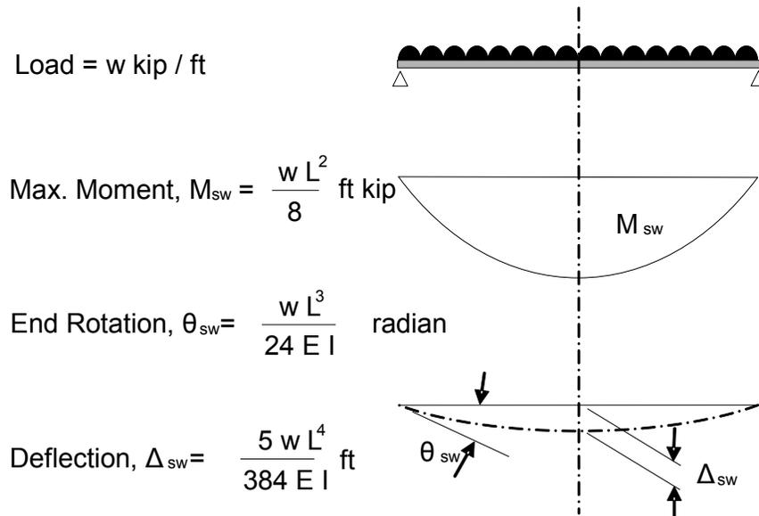
**Figure 5.10.3.3.2.1-2 Simply-Supported Span under Uniform Load**
