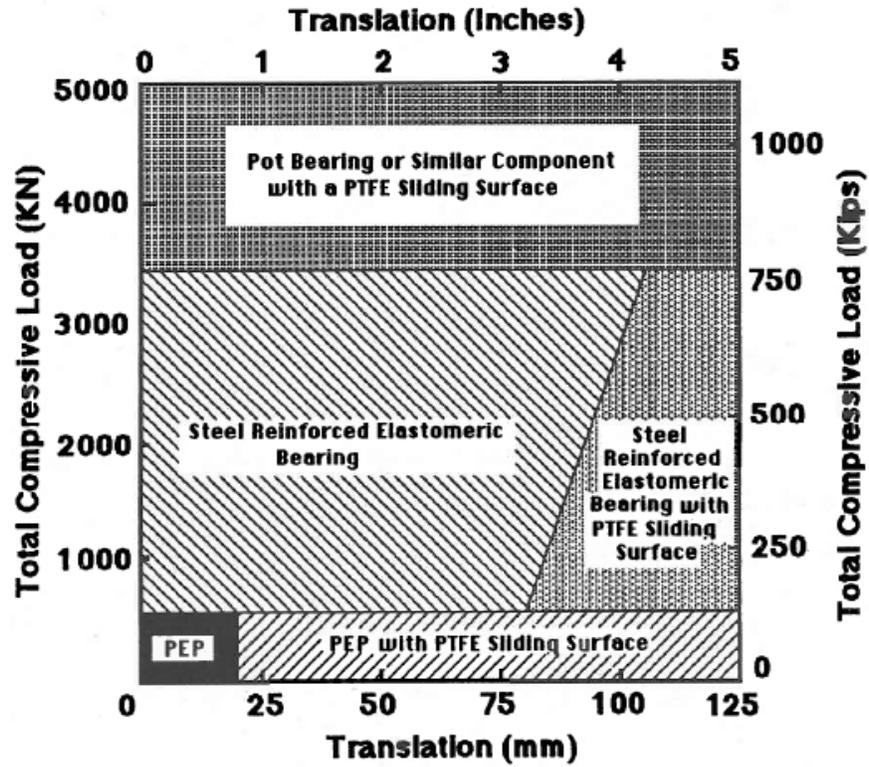
Figure 8.2.3.6-2 Preliminary Bearing Selection Diagram for Moderate Design Rotation ( $\text{Rotation} \leq 0.015$  Radians)
