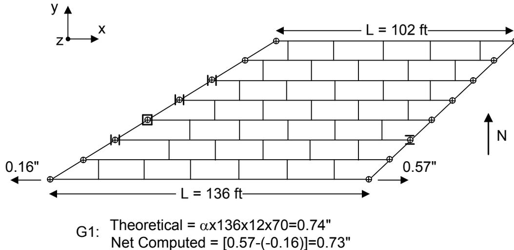
**Figure 6.3.3.3.7-5 Longitudinal Thermal Expansion of G1 – Theoretical vs. Net Computed Expansion from the 3D Analysis**
