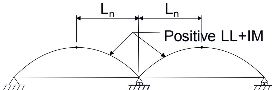
**Figure 6.6.2.4.2.1-2 Definition of Arc Length,  $L_n$**
