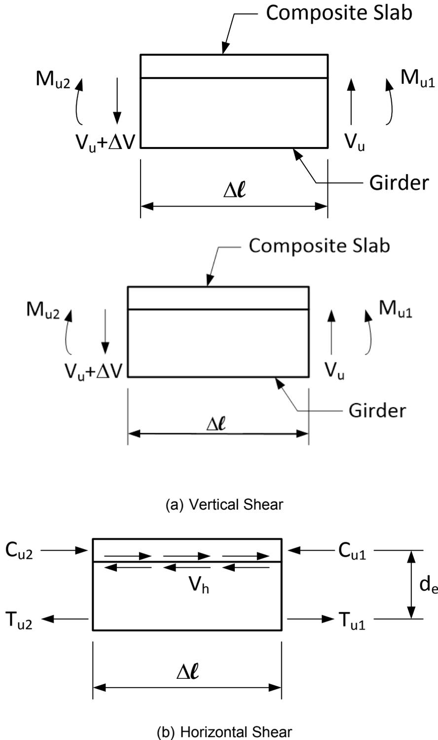
**Figure 5.6.4.2-5 Relationship between Horizontal and Vertical Shear**
