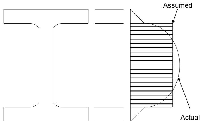
**Figure 6.5.7.1-1 Distribution of Elastic Flexural Shear Stresses (I-Section)**
