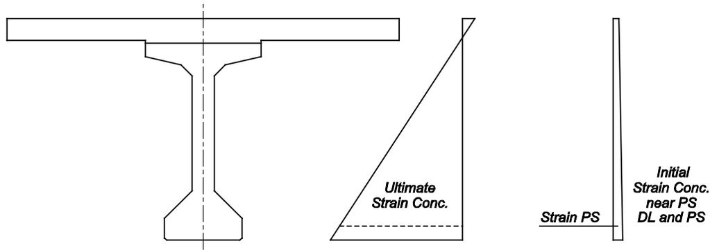
Figure 5.5.4.4.1-1 Total Strain in Prestressing at Strength Limit State
