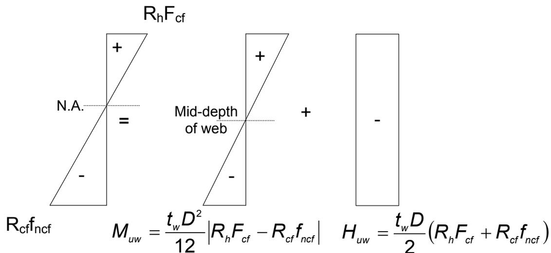
**Figure 6.6.5.2.3.2.3-2 Assumed Flexural Stress Distribution in the Web for the Design of a Bolted Web Splice in a Section Subject to Negative Flexure**
