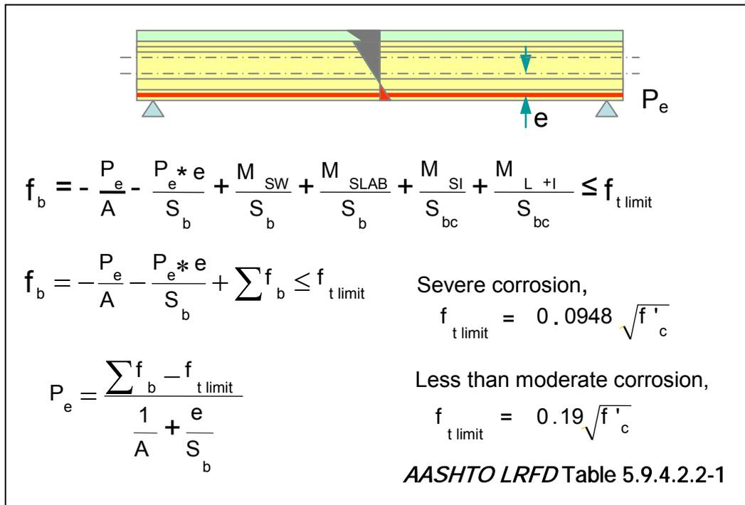
**Figure 5.5.3.4.3-1 Final Effective Prestress Force for Bottom Fiber Tensile Limit**
