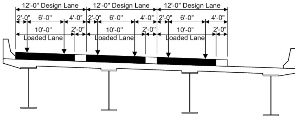
**Figure 4.4.3.2.2-1 Positioning of Design Lanes and Loaded Widths within Lanes**
