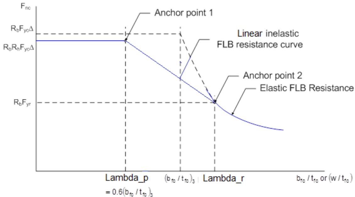
**Figure 6.5.6.2.4.2.1-1 Local Buckling Resistance Curves for Box Flanges in Compression**
