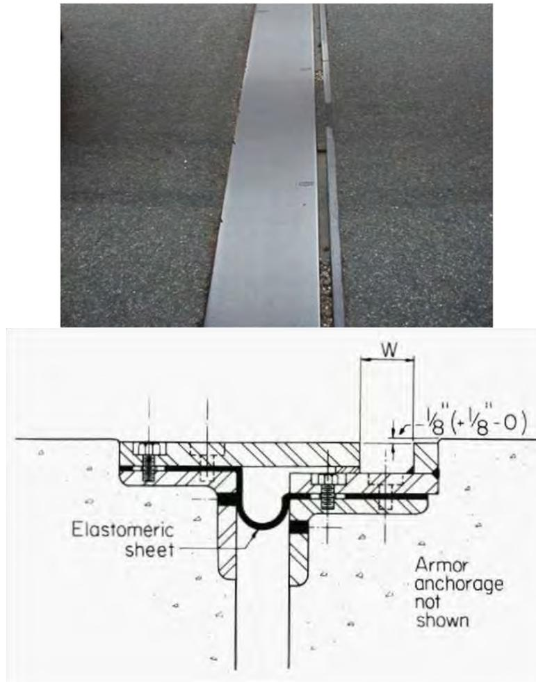
**Figure 8.3.2.1-2 Sliding Plate Joint**
