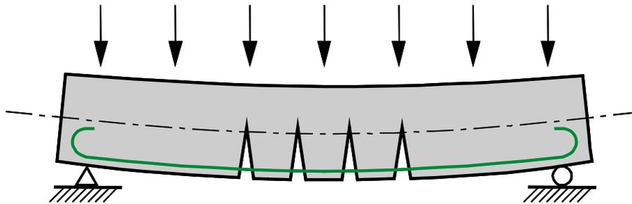
**Figure 5.3.1-2 Reinforced Concrete Beam in Flexure**
