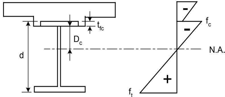
**Figure 6.4.5.4.1.2-1  $D_c$  for a Composite Section in Positive Flexure**
