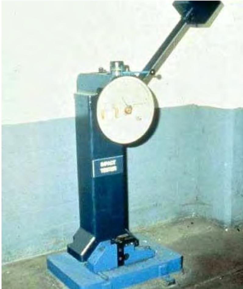
**Figure 6.5.5.3.2.1-1 Charpy V-Notch Testing Machine**
