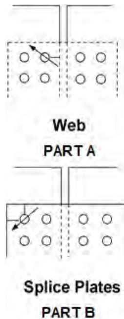
**Figure 6.6.5.2.3.2.4-1 Critical Locations for Checking Bearing Resistance of Outermost Web Splice Bolt Holes**
