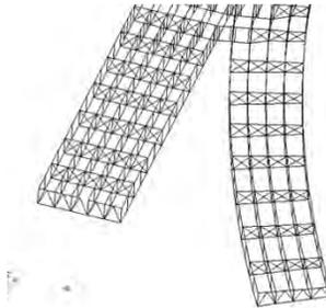
**Figure 6.3.2.5.6-1 Splayed-Girder (Bifurcated) Framing Plan**
