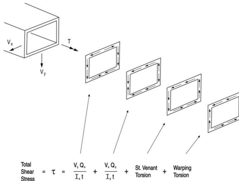
**Figure 5.6.3-3 Components of Shear Flow in Closed Section with Bending about Both Axes**
