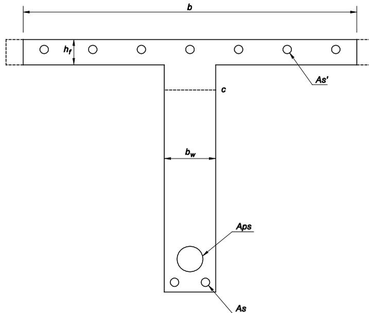
**Figure 5.5.4.3.1-1 Schematic Drawing of T-Section**
