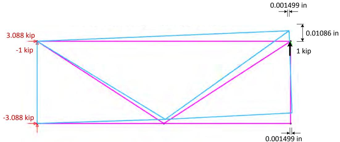
**Figure 4.5.3.2.2.5.3-2 Timoshenko Beam Approach: Calculation of  $A_{seq}$  Based on a Unit Transverse Shear**
