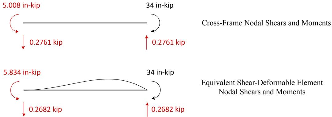
**Figure 4.5.3.2.5.3-3 Comparison of Cross-Frame Nodal Shears and Moments and Equivalent Shear-Deformable (Timoshenko) Beam Shears and Moments**
