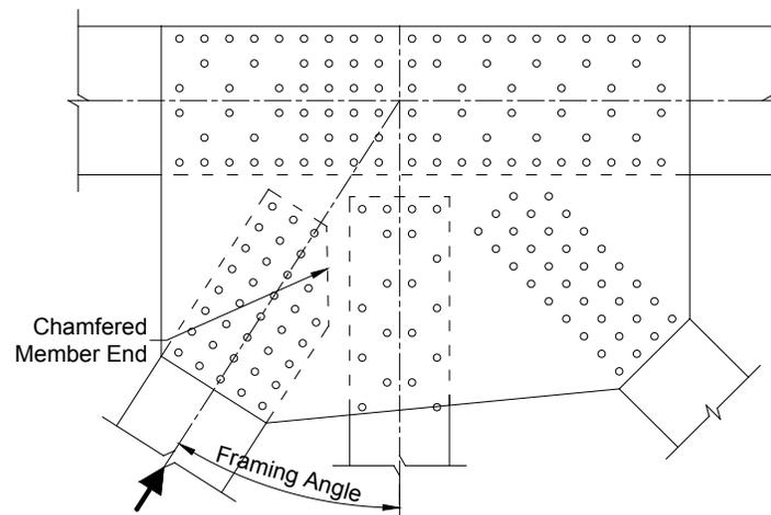
**Figure 6.6.7.3-1 Example Connection Showing a Typical Chamfered Member End and Member Framing Angle**
