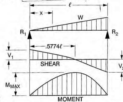
**(8) SIMPLE BEAM – LOAD INCREASING UNIFORMLY TO CENTER (W IS TOTAL LOAD)**
