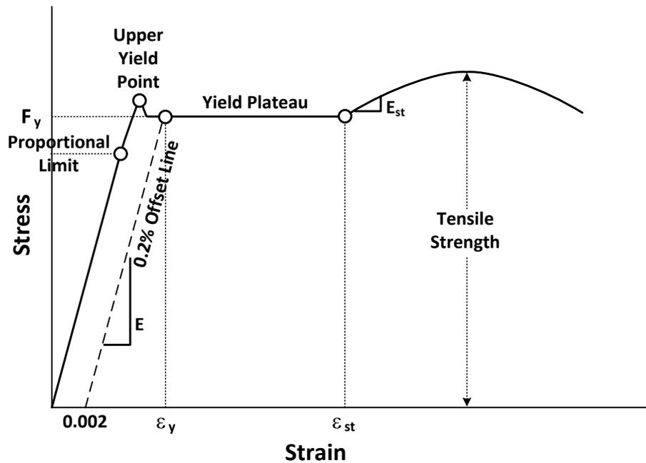
**Figure 6.2.7.1-2 Engineering Tensile Stress vs. Strain Curve for Structural Steels With a Defined Yield Plateau (Wright, 2012)**
