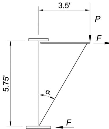
**Figure 6.5.3.4.4.1-1 Example Deck Overhang Bracket**
