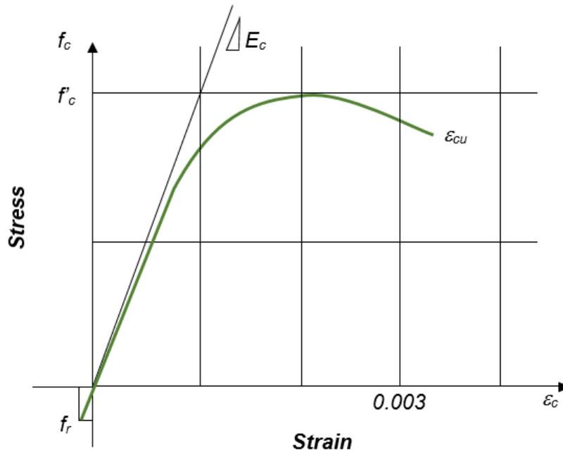
**Figure 5.2.1.2.1-1 Stress-Strain Curve for Concrete**
