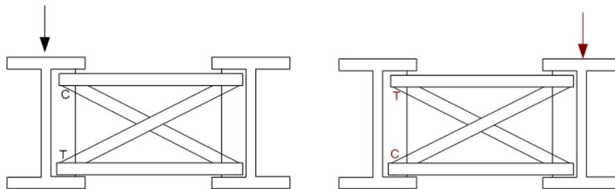
**Figure 6.6.4.4-1 Cross-Frame Diagonal Forces in an X-Type Cross-Frame due to a Concentrated Load Over Each Girder**
