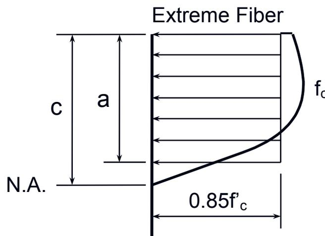
Figure 5.5.4.2-2 Concrete Stress Block Assumption
