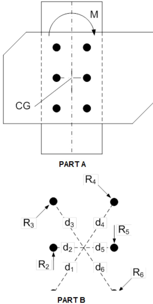
Figure 6.6.4.2.6-2 Analytical Model for Torque on a Bolt Group
