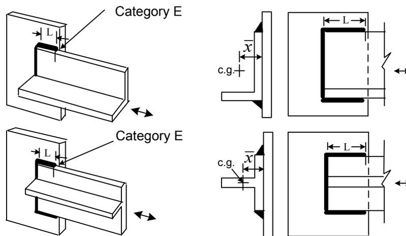
**Figure 6.6.3.3.5.2-1 Welded Connection of a Single-Angle and a Tee Member to a Gusset Plate**
