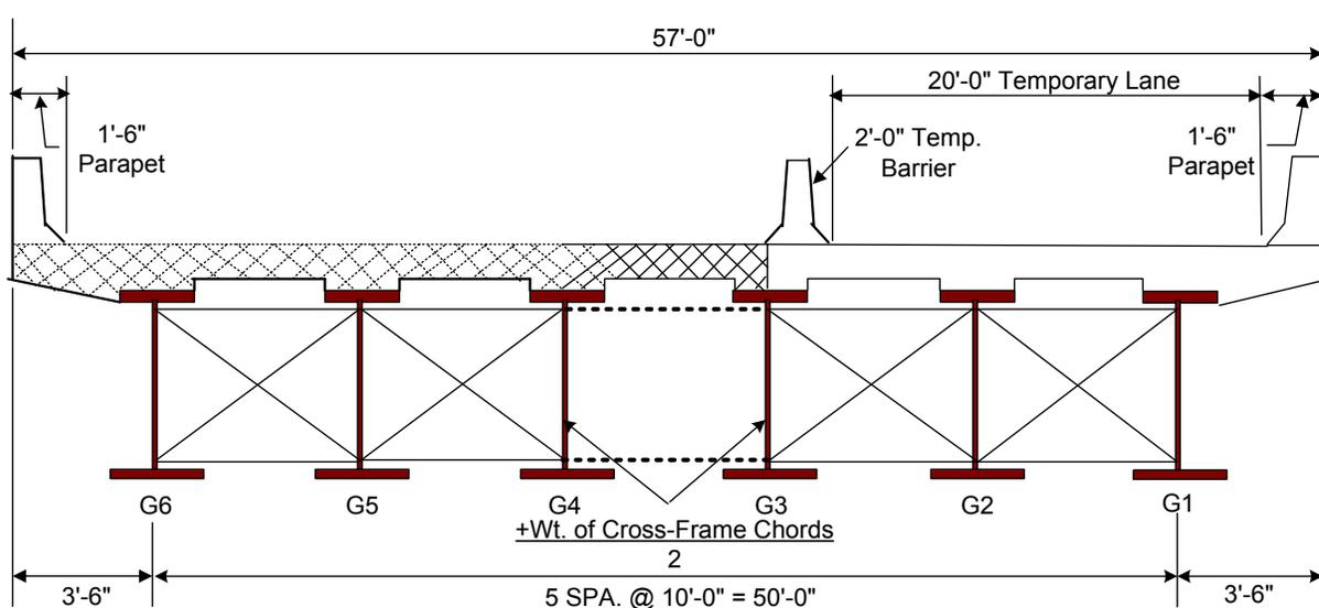
**Figure 6.3.2.5.4.3-2 Phased Construction Without a Closure Pour – Deck Cast onto Last Phase**
