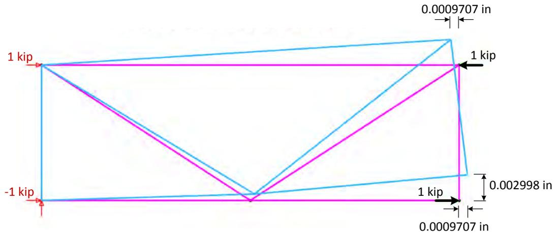
**Figure 4.5.3.2.2.5.3-1 Timoshenko Beam Approach: Calculation of  $I_{eq}$  Based on Pure Bending**
