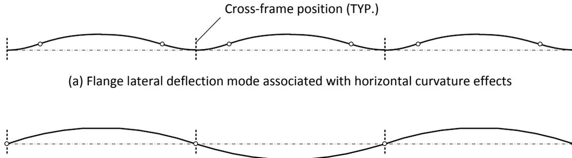
**Figure 6.5.2.1.3.2-2 Second-order Elastic Lateral Deflections due to Horizontal Curvature Effects Versus the Unwinding Stability Failure Mode of the Compression Flange**
