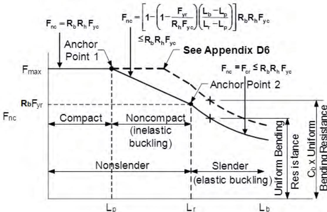
Figure 6.5.6.2.2.2-2 Lateral Torsional Buckling Resistance,  $F_{nc}$
