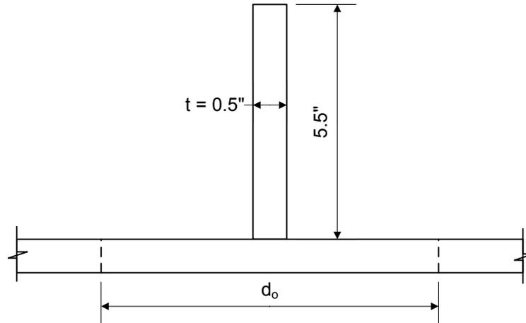
**Figure 6.5.5.2.2.3.2-13 Calculation of Effective Width,  $d_o$ , of the Web Plate**
