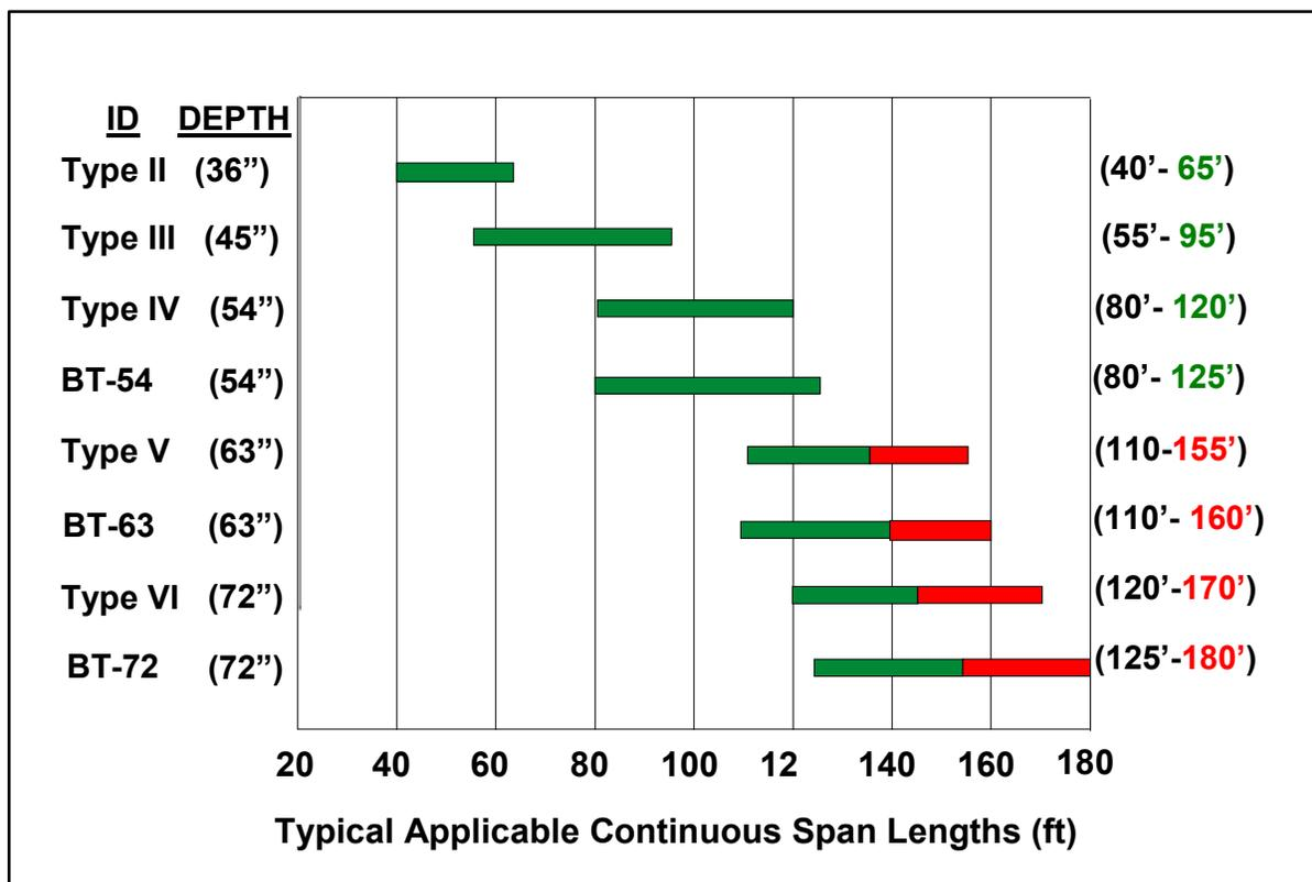
**Figure 5.4.3-2 Increase in Span Length from Structural Continuity**
