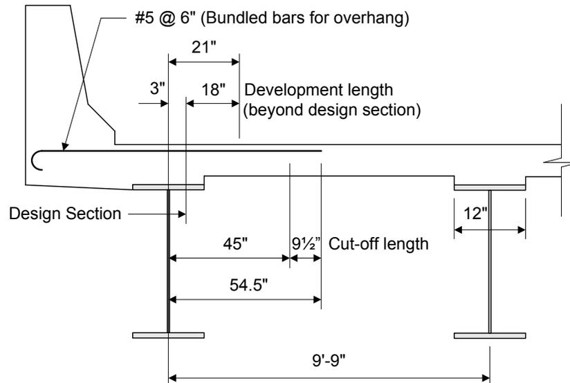
**Figure 7.3.4.4-1 Length of Overhang Negative Moment Reinforcement**
