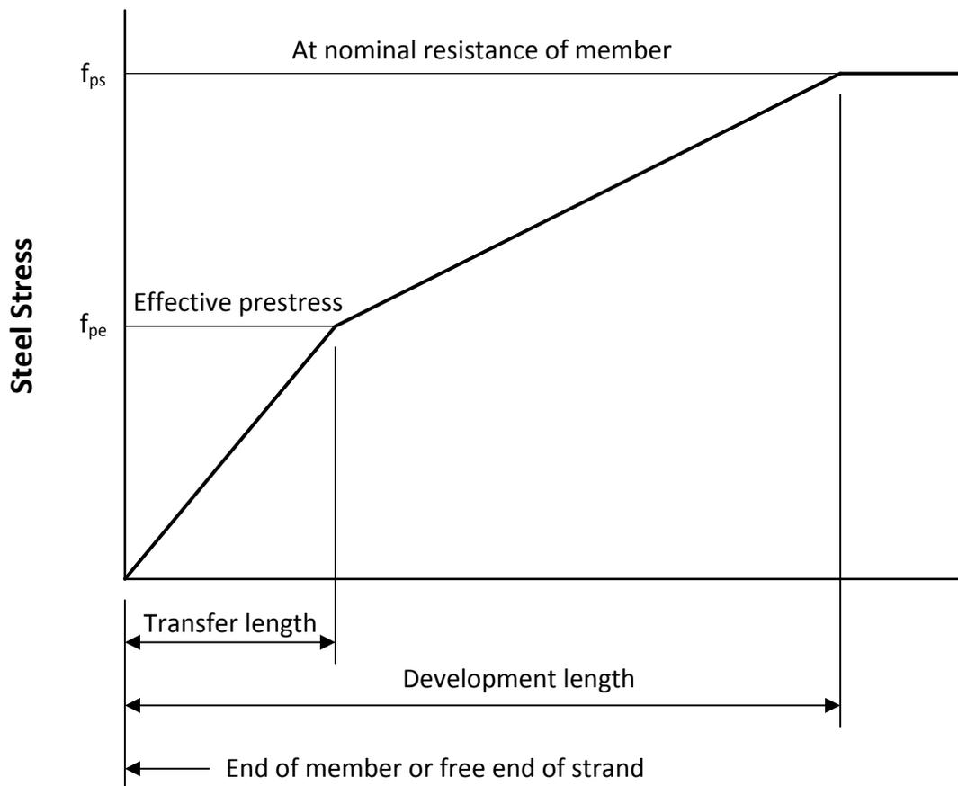
**Figure 5.9.3-1 Idealized Relationship between Steel Stress and Distance from Free End of Strand**
