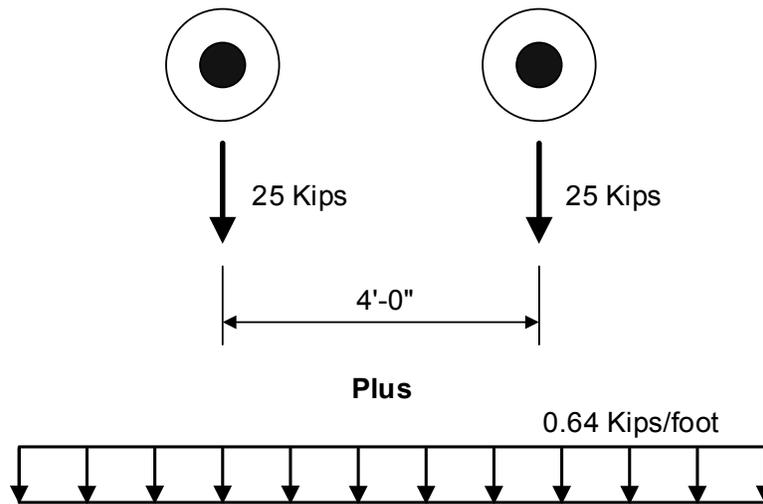
Figure 3.4.3.1-1 Effect of Design Tandem Plus Design Lane Load
