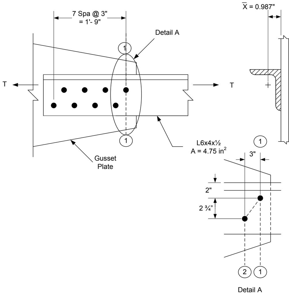
**Figure 6.6.3.3.2.5-3 Example – Factored Tensile Resistance of Single Angle Bracing Member**
