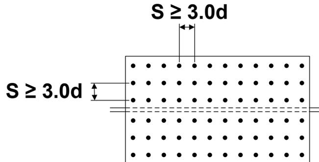
Figure 6.6.4.2.2.2.1-1 Minimum Spacing Requirement Between Centers of Bolts
