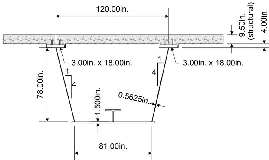
**Figure 6.5.6.2.4.3-1 Example Composite Tub Section at an Interior Pier**
