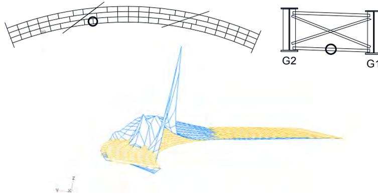
**Figure 4.4.3.2.1-4 Influence Surface for Cross-Frame Force in the Bottom Chord of a Cross-Frame in Span 2 of the Example I-Girder Bridge**
