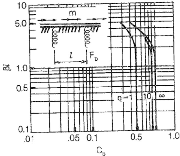
Figure 6.5.5.2.2.3.2-9 BEF Factor,  $C_b$ , for Distortional Axial Cross-Bracing Force due to a Uniform Torque,  $m$
