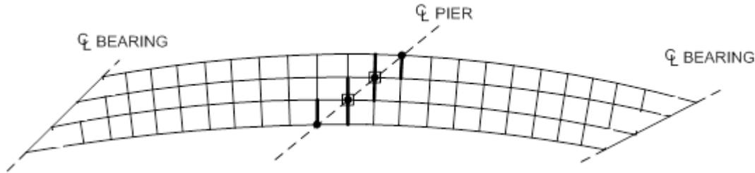
**Figure 6.3.2.9.4.3.3-1 Skewed and Curved I-Girder Bridge: No Cross-Frame Along the Skewed Interior Support Line**
