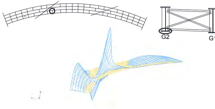
**Figure 4.4.3.2.1-5 Influence Surface for Bottom Flange Lateral Bending Moment in G2 of the Example I-Girder Bridge at a Cross-Frame in Span 2**
