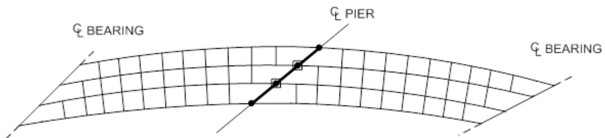
**Figure 6.3.2.9.4.3.3-2 Skewed and Curved I-Girder Bridge with Discontinuous Cross-Frames: Cross-Frame Along the Skewed Interior Support Line**
