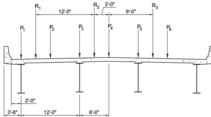
**Figure 4.4.2.2.2-3 Exterior Girder LLDF – Special Rigid Cross-Section Analysis**
