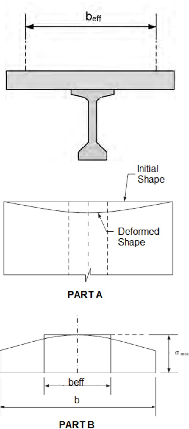
**Figure 4.2.2.1-1 Shear Lag in a Composite Girder**
