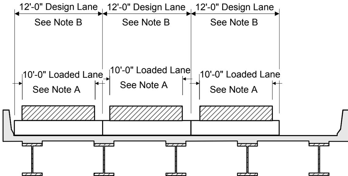
Note A: Position loaded lane within the design lane such that the effect being considered is maximized.
