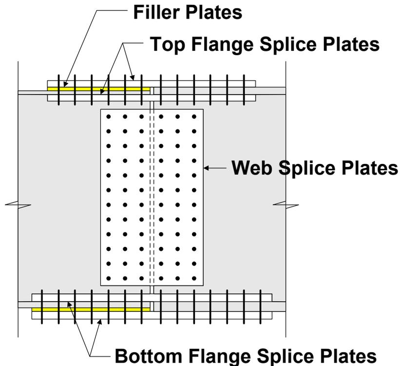
**Figure 6.6.5.2.1-1 Typical Bolted Girder Splice**
