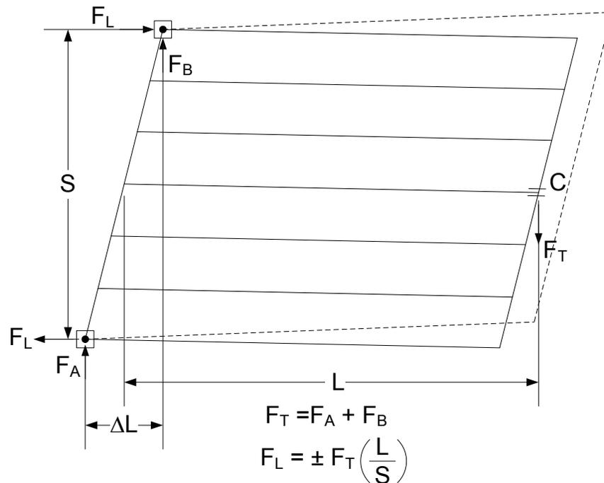
**Figure 6.3.3.3.7-3 Twist of a Simple-Span Skewed Bridge Under Uniform Thermal Expansion & Resulting Lateral Reactions**
