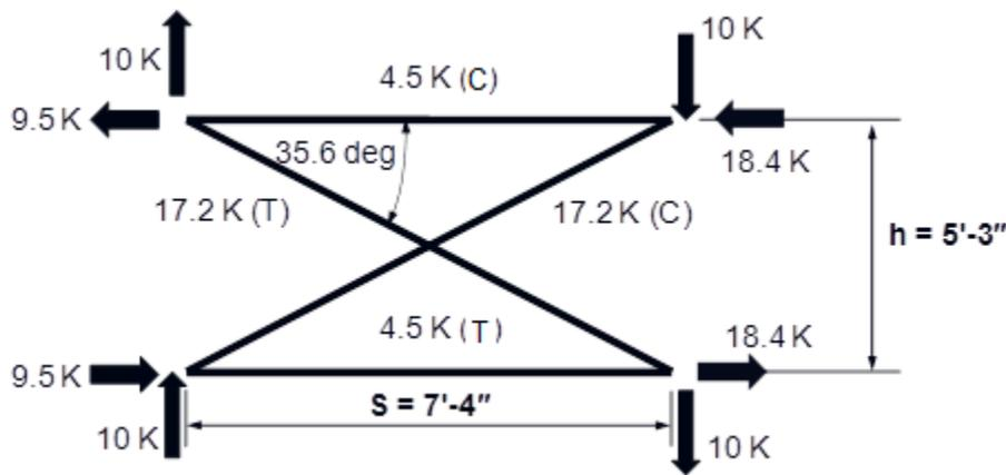
**Figure 4.5.3.2.2.5.3-12 Example Cross-Frame Internal Member Forces Calculated Using the Method of Joints**
