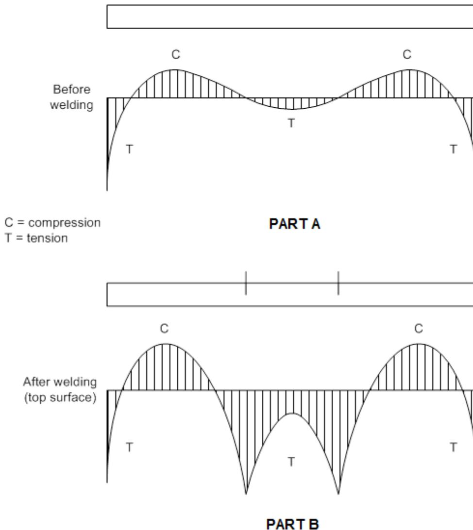
**Figure 6.6.3.4.2.3.2-3 Typical Residual Stress Distribution in Welded Flange Plates**
