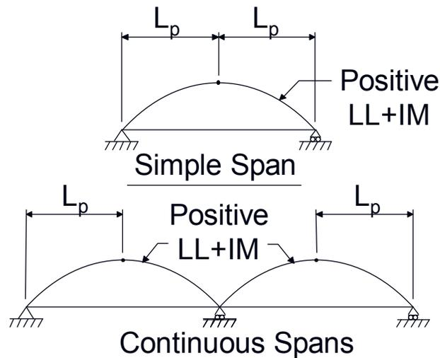
Figure 6.6.2.4.2.1-1 Definition of Arc Length,  $L_p$
