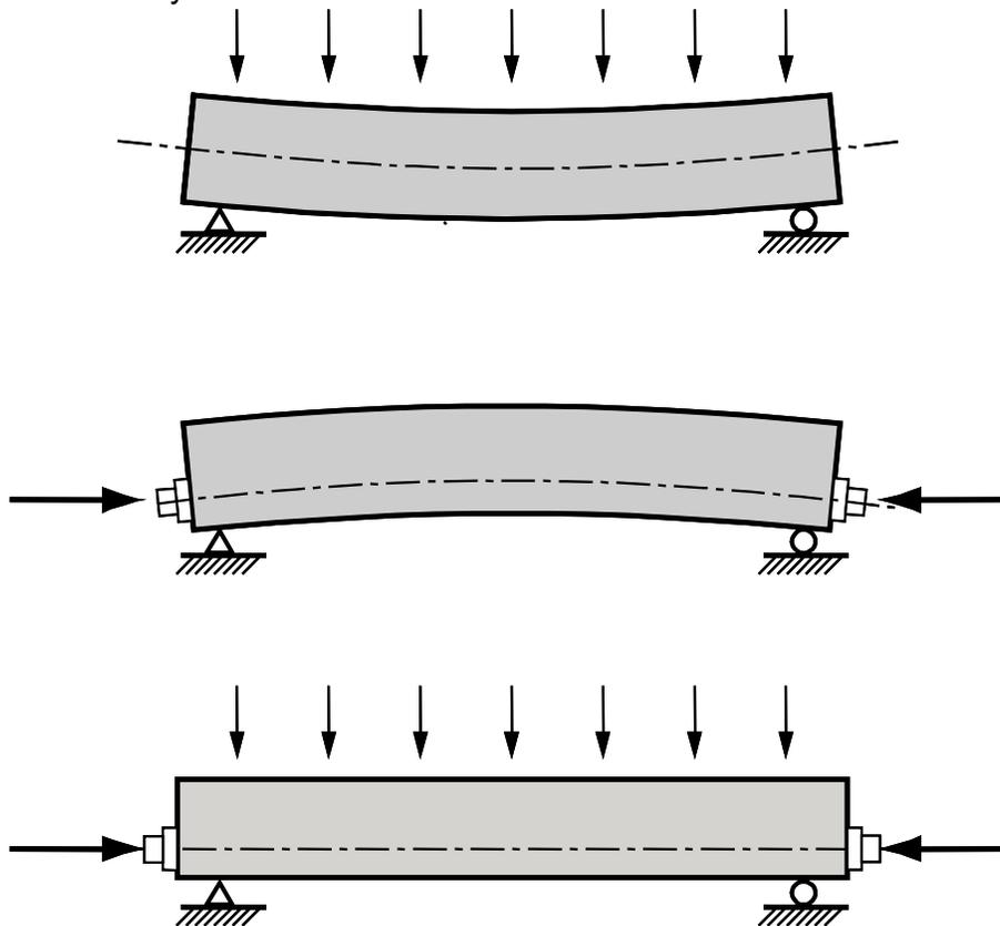
**Figure 5.3.2-1 Effect of Prestressing in Simple-Span Beam**
