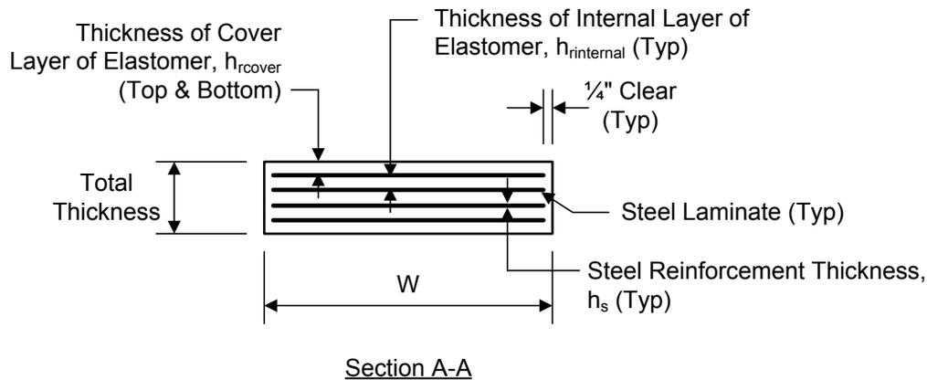
**Figure 8.2.3.2.3-1 Reinforced Elastomeric Pad**
