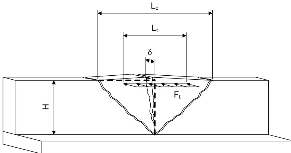
**Figure 7.3.4.2.1-2 Assumed Yield Line Pattern for Barrier Wall**
