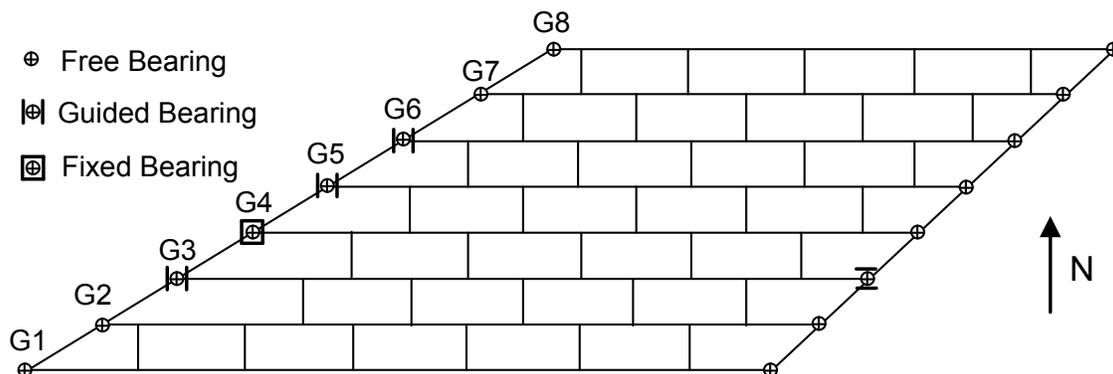
**Figure 6.3.3.3.7-4 Plan View of Straight Simple-Span Skewed Bridge w/
