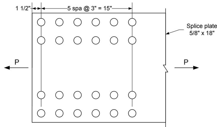
**Figure 6.6.4.2.5.3-3 Bearing Resistance Example – Flange Splice Plate**
