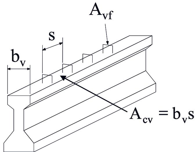
**Figure 5.6.4.4-1 Reinforcement Required**
