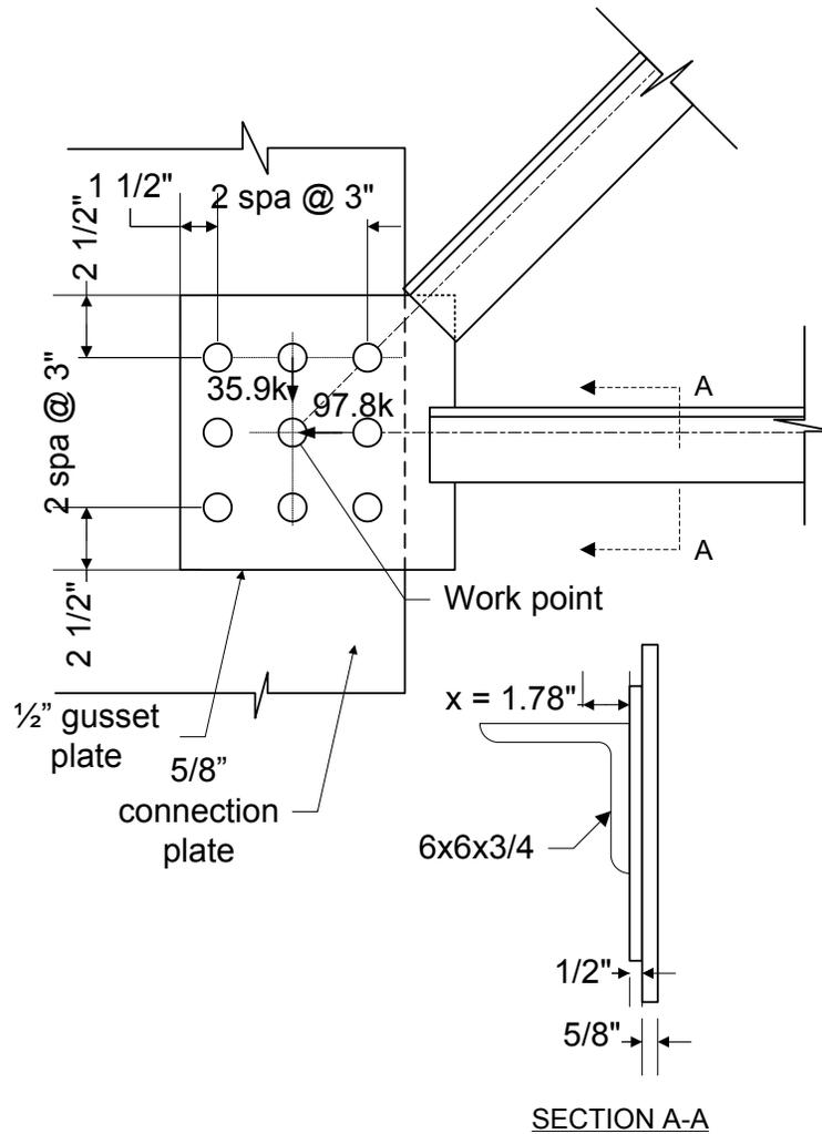
**Figure 6.6.4.2.6-5 Example Gusset-Plate Configuration for Bolted Bracing Member Connection – Option 2**
