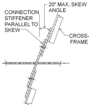
**Figure 6.3.2.9.6.3.1-2 Skewed Connection Plate**
