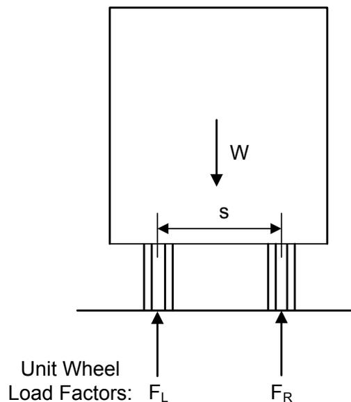
**Figure 3.4.9.2-1 Unit Wheel-Load Factors due to the Combined Effects of Centrifugal Force and Superelevation**
