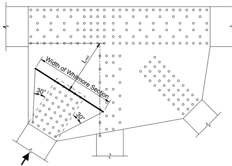
**Figure 6.6.7.3-2 Example Connection Showing the Whitmore Section for a Compression Member Derived from 30 Degree Dispersion Angles, and the Distance  $L_{mid}$**
