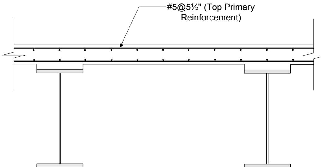
**Figure 7.3.2.4-6 Primary Reinforcement in Top of Deck**
