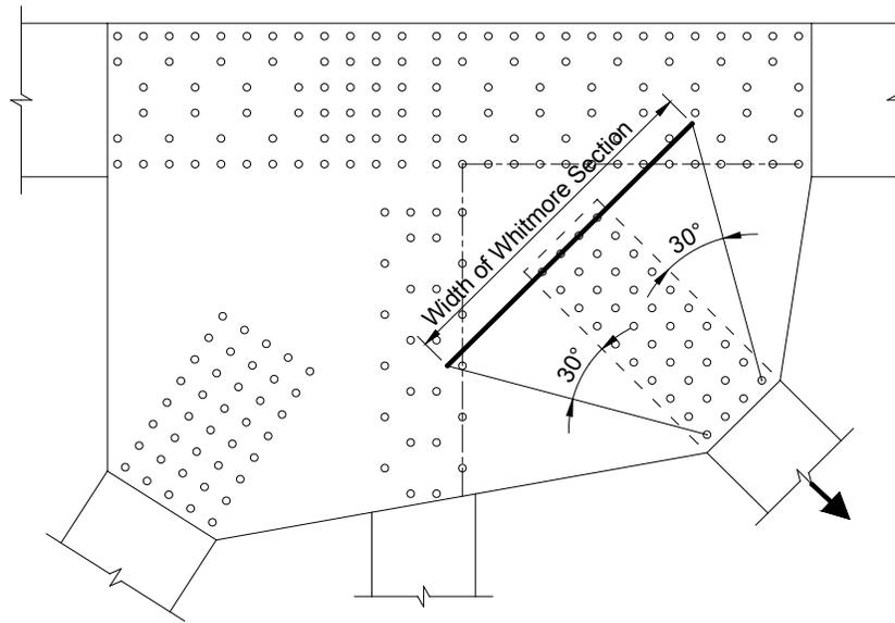
**Figure 6.6.7.4-1 Example Connection Showing the Whitmore Section for a Tension Member Derived from 30 Degree Dispersion Angles**
