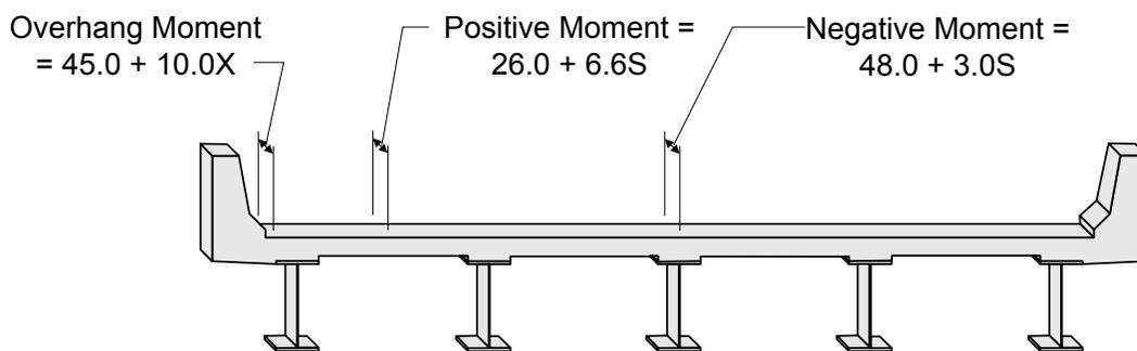
**Figure 7.3.2.4-2 Equivalent Strip Widths**
