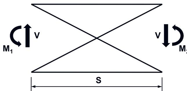
**Figure 4.5.3.2.2.5.3-6 Global Shear and Moment on the Truss-Type Cross-Frame**
