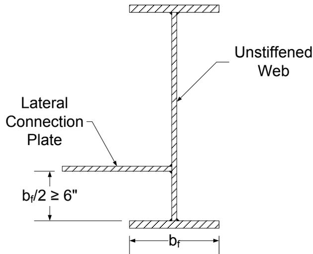
**Figure 6.3.2.10.4-5 Recommended Lateral Connection Plate Detail for Plate Attached to Unstiffened Girder Web**
