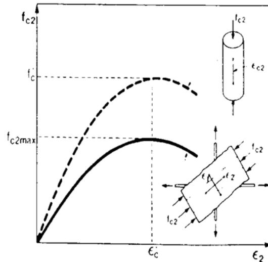
**Figure 5.6.1.1.3-2 Comparison of Concrete Compressive Strength between Cylinder in Uniaxial Compression (Dashed Line) and Beam Subjected to Combined Flexure and Shear (Solid Line)**
