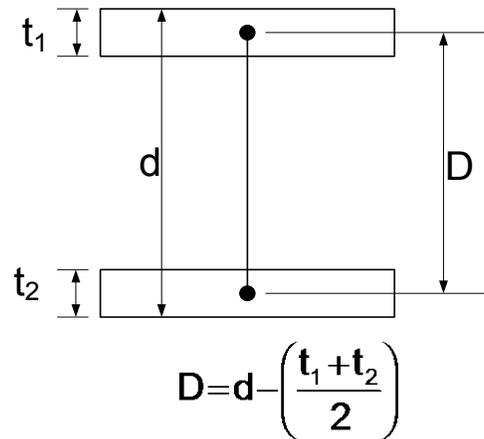
**Figure 4.5.3.3.2.3.6-1 Overstating of the Web Depth in Shallow Girders**
