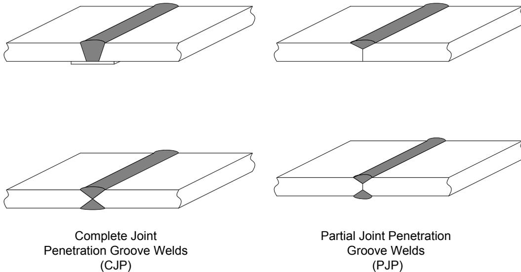
**Figure 6.6.4.3.3.2.1-1 Subcategories of Groove Welds**
