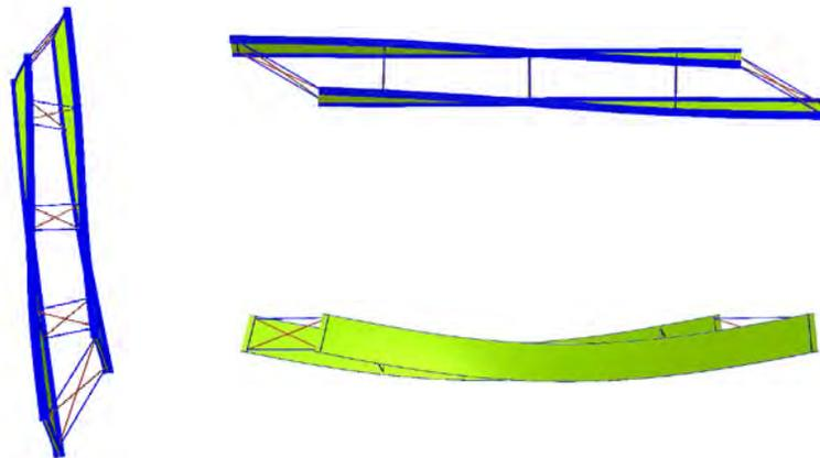
**Figure 6.4.9.5.1.1-2 Magnified Girder Vertical Deflections and Twist for Two Simple-Span I-Girders on Parallel Skewed Supports Subjected to Steel Dead Load when Cross-Frames are Connected to the Girders**
