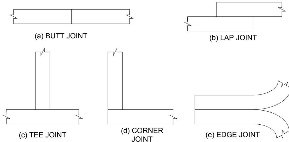
**Figure 6.6.4.3.4-1 Types of Welded Joints**
