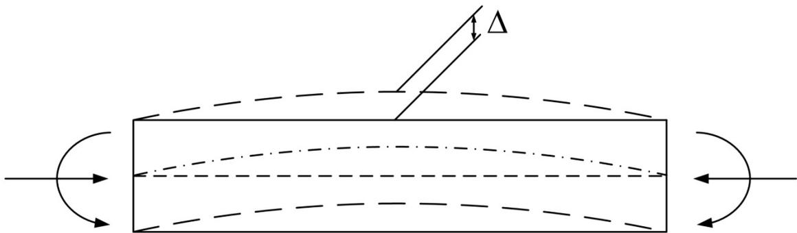
**Figure 6.5.2.1.3.2-1 Amplification Effect in a Discretely Braced Compression Flange**
