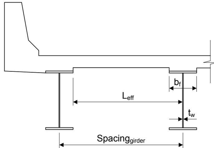
**Figure 7.3.3.3-1 Effective Slab Length**
