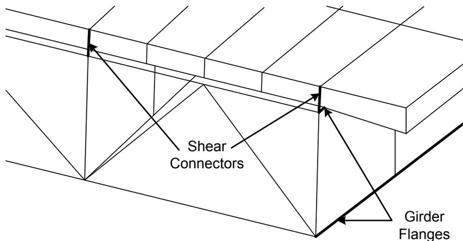
**Figure 4.5.3.3.2.3.1-2 Beam Elements Used to Model Girder Flanges & Shear Connectors**
