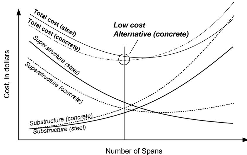
**Figure 2.3.4.2-2 Spans and Materials versus Cost**
