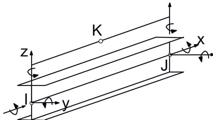
**Figure 4.5.3.2.2.2-2 Beam Element**
