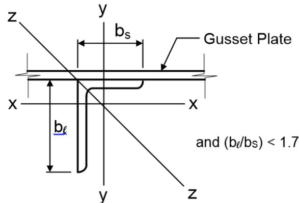
**Figure 6.6.3.4.5.2-2 Unequal-Leg Angles Connected Through the Shorter Leg with Ratio of Leg Lengths < 1.7**
