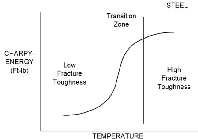
**Figure 6.5.5.3.2-1 Typical Plot of Charpy Energy Versus Temperature for a Steel**
