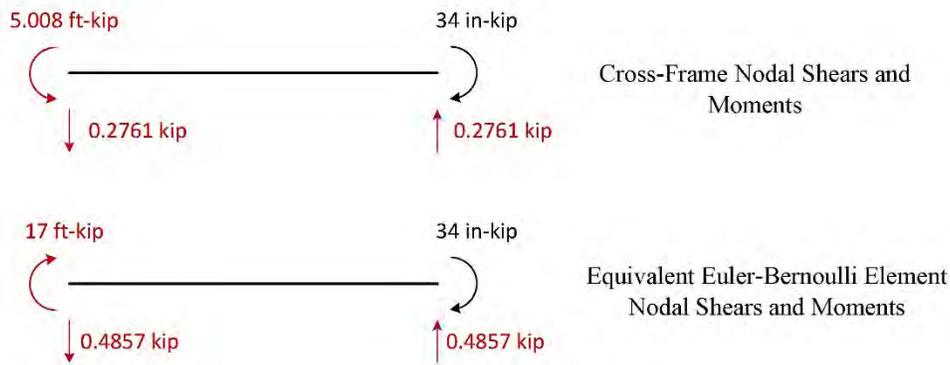
**Figure 4.5.3.2.5.3-4 Comparison of Cross-Frame Nodal Shears and Moments and Equivalent Euler- Bernoulli Beam Shears and Moments (Flexure Stiffness Approach)**
