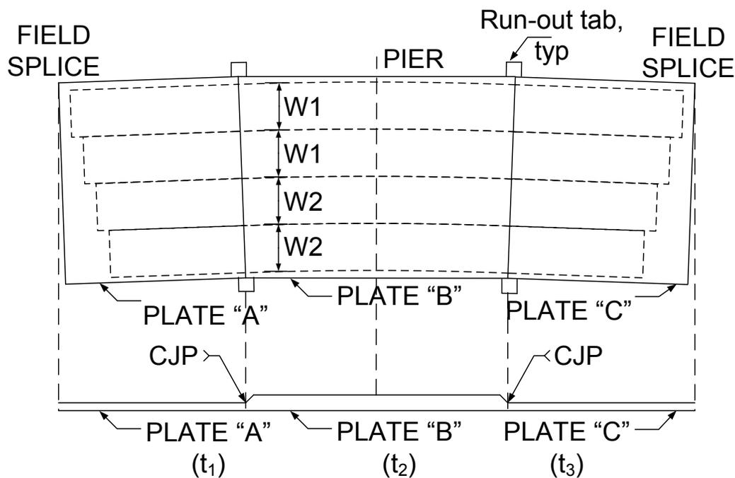
**Figure 6.3.4.4.5-4 Slab Welding – Nesting of Curved Flange Plates for a Pier Section**
