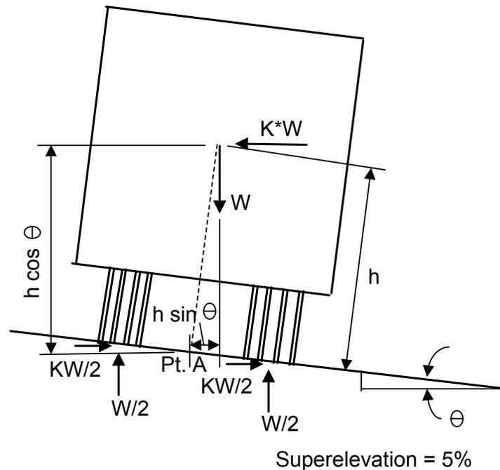
**Figure 3.4.9.4-2 Centrifugal Force Balanced by Superelevation**
