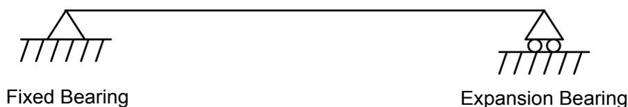
**Figure 8.2.1-2 Schematic of Fixed and Expansion Bearings**
