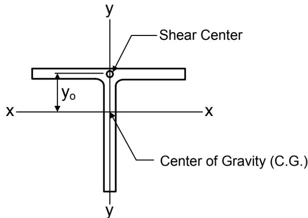
Figure 6.6.3.4.2.3.4-1 Calculation of  $y_o$  for a Tee Section
