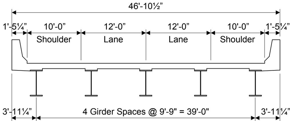
**Figure 7.3.2.4-1 Superstructure Cross Section for Design Example**
