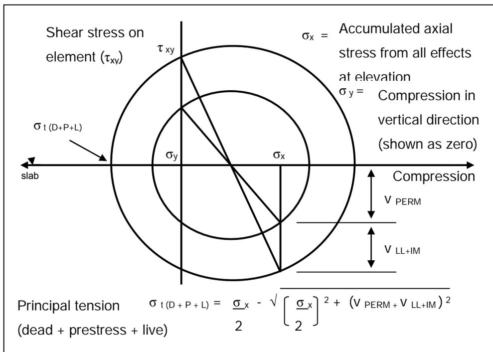
Figure 5.6.2-2 Mohr's Circle for Stress (Principal Tension)
