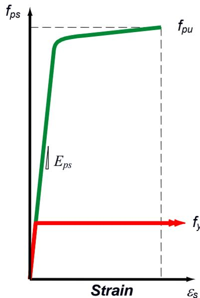
**Figure 5.2.3-1 Stress-Strain Curves for Prestressing Strand and Mild Steel**
