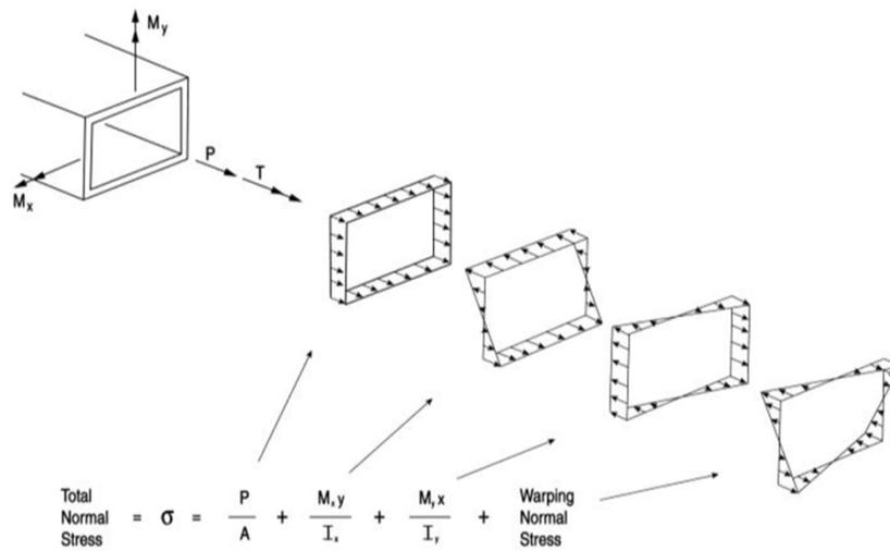
**Figure 5.6.3-4 Components of Flexural Stress in Closed Section with Bending about Both Axes**
