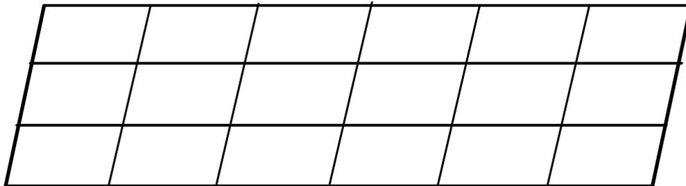
**Figure 6.3.2.9.4.3.1-1 Contiguous Cross-Frame/Diaphragm Lines Parallel to Skew (for Skew  $\leq 20^\circ$ )**
