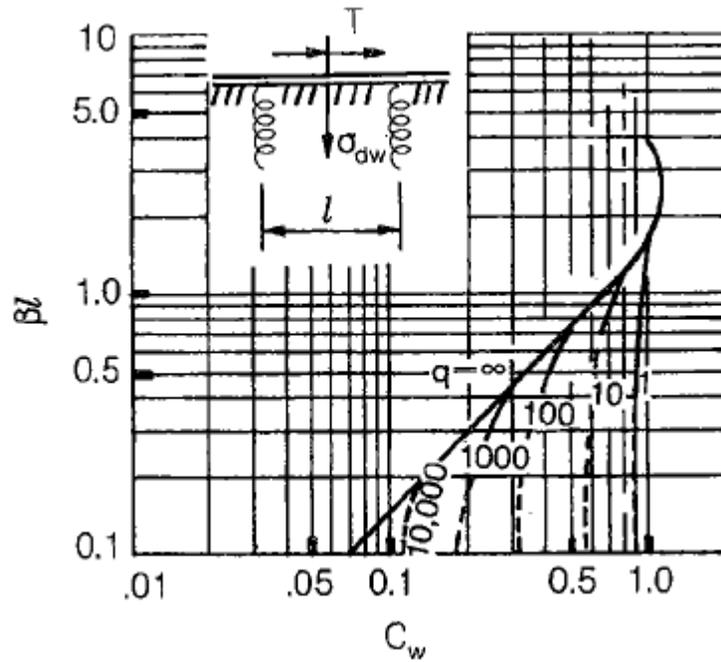
Figure 6.5.5.2.2.3.2-4 BEF Factor,  $C_w$ , for Distortional Longitudinal Warping Stress at Midpanel due to a Concentrated Torque,  $T$ , at Midpanel
