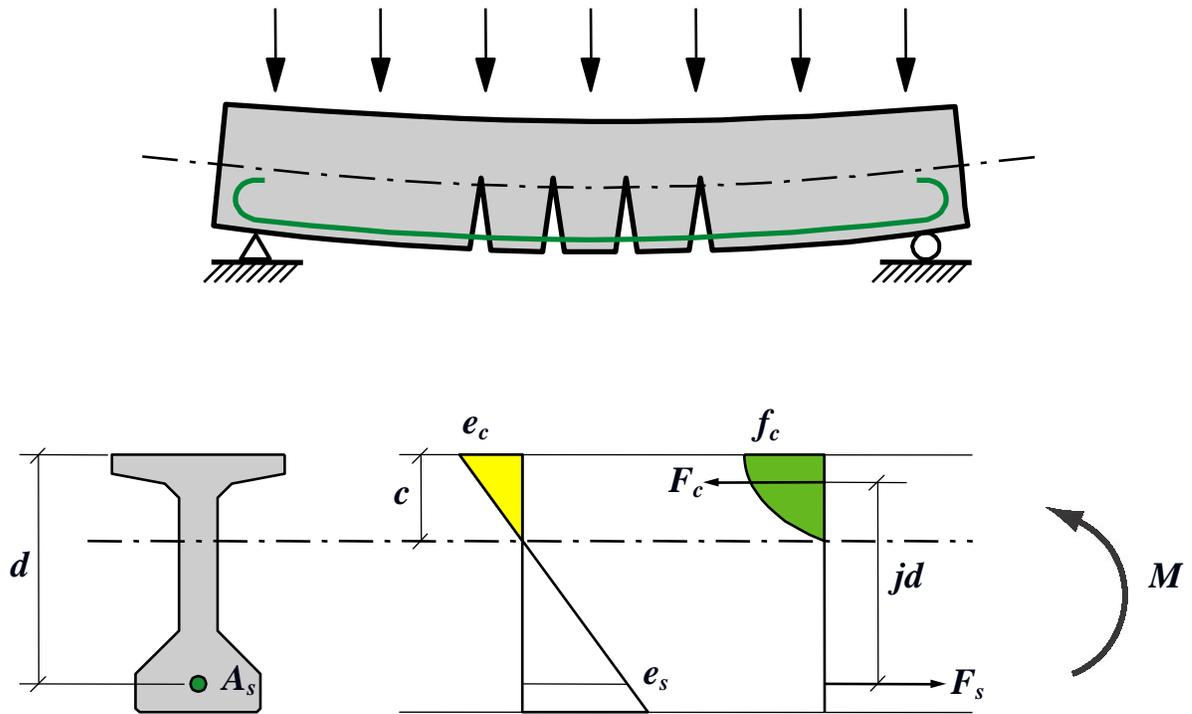
**Figure 5.5.4-1 Ultimate Flexural Resistance in Girders**
