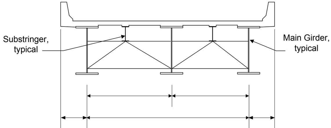
**Figure 6.3.2.5.7-1 Girder-Substringer Cross-Section**
