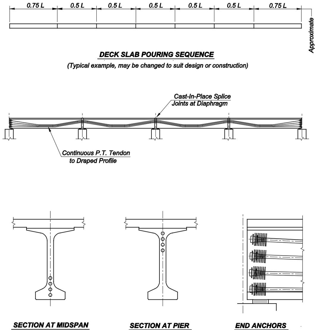
**Figure 5.10.4.3.2-1 Post-Tensioning for Four-Span Continuous Girder Spliced at Piers**
