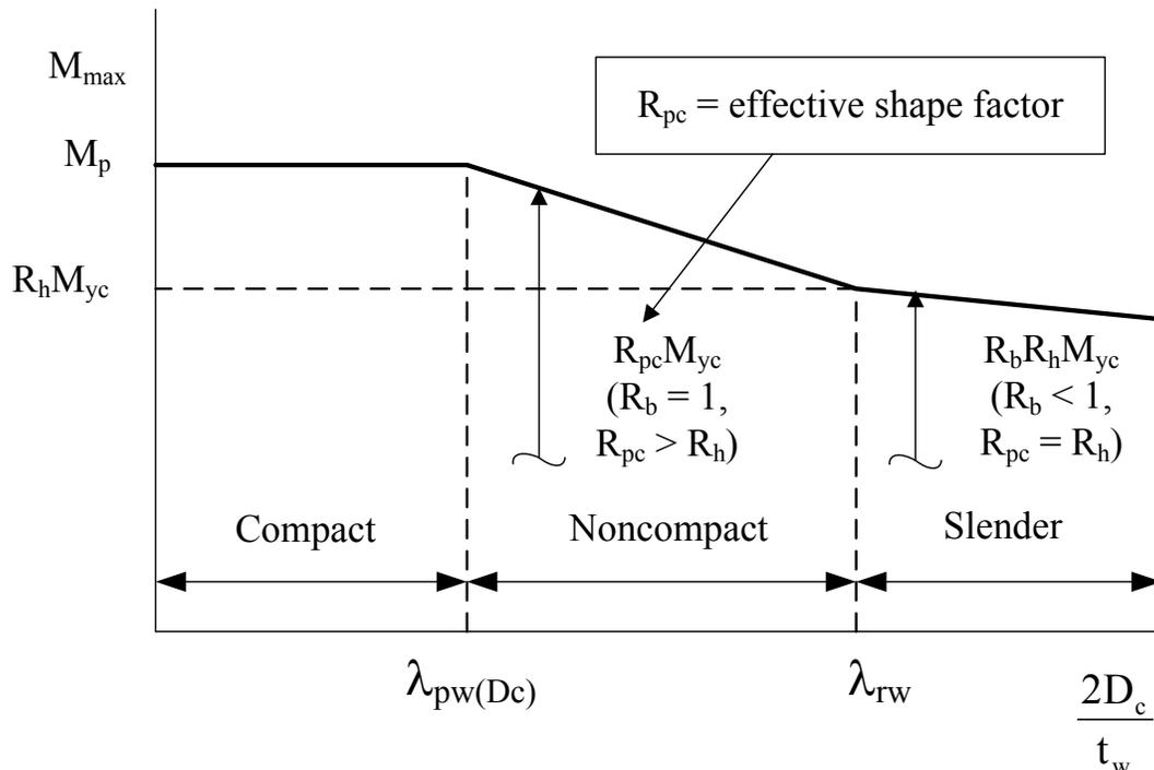
**Figure 6.5.6.2.2.1.1-1  $M_{max}$  versus Web Slenderness for Composite I-Sections Subject to Negative Flexure and Non-Composite I-Sections**
