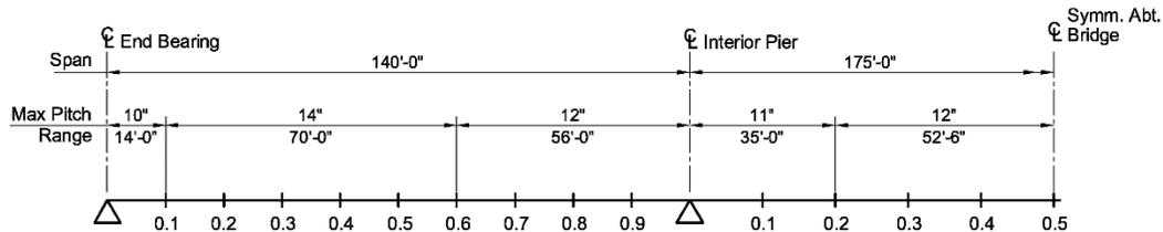
**Figure 6.6.2.4.3-1 Final Recommended Pitches - Example**
