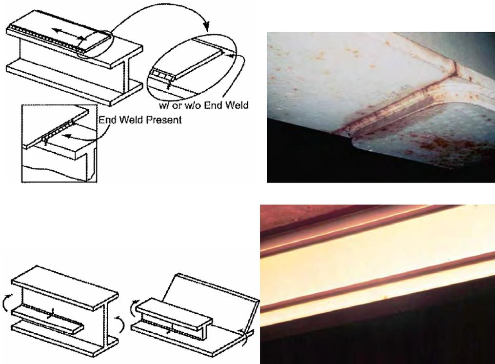
Figure 6.5.5.2.2.1.2-2 Sample Illustrative Examples of Fatigue Details
