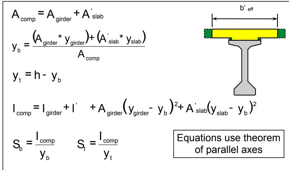
Figure 5.5.3.2.2-4 Calculation for Composite Section Properties
