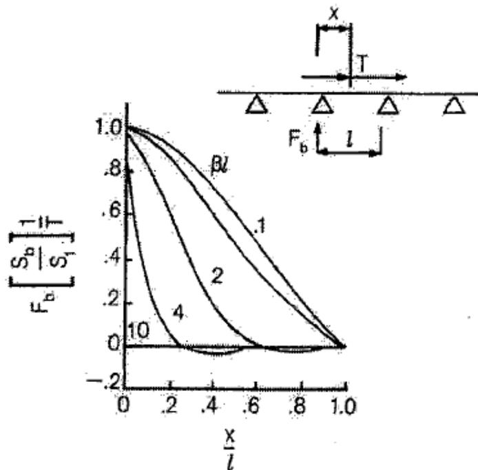
Figure 6.5.5.2.3.2-11 Influence Line for Distortional Axial Cross-Bracing Force for a Rigid Cross-Brace due to a Concentrated Torque,  $T$
