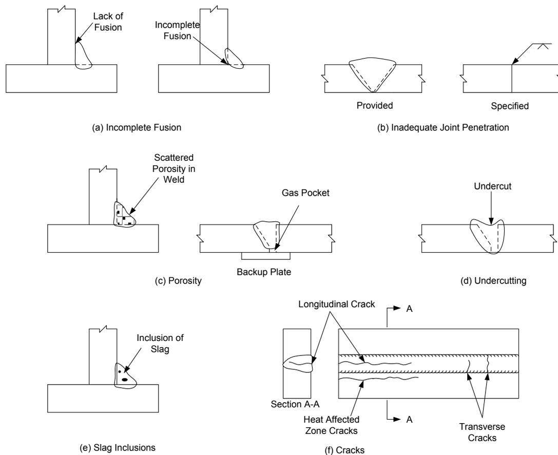
**Figure 6.6.4.3.6.1-1 Potential Weld Defects**
