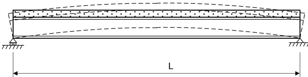
**Figure 3.7.3-1 Temperature Gradient**
