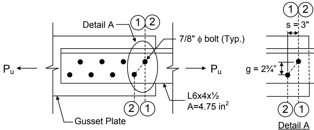
$$\begin{aligned} \text{Chain 1-1: } A_n &= 4.75 - [1(0.9375)(0.5)] = 4.28 \text{ in.}^2 \\ \text{Chain 2-2: } A_n &= 4.75 - [2(0.9375)(0.5)] + \left[ \frac{(3.0)^2}{4(2.75)}(0.5) \right] = 4.22 \text{ in.}^2 \quad (\text{Governs}) \end{aligned}$$
