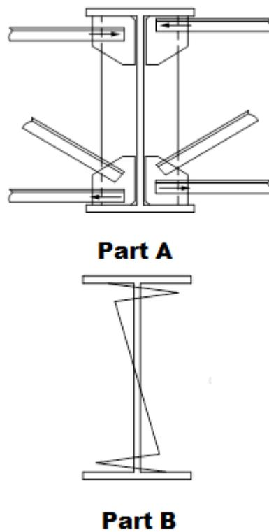
**Figure 6.3.2.9.6.2-2 Connection-Plate Bending Resulting from Cross-Frame Alignment**
