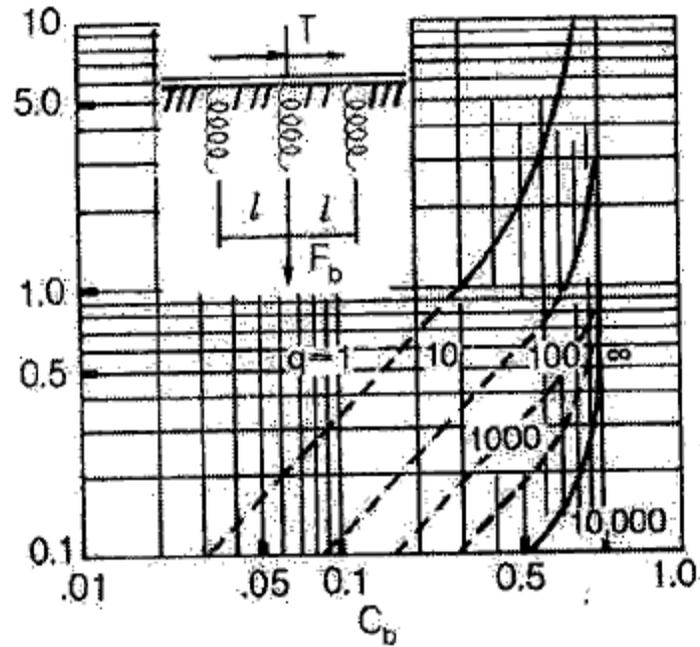
Figure 6.5.5.2.3.2-10 BEF Factor,  $C_b$ , for Distortional Axial Cross-Bracing Force due to a Concentrated Torque,  $T$ , at Cross-Bracing
