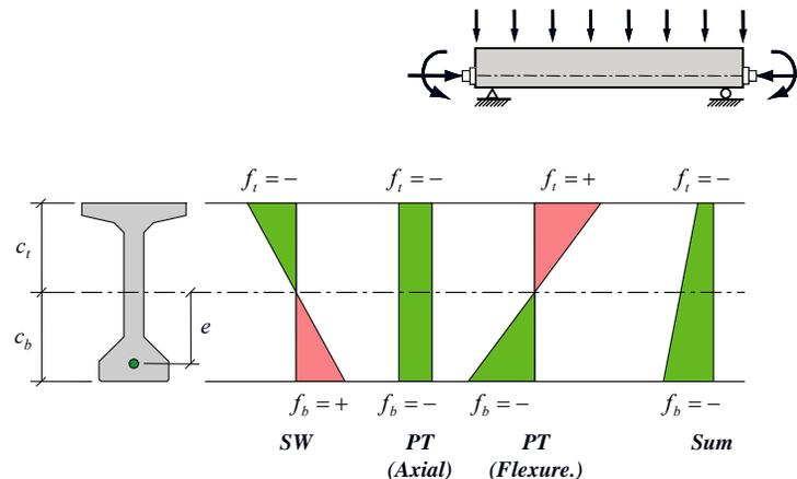
**Figure 5.3.3-4 Summation of Self Weight, Axial and Eccentric Prestress Stresses**
