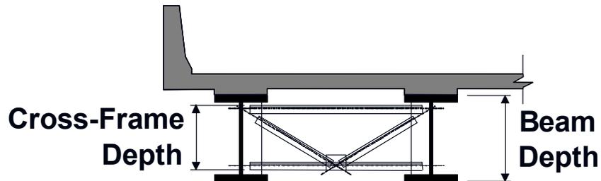
**Figure 6.3.2.9.5.1-1 Cross-Frame and Beam Depth**
