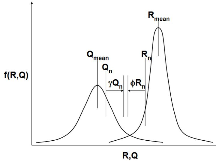
Figure 1.2.3-1 Bell Curves Illustrating Distribution of Load and Resistance
