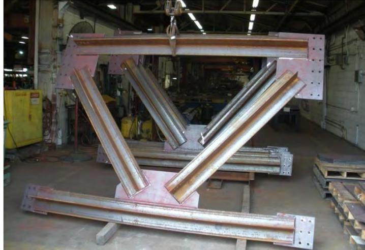
**Figure 6.6.3.5.3-1 Cross-Frame Composed of Structural Tees**
