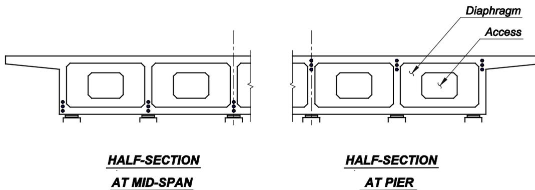
Figure 5.4.4.1-1 Typical Multi-Cell Cast-in-Place Superstructure
