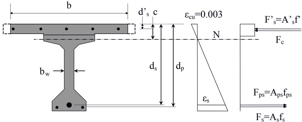
**Figure 5.5.4.2-1 Strain Compatibility for a Composite Concrete Girder**
