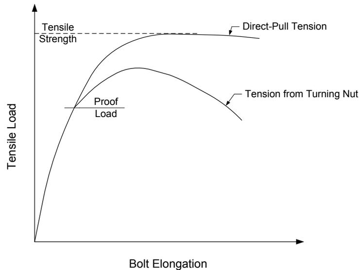
**Figure 6.2.3.1.2-1 Typical Tensile Load-Elongation Curve for a High-Strength Bolt**
