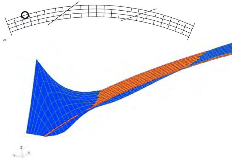
**Figure 4.4.3.2.1-1 Influence Surface for Vertical Bending Moment in Span 1 of G4 of the Example I-Girder Bridge**
