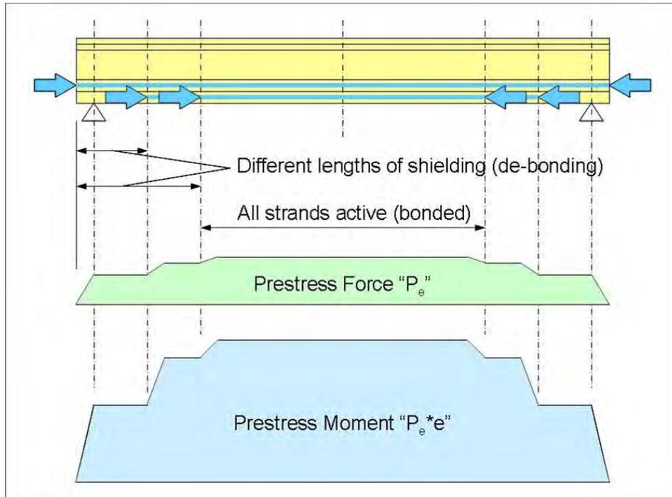
**Figure 5.5.3.4.6-1 Reduction of Prestress Force by Shielding Strands (Debonding)**
