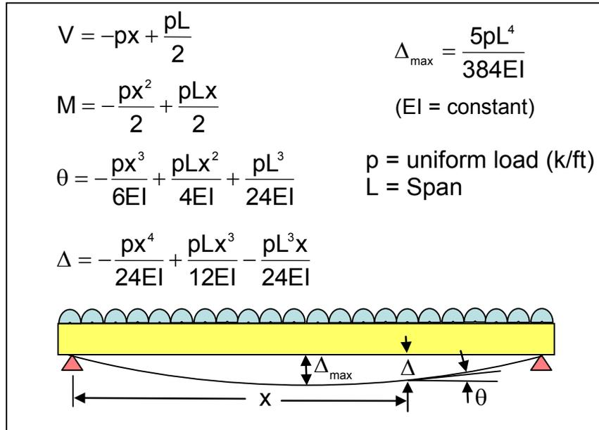
**Figure 5.5.8.2-2 Deflection of a Beam under Uniform Load**
