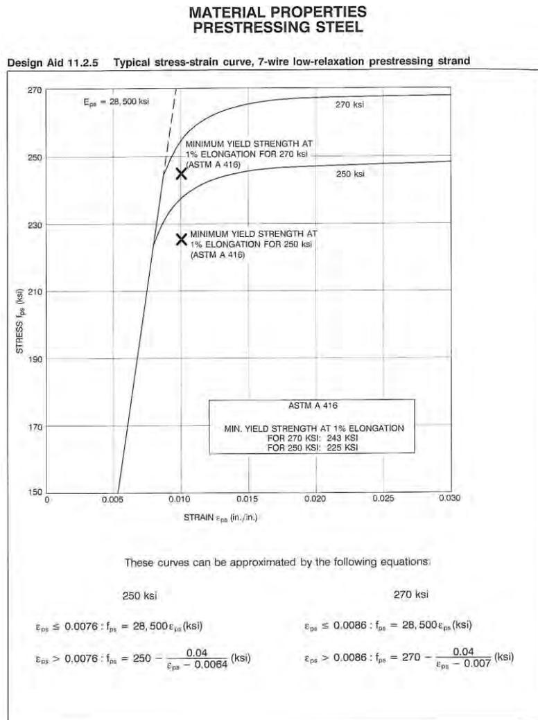
Figure 5.5.4.4.1-2 Material Properties of Prestressing Steel
