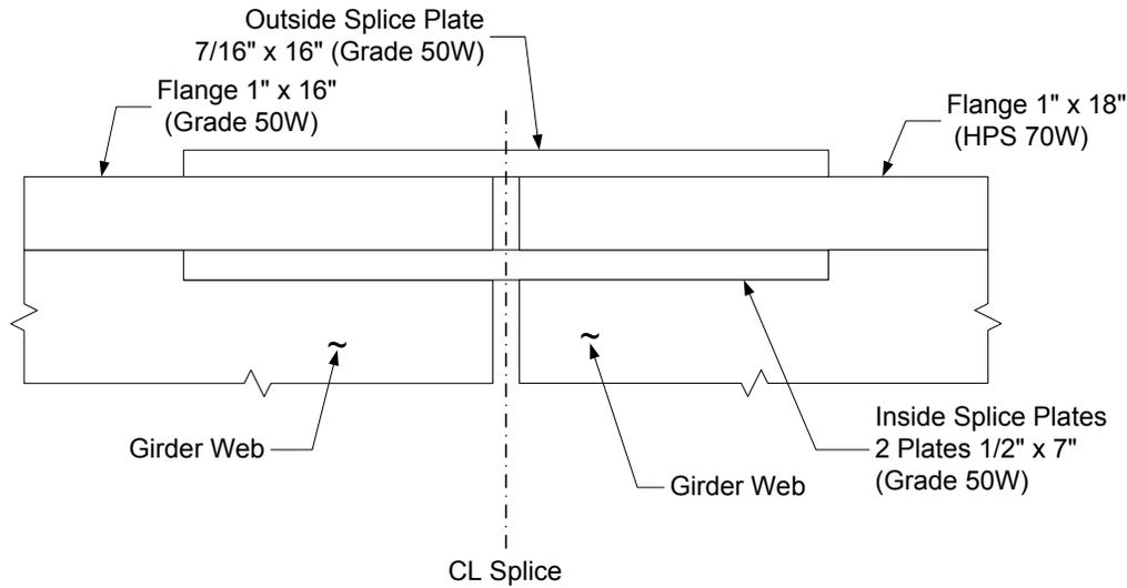
**Figure 6.6.5.2.3.4-5 Example Top Flange Splice**
