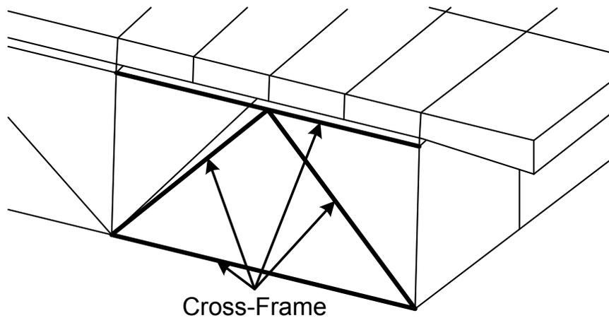
**Figure 4.5.3.3.2.3.4-2 Truss Elements Used to Model a Cross-Frame**
