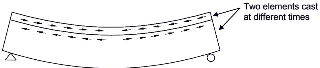
**Figure 5.6.4.2-4 Interdependent (Composite) Behavior between Precast Girder and Deck**
