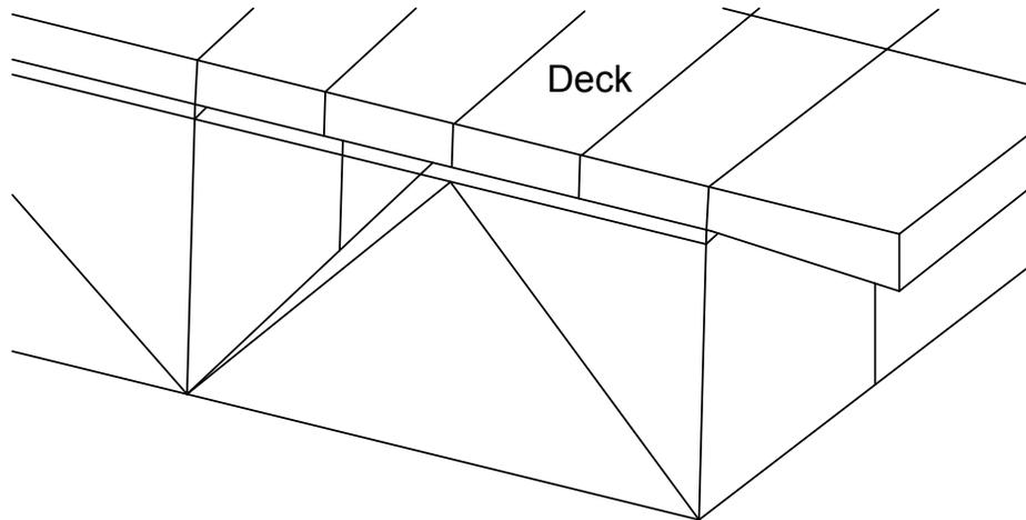
**Figure 4.5.3.3.2.3.3-2 Solid Elements Used to Model the Concrete Deck**
