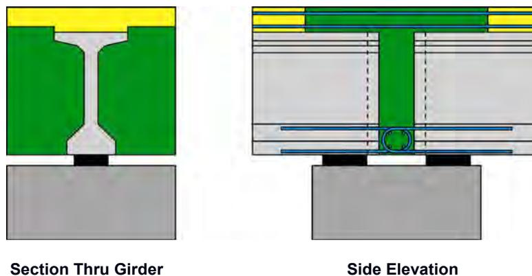
**Figure 5.10.3.2.2-1 Full-Depth Reinforced Concrete Joint**
