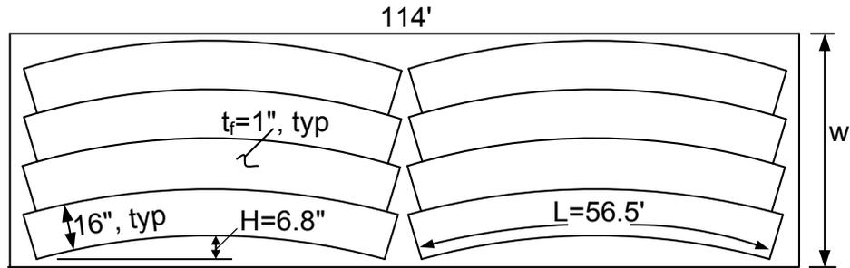
Assume 8 half-length flanges are taken from a single plate – flanges to be spliced
