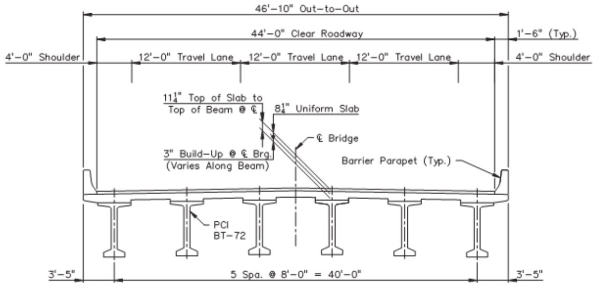
Figure 5.4.2-5 Typical AASHTO Bulb-Tee Girder Bridge
