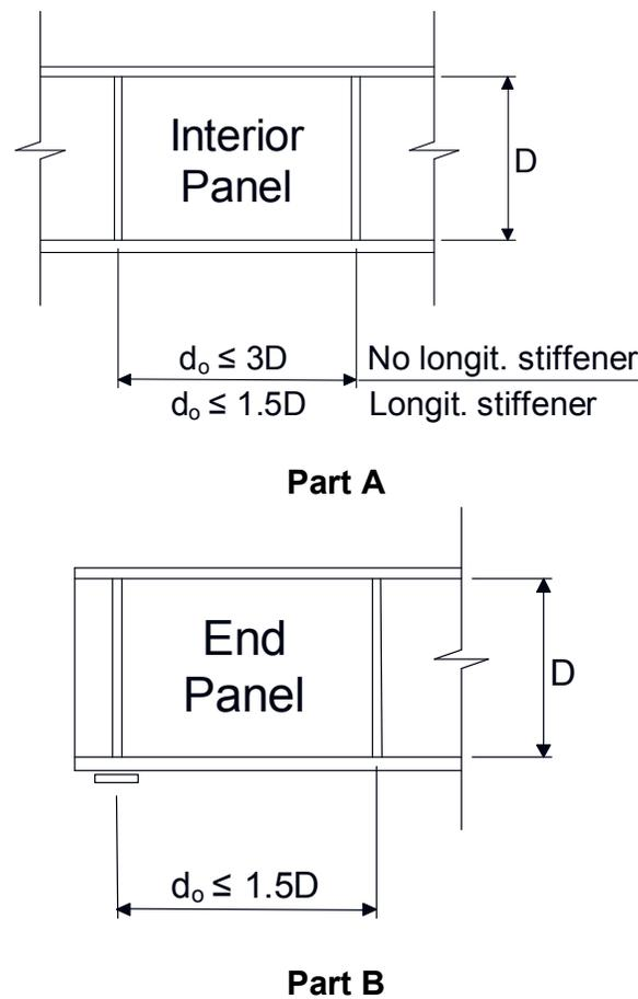
**Figure 6.5.7.1-2 Maximum Transverse Stiffener Spacing Requirements**
