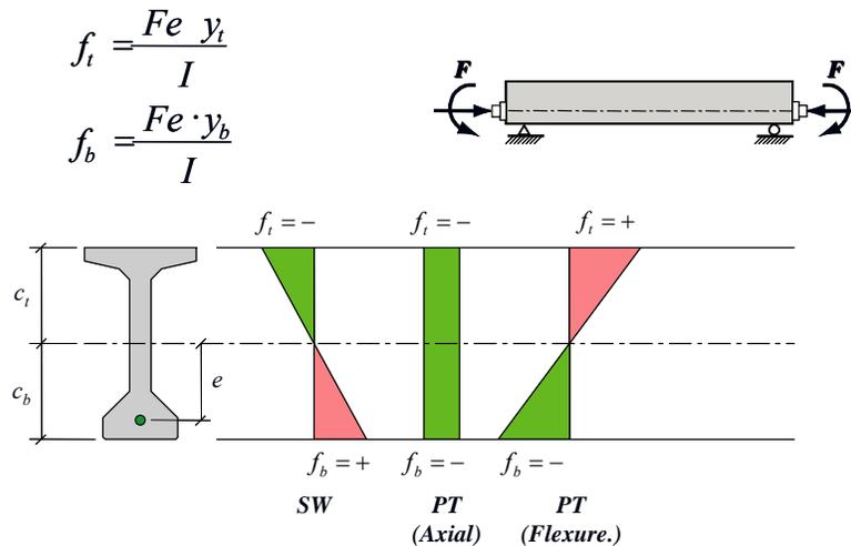
**Figure 5.3.3-3 Self Weight, Axial and Eccentric Prestress Stresses**
