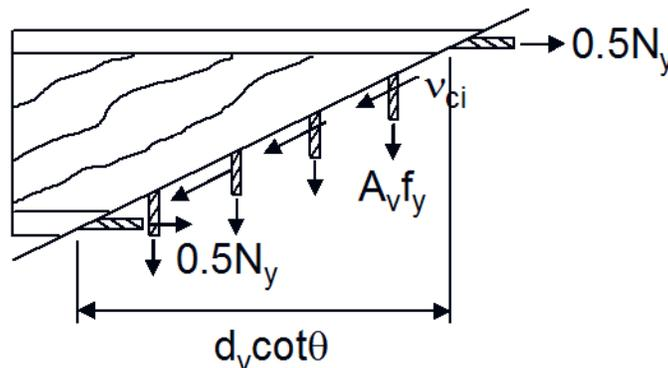
**Figure 5.6.1.1.5-1 Force Transfer Across a Crack (Local Stresses)**
