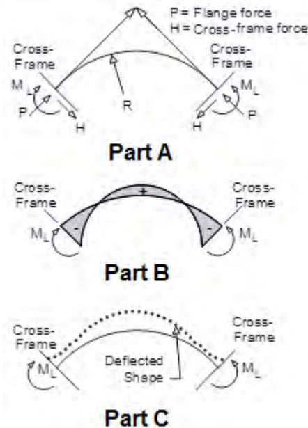
**Figure 6.4.9.5.1.2-2 Curved I-Girder Compression Flange In-Between Two Cross-Frames**
