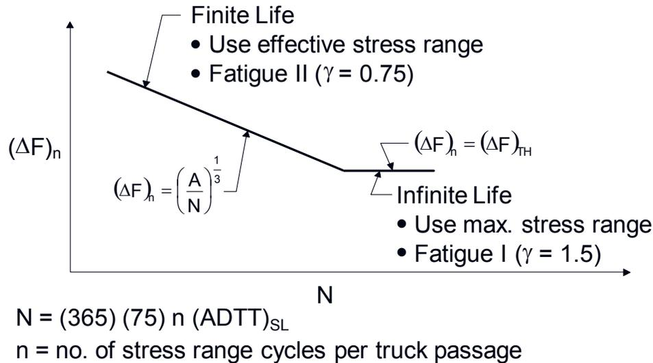
**Figure 6.5.5.2.2.1.5-2 Nominal Fatigue Resistance,  $(\Delta F)_n$**
