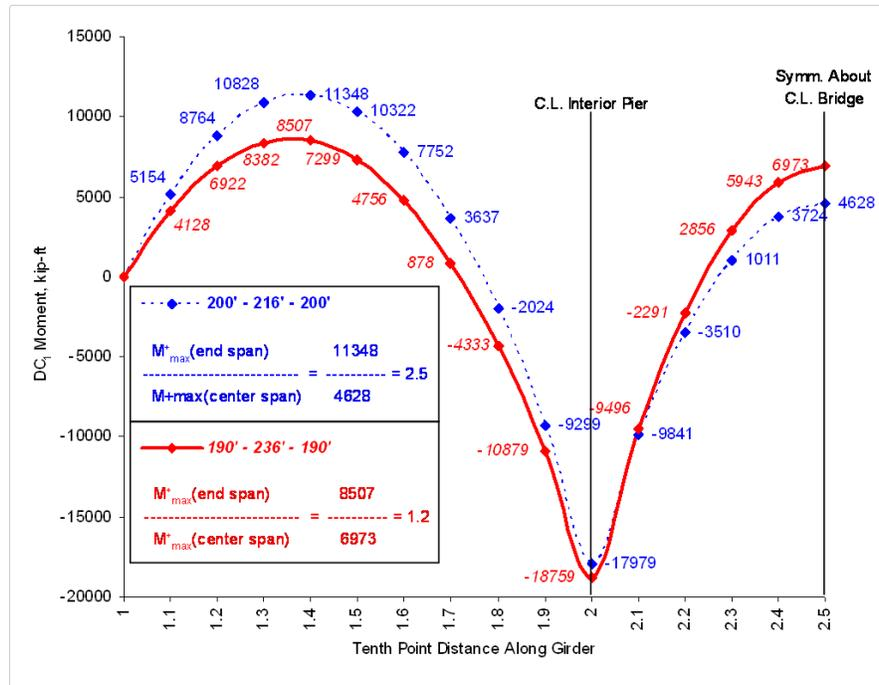
**Figure 6.3.2.3.1-2 Component Dead Load ( $DC_1$ ) Moments for Different Span Arrangements**
