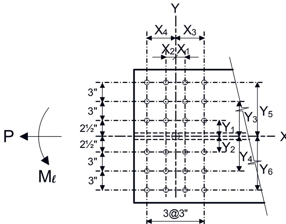
**Figure 6.6.5.2.2.4-3 Sample Bottom Flange Bolt Pattern for Computation of  $I_p$**
