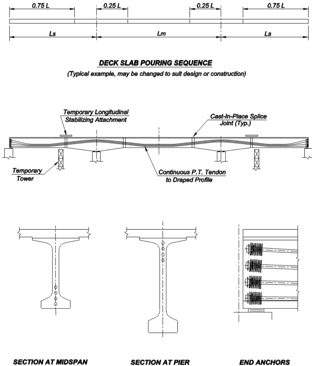
Figure 5.10.4.3.3-1 Post-Tensioning for Three-Span Haunched Girder Unit
