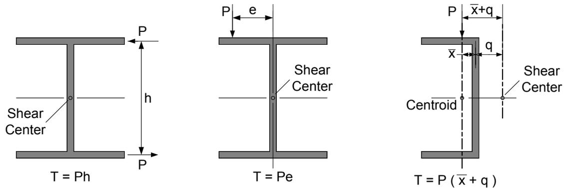
**Figure 6.4.8.1-1 Torsional Loadings on an I-Section and a Channel**
