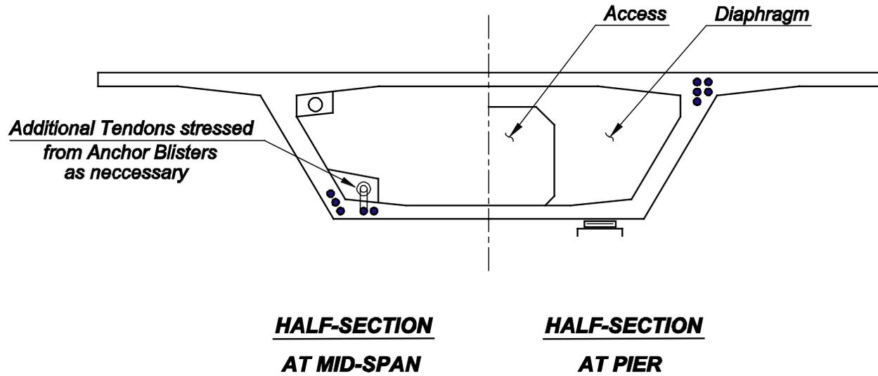
**Figure 5.4.2-7 Single-Cell Precast Segmental Box Girder Bridge**
