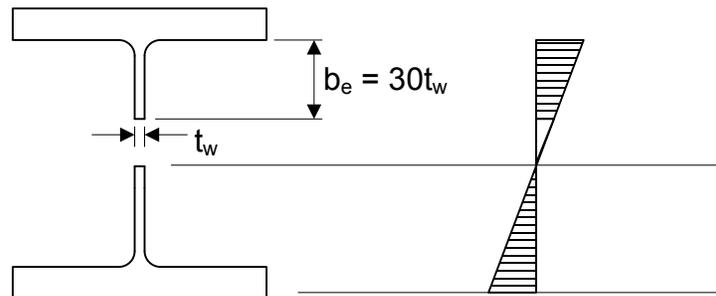
**Figure 6.4.5.6-2 Effective Cross-Section Assumed in the Derivation of  $R_b$**
