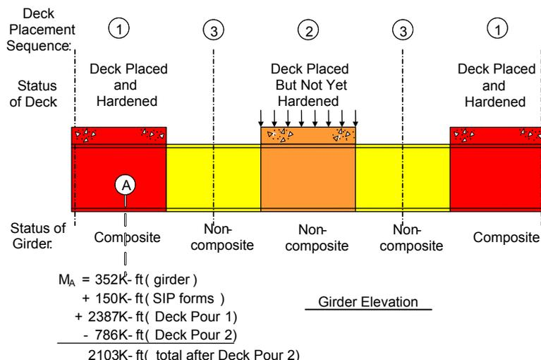
**Figure 6.5.3.3.4-5 Sample Deck Placement Analysis (Cast 2)**
