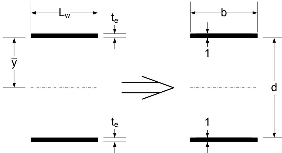
**Figure 6.6.4.3.7.2.3-2 Weld Configuration Considered as Lines of Unit Thickness**
