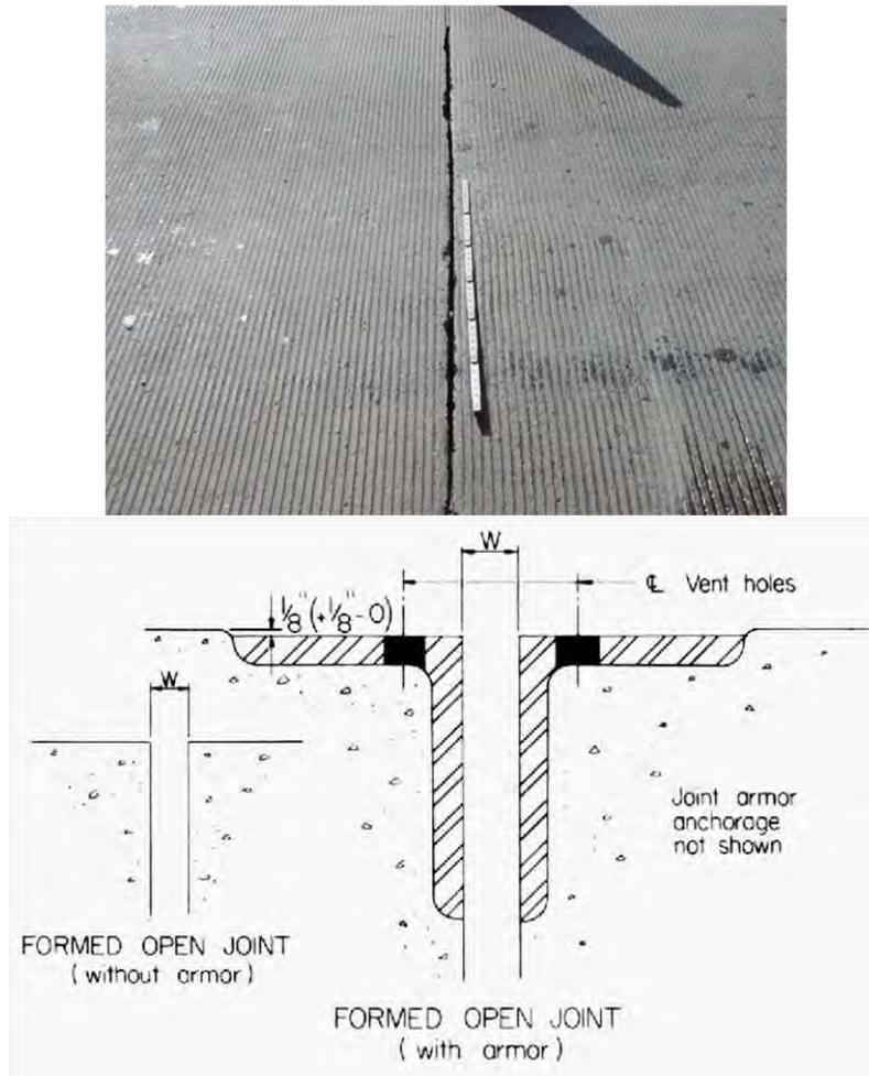
**Figure 8.3.2.1-1 Butt Joint**
