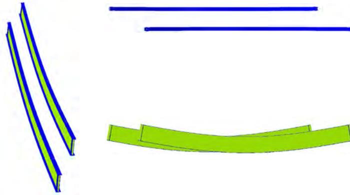
**Figure 6.4.9.5.1.1-1 Magnified Girder Vertical Deflections for Two Simple-Span I-Girders on Parallel Skewed Supports Subjected to Steel Dead Load Prior to Interconnecting the Cross-Frames**
