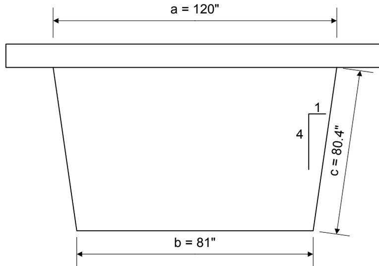
**Figure 6.5.5.2.2.3.2-12 Example Box-Girder Cross-Section**
