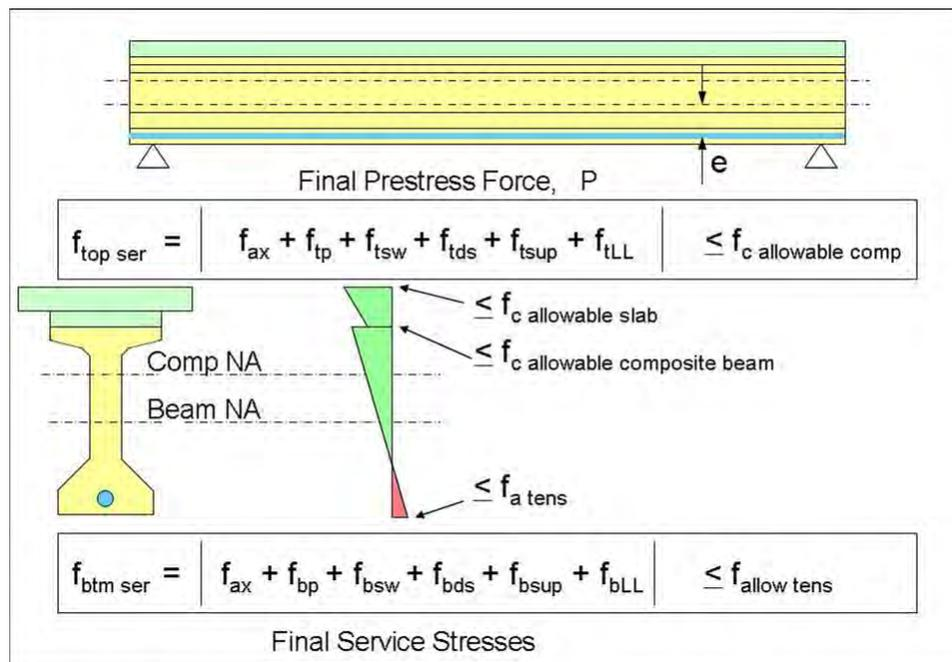
**Figure 5.5.3.4.3-2 Final Stresses in Service After All Prestress Losses**
