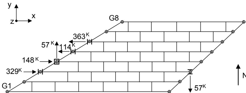
**Figure 6.3.3.3.7-7 Horizontal Bearing Reactions (X-Y Plane) due to Thermal Expansion – Bearing Constraints Orthogonal to Girders**
