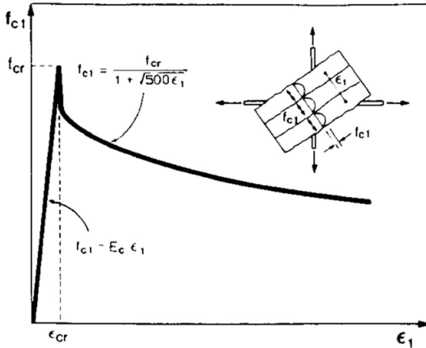
**Figure 5.6.1.1.3-1 Average Tensile Stress-Strain Relationship in Reinforced Concrete Section Before and After Cracking**
