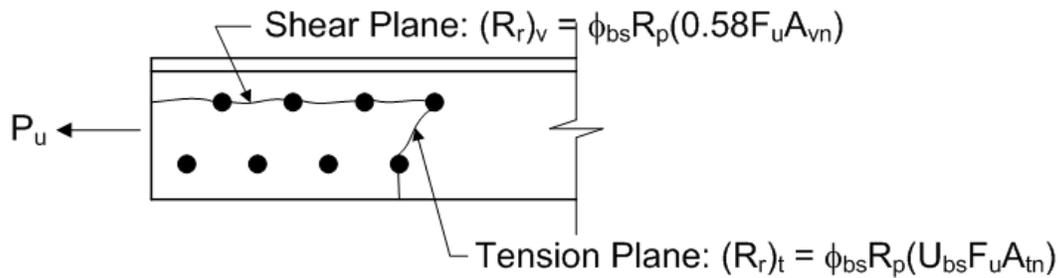
**Figure 6.6.3.3.2.5-2 Factored Resistance of Shear and Tension Planes**
