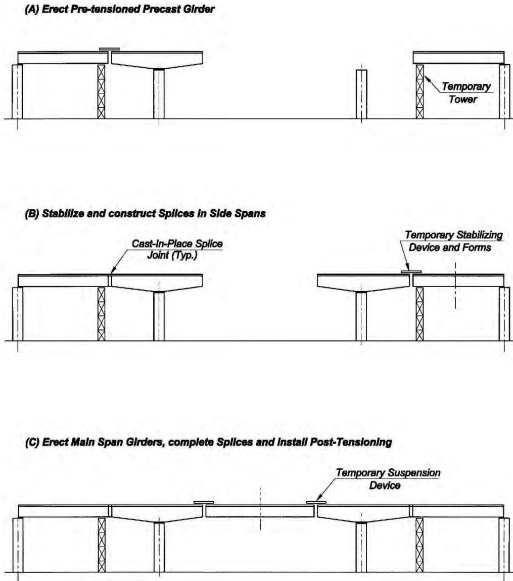
**Figure 5.10.4.3.3-2 Erection of Precast Girders for Three-Span Unit**
