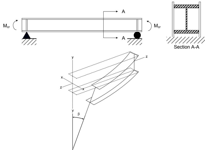
**Figure 6.5.6.2.2.2-1 Lateral-Torsional Buckling of a Doubly Symmetric I-Section Member**
