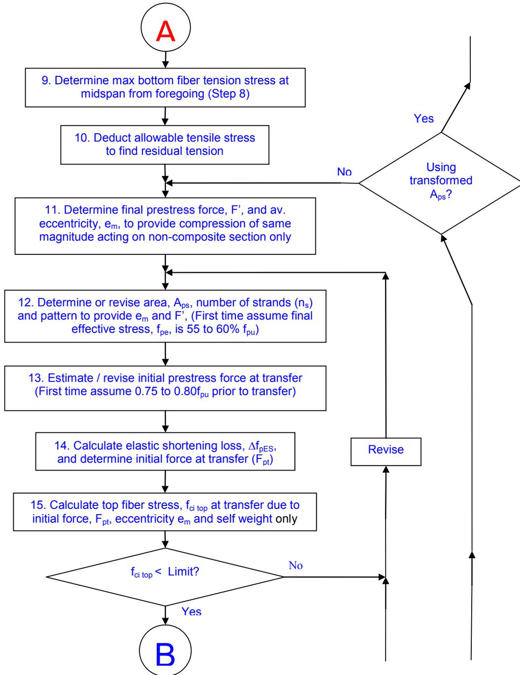
Figure 5.5.3.4.3-4 Flowchart for Determination of Prestress Force and Strand Pattern, Part (b)
