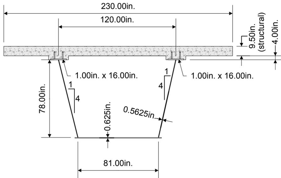
**Figure 6.5.6.3.2.3-1 Example Composite Tub Section in a Region of Positive Flexure**
