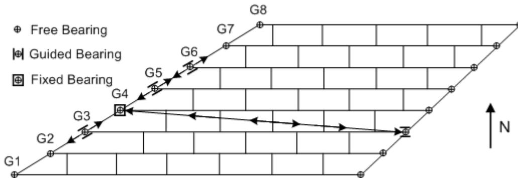
**Figure 6.3.3.3.7-8 Guided Bearings All Guided Toward Fixed Bearing at West End of G4**
