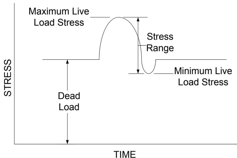
**Figure 6.5.5.2.2.1.1-1 Components of a Stress Cycle**
