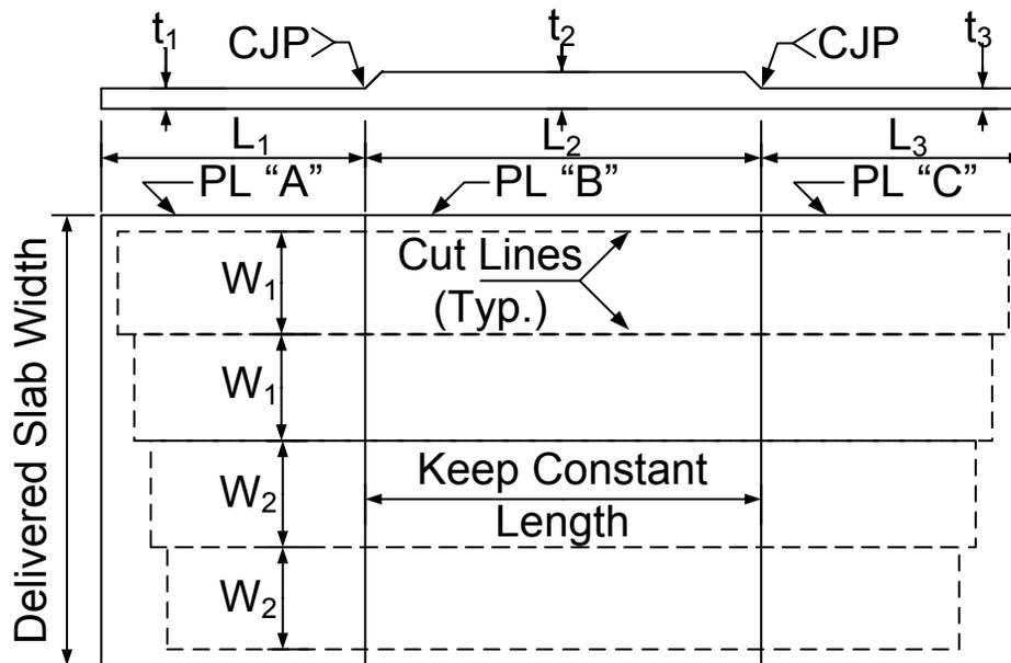
**Figure 6.3.4.4.5-5 Slab Welding – Nesting of Straight Flange Plates for a Pier Section**
