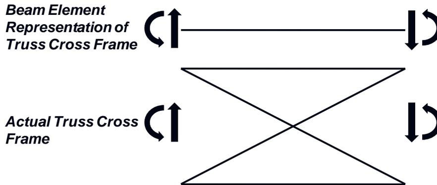
**Figure 4.5.3.2.2.5.3-5 Global Forces Acting on the Beam Element Representation of the Truss-Type Cross-Frame and the Actual Truss-Type Cross-Frame**
