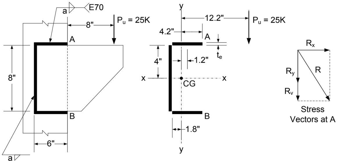
**Figure 6.6.4.3.7.2.3-4 Eccentrically Loaded Fillet-Welded Bracket Example 1**
