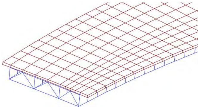
**Figure 6.4.9.4-2 3D Analysis Model of Curved I-Girder Bridge with Deck**
