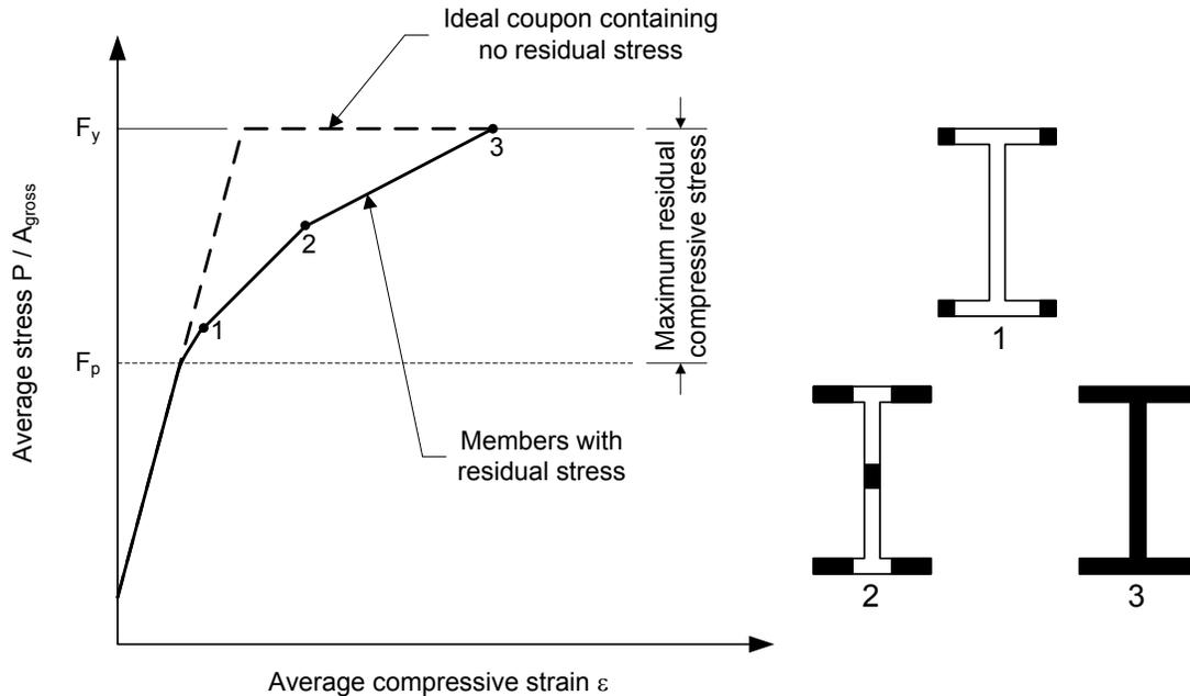
**Figure 6.6.3.4.2.3.2-2 Residual Stress Effects on the Average Stress-Strain Curve for a Rolled Shape**
