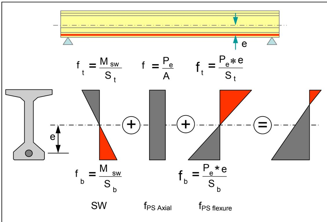
Figure 5.5.3.4.1-2 Non-Composite Section under an Assumed Final Prestress
