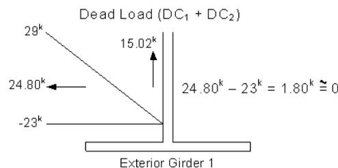
**Figure 6.6.4.4-2 Equilibrium Check for  $DC_1 + DC_2$  Cross-Frame Horizontal Forces at the Bottom of an Exterior Girder**
