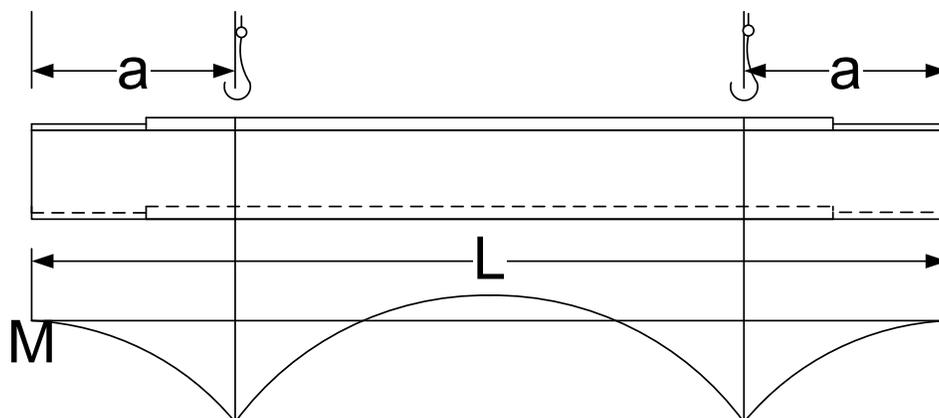
**Figure 6.3.2.4.3.2-2 Moment Diagram Due to Lifting**
