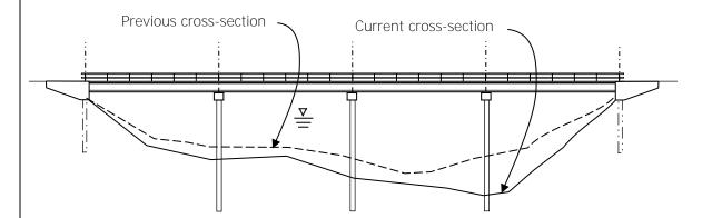
Figure 156. Elevation view showing current cross-section and previous cross-section for a bridge over water.
