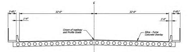
Figure 158. Cross-section view of RC voided slab spans one to four for Bridge Number 15558X. (Source: Missouri DOT)
