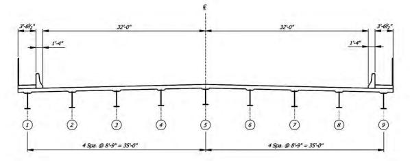
Figure 159. Cross-section view, looking north, indicating steel beam numbering in spans five to seven for Bridge Number 15558X. (Source: Missouri DOT)
