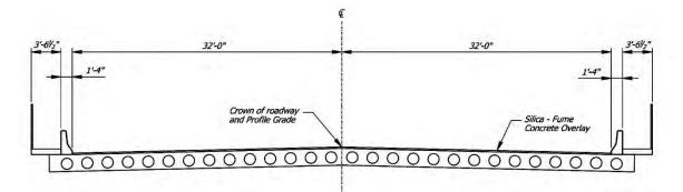
Figure 9. Cross-section view for Bridge Number 15558X, spans one through four. (Source: Missouri DOT)
