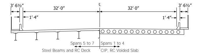
Figure 5. Typical section views for Bridge Number 15558X.
