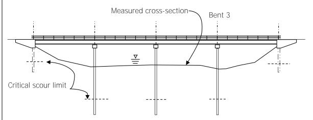
Figure 154. Elevation view showing scour elevations and stream cross-section for a bridge.
