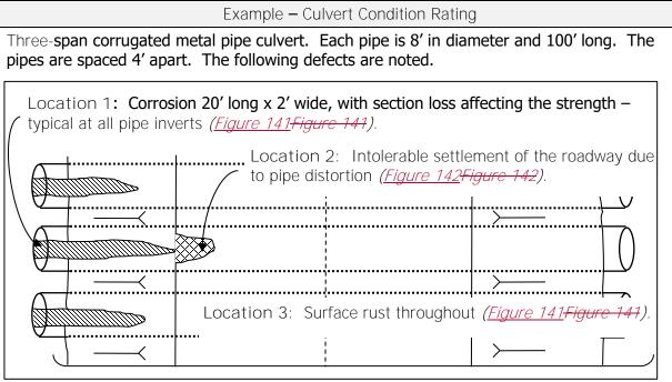
Figure 140. Plan view of pipe culvert showing defects.
