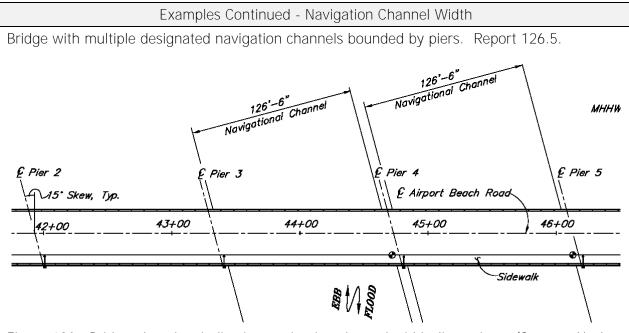
Figure 120. Bridge plan view indicating navigation channel width dimensions. (Source: Alaska DOT)
