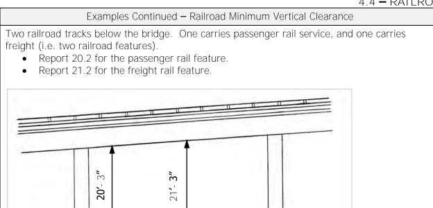
Figure 110. Bridge elevation view with one passenger rail and one freight rail track below the bridge.
