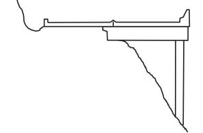
Figure 75. Cross-section view of a sidehill bridge.
