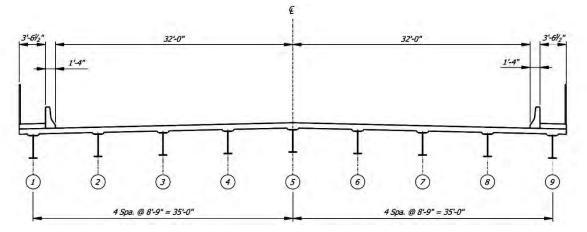
Figure 10. Cross-section view for Bridge Number 15558X, spans five through seven. (Source: Missouri DOT)
