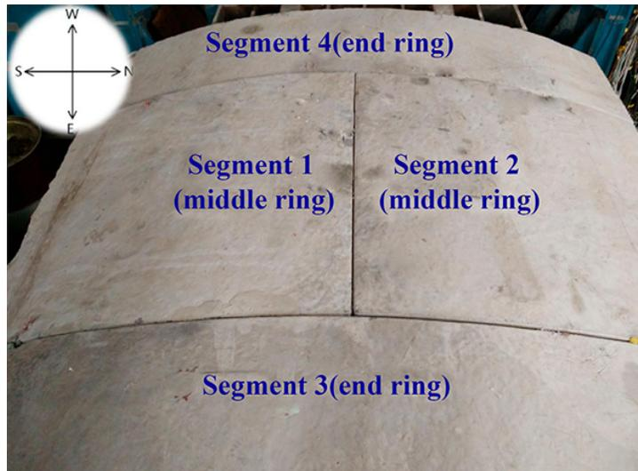
**Figure 1-14: A full scale staggered joint two-segment three-ring configuration**
