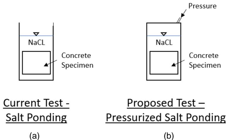
**Figure 1-21: (a) Current salt ponding test and (b) proposed pressurized salt ponding test.**
