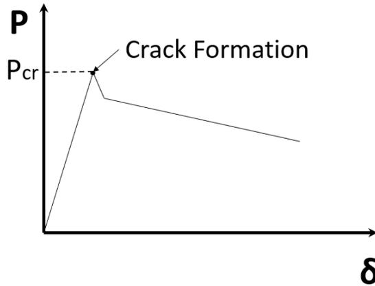
**Figure 1-24: Typical Load vs. Deflection flexural beam plot**
