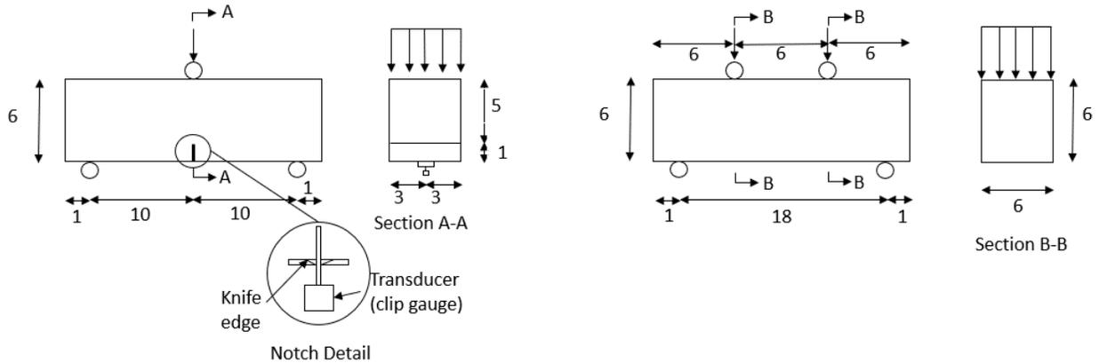
**Figure 1-23: EN 14651 (left) and ASTM C1609 (right) flexural beam tests.**
