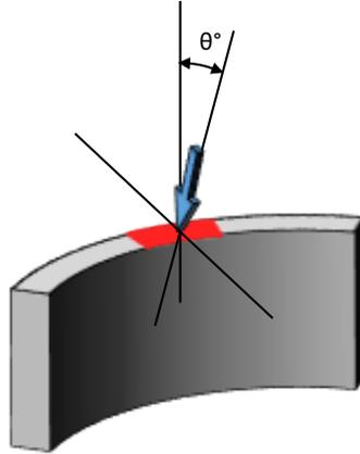
**Figure 1-8: Conceptual model for thrust loading eccentricity.**
