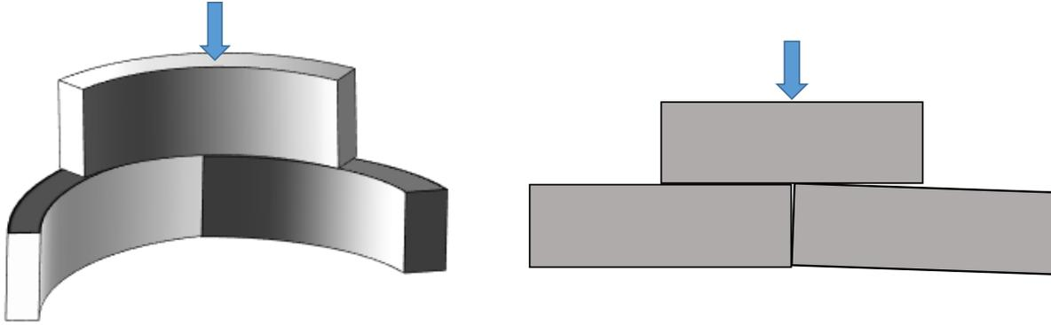
**Figure 1-10: Conceptual continuum modeling layout for the investigation of staggered joint tolerance.**
