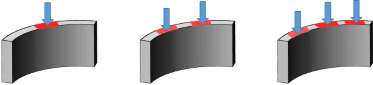
**Figure 1-7: Conceptual layout for single segment bursting stress FE analysis.**
