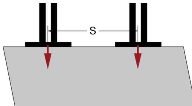
**Figure 1-18: Schematic of a two-jack loading configuration with variable jack spacing. Shear loading can be included.**
