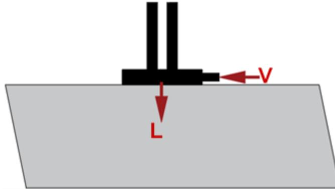
**Figure 1-17: Single vertical actuator with a laterally oriented actuator to simulate the torque-induced shearing load applied to segments.**
