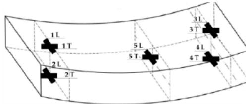
**Figure 1-15: Strain gauge layout used in the Metro Line 6 of Naples**
