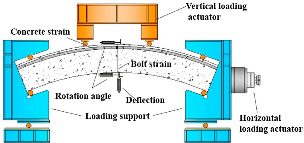
**Figure 1-11: Two segment test configuration for joint behavior testing.**
