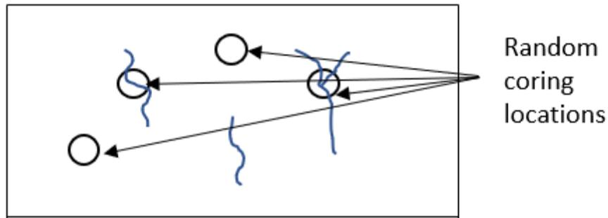
**Figure 1-22: Cores with and without micro-cracking to be tested.**
