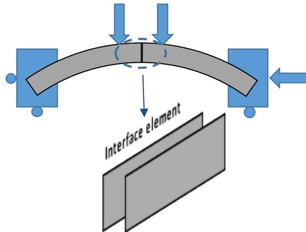
**Figure 1-4: Conceptual continuum modeling layout for the investigation of radial joints.**
