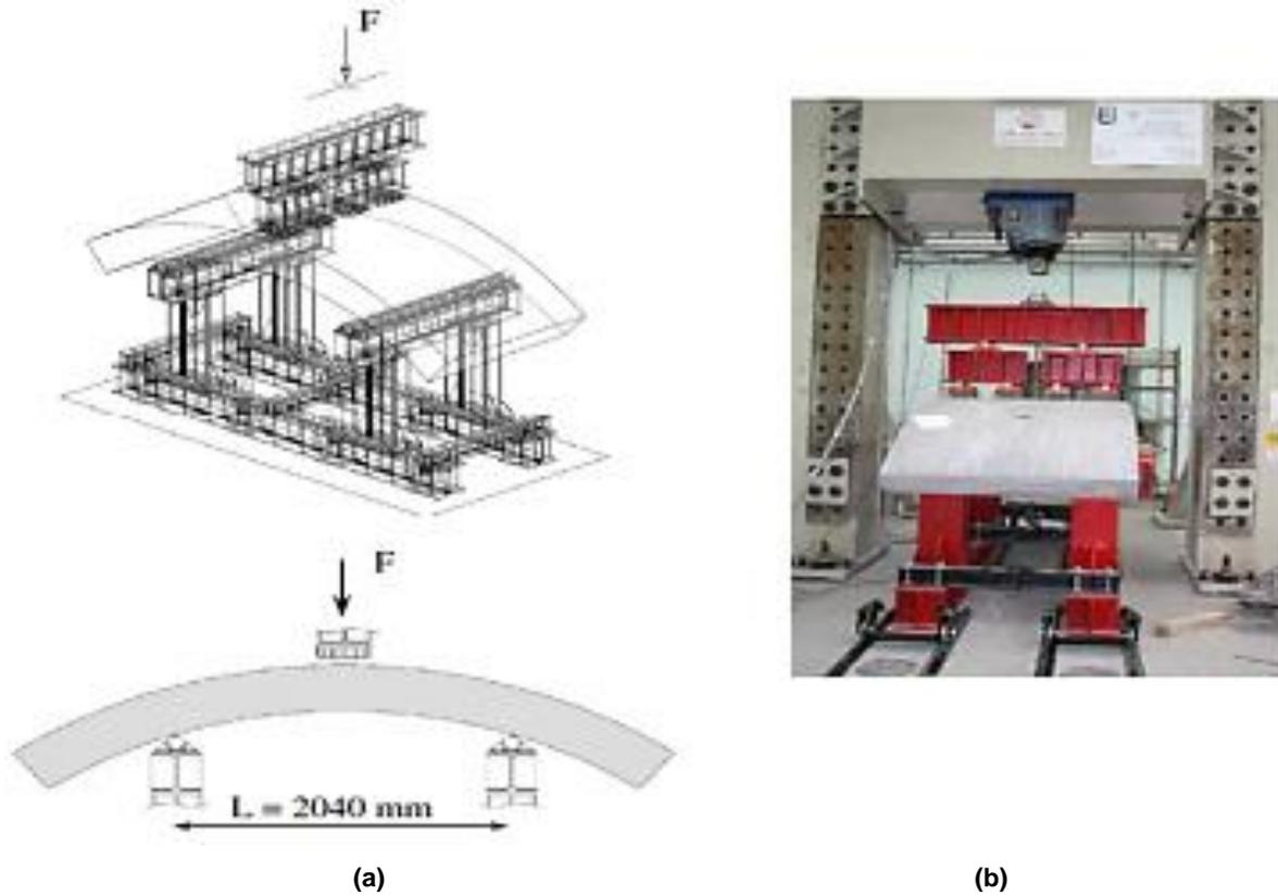
**Figure 1-25: (a) Schematic of Flexure segment test (b) Side view of flexural test.**
