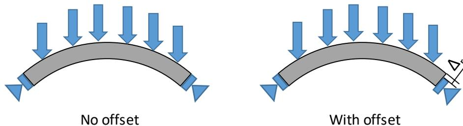
**Figure 1-9: Layout for single segment radial tolerance analysis.**
