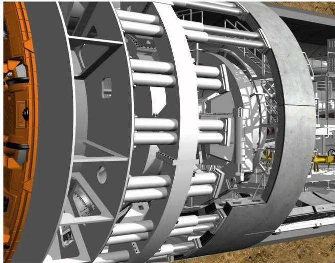
**Figure 1-16: Illustration of TBM thrust jacking loads applied to ring end/bearing area of most recently installed segments.**
