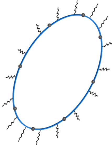
**Figure 1-1: Single ring bedded beam model.**
