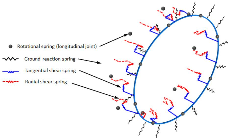
**Figure 1-2: Double ring bedded beam model.**
