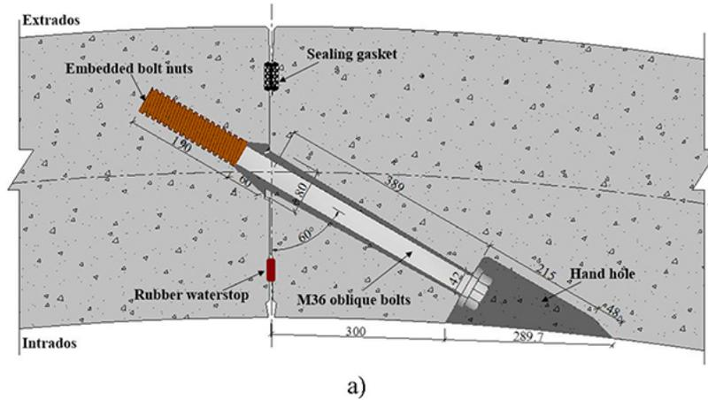
**Figure 1-12: Bolt passing through the segment neutral axis.**
