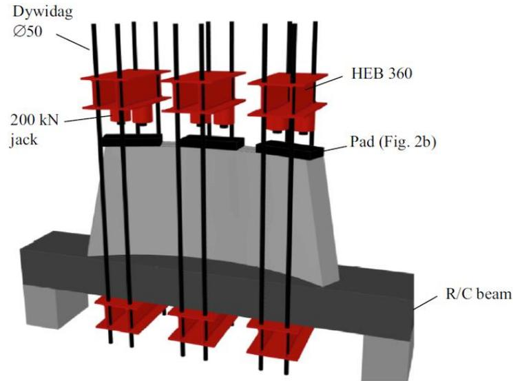
**Figure 1-19: Schematic of a three-jack loading configuration with variable jack spacing. Shear loading can be included.**
