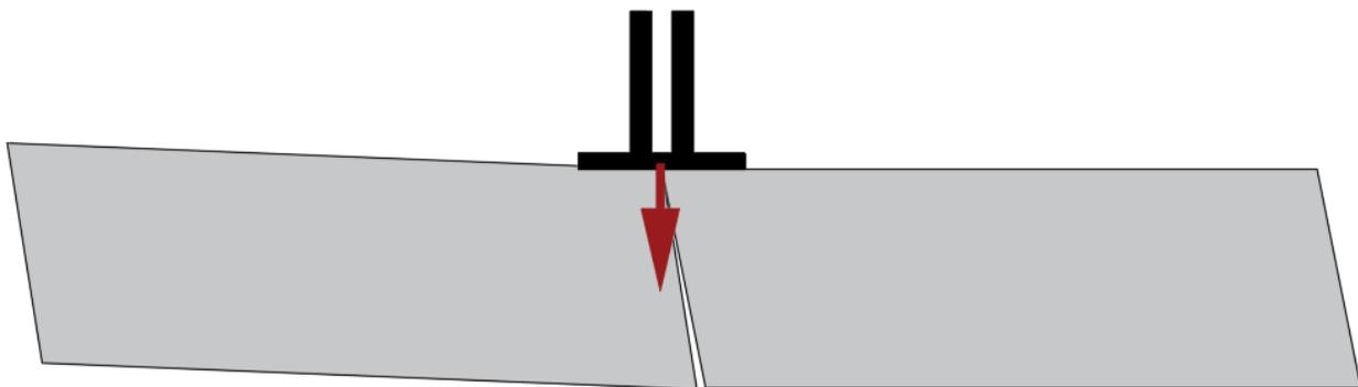
**Figure 1-20: Schematic of a single jack loading over the longitudinal joint with reaction surface inaccuracy. Shear loading can be included.**
