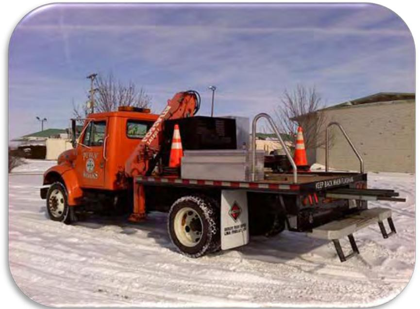
the bed of the truck (the bottom step is attached using recycled rubber). This way, if the steps hit anything they will bend up out of the way. At bed height are stainless steel hand rails on each side that were made from a recycled swimming pool ladder. The bed has two steel posts mounted to it that hold cones and keep them neatly stored on the bed. Built into the rear of the bed is a storage area for carrying posts up to 12' in length.
