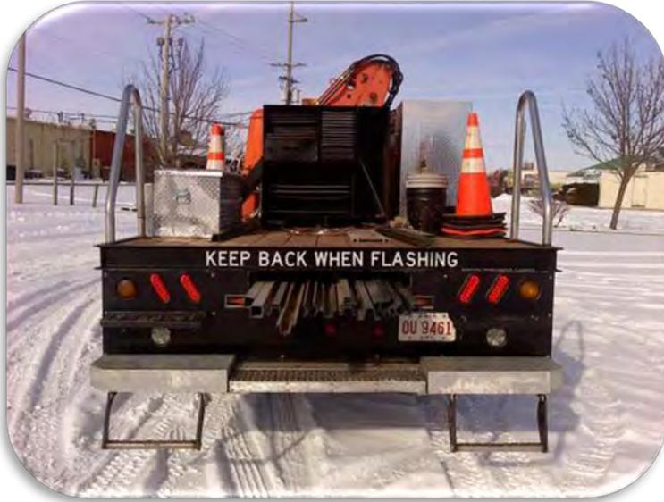
Even with all this equipment, a very large area for two people to work at the same time or for storing work zone signs/a hundred or more cones still remains. Also, on the end of the truck is a directional arrow used when setting up work zones or during other unexpected jobs, accidents, or emergencies. The truck is fitted with an overhead strobe light along with strobes at each corner of the truck, and the bed was updated with all new LED lights.
