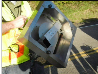
Figure 6: Circular Track Meter CTM Base Source: National Park Service
