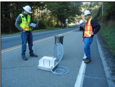
Figure 7: Dynamic Friction Tester Test Source: National Park Service
