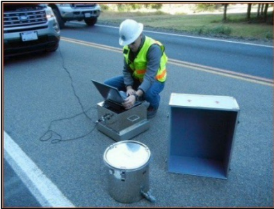
Figure 5: CTM Circular Track Meter Test Source: National Park Service
