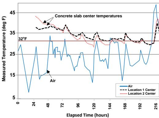
Figure 3. Ambient air and internal concrete temperature measurements for the sidewalk replacement at the Rochester Ranger Station, Rochester, VT.
