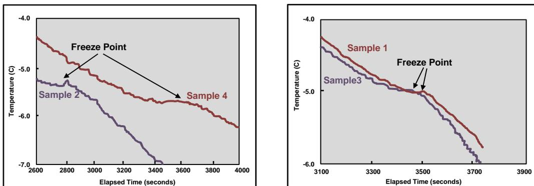
Figure 6. Initial freezing point temperature measurements for the Rochester Ranger Station sidewalk repair (left) and Saint Croix sign base (right).
