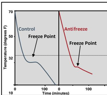
*Figure 1. Comparison of initial freezing point temperature for ordinary and antifreeze concrete mixtures (Barna and Korhonen 2012).*
