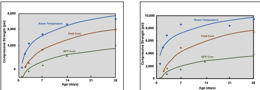
Figure 8. Compressive strength gain with age at room temperature and during field curing conditions for the Rochester Ranger Station sidewalk replacement (left) and Saint Croix Historic Site sign base replacement (right). Included is a comparison of strength gain for normal concrete cured at continuous 40°F (based on ACI 306).
