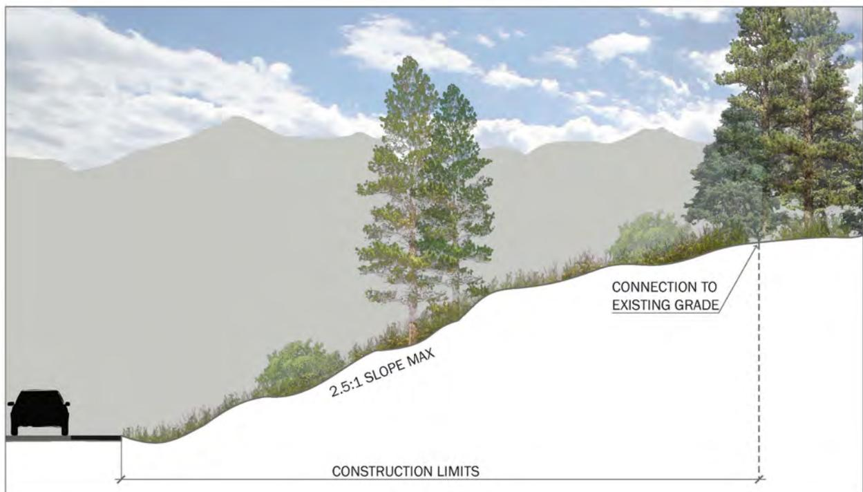
*Figure 3-20: Slope transitions*
