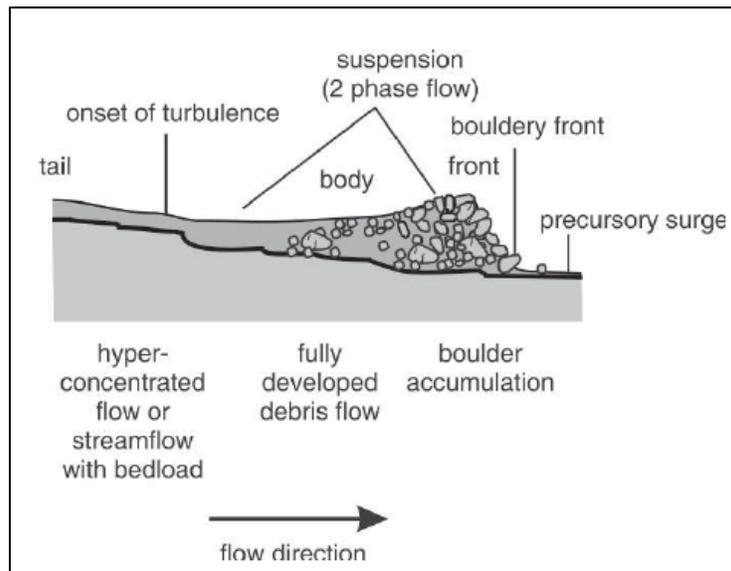
Figure 3. Depiction of Debris Flow Structure
