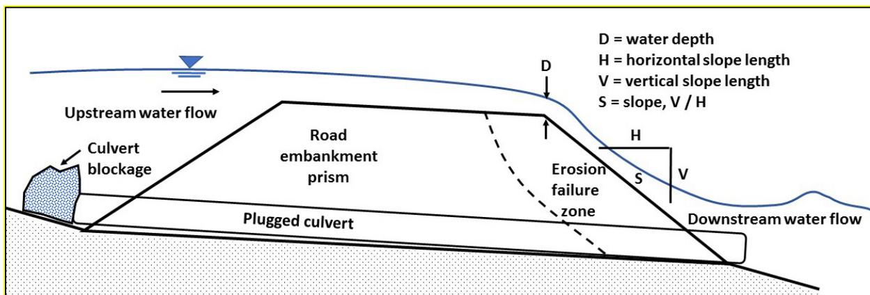
Figure 1. Road embankment with plugged culvert, failing due to overtopping (Provided by USFS)
