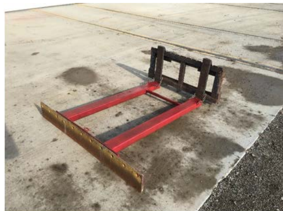
Figure 2. Scraper with the Bull Blade. Gunnison County Public Works Department
