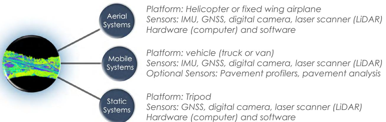
Figure 3: LiDAR Surveys Data Acquisition Platforms
