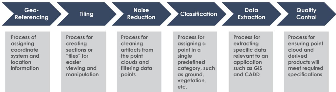
Figure 4: Basic Workflow for Post-Processing Point Clouds
