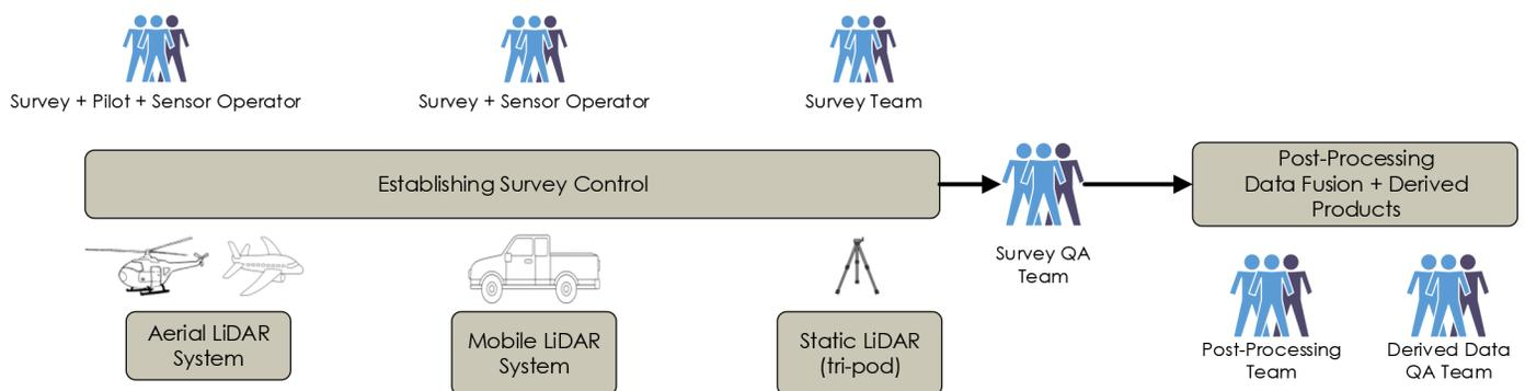
Figure 7: LiDAR Survey Data Acquisition Workflow
