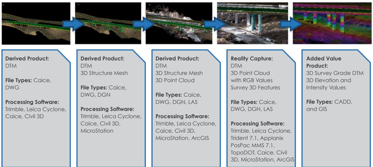
**Figure 2: Caltrans District 4 Process for DTM Creation<sup>4</sup>**
