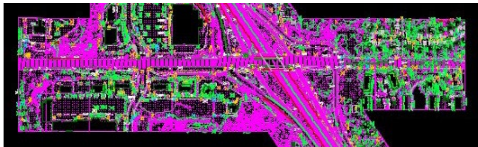
Figure 1. Helicopter LiDAR 1 Survey Dataset for Roadway 3D Design 2
