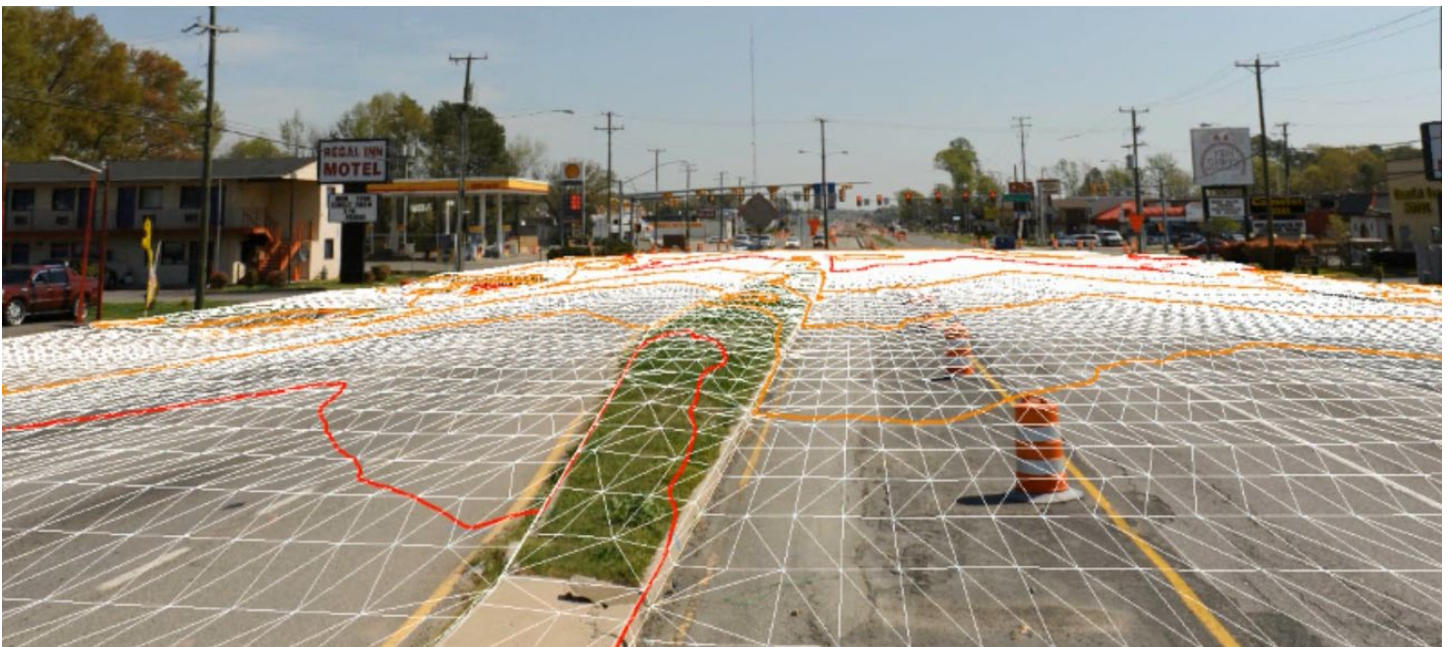
Figure 2. Triangulated Irregular Network (TIN) Model Superimposed on Project Site Photograph 3
