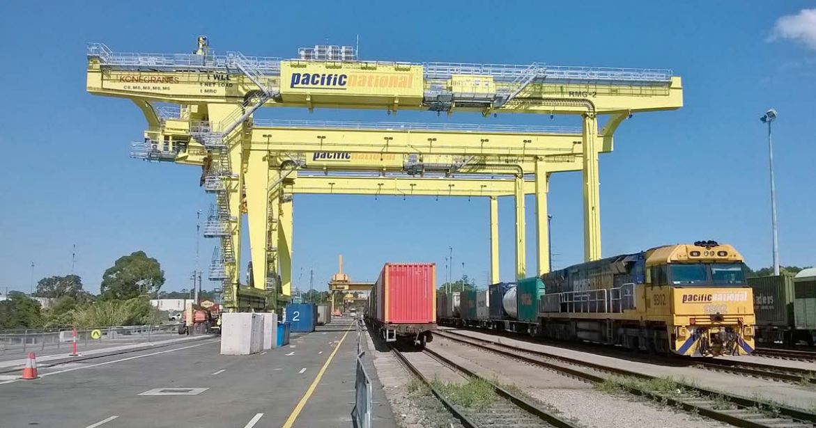
Figure 4: RMG Crane at Pacific National Sydney
