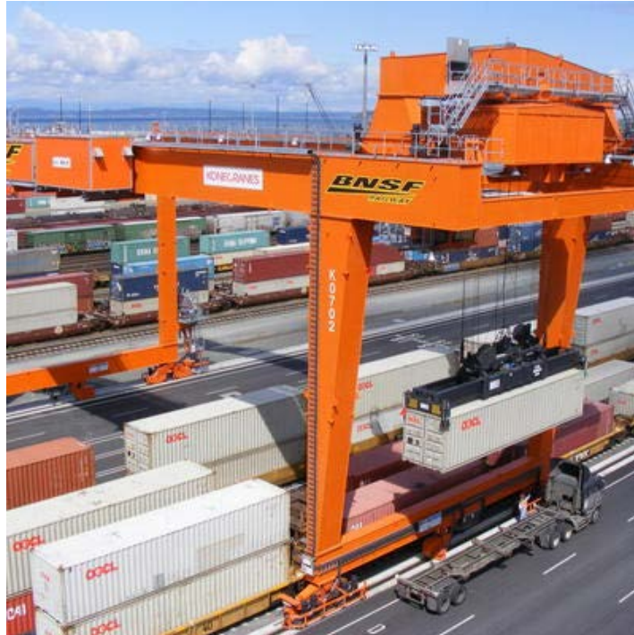
Figure 2: Konecranes of Finland RMG Crane at Burlington Northern Intermodal Facility
