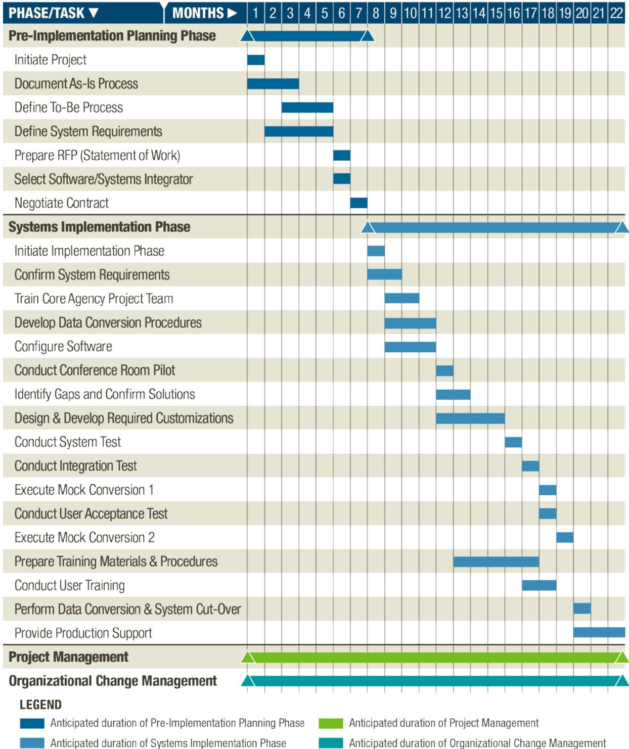
**Figure 17. Timeline. Potential schedule for implementation of a project construction management system.**
