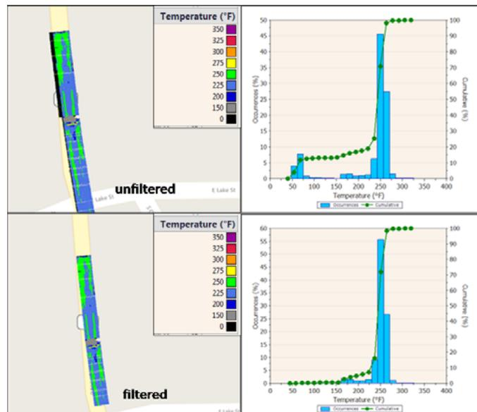
An example of temperature maps and histogram for unfiltered data and filtered data (Data Source: Undisclosed DOT data)
