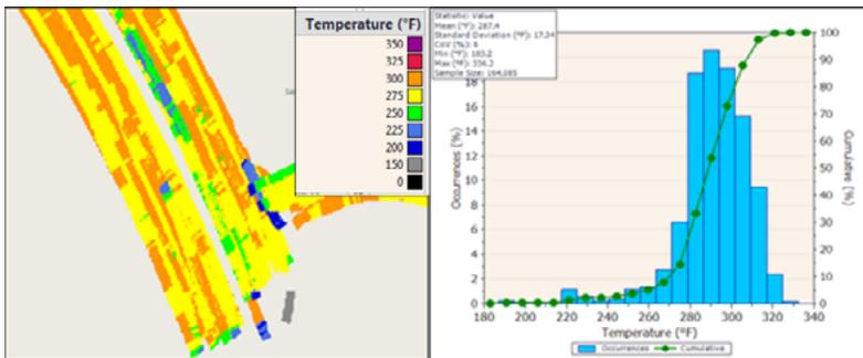
The IC temperature map using the Veta default color palette and associated histogram (Data Source: FHWA-TXDOT IC Retrofit Study - CA IC Rodeo – Hamm Day 1 – Asphalt Compaction)
