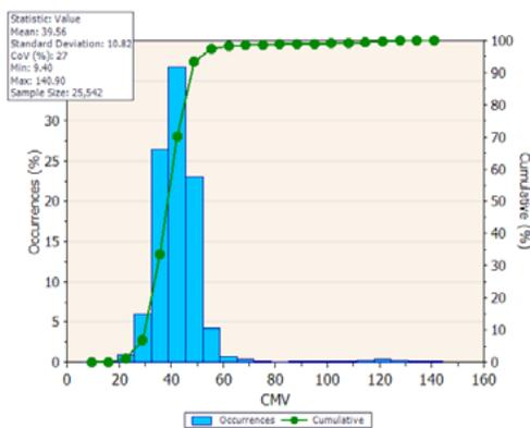
*The CAT histogram. (Data Source: TPF FHWA IC and Asphalt In-Place Density Study - ME IC Project - Caterpillar Day 1 - Asphalt Compaction)*
