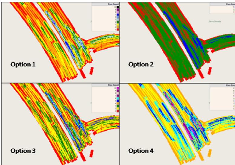
*Four different pass count maps for the same set of data but with different color palettes (Data Source: FHWA-TXDOT IC Retrofit Study - CA IC Rodeo - Hamm Day 1 - Asphalt Compaction)*
