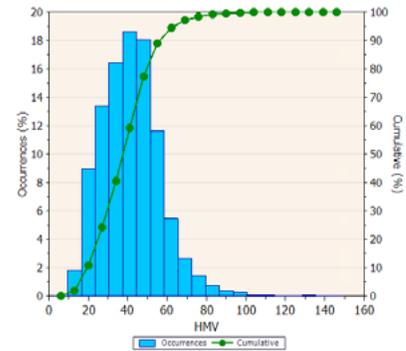
*An example of HMV histogram. (Data Source: FHWA-TXDOT IC Retrofit Study - CA IC Rodeo - Hamm Day 1 - Asphalt Compaction)*
