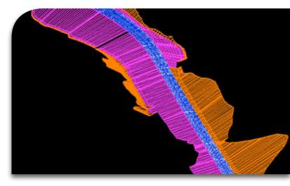
KYTC will develop and use 3D models for the proposed top surface and sub grade. The ultimate purpose of this process is to refine the way designers create the construction model so that it is more useful for contractors. The goals of this pilot project, as seen by KYTC, are to: 1) determine the best modeling practices for design, so better models can be provided to contractors in the future; and 2) set new policy to require better 3D models from design.
