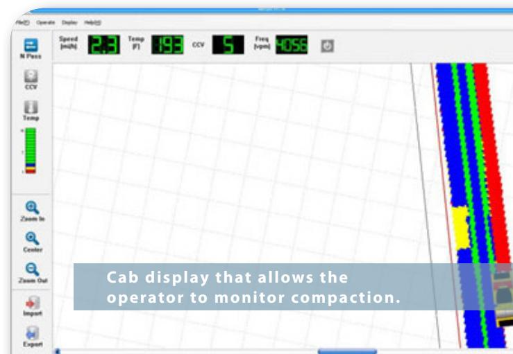
**Cab display that allows the operator to monitor compaction.**
