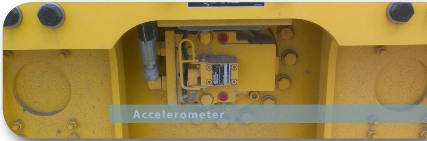
• **Processing:** The downward displacement, roller amplitude, frequency, and speed information are used to determine the level of compaction. As the roller moves, the system generates a continuous, real-time profile of the level of compaction achieved.
