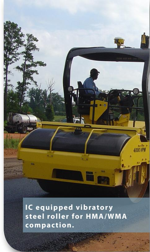
**IC equipped vibratory steel roller for HMA/WMA compaction.**
