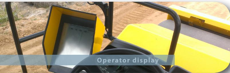
• **Display:** A video monitor in the cab of the roller provides a real time display of the compaction information, including a color-coded map that helps the operator identify the number of passes, stiffness, temperature (HWA/WMA), frequencies, amplitude, and roller speed.
