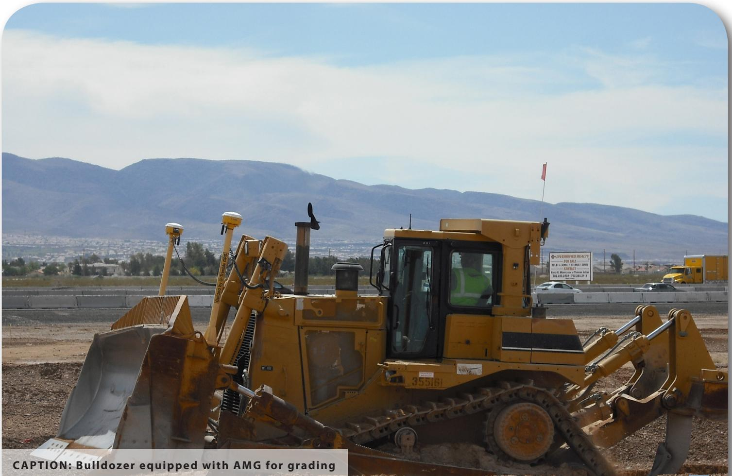
**CAPTION:** Bulldozer equipped with AMG for grading
