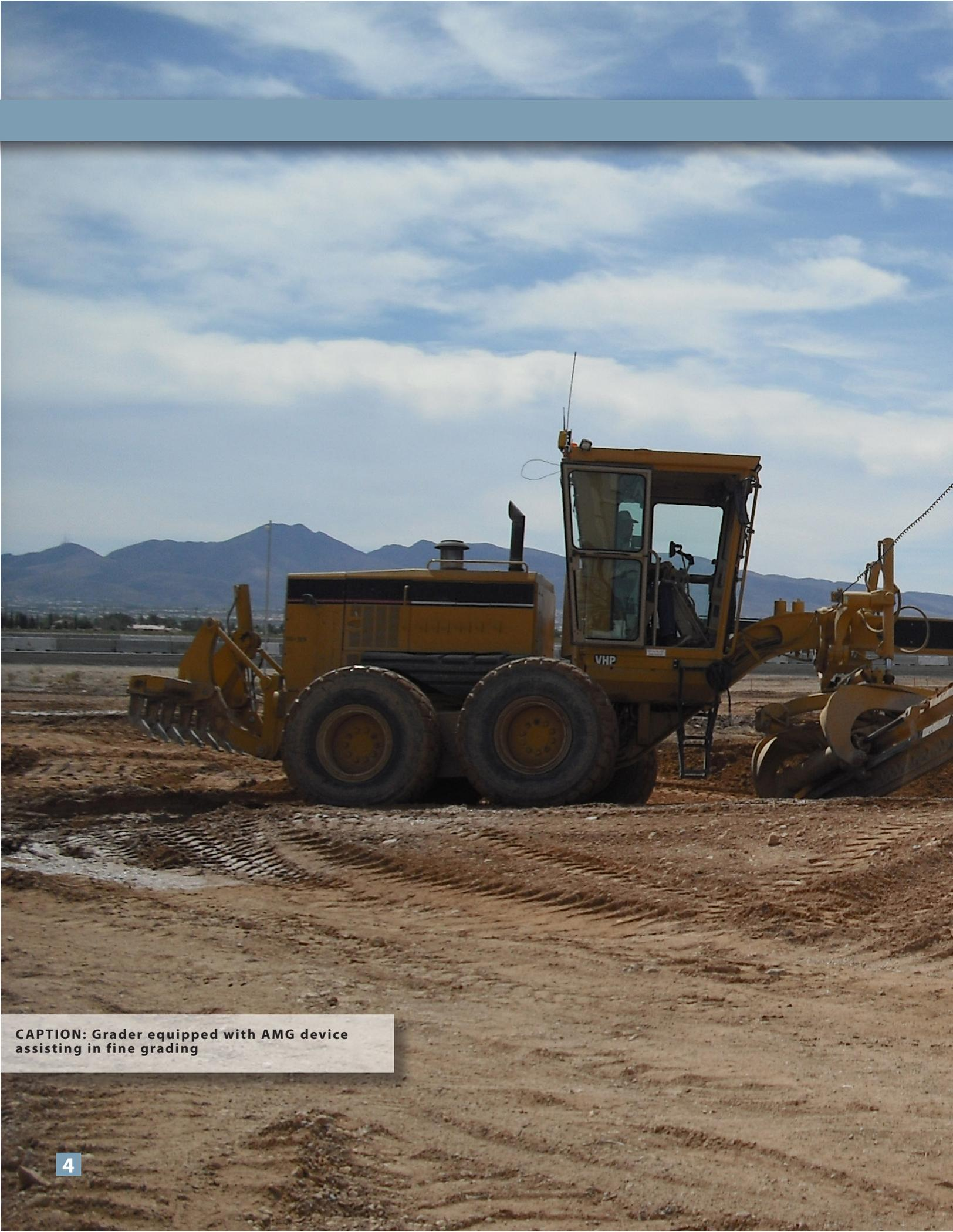
**CAPTION: Grader equipped with AMG device assisting in fine grading**
