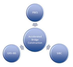
Three particular ABC technologies being promoted under EDC-2 are prefabricated bridge elements and systems, geosynthetic reinforced soil–integrated bridge systems, and slide-in bridge construction.
