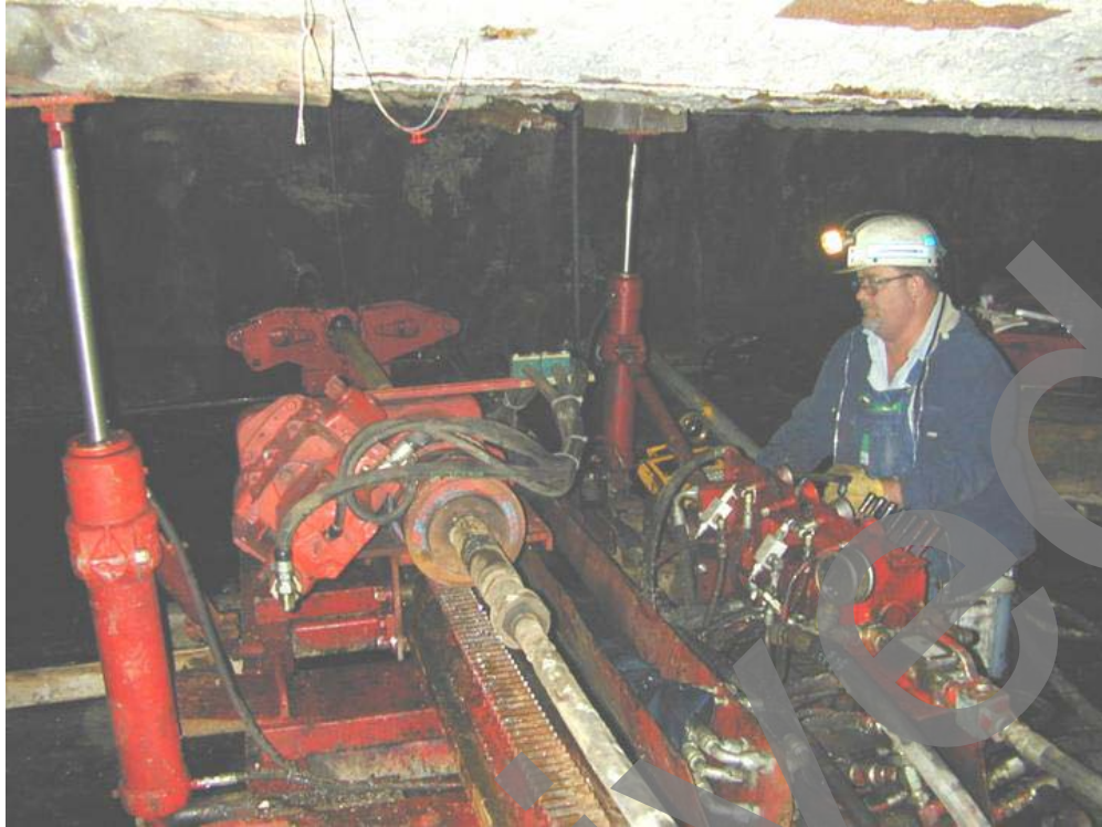
Figure 17. Photo of electrohydraulic drill rig that was used to drill the horizontal borehole.
