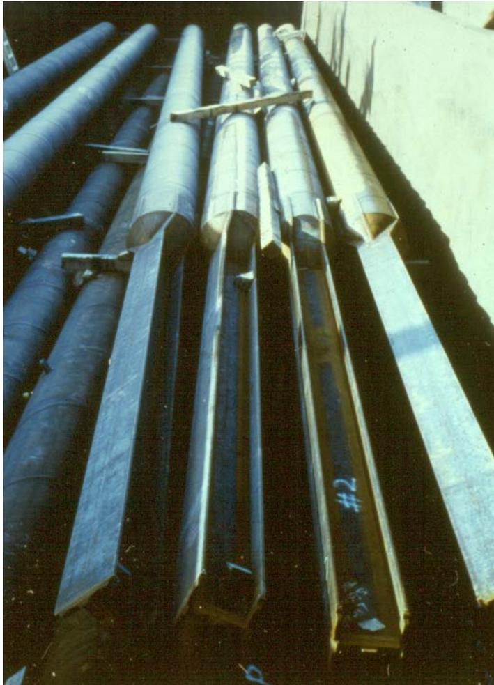
Figure 6-25 Steel pipe - H-pile composite piles.
