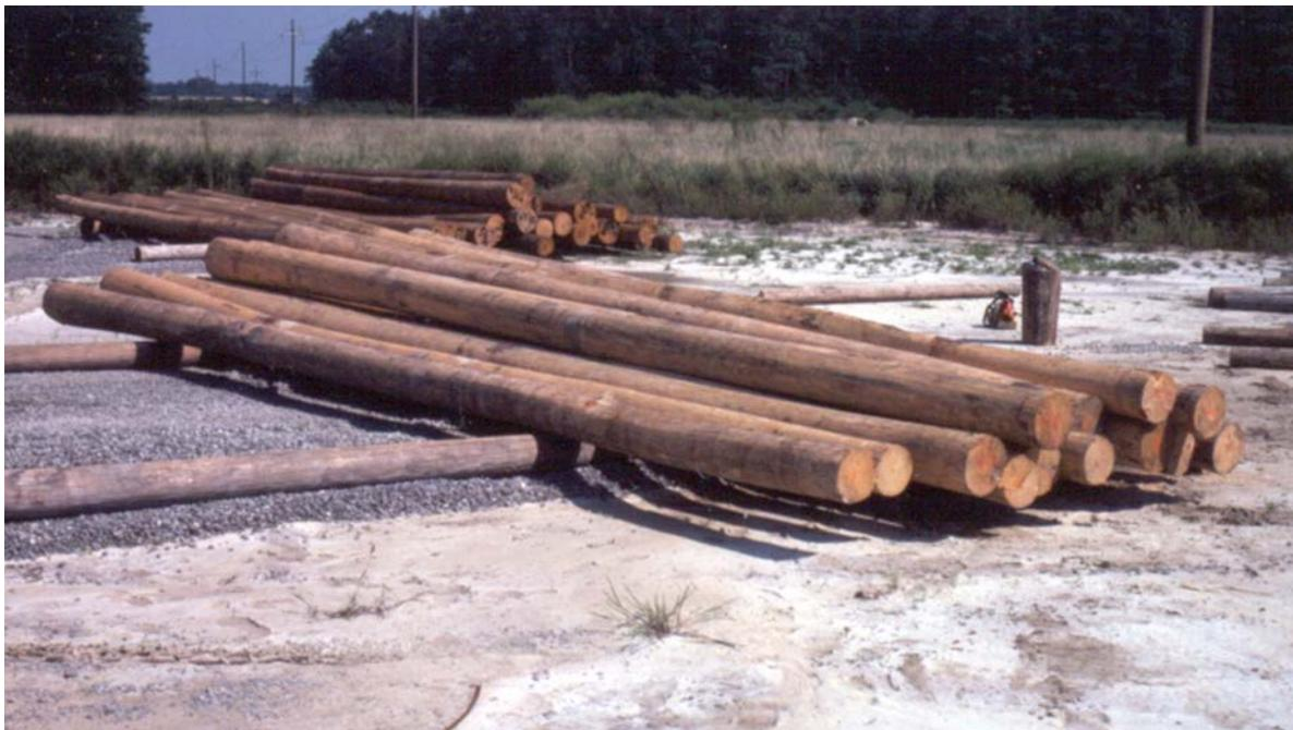
Figure 6-9 Timber piles.
