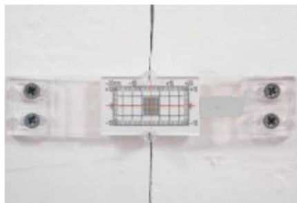
Figure 5- 12: Crack Gauge (Avongard Products USA)
