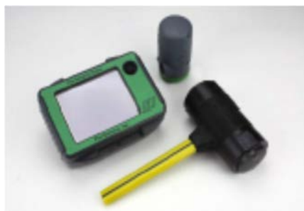
Figure 5-3: Pile Integrity Tester (Pile Dynamics, Inc.)
