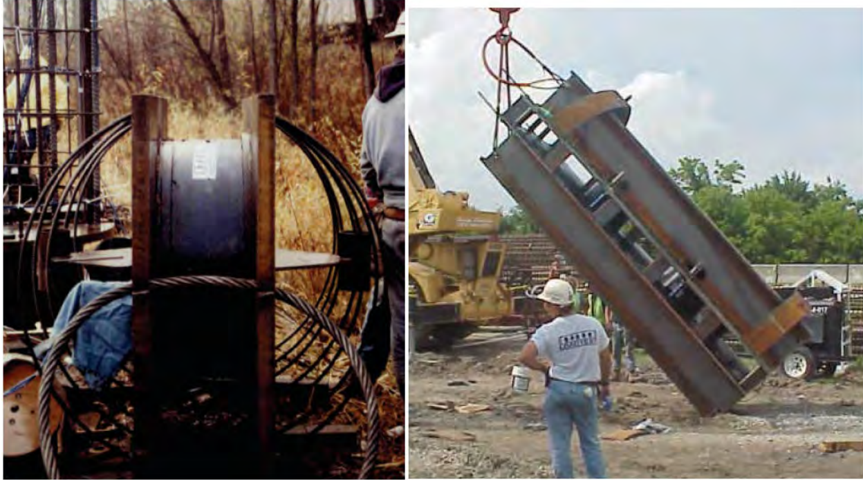
Figure 12-4: Bi-directional Lateral Testing Apparatus Using Embedded Load Cells (from Brown et al. 2010)
