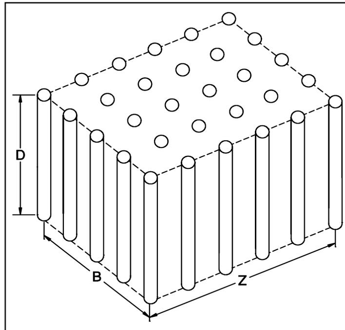
**Figure 9-34. Three dimensional pile group configuration (after Tomlinson, 1994).**
