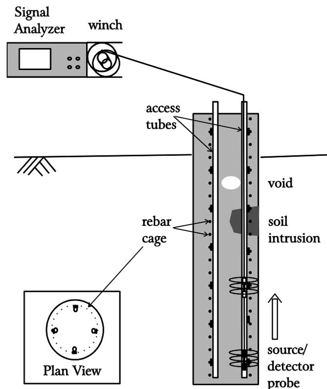
**Figure 9-60. Schematic of GDL Test (Samtani, *et al.*, 2005).**
