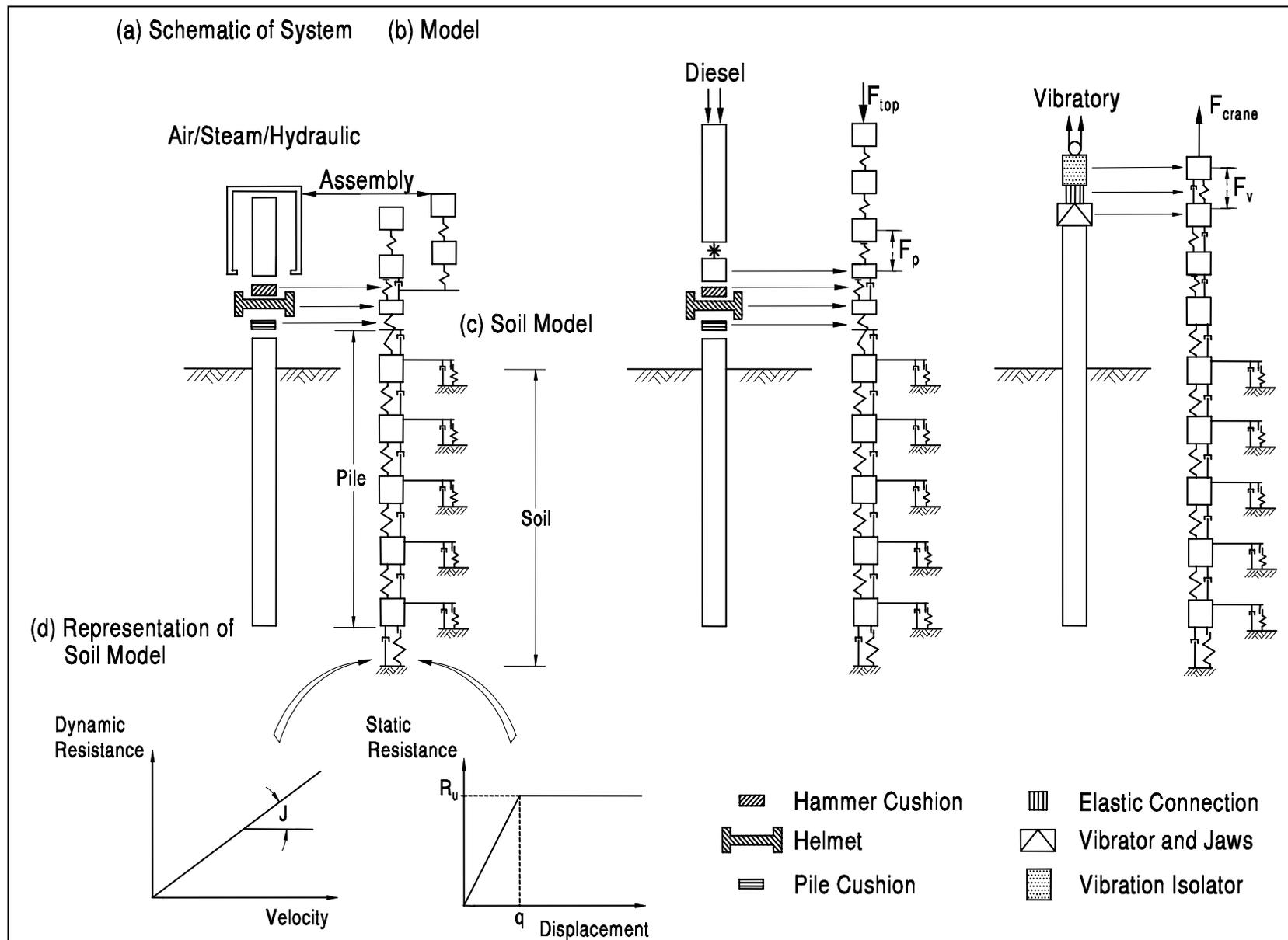
Figure 9-41. Typical Wave Equation models (FHWA 2006a).
