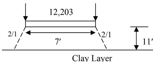
**Step 1 Determine pressure on clay layer (Refer to Section A.6-3 of text)**
