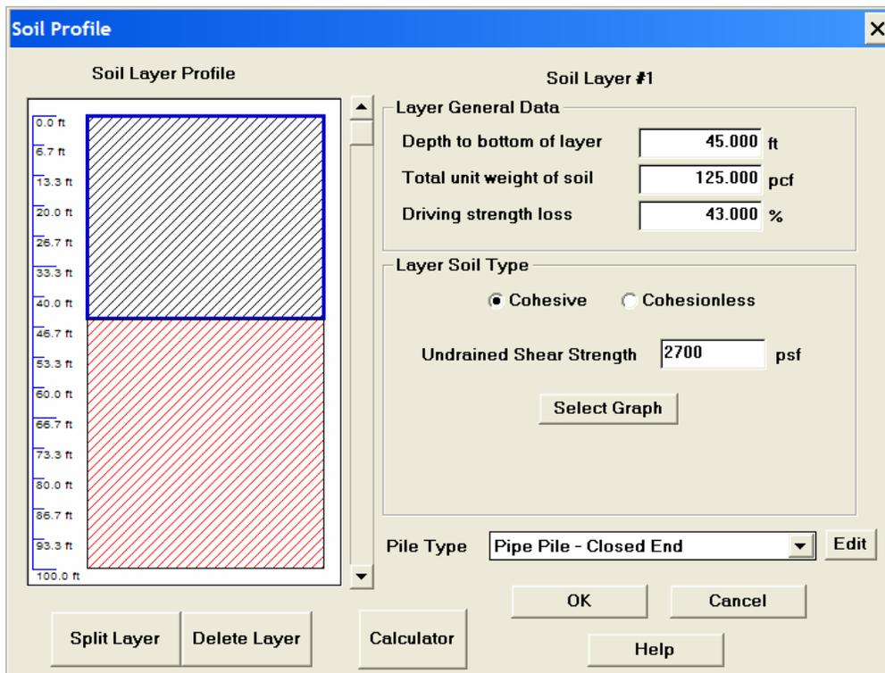
Figure 9-22. DRIVEN Soil Profile screen – cohesive soil.
