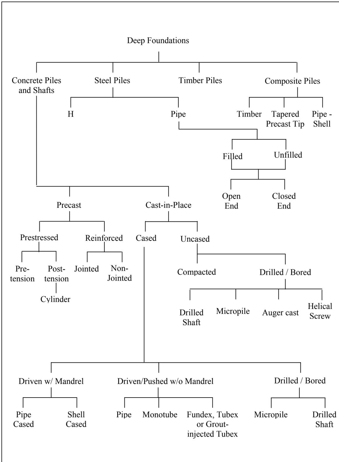
**Figure 9-2. Deep foundation classification system (after FHWA, 2006a).**
