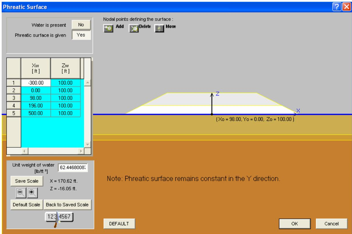
**Figure E-9. Input of water table.**
