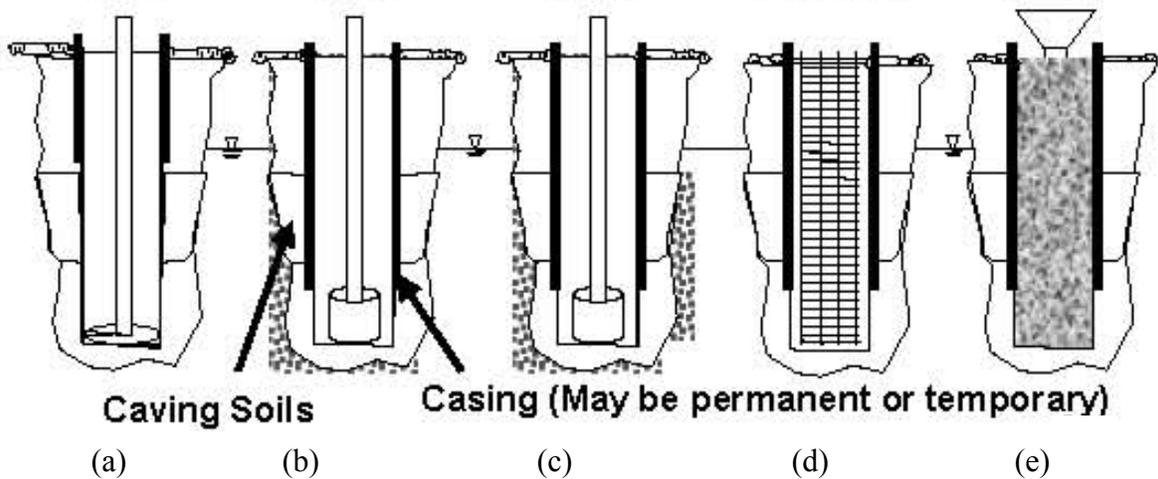
**Figure 9-56. Steps in construction of drilled shafts by the casing method (a) start drilling and introduce casing in the excavation PRIOR to encountering the known piezometric level and/or caving soil, (b) advance the casing through the soils prone to caving, (c) clean the excavation, (d) position reinforcement cage, and (e) place concrete and remove the casing if it is temporary.**
