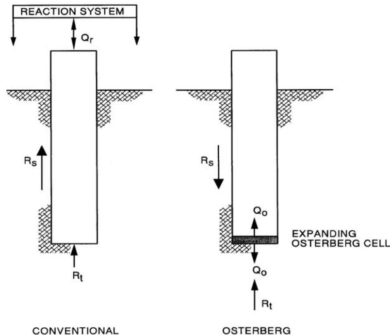
**Figure 9-72. Comparison of reaction mechanism between Osterberg Cell<sup>®</sup> and Static test.**
