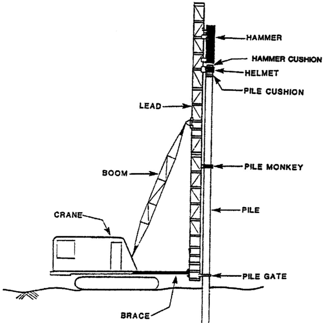
Figure 9-38. Typical components of a pile driving system.
