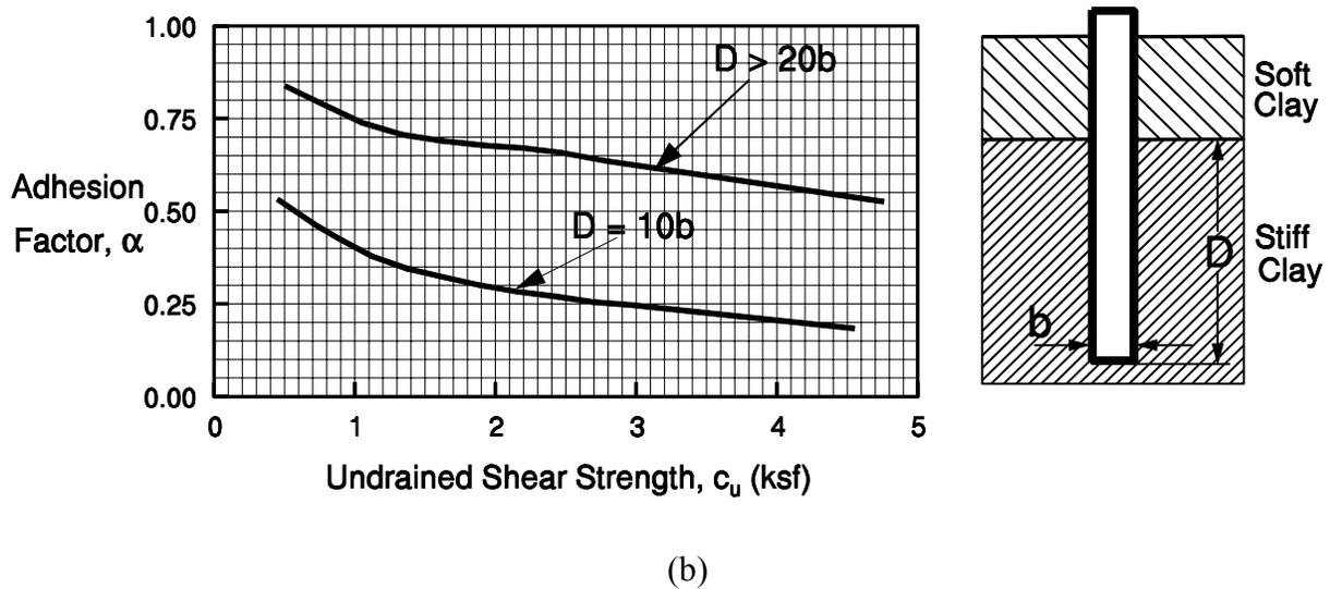
**Figure 9-15. Adhesion values for driven piles in mixed soil profiles, (a) Case 1: piles driven through overlying sands or sandy gravels, and (b) Case 2: piles driven through overlying weak clay (Tomlinson, 1980).**
