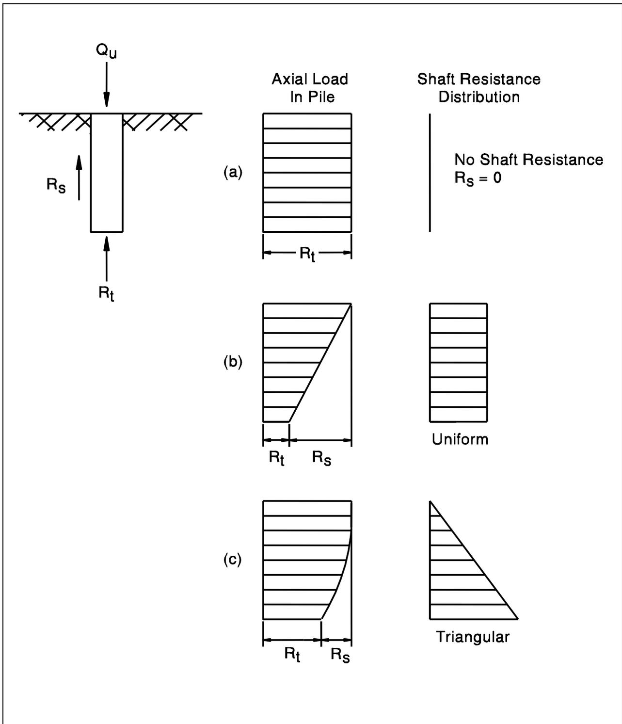
Figure 9-4. Typical load transfer profiles (FHWA, 2006a).
