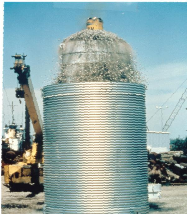
Figure 9-77. Photograph of Statnamic<sup>®</sup> test arrangement showing masses being accelerated inside gravel-filled sheath.
