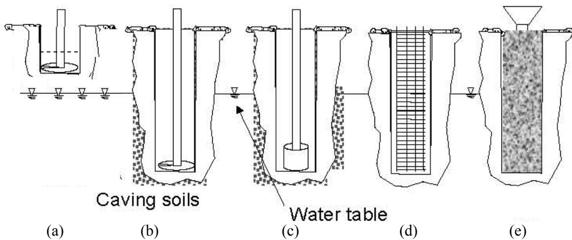
**Figure 9-55. Steps in construction of drilled shafts by the wet method (a) start drilling and introduce slurry (bentonite or polymer) in the excavation PRIOR to encountering the known piezometric level, (b) continue drilling with slurry in the excavation, (c) clean the excavation and slurry, (d) position reinforcement cage, and (e) place concrete by tremie.**
