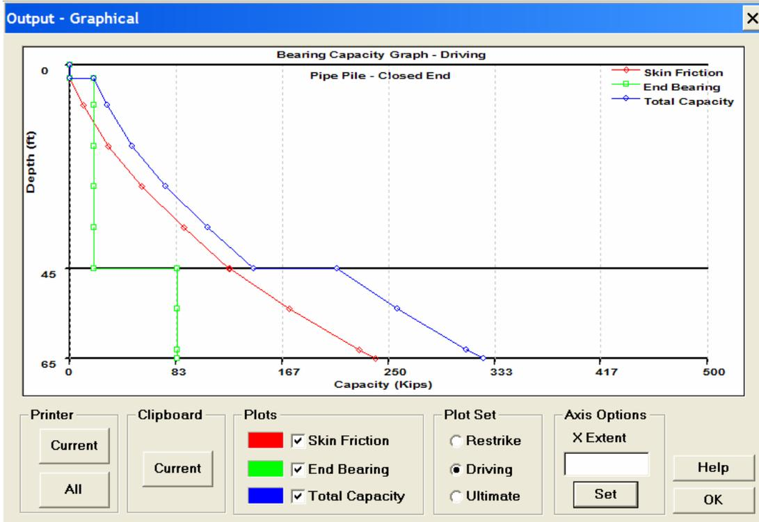
Figure 9-29. DRIVEN Output-Graphical screen for end of driving.
