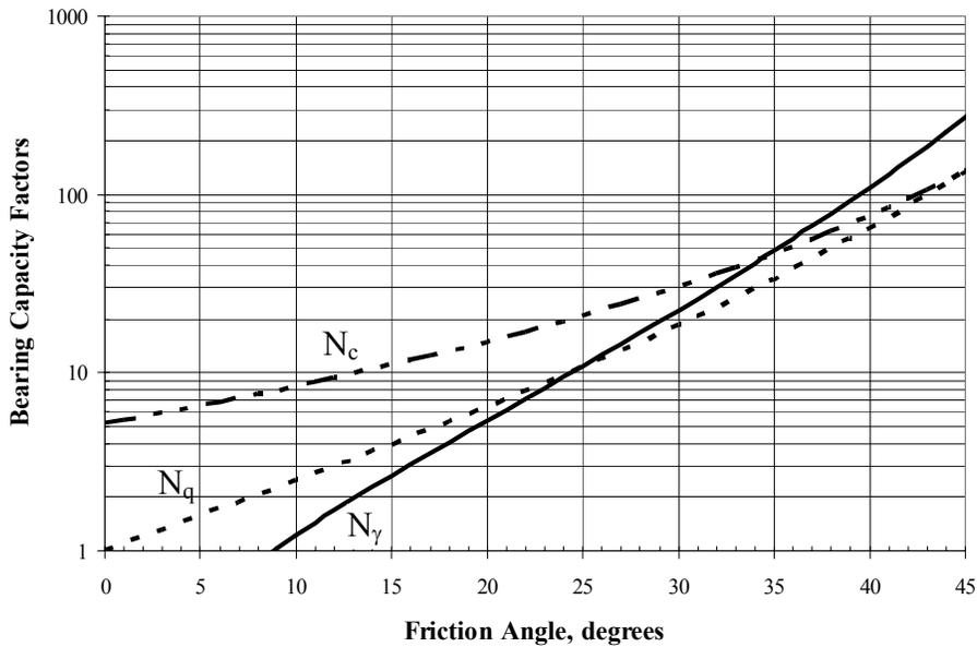
**Figure 8-15. Bearing capacity factors versus friction angle.**
