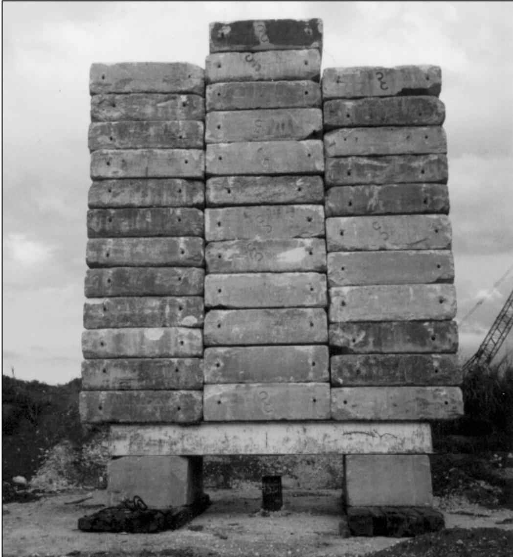
**Figure 9-67. Typical compression load test arrangement using a weighted platform (FHWA, 2006a).**
