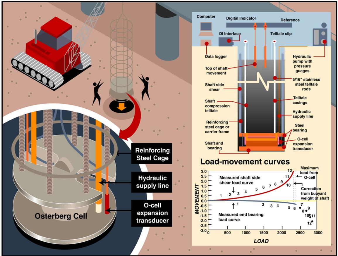
Figure 9-73. Some details of the O-Cell<sup>®</sup> test (after [www.bridgebuildermagazine.com](http://www.bridgebuildermagazine.com)).
