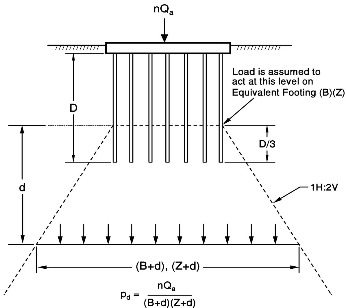
Note: Pile Group has Plan Dimension of B and Z
