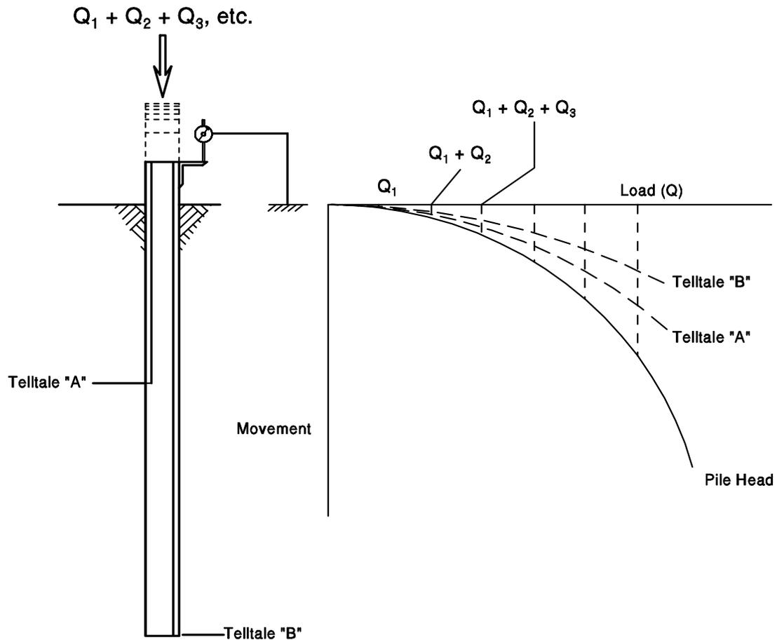
**Figure 9-62. Basic mechanism of a compression pile load test (FHWA, 2006a).**
