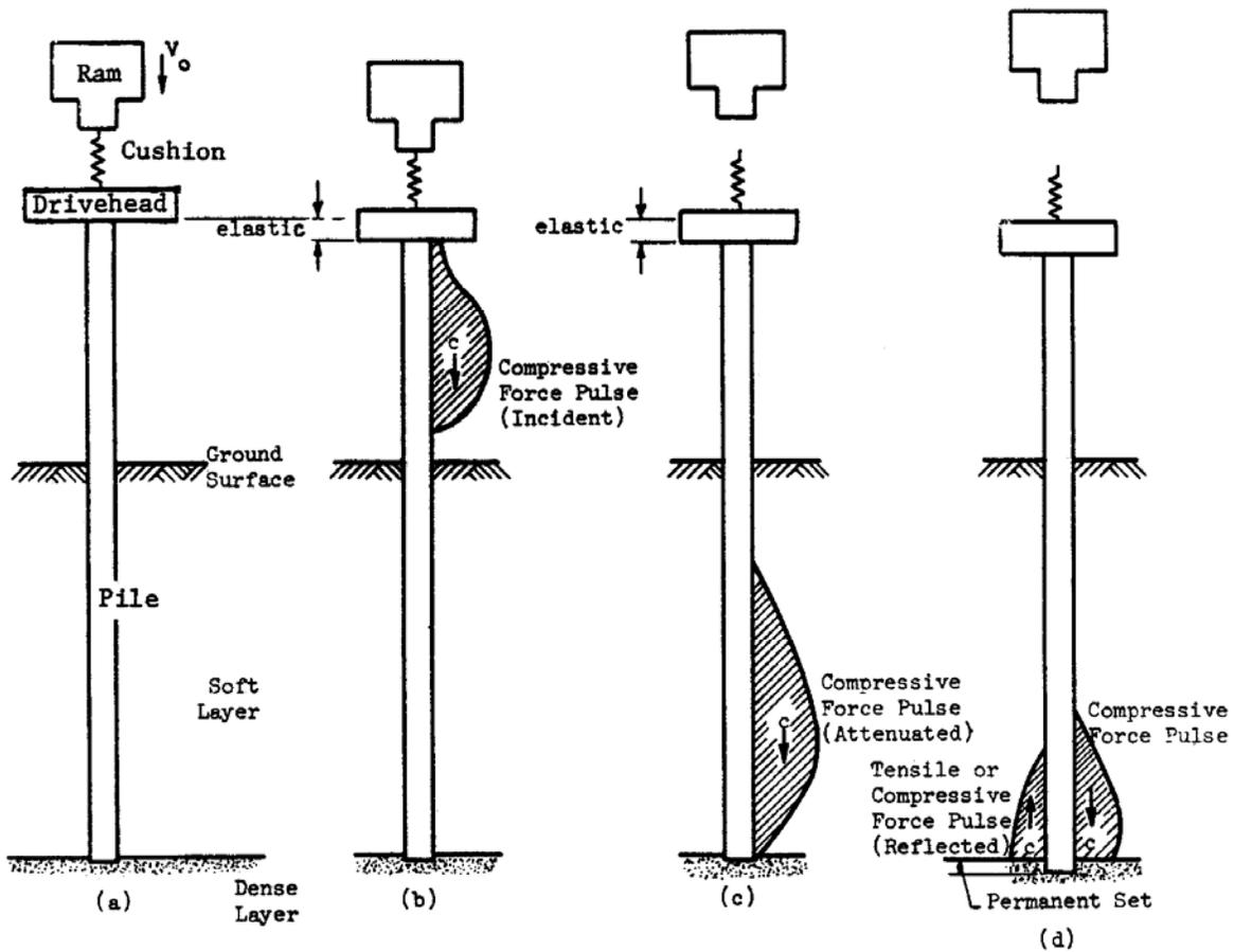
Figure 9-40. Hammer-pile-soil system.
