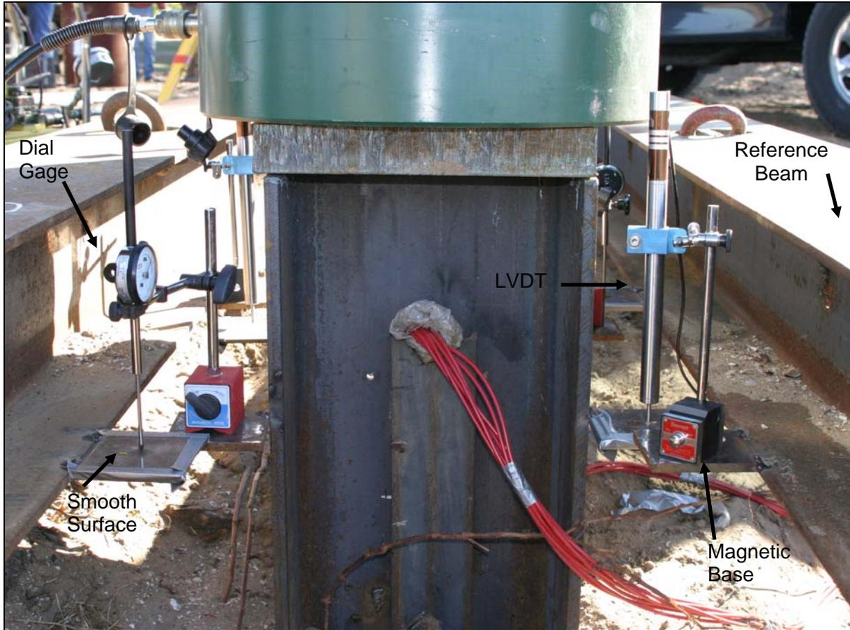
**Figure 9-65. Load test movement monitoring components (FHWA, 2006a).**
