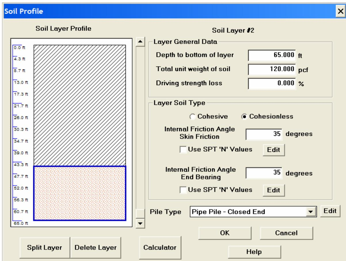
Figure 9-24. DRIVEN Soil Profile screen – cohesionless soil.
