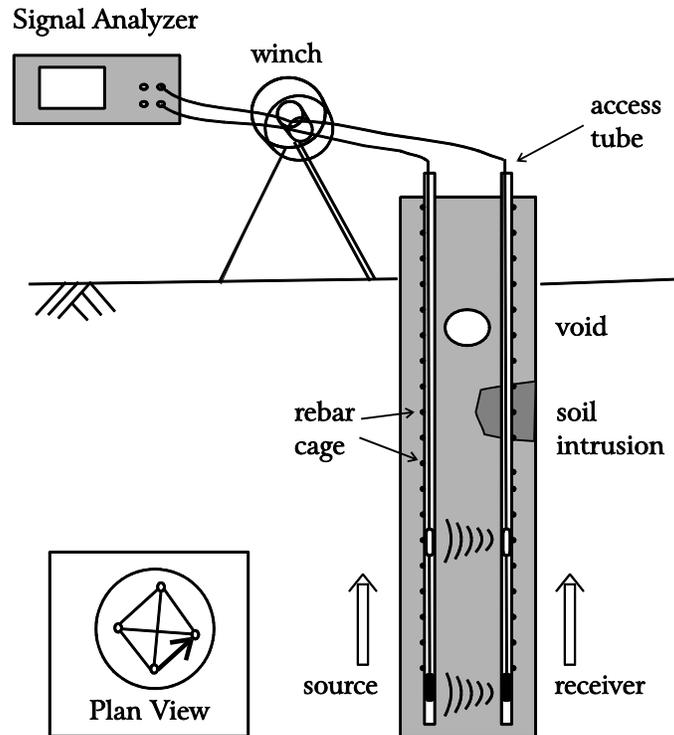
Figure 9-58. Schematic of CSL Test (Samtani, *et al.*, 2005).
