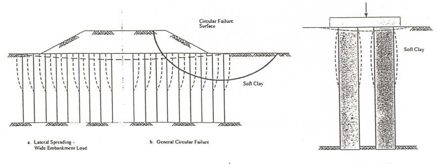
c. Bulging Failure - Small Group
