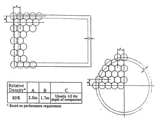
Figure 4-35. Typical compaction point spacing for area layouts.
