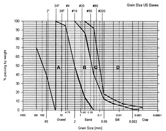
Figure 4-27. Range of soil types treated by vibro-compaction.
