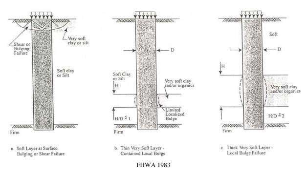
Figure 5-19. Failure modes of a single stone column in a non-homogeneous cohesive soil.
