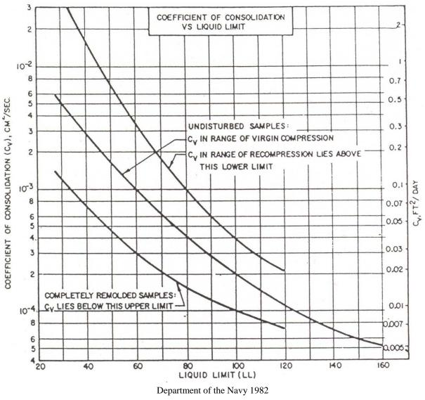
Figure 2-10. Coefficient of consolidation versus liquid limit.
