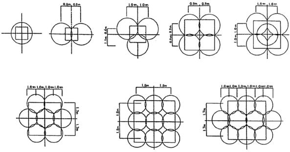
Figure 4-36. Typical compaction point layouts for column footings.
