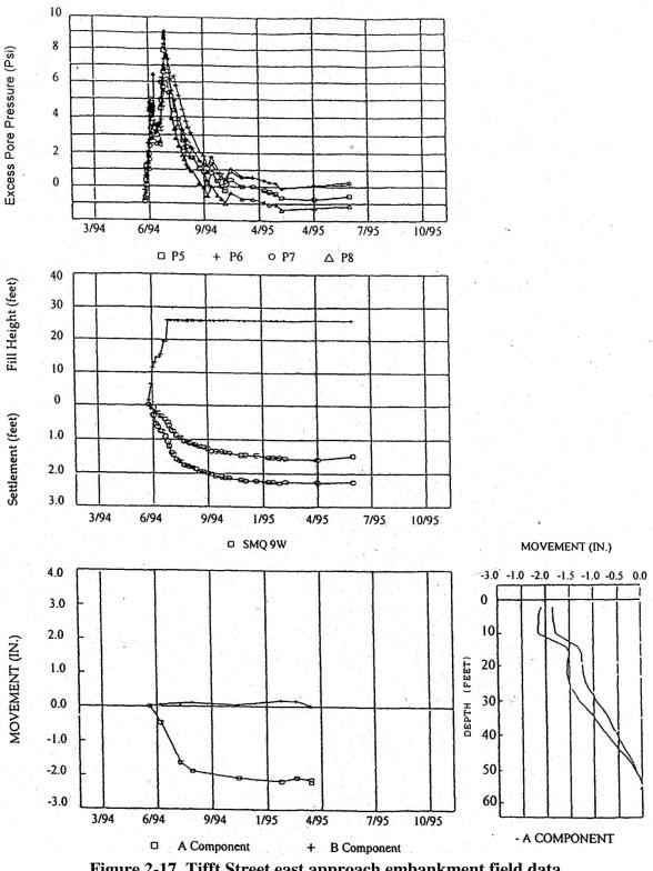
Figure 2-17. Tifft Street east approach embankment field data.
