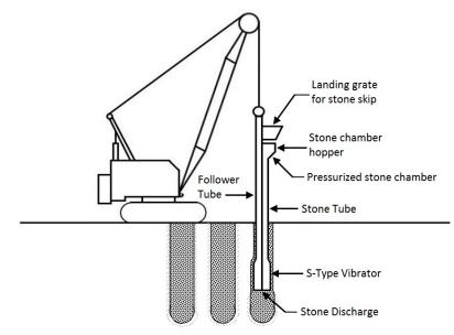
Figure 5-3. Bottom feed vibro-displacement.
