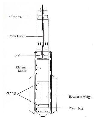
Figure 4-30. Cross-section of a typical vibrator.
