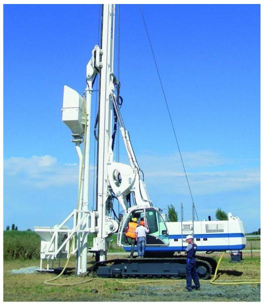
Courtesy Treviicos Figure 5-8. Dry bottom feed rig.
