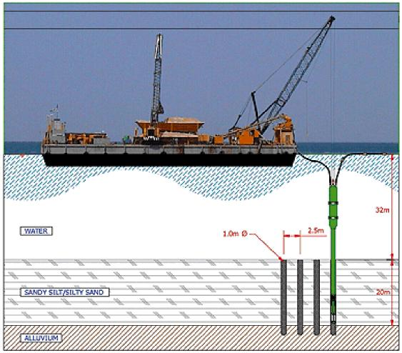
Vibroflotation Group Figure 5-10. Marine double-lock gravel pump.
