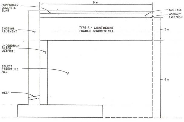
Harbuck 1993, TRB Figure 3-13. Foamed concrete fill behind existing abutment, New York project.
