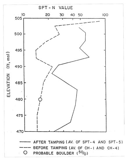
Figure 4-24. Increase in SPT values in a mine spoil after deep dynamic compaction.
