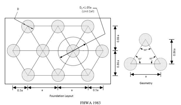
Figure 5-16. Equilateral triangular pattern of stone columns.
