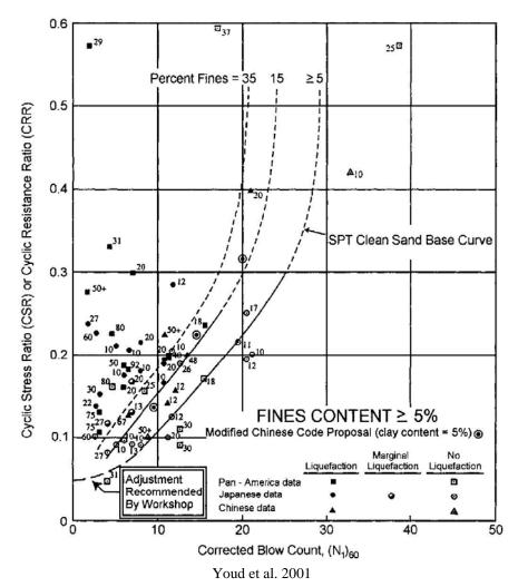
Figure 4-3. SPT liquefaction chart for magnitude 7.5 earthquakes.
