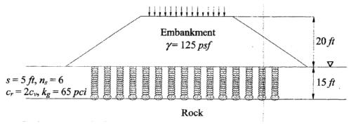
Figure 5-25. Aggregate column ground improvement layout.
