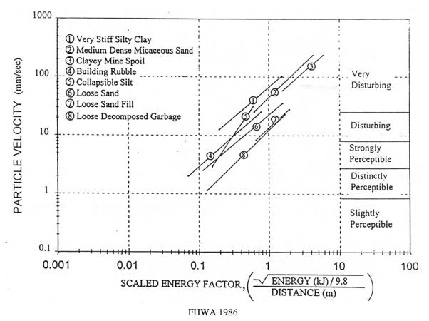
Figure 4-7. Scaled energy factor versus particle velocity.
