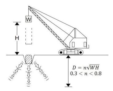
Figure 4-1. Schematic illustration of deep dynamic compaction.
