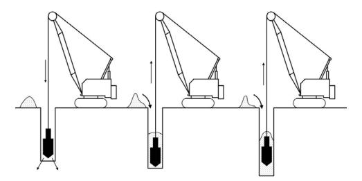
Figure 4-2. The vibro-compaction process.
