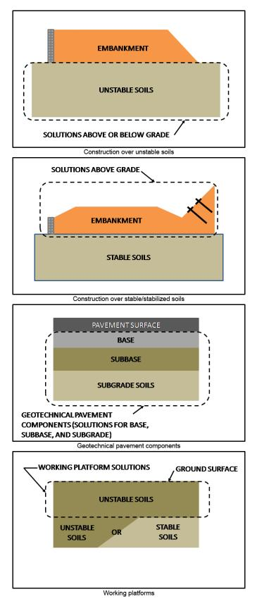
Figure 1-1. Elements of construction.
