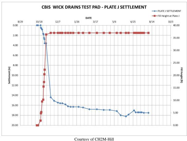
Figure 2-15. Settlement versus fill height for test pad.
