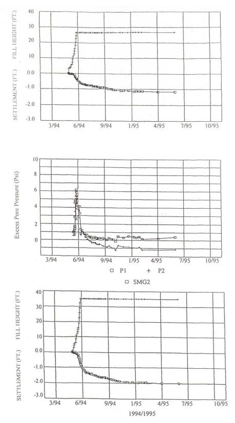
Figure 2-16. Tifft Street west approach embankment field data.
