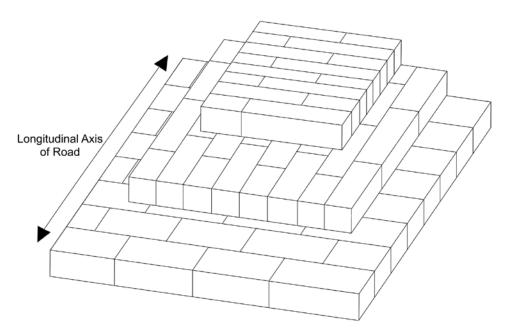
After Stark et al. 2004b Figure 3-9. Isometric view of typical EPS block layout.
