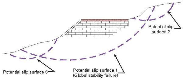
Arellano et al. 2011. Copyright National Academy of Sciences. All rights reserved. Figure 3-8. Multiple potential failure surfaces to consider with EPS-block geofoam slope systems.
