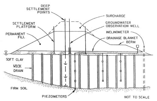
Figure 2-14. PVD Installation showing typical instrumentation and monitoring.
