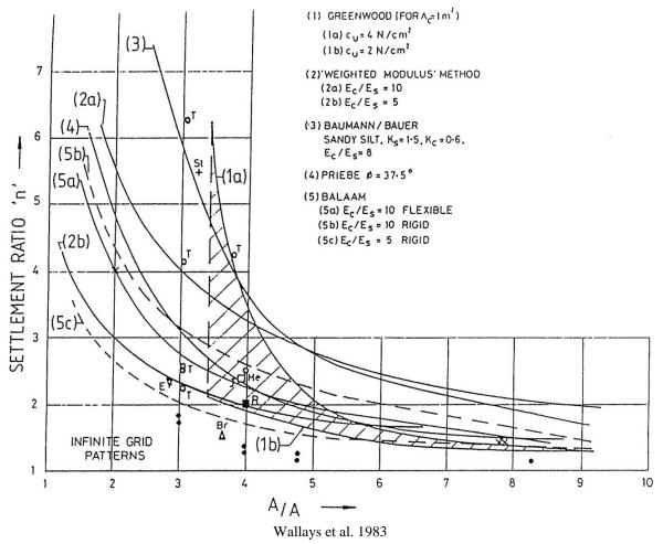
Figure 5-21. Comparison of elastic theories and field observations.
