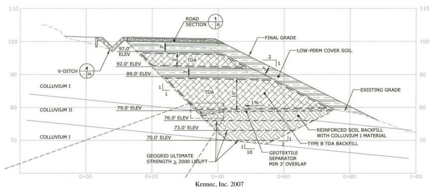
Figure 3-14. Marina Drive slope cross section.
