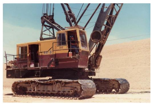
Figure 4-16. Dragline-type lifting crane with 1<sup>1</sup>/<sub>4</sub>-inch cable for use with 40 kip tamper.
