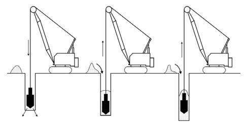
Figure 5-2. Top feed vibro-replacement.
