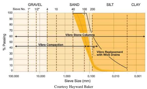
Figure 5-1. Soils applicable for stone columns.
