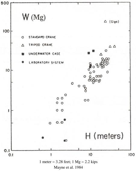
Figure 4-22. Relationship between tamper mass and drop height.
