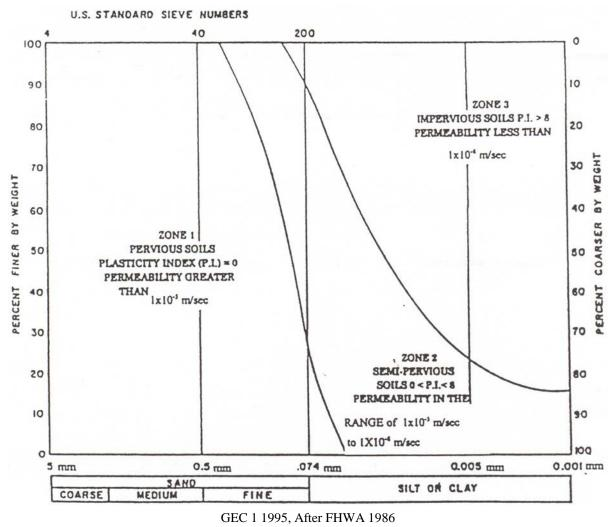
Figure 4-5. Grouping of soils for deep dynamic compaction.
