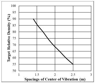
Figure 4-34. Relative density versus probe spacing for silty sands.
