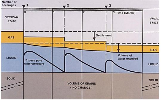
The soil behavior during deep dynamic compaction is illustrated in Figure 4-4.
