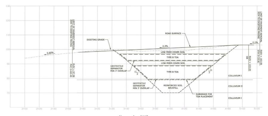
Kennec, Inc. 2007 Figure 3-15. Marina Drive longitudinal section of fill replacement.
