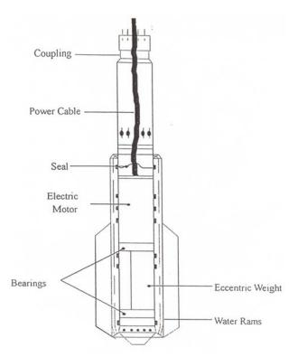
Figure 5-5. Typical vibrator cross-section.
