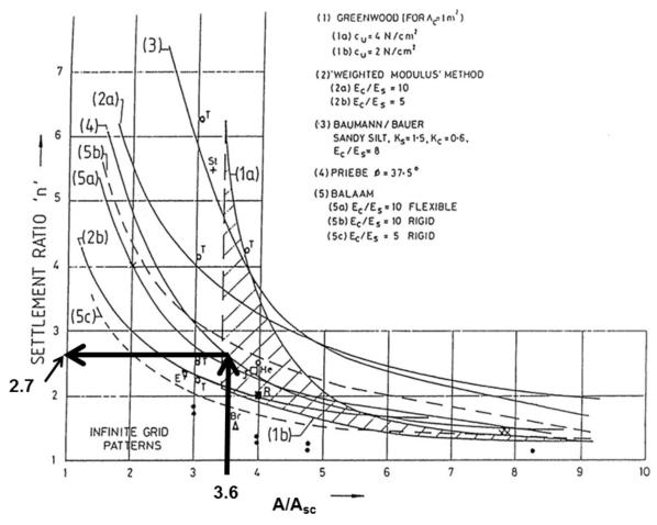
After Wallays et al. 1983 Figure 5-27. Example problem 2 settlement ratio determination.
