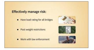
To effectively manage the risk of a bridge failure due to overload, a bridge owner must:
