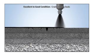
When existing pavements develop these conditions but are still in good condition, some agencies are able to extend the useful life of pavements by 3 to 7 years by sealing the surface with a more robust combination of asphalt and aggregate.
