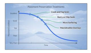
Crack and fog seals are most appropriate for pavements in excellent to good condition and can extend the life of pavement by 1 to 4 years.
