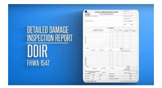
The team documents the damage at each site with FHWA's Detailed Damage Inspection Report form, or DDIR. The report lists the specific location and type of Federal-aid roadway along with describing the damage. Location maps, field site sketches, and photographs help document the damage. The DDIR also alerts FHWA of potential environmental or historical impacts, and includes any recommendations from the FHWA field engineer.
