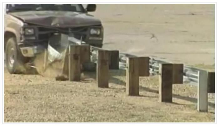
But lawsuits filed after crashes across the country allege that the device called the ET-Plus can lock up, causing the guardrail to pierce the car. Or it can kick off to the side, allowing the car to continue on.
