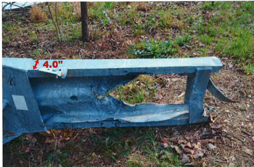
Figure 9 – End Terminal Sleeve Dimensions
