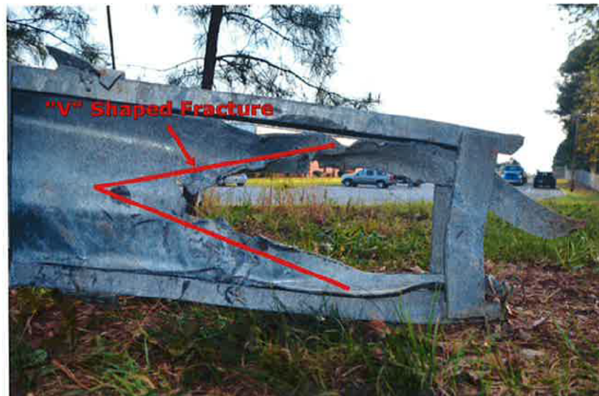
Figure 8 – End Terminal Detail
