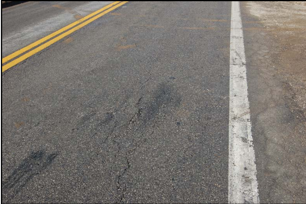
DSC9.JPG - View of Vehicle #1 front left pre- and post-impact tire marks and Vehicle #2 left front post-impact tire mark and gouges in the westbound lane, looking west
