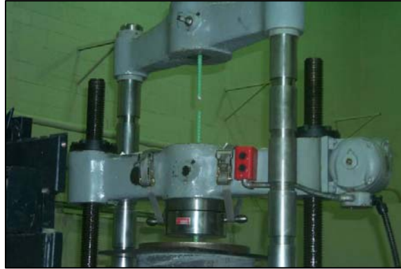
Fig. 6 Pullout Test Set-up showing Failure Behavior
