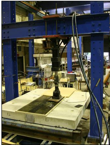
Fig. 7 Bridge deck panels with water ponding under fatigue loading (courtesy of FHWA)
