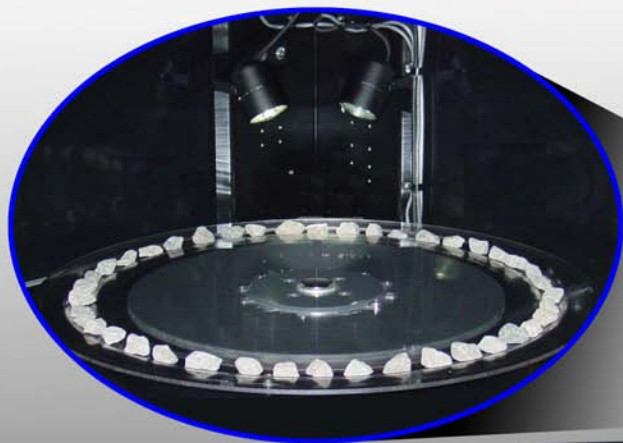
Research has shown a link between aggregate characteristics and pavement performance. The AIMS2 device analyzes aggregate characteristics objectively and accurately.
