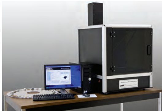
AIMS2 is an integrated hardware/software system that automates the process of measuring the particle angularity, form, and surface texture. The AIMS2 image-based analysis removes operator influence from the characterization while improving productivity and precision.
