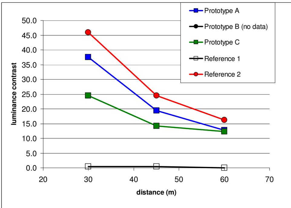
**Figure 29. Luminance contrast between the test marking and the adjacent roadway surface as a function of distance (rain conditions, Contrast = (L<sub>marking</sub>-L<sub>road</sub>)/L<sub>road</sub>).**
