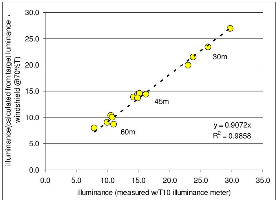
**Figure 22. Correlation between the total illuminance from the vehicle headlights measured with the handheld luminance meter and total illuminance calculated from the average luminance of the right & left diffuse target, corrected for the transmission of the windshield (dry conditions).**
