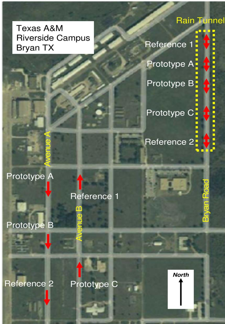
Figure 15. Experimental test course layout.
