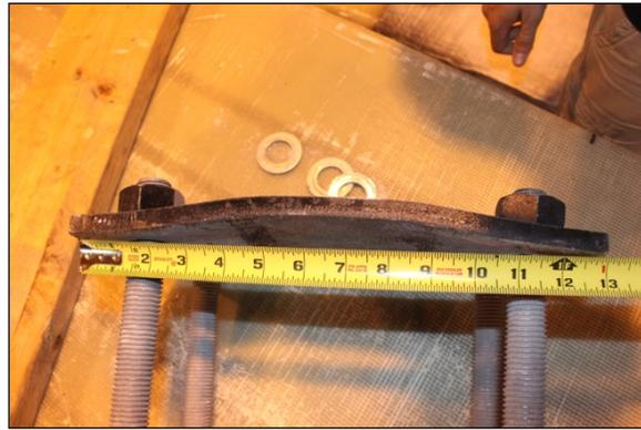
(b) Bent on steel plate
