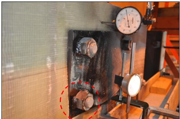
(a) Steel plate wedging failure
