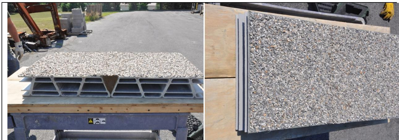
Figure 89. Photos. FRP specimen used for pull-off tests.
