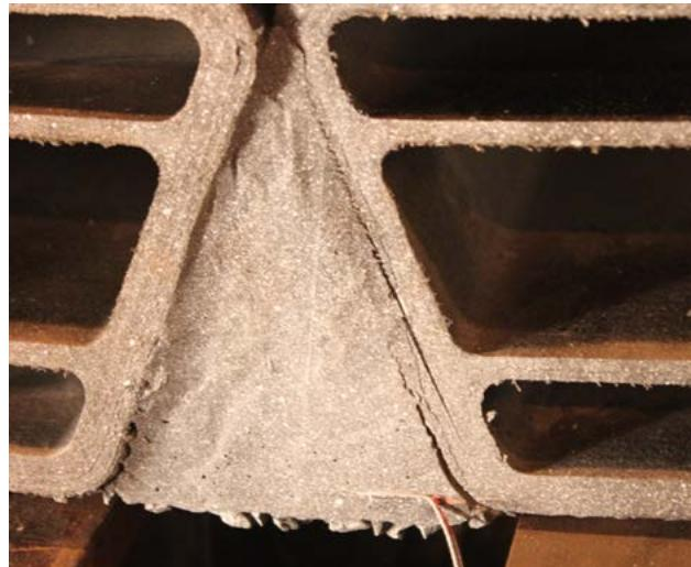
Figure 68. Photo. Crack at maximum load of 14.7 kips.
