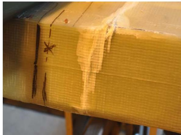
Top surface of the damaged outer wrap
