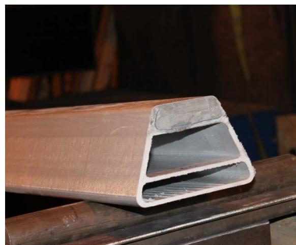
Figure 27. Photos. Cementitious grout slipping at the end of FRP tube #60.
