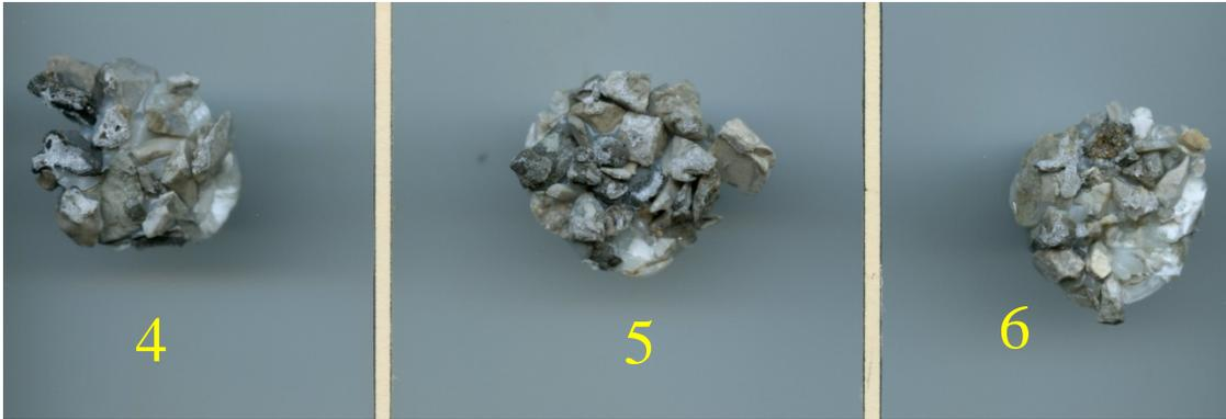
Figure 91. Photos. Failure surfaces of aggregate to adhesive pull-off tests (dollies 4, 5, and 6).
