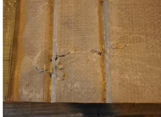
Craking detail-top surface FRP tubes
