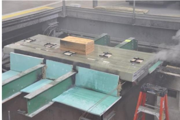
Figure 97. Photo. The test panel just after the test stopped. Note that the top surface kept cooler and ended up with little deterioration.
