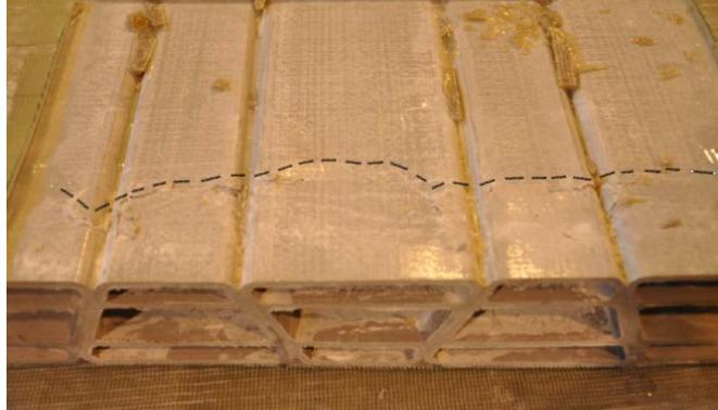
Compression cracks on top of FRP tubes
