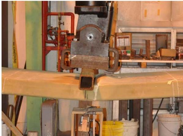
Failure at midspan: buckling of outer wrap
