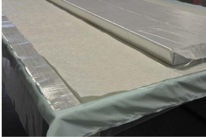
Figure 4. Photo. The panel is wrapped in glass fiber in preparation for infusion with vinyl ester resin.
