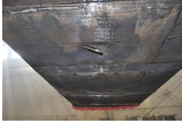
Figure 100. Photo. The glass fiber on the bottom has frayed due to burn-off of the resin matrix.
