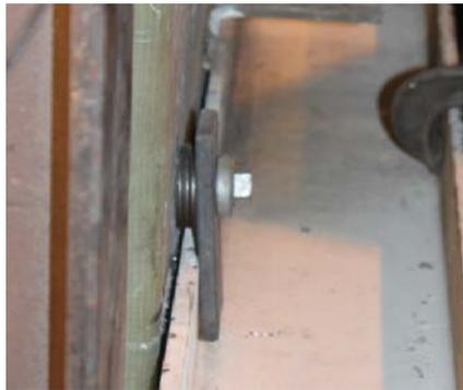
(c) Profile view of bolted connection
