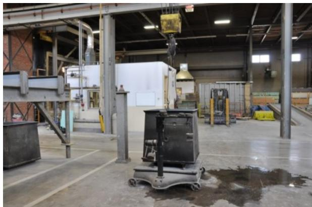
Figure 95. Photo. 1,600-lb water tank used as concentrated load.
