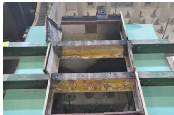
Figure 94. Photo. Support beams spaced at 2 feet.
