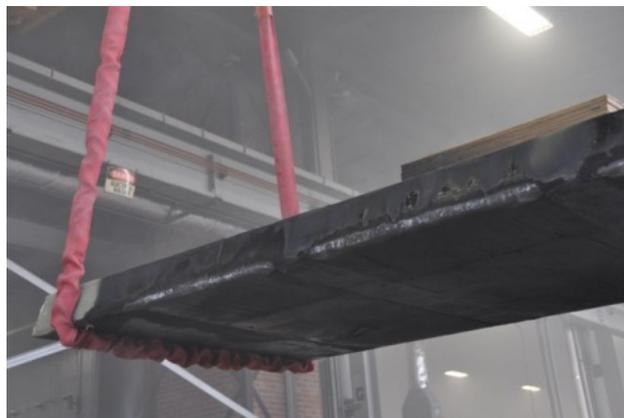
Figure 98. Photo. Specimen immediately after the test. Note the extent of damage on the bottom.
