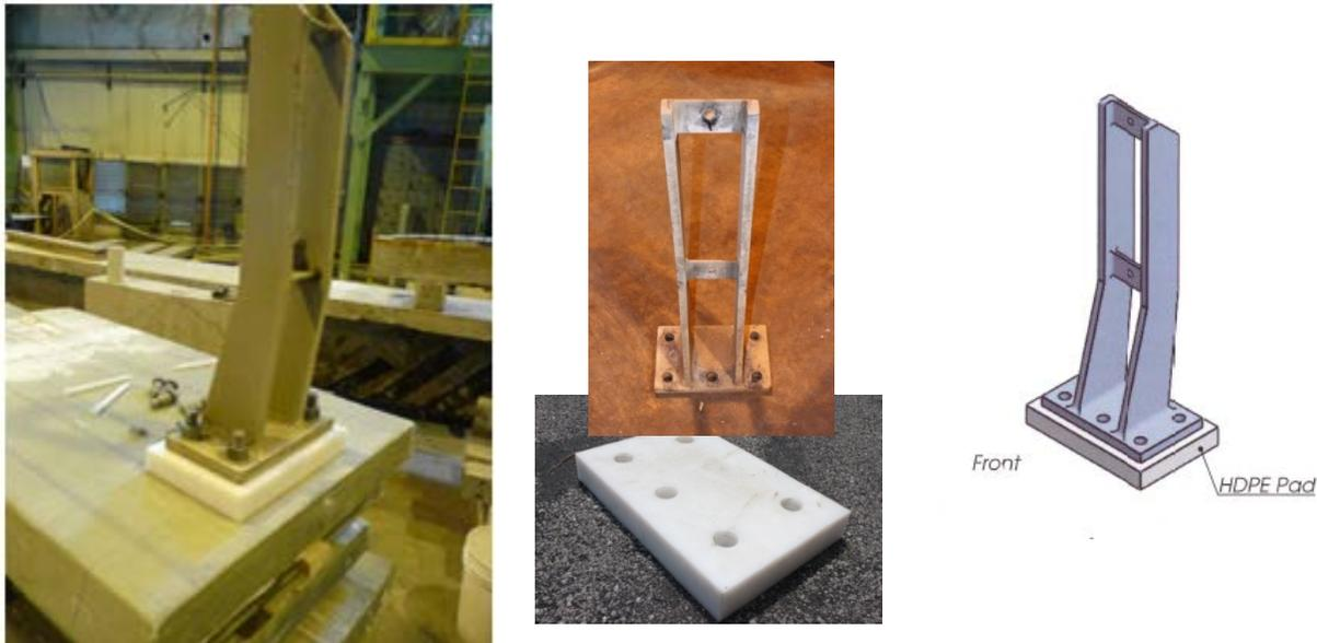
Figure 75. Photos and sketch. Railing post specimen.
