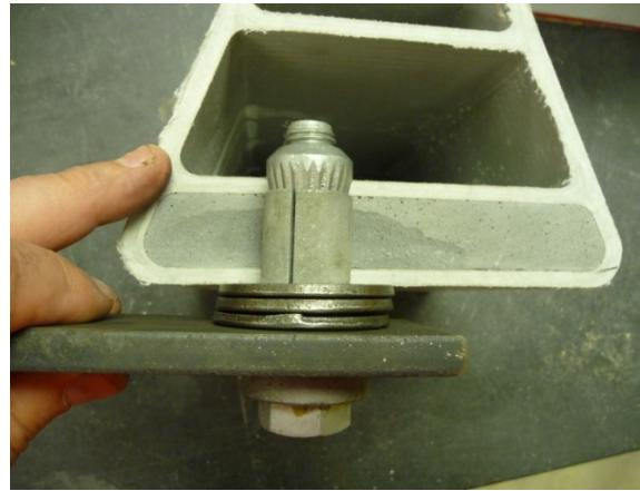
(b) Cross section of FRP tube & connection
