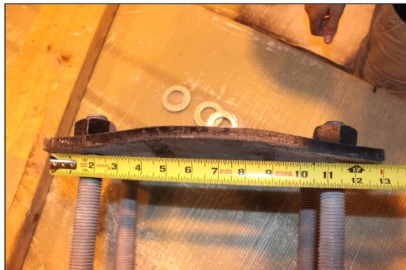
(b) Bent on steel plate
