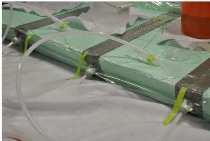
Figure 5. Photo. Resin is infused for the outer wrap using a vacuum-assisted resin transfer molding (VARTM) method.
