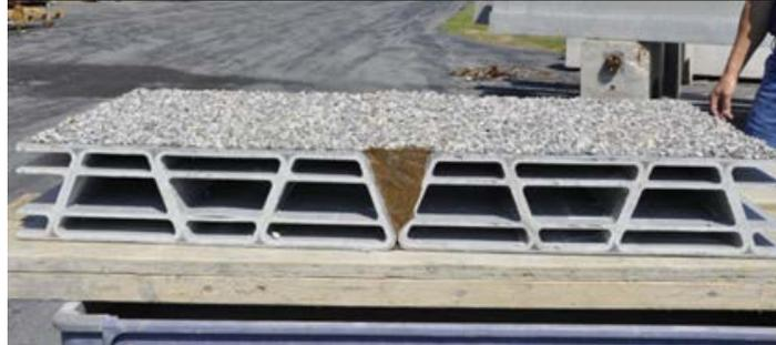
Figure 64. Photo. Panel-to-panel field joint.
