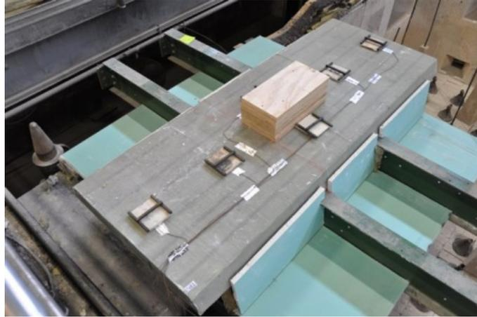
Figure 93. Photo. Test panel mounted on top of fire chamber.
