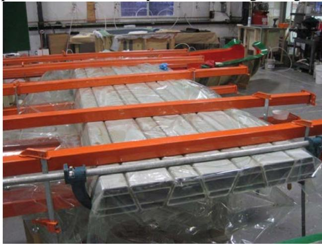
Figure 2. Photo. Tube subcomponents are bonded together with adhesive to form a panel.
