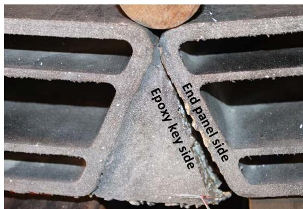
Figure 69. Photo. Failure of the specimen (11.8 kips).
