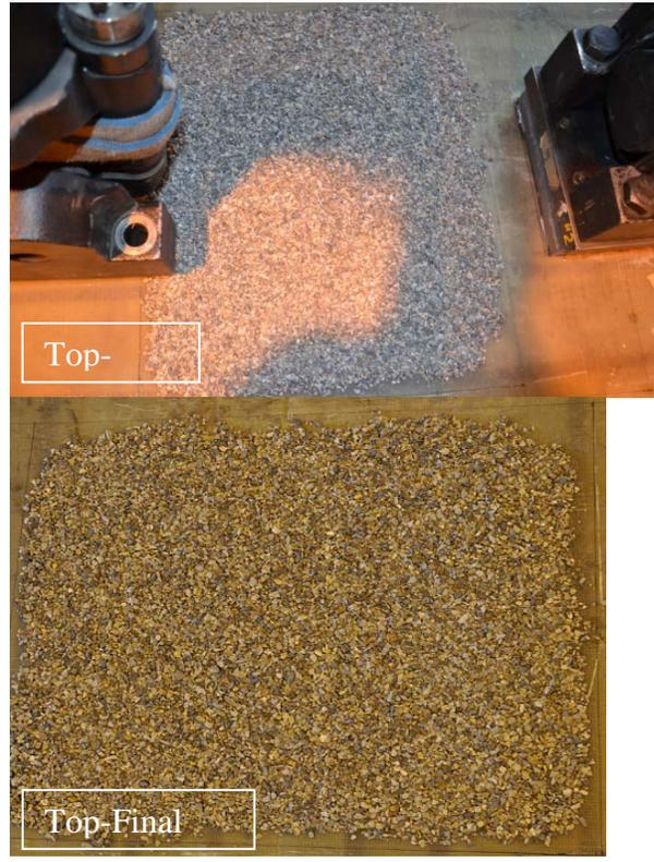
Figure 57. Photos. Top wearing surface before and after 350,000 cycles fatigue load
