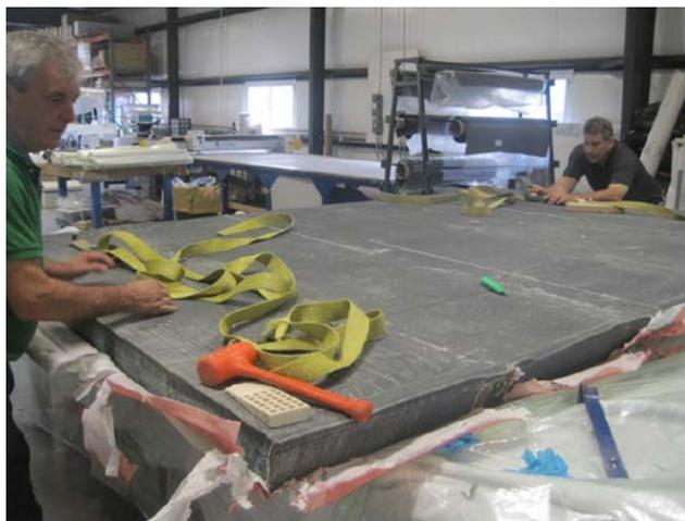
Figure 6. Photo. Each infused deck panel is stripped and inspected to ensure that fibers have been thoroughly wet-out with resin.
