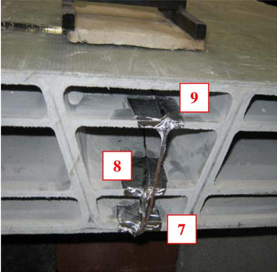
Figure 96. Photos. Placement of thermocouples on the test panel.
