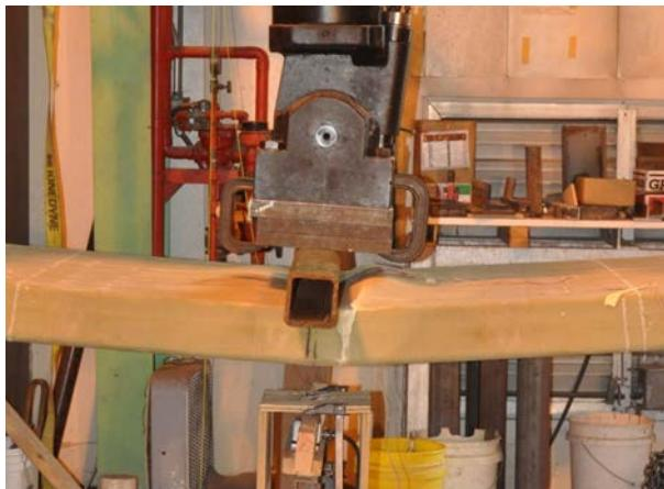
Failure at midspan: buckling of outer wrap
