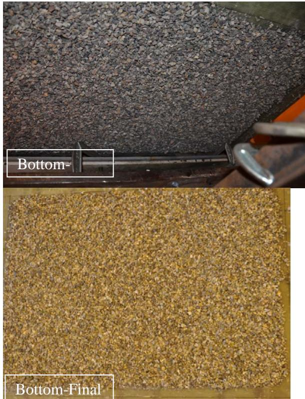
Figure 56. Photos. Bottom wearing surface before and after 500,000 cycles fatigue load.
