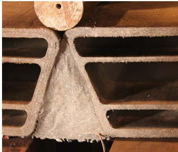
Figure 67. Photo. Crack at load of 7 kips.
