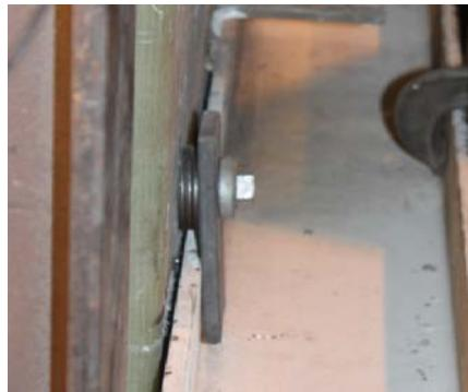
(c) Profile view of bolted connection
