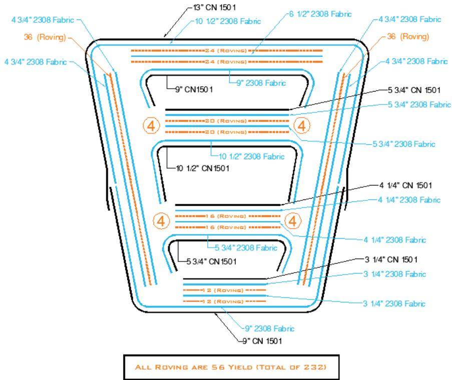
Figure 7. Diagram. Laminate construction for pultruded combi tube.
