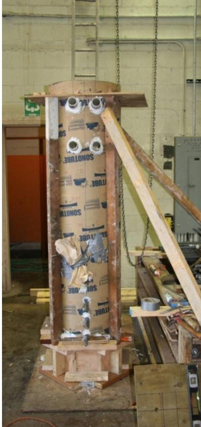
Figure 158. Photo. Specimen SF-3, column formed and ready to be cast.
