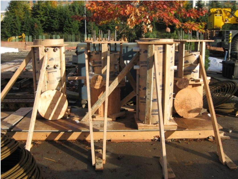
Figure 157. Photo. Specimens SF-1 and SF-2, column segments formed and ready to be cast.
