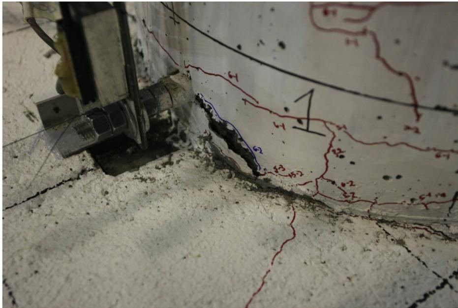
Figure 141. Photo. Specimen SF-3: first column spalling in cycle 6-2 (+2.48/-2.48 target drift ratio).
