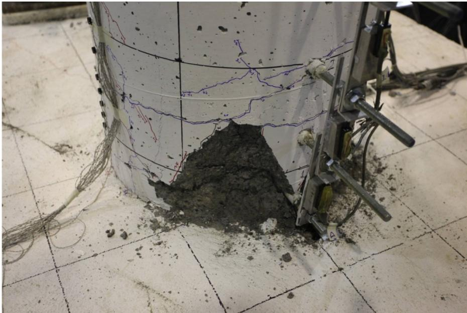
Figure 145. Photo. Specimen SF-3: full column spalling in cycle 9-1 (+6.16/-6.16 target drift ratio).
