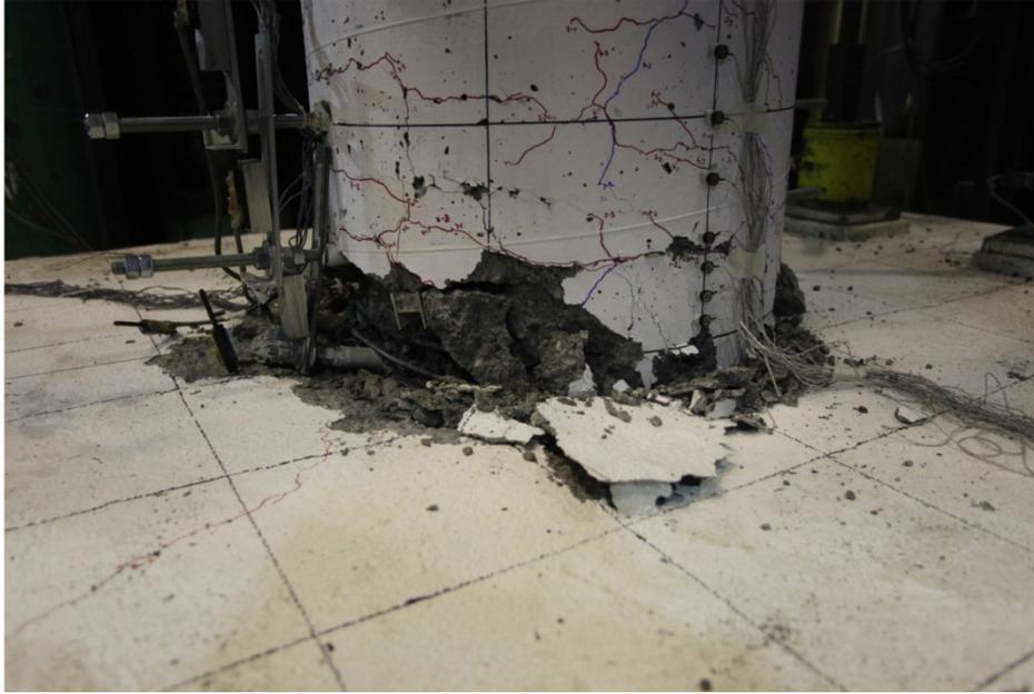
Figure 154. Photo. Specimen SF-3: column after punching through in last cycle (cycle 10-3, +10.65/-10.65 target drift ratio).
