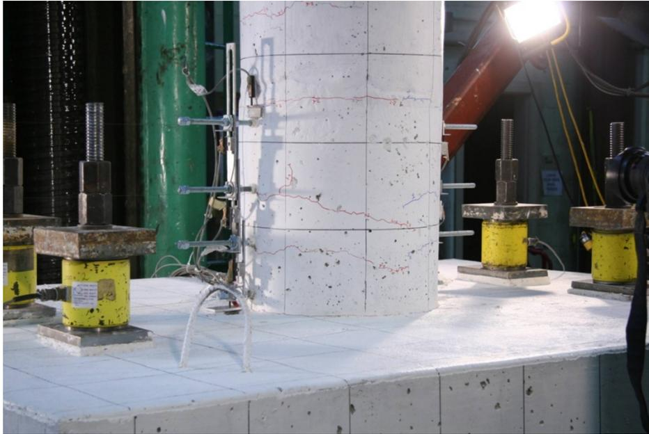
Figure 130. Photo. Specimen SF-2: flexural cracks after cycle 3-2 (+0.83/-0.83 target drift ratio).
