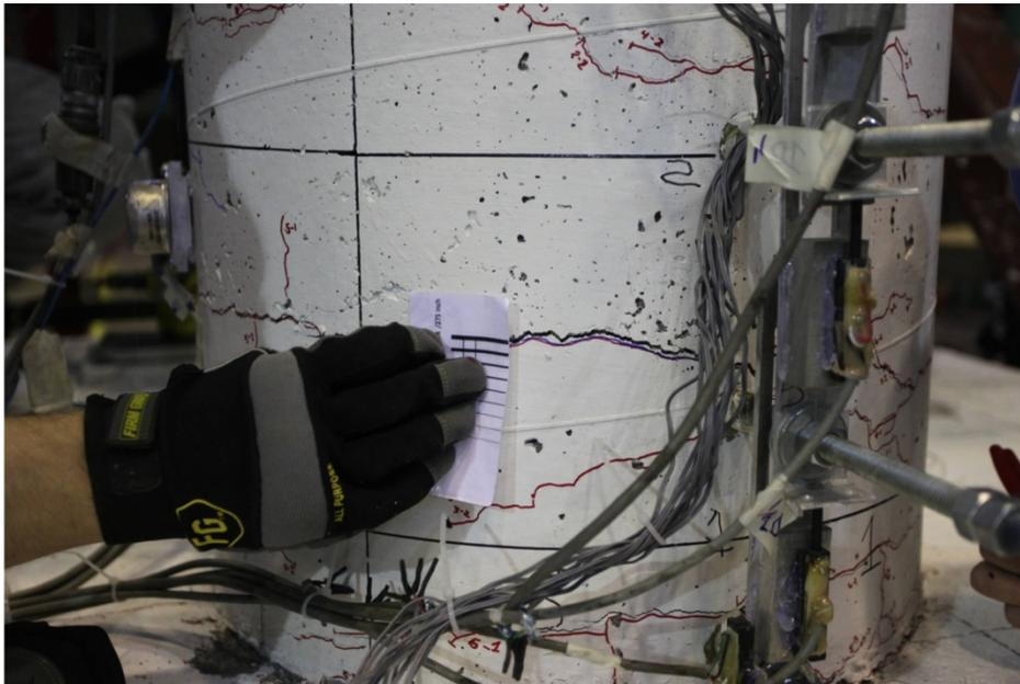
Figure 143. Photo. Specimen SF-3: large horizontal crack in cycle 6-2 (+2.48/-2.48 target drift ratio).
