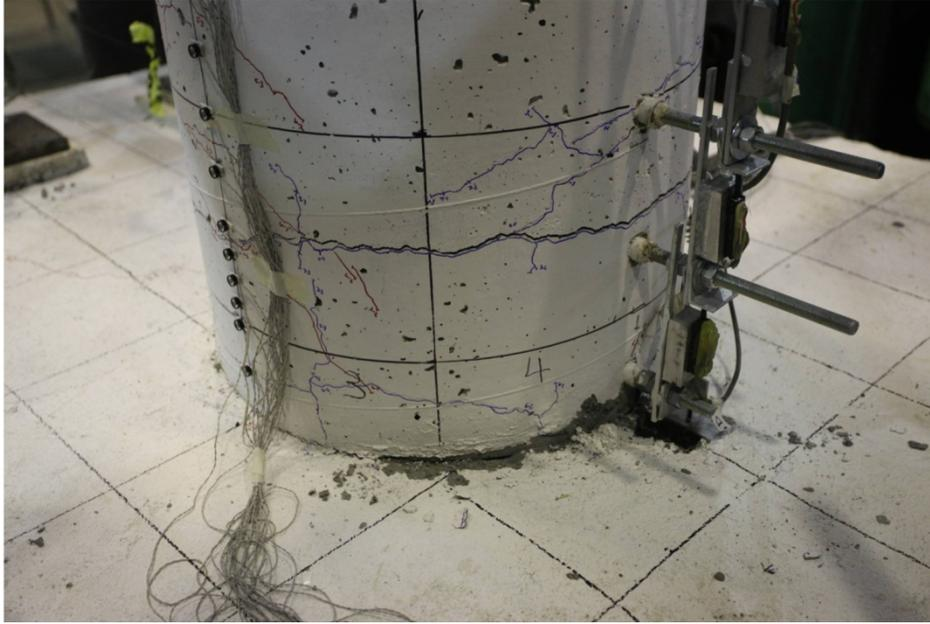
Figure 140. Photo. Specimen SF-3: first diagonal cracking in cycle 6-1 (+2.06/-2.06 target drift ratio).
