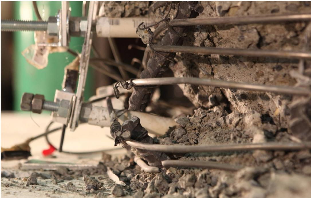
Figure 19. Photo. Specimen SF-1 longitudinal bars fractured after one cycle to 10.65 percent drift ratio.
