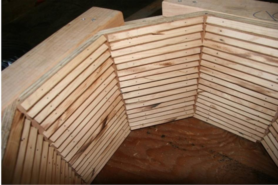
Figure 156. Photo. Roughened surface of octagonal, bottom portion of column.
