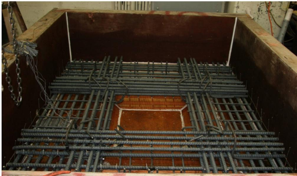
Figure 160. Photo. Specimen SF-3 footing formwork and reinforcement.
