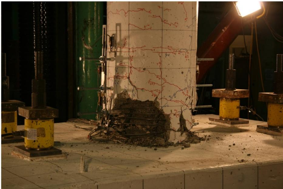
Figure 127. Photo. Specimen SF-1: damage after the cyclic testing.
