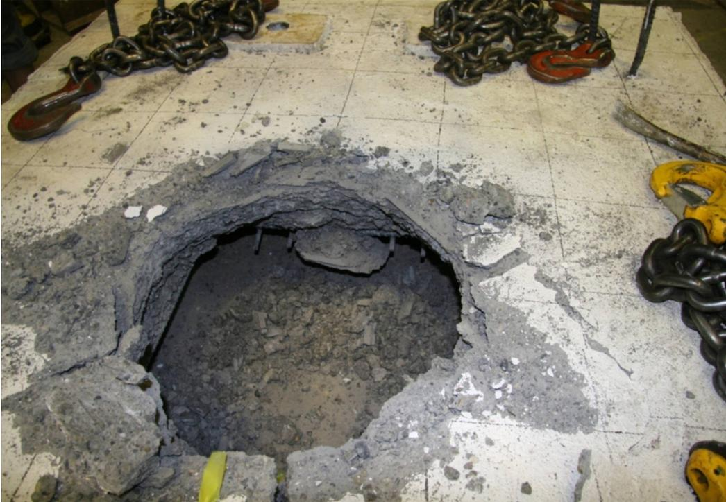
Figure 21. Photo. Damage on top of footing after test.
