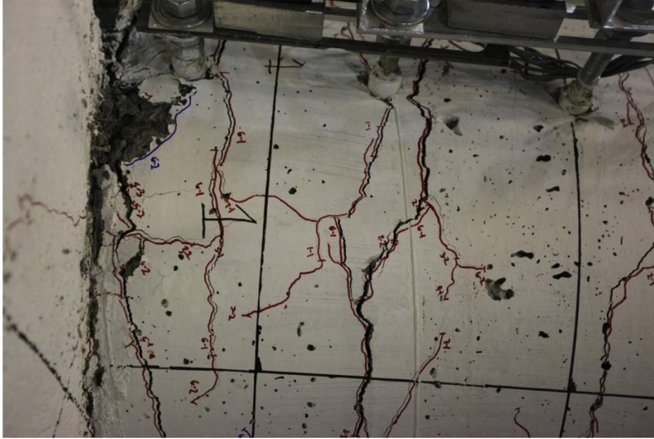
Figure 144. Photo. Specimen SF-3: large column flexural cracks occurring in cycle 7-2 (+3.57/-3.57 target drift ratio).
