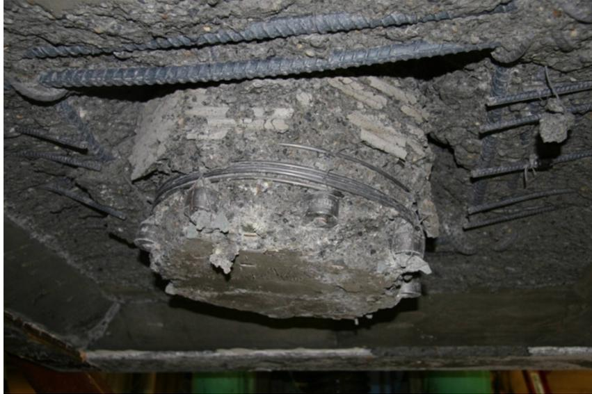
Figure 75. Photo. Joint region of specimen SF-3 after failure.
