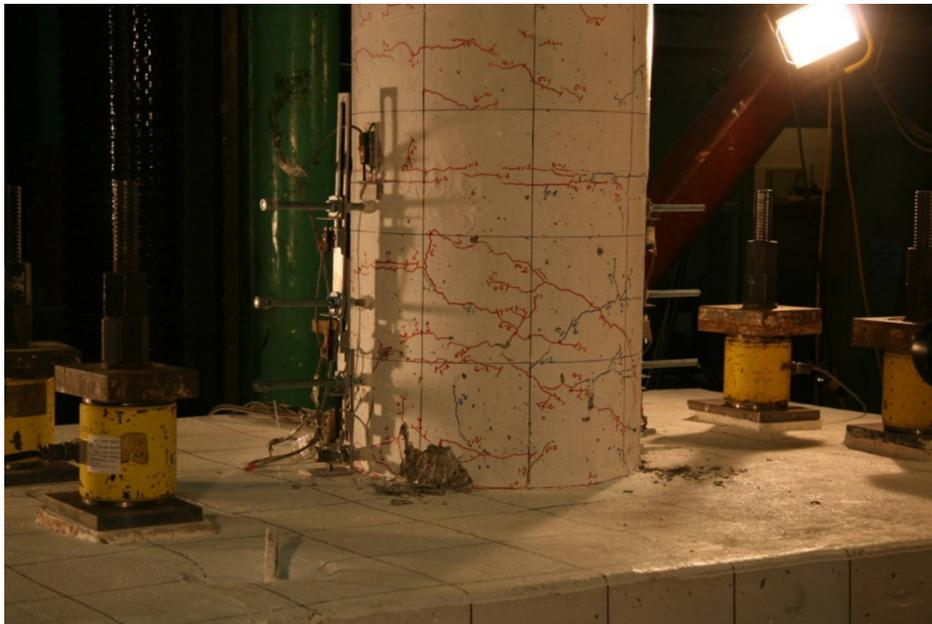
Figure 123. Photo. Specimen SF-1: first significant spalling at cycle 6-2 (+2.48/-2.48 target drift ratio).
