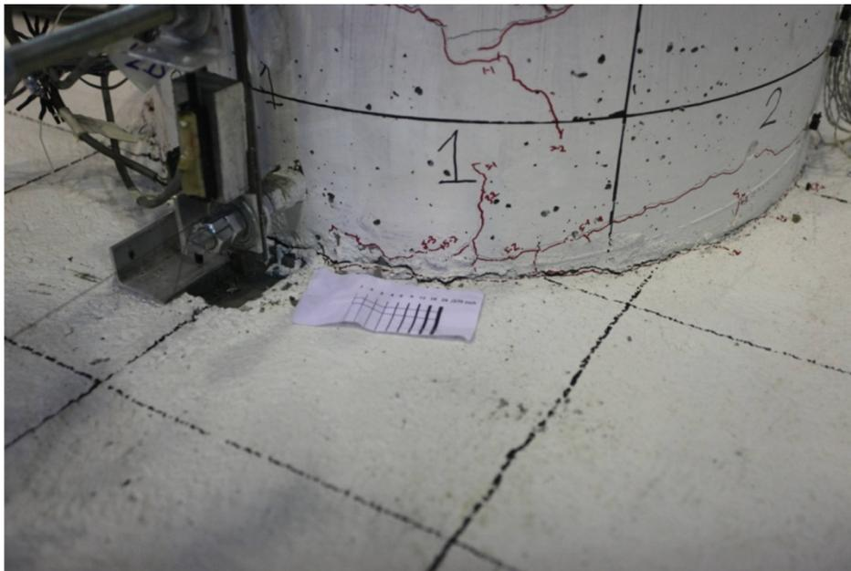
Figure 139. Photo. Specimen SF-3: separation at column-footing interface in cycle 5-3 (+1.72/-1.72 target drift ratio).
