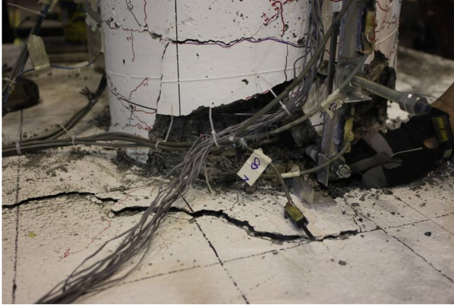
Figure 150. Photo. Specimen SF-3: major footing spalling occurring in cycle 10-1 (+8.87/-8.87 target drift ratio).
