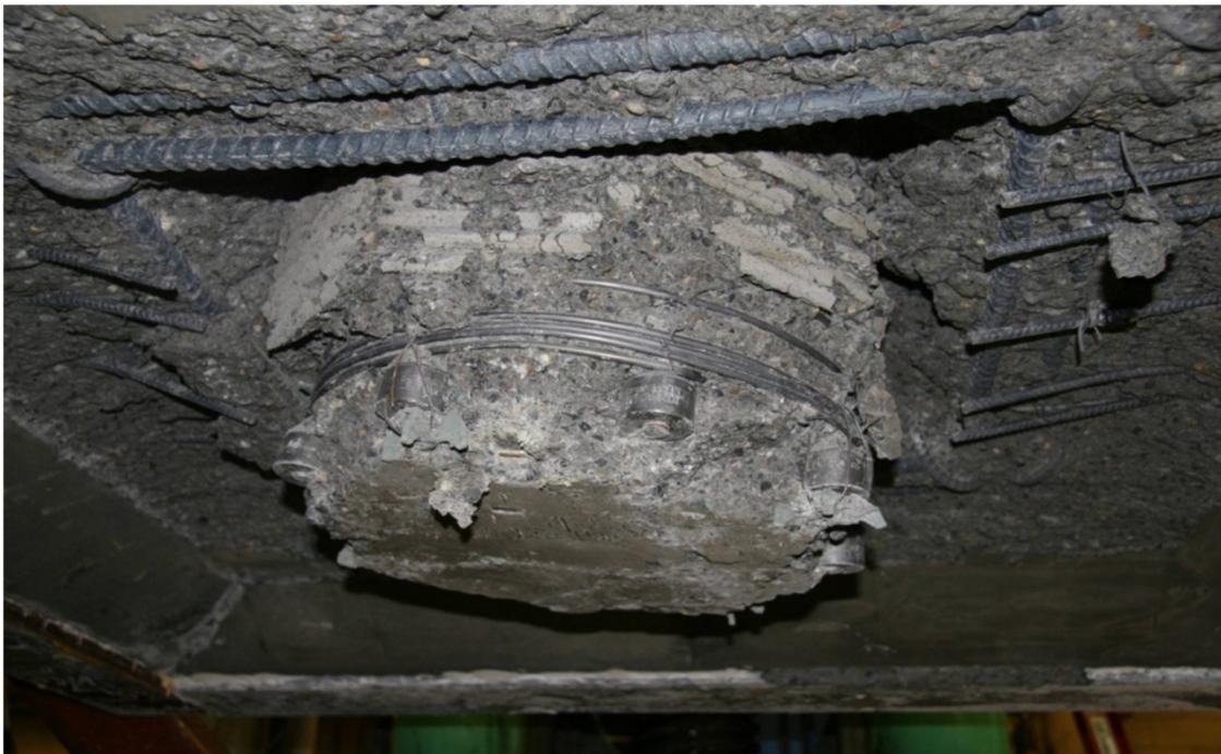
Figure 20. Photo. Specimen SF-3 footing failure.
