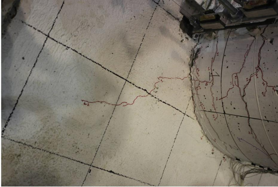
Figure 142. Photo. Specimen SF-3: radial footing crack propagation in cycle 6-2 (+2.48/-2.48 target drift ratio).
