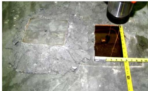
**c) Punching failure surface**
