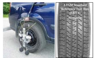
Figure 23. OBSI dual probe system and the SRTT.
