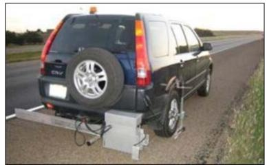
Figure 25. High-speed inertial profiler mounted behind the test vehicle.
