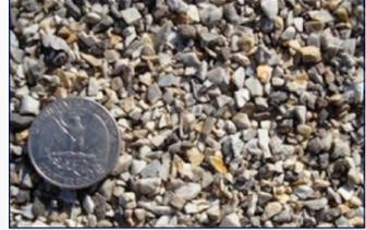
**FIGURE 5:** Close-up of typical aggregate used as surface topping showing angularity and size.
