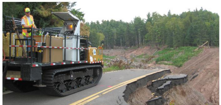
Track-mounted cone penetration testing (CPT) rig preparing to investigate embankment failure.
