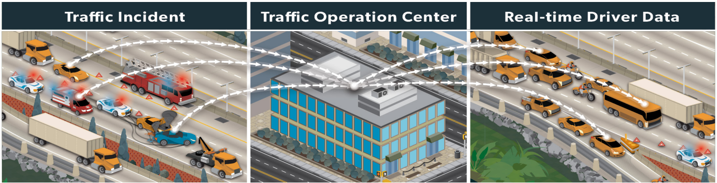
Real-time crowdsourced data from motorists supports operations by expediting notification of events such as crashes and unexpected congestion.
