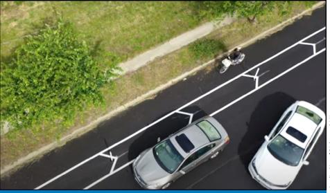
This design uses parking as an additional layer of separation between traffic and bike lanes.
